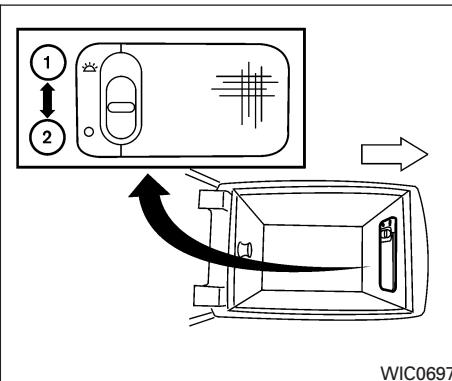
The light inside the rear center console box may be turned on ① and off ② with the switch.
