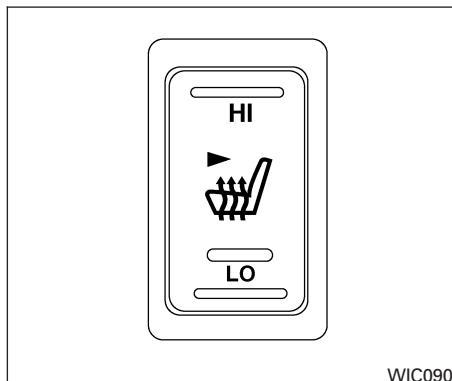
The front and rear seats are warmed by built-in heaters (if so equipped). The switches are located on the center consoles.
