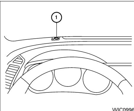
**Be sure you do not put anything on top of the autelight sensor ① located in the top side of the instrument panel. The autelight sensor controls the autelight; if it is covered, the autelight sensor reacts as if it is dark out and the headlights will illuminate. If this occurs while parked with the engine off and the key in the ON position, your vehicle's battery could become discharged.**
