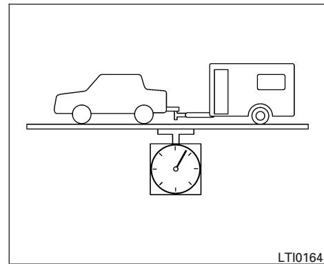
The Gross Combined Weight Rating (GCWR) equals the combined weight of the towing vehicle (including passengers and cargo) plus the total trailer load. Towing loads greater than these or using improper towing equipment could adversely affect vehicle handling, braking and performance.
