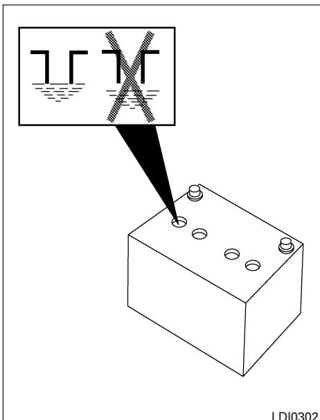
Vehicles operated in high temperatures or under severe conditions require frequent checks of the battery fluid level.
