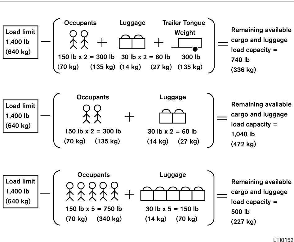
Steps for determining correct load limit
