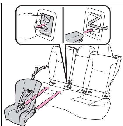
3 If the child restraint has a top strap, follow the child restraint manufacturer's operation manual regarding the installation, using the top strap to latch onto the top tether anchorage. (→P.64)
