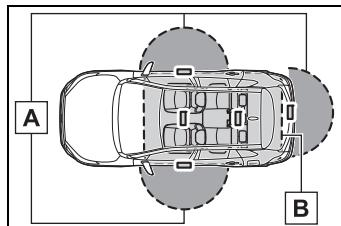
[A] When locking or unlocking the doors
