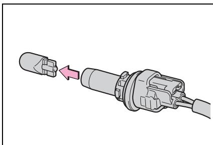
5 When installing the light bulb, install it by conducting steps 4 and 3 with the directions reversed.
