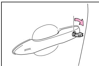
If a door is unlocked using the mechanical key while the alarm is set, a warning will sound intermittently for approximately 10 seconds. If the alarm is not canceled or stopped during this time, the warning pattern changes and the warning sounds for a certain period of time.
