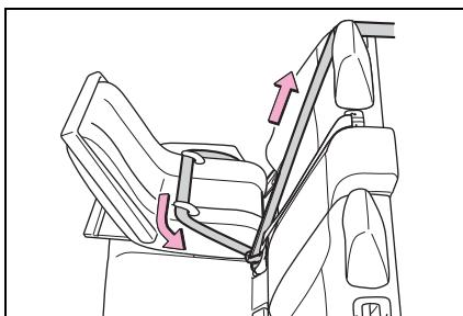
5 After installing the child restraint system, rock it back and forth to ensure that it is installed securely. (→P.58)
