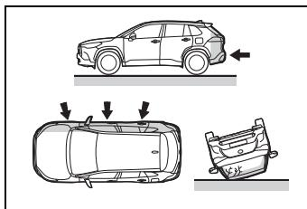
**■ The SRS airbags deploy in an underside impact when**
