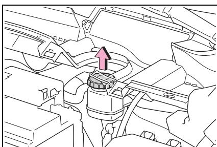
4 Add brake fluid slowly while checking the fluid level.
