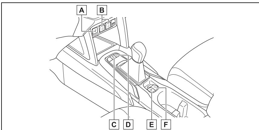
**A** **Heated steering wheel switch\* ..... P.308**
