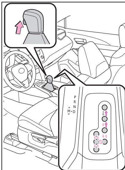
←: While the engine switch is in ON and the brake pedal depressed\*, shift the shift lever
