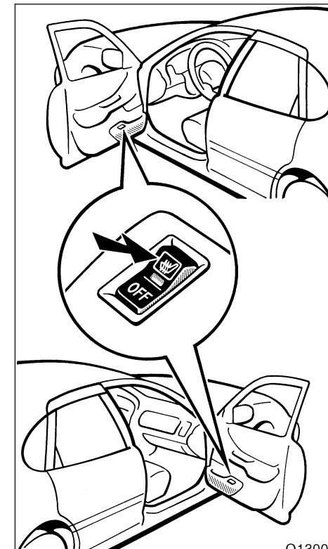
To turn on the seat heater, push the switch.
