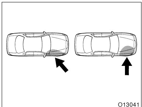
There may be the case that the SRS side airbags will not activate with such an impact in which the occupant wearing the seat belt correctly would not get serious injury.
