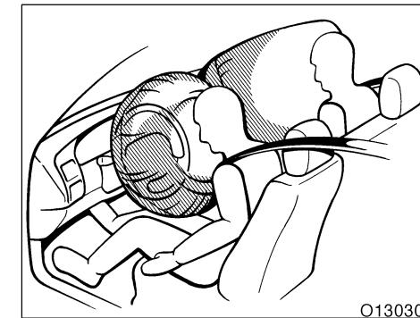
The **SRS (Supplemental Restraint System)** airbags are designed to provide further protection for occupants in the following seats when added to the primary protection provided by the seat belts.
