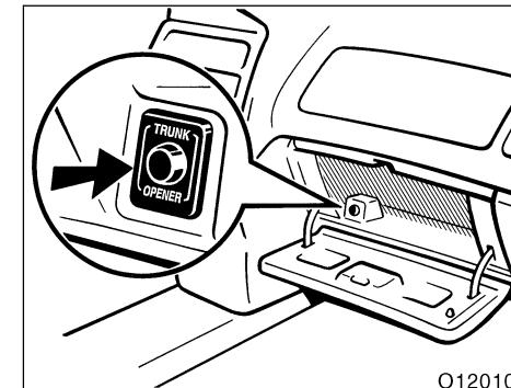
**To open the trunk lid from the driver's seat, push the lock release button in the glove box.**
