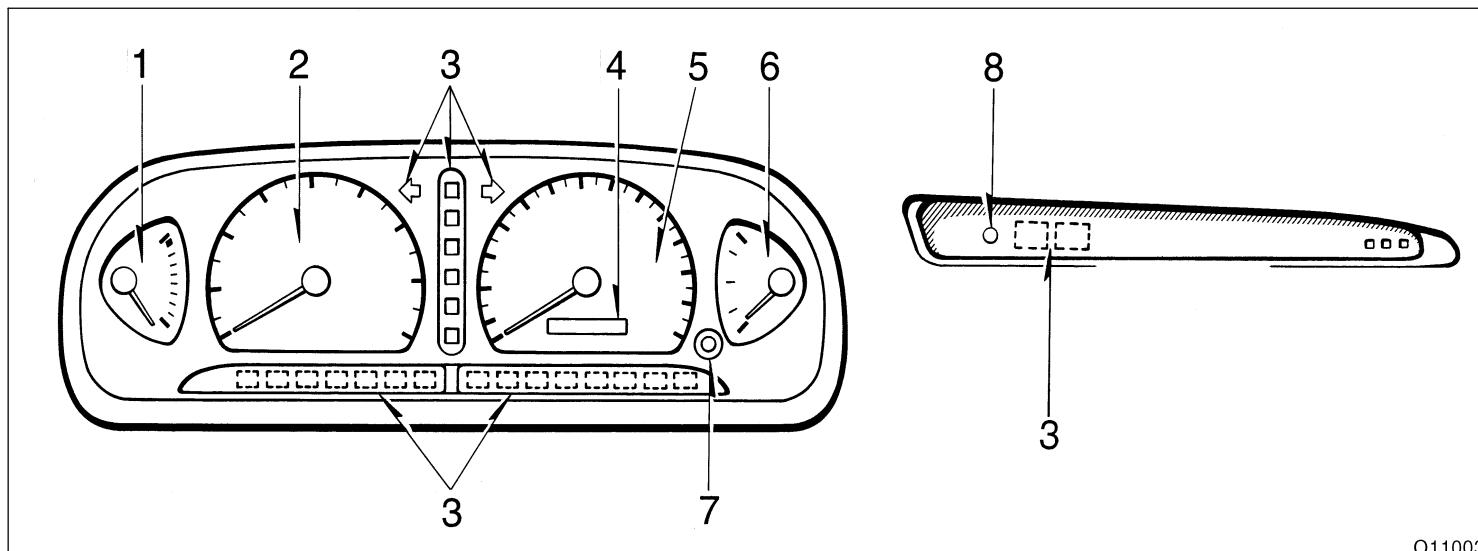
1. Engine coolant temperature gauge
