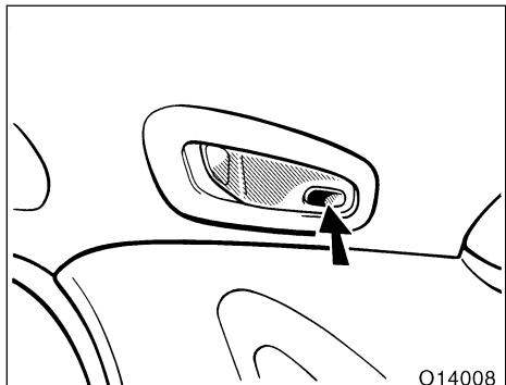
To turn on the rear personal light, push the switch. To turn the light off, push the switch once again.
