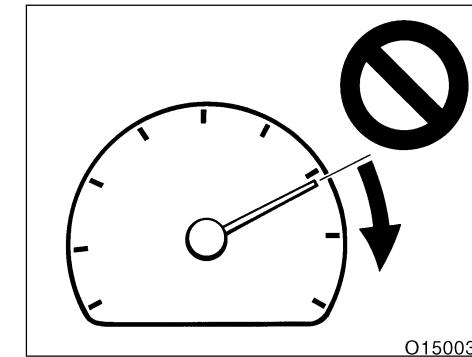
The tachometer indicates engine speed in thousands of rpm (revolutions per minute). Use it while driving to select correct shift points and to prevent engine luggering and overrevving.
