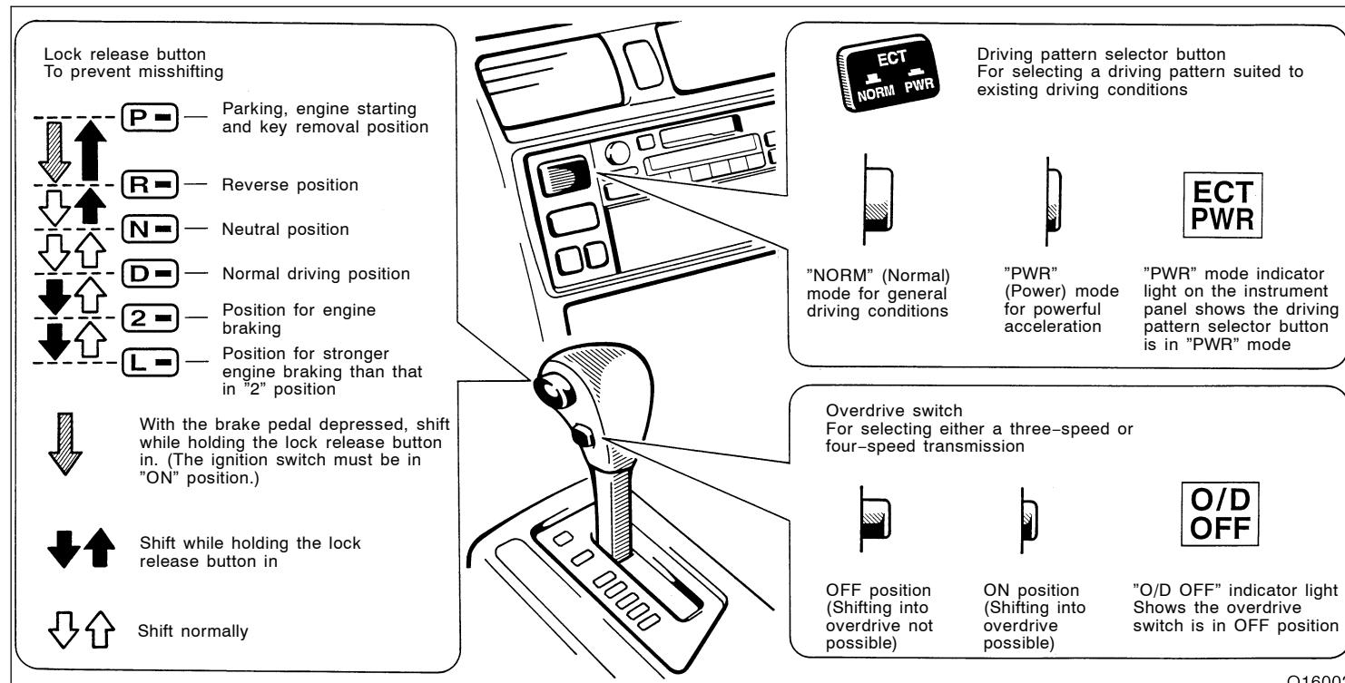
When the cruise control is being used, even if you downshift the transmission by turning off the overdrive switch, engine braking will not be applied because the cruise control is not cancelled. For ways to decrease the vehicle speed, see "Cruise control" in this chapter.
