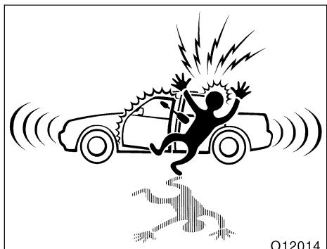
**To deter the vehicle theft, The system is designed to give an alarm if any of the doors, trunk or hood is forcibly unlocked or the battery terminal is disconnected and then reconnected when the vehicle is locked.**
