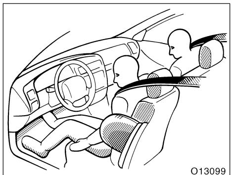
The SRS (Supplemental Restraint System) side airbags are designed to provide further protection for occupants in the following seats when added to the primary protection provided by the seat belts.
