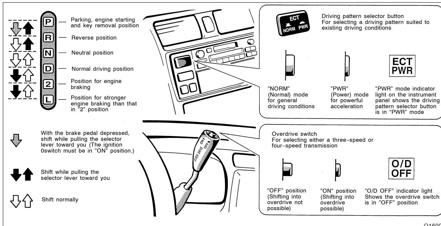
When the cruise control is being used, even if you downshift the transmission by turning off the overdrive switch, engine braking will not be applied because the cruise control is not cancelled. For ways to decrease the vehicle speed, see "Cruise control" in this chapter.
