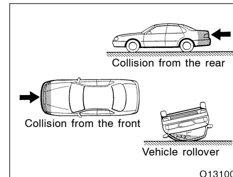
The SRS side airbags are not designed to inflate if the vehicle is subjected to a front or rear impact, if it rolls over, or if it is involved in a low-speed side collision.
