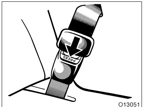
3. To remove the convertible seat, press the buckle-release button and allow the belt to retract completely. The belt will move freely again and be ready to work for an adult or older child passenger.
