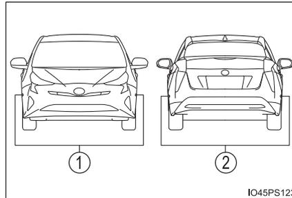
● The sensor detection range when using back-in parking assist mode
