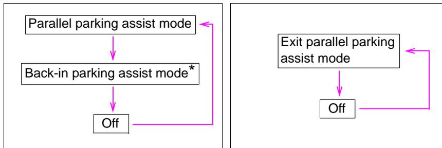
\*: The back-in parking assist mode can be switched to when its operating conditions are met (→P. 367). When the operating conditions are not met, it switches to off.
