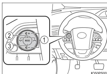
Cursor switch (CD, MP3/WMA disc, Bluetooth<sup>®</sup>, iPod or USB mode)
