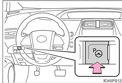
While the power switch is on, the vehicle speed is approximately 19 mph (30 km/h) or less, each time the S-APGS switch is pressed the function switches as follows.
