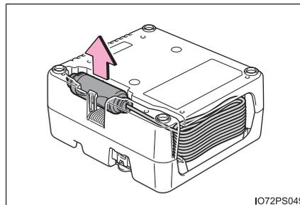
8 Connect the power plug to the power outlet socket. (→P. 541)
