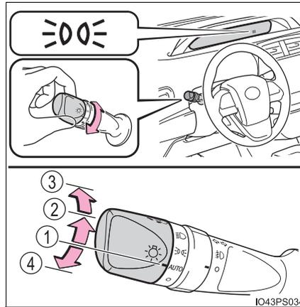
**Turning on the high beam headlights**
