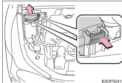
► Engine compartment type B fuse box
