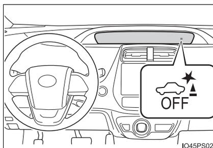
When the Intelligent Clearance Sonar function is switched OFF, system operation does not resume until the function is switched back ON through the settings screen on the multi-information display. (System operation does not resume by operating the power switch.)
