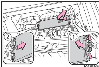
**6** Remove the filter case.
