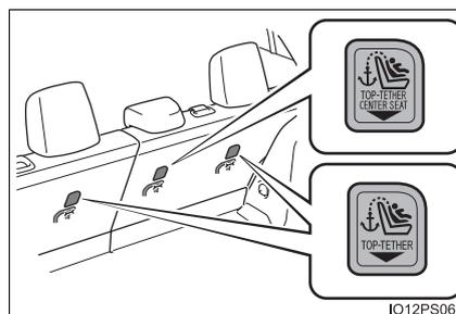
**■ Fixing the top tether strap to the anchor bracket**
