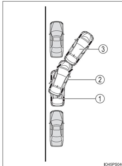
Depending on the condition of the parking space, guidance to starting points for moving forward and backing up, as well as the steering wheel auto operation, are repeated any time multi-turn maneuvering is necessary from the time the steering wheel auto operation begins in step ② up until the vehicle reaches a position from which it can take off.
