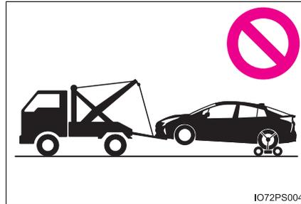
**Towing with a wheel-lift type truck**
