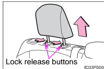
■ **Installing the head restraints**
