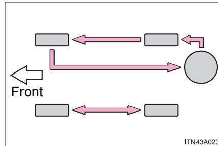
To equalize tire wear and extend tire life, Toyota recommends that tire rotation is carried out at the same interval as tire inspection.
