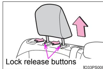
**■ Installing the head restraints****▶ Front and rear center seats**
