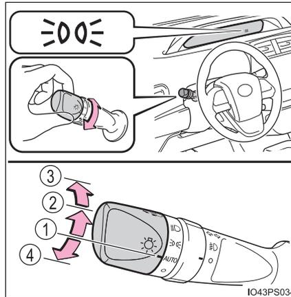
**Turning on the high beam headlights**
