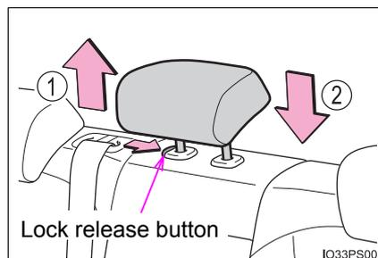
**■ Removing the head restraints****▶ Front and rear center seats**
