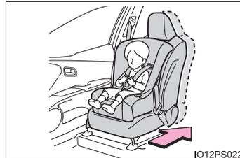
If the head restraint interferes with the child restraint system installation and the head restraint can be removed, remove the head restraint.
