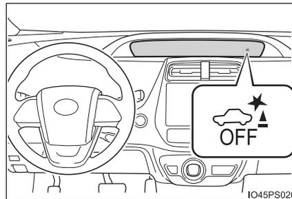
When the Intelligent Clearance Sonar function is switched OFF, system operation does not resume until the function is switched back ON through the settings screen on the multi-information display. (System operation does not resume by operating the power switch.)
