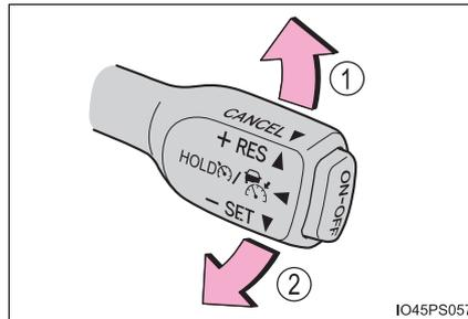
Large adjustment: Hold the lever in the desired direction.
