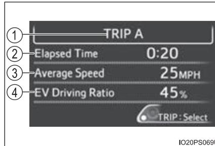
For the displayed distance of the mileage display, the percent traveled using only electric motor power is displayed.
