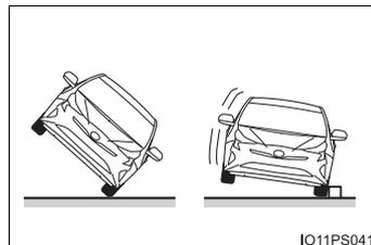
**■ Types of collisions that may not deploy the SRS airbags (SRS front airbags)**
