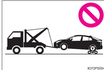
**Towing with a wheel-lift type truck**
