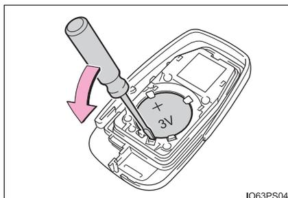
**4** When installing, reverse the steps listed.**■ Use a CR2032 lithium battery**
