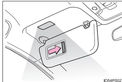
If the vanity light remain on when the power switch is turned off, the light will go off automatically after 20 minutes.
