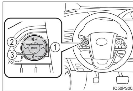
Cursor switch (CD, MP3/WMA disc, Bluetooth<sup>®</sup>, iPod or USB mode)
