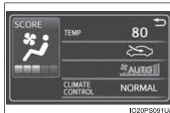
● The pop-up display function that displays when the air conditioning settings are changed using the air conditioning system switches can be turned off in the “Meter Customize” settings. (→P. 142)
