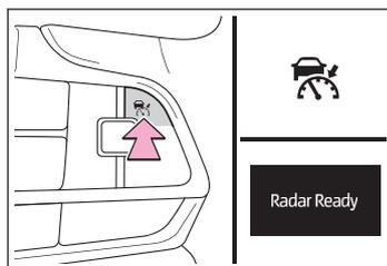
If the cruise control main switch is pressed and held for 1.5 seconds or more, the system turns on in constant speed control mode. (→ P.385)
