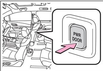
Pressing the switch again while the power sliding door is operating will cause the operation to stop.
