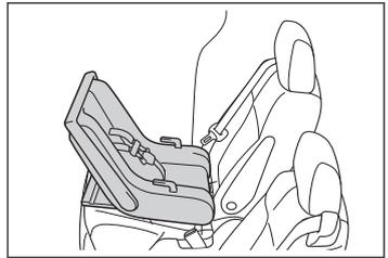
**3 Run the seat belt through the child restraint system and insert the plate into the buckle. Make sure that the belt is not twisted.**
