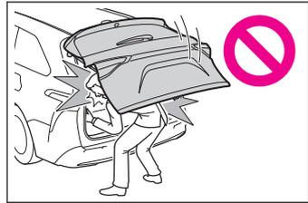
Vehicles with power back door: The back door may suddenly shut if it is not opened fully, while on a steep incline. Make sure that the back door is secured before using the luggage compartment.
