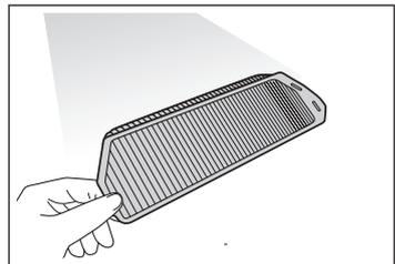
**7 Reinstall the filter to the cover.**
