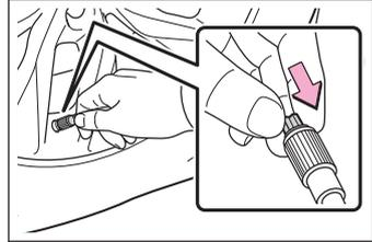
3. Disconnect the hose from the valve, remove the air release cap from the hose and then reconnect the hose.
