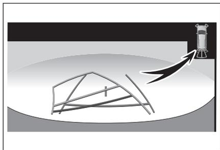
A simplified image is displayed on the upper corner of the screen when an obstacle is detected.
