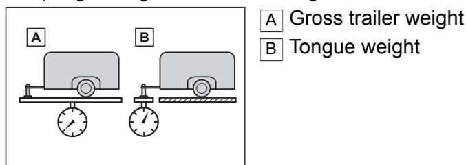
The gross trailer weight, gross axle weight and tongue weight can be measured with platform scales found at a highway weighing station, building supply company, trucking company, junk yard, etc.
