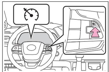
Switching to constant speed control mode is only possible when operating the switch with the cruise control off.
