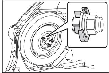
**2 Firmly tighten each wheel nut two or three times in the order shown in the illustration.**
