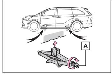
The jack point guides are located on the side of rocker moulding. They indicate the jack point positions.
