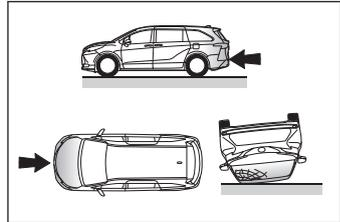
The SRS curtain shield airbags do not generally inflate if the vehicle is involved in a rear collision, if it pitches end over end, or if it is involved in a low-speed side or low-speed frontal collision.
