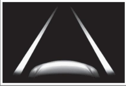
Indicates that the system is recognizing white (yellow) lines or a course\*<sup>1</sup>. When the vehicle departs from its lane, the white line displayed on the side the vehicle departs from flashes orange.
