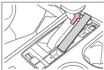
6. Press and hold the shift lock override button and then push the button on the shift knob.
