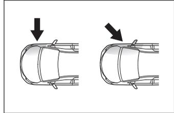
The SRS side airbags do not generally inflate if the vehicle is involved in a frontal or rear collision, if it rolls over, or if it is involved in a low-speed side collision.
