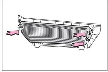
**8 Install the air intake vent cover.**
