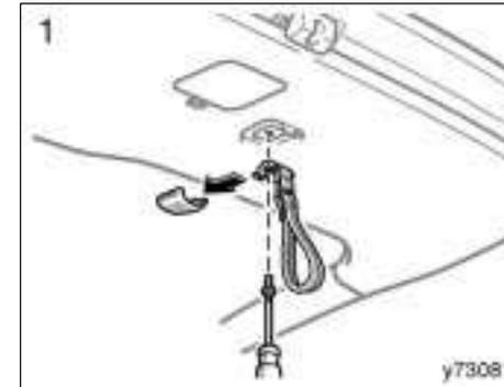
Remove the strap with a Phillips-head screwdriver.
