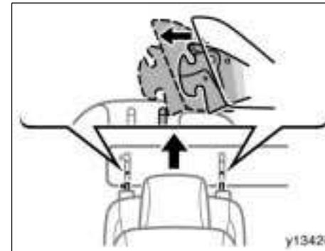
You can easily align the front leg hooks with the rear strikers by using the floor bezel. Put the front legs of the seat short of the rear strikers as shown in the illustration. Then slide the seat forward along the groove of the bezel until the front legs will reach the striker. Make sure the front legs align with the striker, swing up the seat.
