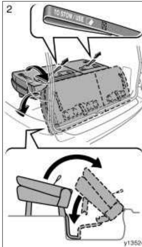
2. Pull and hold the seat lock release strap ("TO STOW/USE" printed on its surface) and lift up the seat rearward. Then push the seat down.
