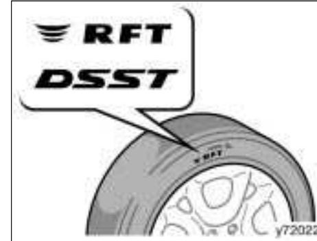
Some vehicles are equipped with run-flat (RFT) tires. The run-flat tire allows you to continue driving for up to 160 km (100 miles) at a speed below 90 km/h (55 mph) even if any tire goes flat. However, in some conditions (such as high temperatures), you could not continue driving for up to 160 km (100 miles).
