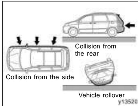
The SRS front airbags are not generally designed to inflate if the vehicle is involved in a side or rear collision, if it rolls over, or if it is involved in a low-speed frontal collision. But, whenever a collision of any type causes sufficient forward deceleration of the vehicle, deployment of the SRS front airbags may occur.
