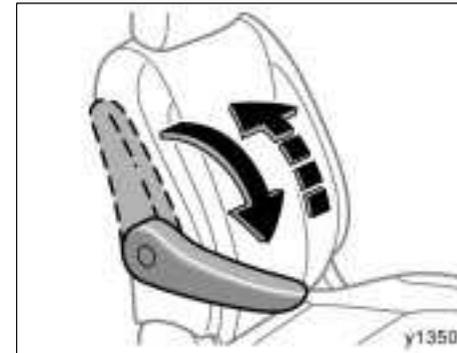
To adjust the armrest, lower the armrest to the lowest position and raise it to the desired angle. Raising the armrest to the highest position unlocks the armrest to let you return it to the lowest position.
