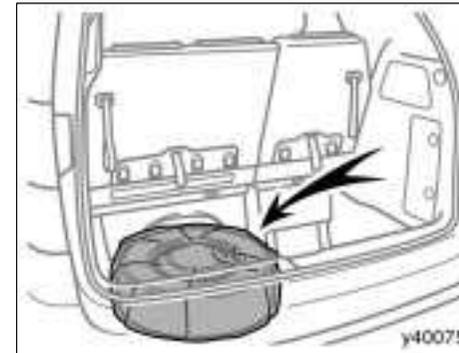
**13. Wrap the flat tire in the tire bag and stow temporarily in the luggage compartment. The tire bag is stored with the jack handle.**
