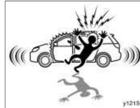
To deter the vehicle theft, the system is designed to sound an alarm if any of the side doors, back door or hood is forcibly unlocked or opened or the battery terminal is disconnected and then reconnected when the vehicle is locked.
