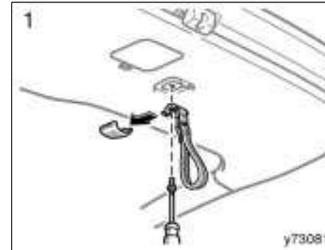
Remove the strap with a Phillips-head screwdriver.
