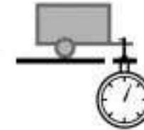
$$\frac{\text{Tongue load}}{\text{Total trailer weight}} \times 100 = 9 \text{ to } 11\% \text{ }^{(*1)}$$
