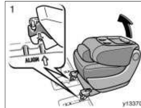
1. Align the front leg hooks with the rear strikers in the floor. Then swing up the seat.
