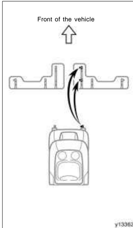
When you install the second seats, be sure to place it where the seat is originally positioned because each second seat is not interchangeable. You can distinguish the original seat position by the position of the front seat leg pin and the shape of the seat striker bezel in the floor.
