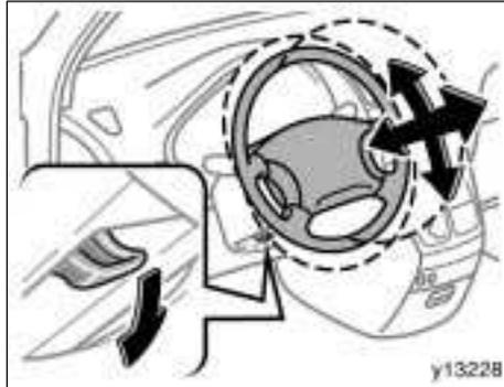
To adjust the steering wheel position, push down the lock release lever. Then tilt the steering wheel to the desired angle, push or pull it to the desired steering column length and pull up the lock release lever.
