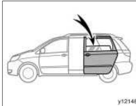
When the sliding door window is opened more than about 15 cm (6 in.), the sliding door will stop at half-opened position for safety reasons. Close the window and then operate the sliding door.
