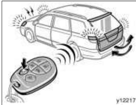
**Push and hold the back door open switch on the wireless remote control transmitter for about one second. The power back door opens and closes completely.**
