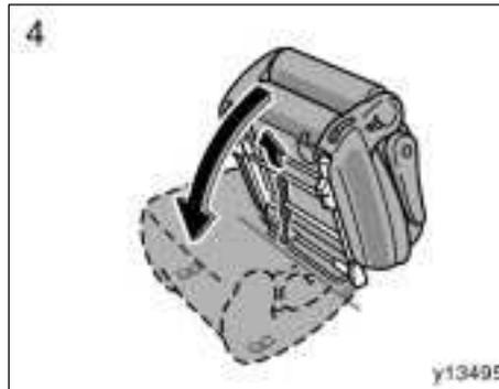
4. Pull and hold the front leg release strap and fold down the seat. Then the front leg locks will disengage and you can remove the seat.
