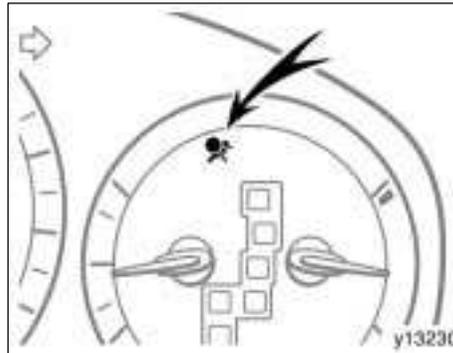
This indicator comes on when the ignition switch is turned to the "ON" position. It goes off after about 6 seconds. This means the SRS side airbags and curtain shield airbags are operating properly.
