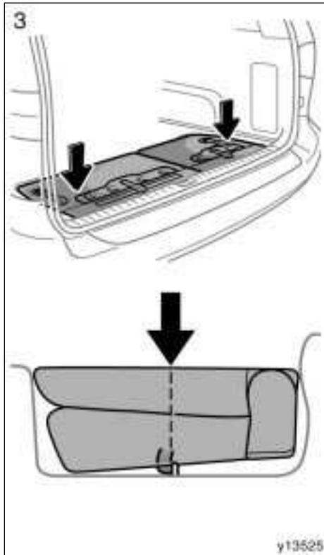
3. Push the seat against the floor and make sure it is locked securely.
