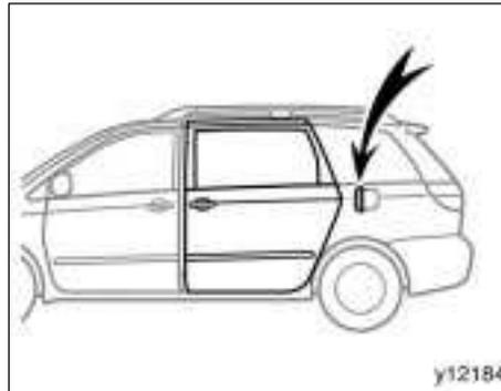
When the fuel filler door is opened, the left side sliding door will not open. Close the fuel filler door securely and then operate the sliding door.
