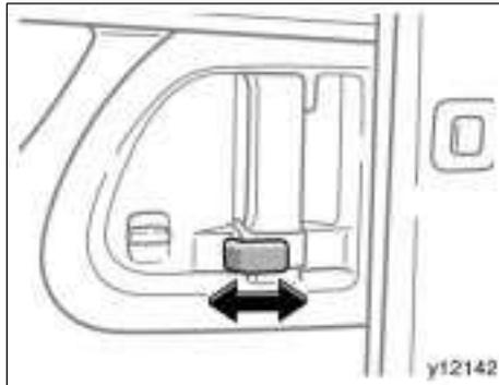
**LOCKING AND UNLOCKING WITH INSIDE LOCK KNOB**
