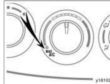
For quick cooling, turning the temperature selector knob fully towards COLD changes the air intake selector mode to RECIRCULATE. It is not possible to return to FRESH and to turn the air conditioning system off in this position.
