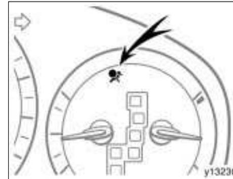
This indicator comes on when the ignition switch is turned to the "ON" position. It goes off after about 6 seconds. This means the SRS front airbags are operating properly.
