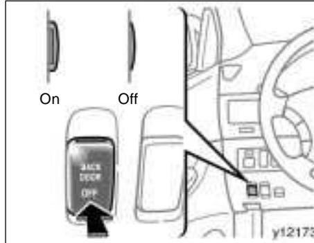
This switch is used to turn on and off the power back door system. In order to operate the power back door, the “BACK DOOR OFF” switch on the instrument panel must be pushed out. (The orange line on top of the switch indicates that the power back door system is on.) To disable the power back door feature, push in the switch.
