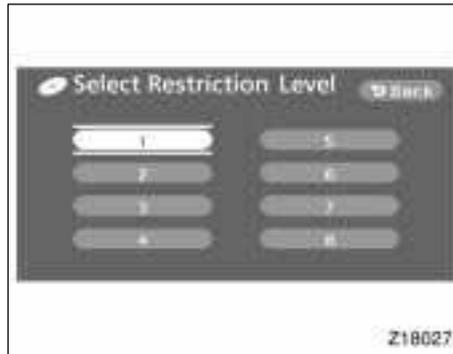
Push a parental level (1—8). The smaller the level number, the stricter the age limit. Push the “Back” switch to return to the “Setup Menu” screen.
