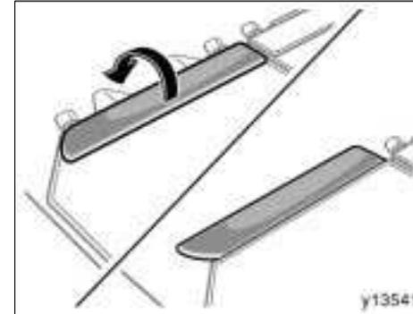
After stowing the seats, open the flaps as shown in the illustration.
