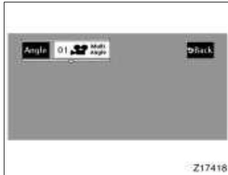
The angle can be selected for discs that are multi-angle compatible when the “
