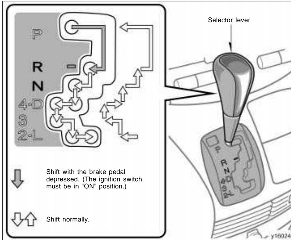
Your automatic transmission has a shift lock system to minimize the possibility of incorrect operation. This means you can only shift out of "P" position when the brake pedal is depressed (with the ignition switch in the "ON" position).
