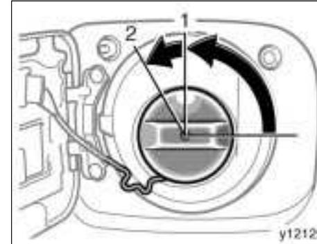
2. To remove the fuel tank cap, turn the cap counterclockwise by 90 degrees (to the pressure point 1), and then turn it an additional 30 degrees (to point 2). Pause slightly before removing it.
