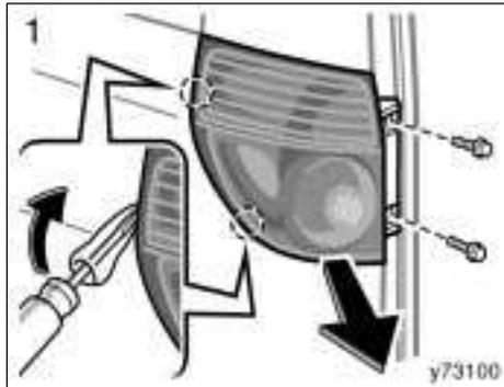
Remove the bolts. Remove the unit by pry the unit by using the flathead screwdriver with cloth.
