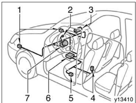
The SRS airbag system mainly consists of the following components, and their locations are shown in the illustration.
