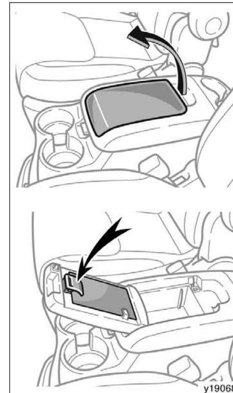
The note pad holder is designed to hold small paper such as note pads.
