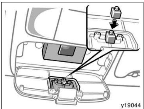
If the center panel does not contact your garage door opener transmitter:
