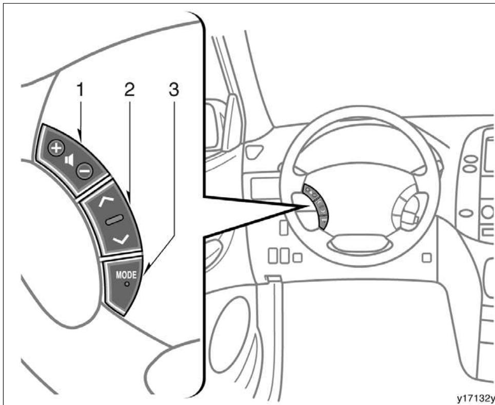
Some parts of the audio system can be adjusted using the switches on the steering wheel.
