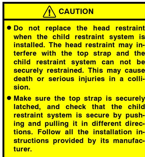
—Installation with child restraint lower anchorages (for second seats)
