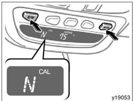
2. Push and hold both the "MODE" and "E/M" buttons simultaneously for 10 seconds until the "CAL" indication appears on the compass display. (At this time, the compass display is locked in "N".)
