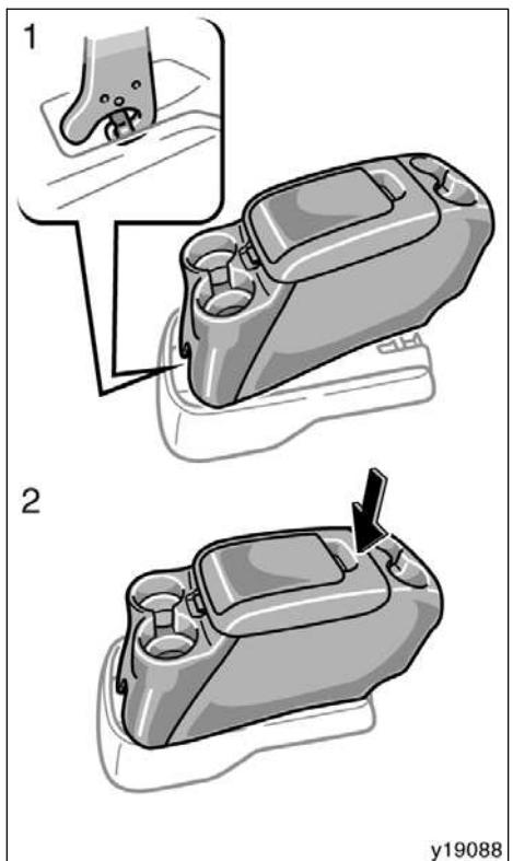
To install the console box between the front seats:
