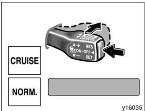
However, once the vehicle-to-vehicle distance control mode activates and is used, it cannot be changed to the conventional cruise control mode using the above operation. To change the mode, press the "ON-OFF" button to turn the system off and then press it again to turn it on. Next push the lever in the "MODE" direction for longer than about 1 second.
