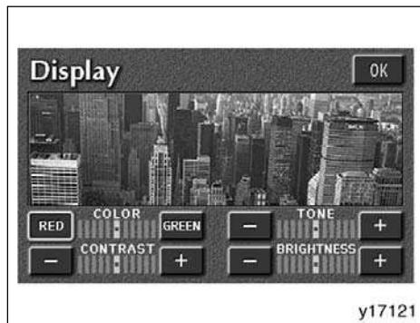
After adjusting the screen, push the "OK" switch to return to the previous screen.
