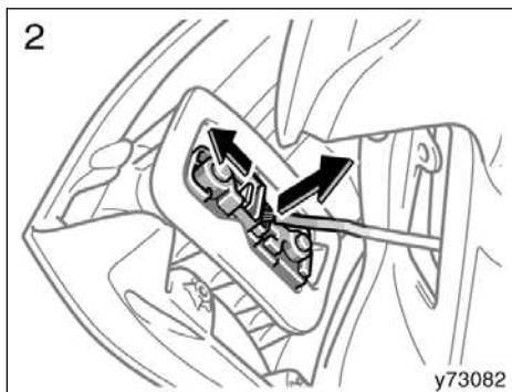
Pull and hold the tab and remove the
