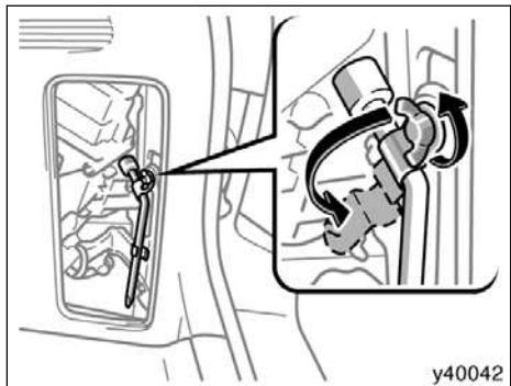
To remove the wheel nut wrench, turn the wingnut counterclockwise.
