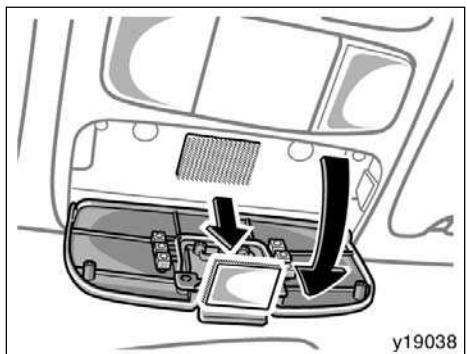
**The box is designed to store a garage door opener transmitter.**
