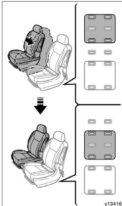
7-passenger models only: The right side seat can be moved to the inside when the console box is not installed between the second seats.
