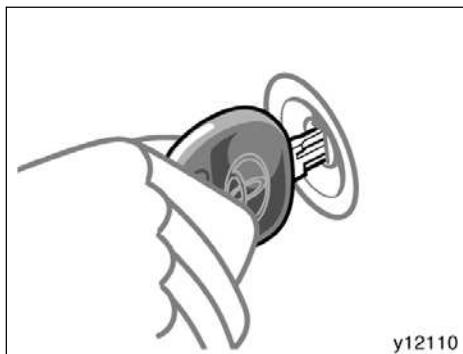
The engine immobilizer system is a theft prevention system. When you insert the key in the ignition switch, the transponder chip in the key's head transmits an electronic code to the vehicle. The engine will start only when the electronic code in the chip corresponds to the registered ID code for the vehicle.
