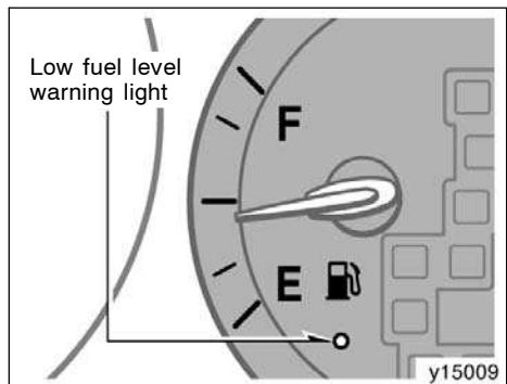
**The gauge indicates the approximate quantity of fuel remaining in the tank when the ignition switch is on.**
