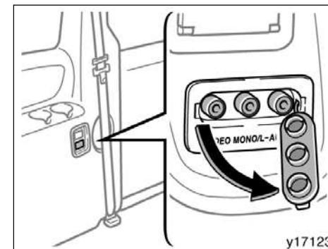
To use the input terminal adapter, open the cover.
