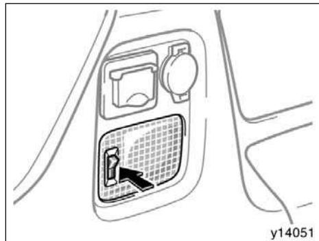
To turn on the luggage compartment light, push the luggage compartment light switch upwards. The light turns on when the personal light main switch is in the "ON" or "DOOR" position.
