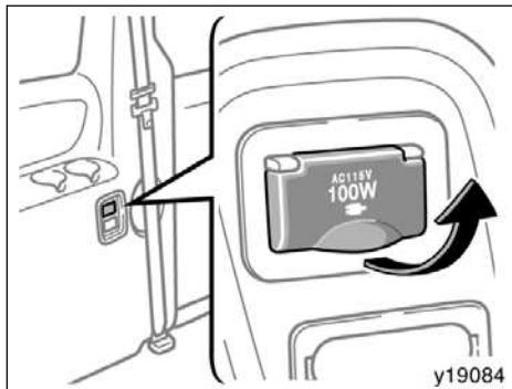
This power outlet is designed for use as a power supply for the audio device connected to the input terminal adapter.
