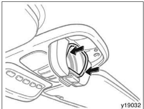
The mirror angle can be adjusted by pushing its edge.
