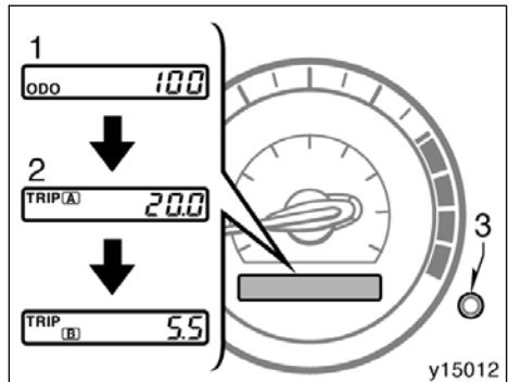
**This meter displays the odometer and two trip meters.**
