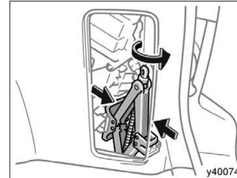
To remove the jack, turn the jack joint by hand until the jack becomes free.
