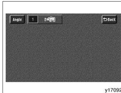
The angle can be selected for discs that are multi-angle compatible when the "CAM" mark appears on the screen. Each time you push the "Angle" switch, the angle changes. The angle number which you can select will appear on the screen.
