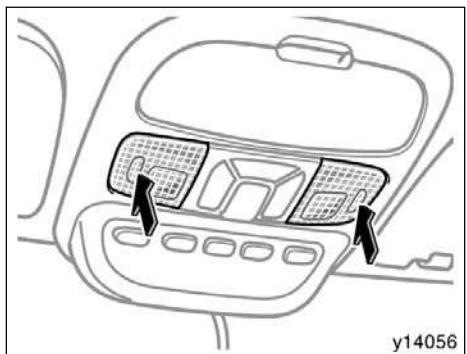
To turn on the front personal lights, operate the personal light main switch. The lights can be turned on or off by pushing each lens when the personal light main switch is in the "DOOR" or "OFF" position.
