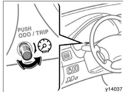
To adjust the brightness of the instrument panel lights, turn the knob.
