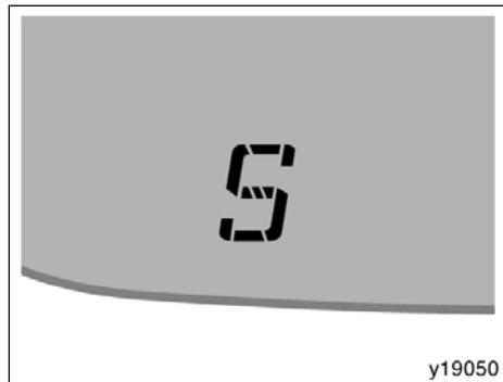
**The compass indicates the direction that the vehicle is heading. In the above case, it shows that the vehicle is heading south.**
