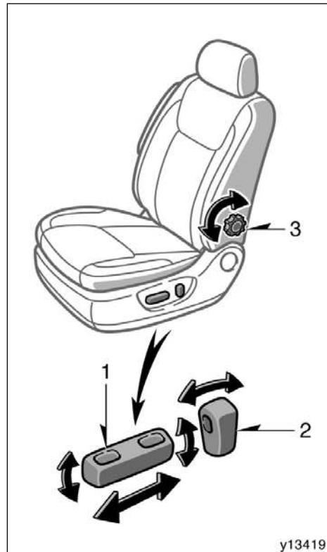
**1. SEAT POSITION, SEAT CUSHION ANGLE AND SEAT HEIGHT ADJUSTING SWITCH**
