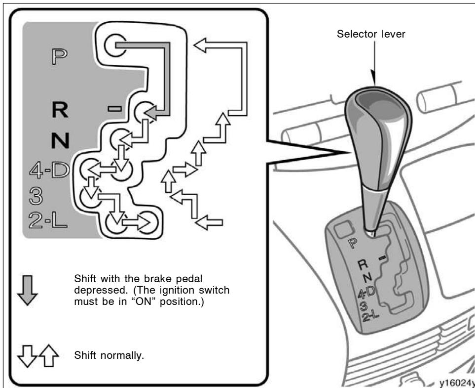
Your automatic transmission has a shift lock system to minimize the possibility of incorrect operation. This means you can only shift out of "P" position when the brake pedal is depressed (with the ignition switch in "ON" position).
