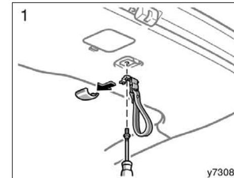
Remove the strap with a Phillips-head screwdriver.
