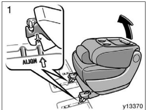
1. Align the front leg hooks with the rear strikers in the floor. Then swing up the seat.
