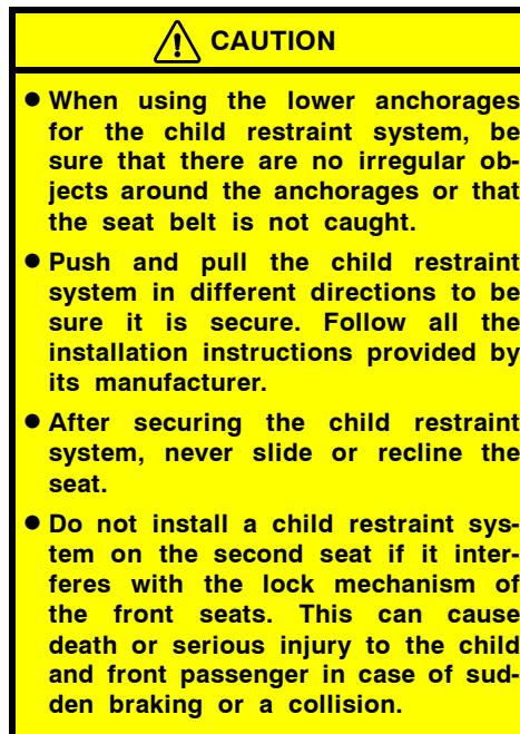
—Installation with child restraint lower anchorages (for third seats)
