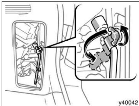
To remove the wheel nut wrench, turn the wingnut counterclockwise.
