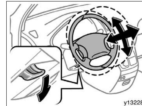
To adjust the steering wheel position, push down the lock release lever. Then tilt the steering wheel to the desired angle, push or pull it to the desired steering column length and pull up the lock release lever.
