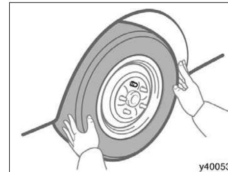
6. After making sure that no one is in the vehicle, raise it high enough so that the spare tire can be installed.
