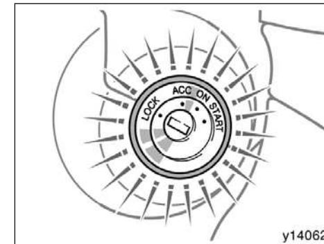
For easy access to the ignition switch, the ignition switch light comes on when any of the side doors and back door is opened or when the ignition switch is turned to the "LOCK" position.
