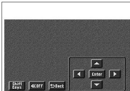
To select the menu for the disc, push the "◀", "▲", "▶" or "▼" switches on the screen. Push the "Enter" switch to select the menu for the disc.
