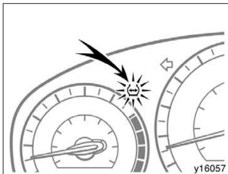
When initializing the system, make sure the low tire pressure warning light blinks three times. If the warning light does not blink three times, initializing will be failed and the tire pressure warning system will not function properly.
