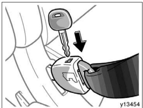
To release the concave end tab, insert the key into the hole on buckle 1 and allow the belt to retract.
