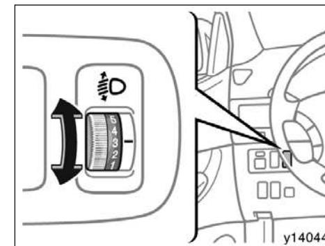
**To adjust the headlight beam level, turn the dial.**
