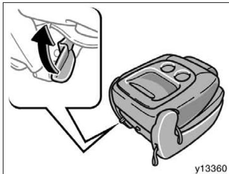
If you lock the rear legs before the front legs are not lock securely, disengage the rear leg lock by pulling the rear leg release lever. Then reinstall the seat following the correct procedure.
