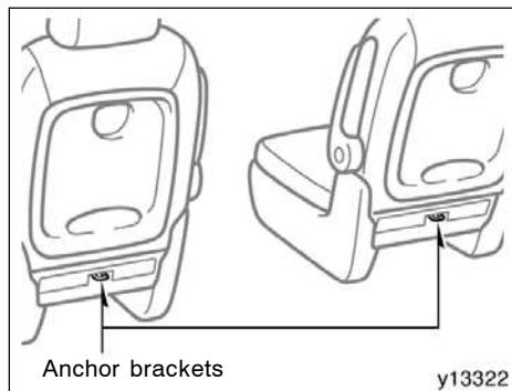
Use the anchor brackets on the back of the second seats to attach the top strap. Anchor bracket is installed for each second seating position.
