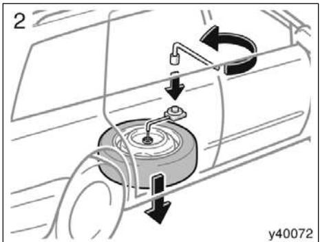
2. Loosen the spare tire clamp bolt by turning it counterclockwise with the wheel nut wrench.
