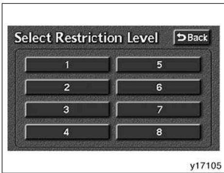
Push a parental level (1—8). The smaller the level number, the stricter the age limit. Push the "Back" switch to return to the "Setup Menu 1" screen.
