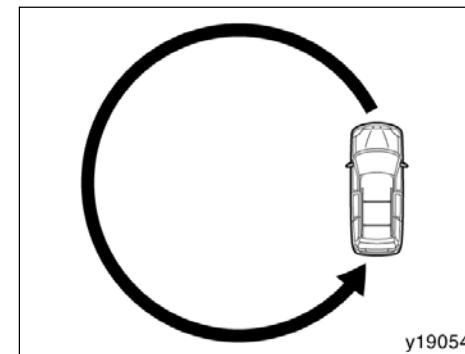
3. Drive the vehicle in a circle at 8 km/h (5 mph) or less. If there is not enough space to drive in a circle, drive around the block.
