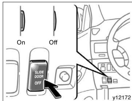
This switch is used to turn on and off the power sliding door system. In order to operate the power sliding door, the "SLIDE DOOR OFF" switch on the instrument panel must be pushed out. (The orange line on the top of the switch indicates that the power sliding door system is on.) To disable the power sliding door feature, push in the switch.
