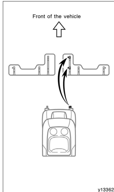
When you install the second seats, be sure to place it where the seat is originally positioned because each second seat is not interchangeable. You can distinguish the original seat position by the position of the front seat leg pin and the shape of the seat striker bezel in the floor.
