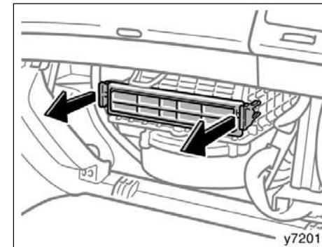
3. Remove the filter case from the filter outlet as shown in the illustration.
