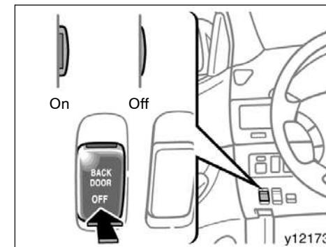
This switch is used to turn on and off the power back door system. In order to operate the power back door, the "BACK DOOR OFF" switch on the instrument panel must be pushed out. (The orange line on the top of the switch indicates that the power back door system is on.) To disable the power back door feature, push in the switch.
