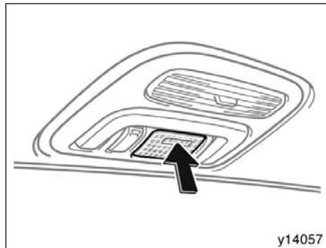
To turn on the rear personal lights, operate the personal light main switch. The lights can be turned on or off by pushing each lens when the personal light main switch is in the "DOOR" position.
