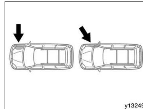
The SRS side airbag and curtain shield airbag system may not inflate if the vehicle is subjected to a collision from the side at certain angles, or a collision to the side of the vehicle body other than the passenger compartment as shown in the illustration.
