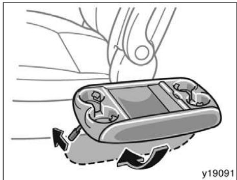
To fold down the table, pull up the lock release lever and push against the front passenger's seat side.
