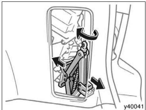
To store the jack, turn the jack joint until the jack base fits securely with the vehicle body.
