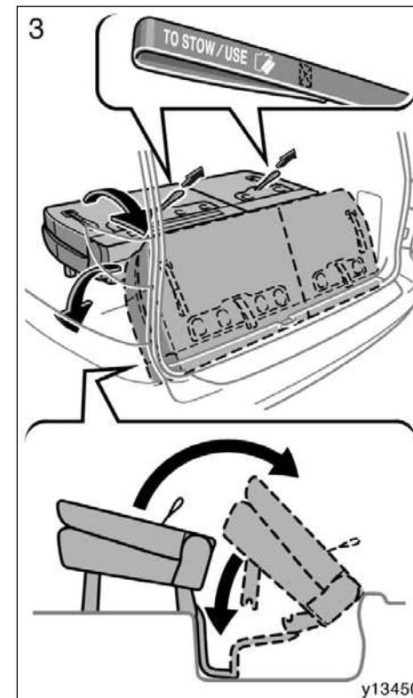
**3. Pull and hold the seat lock release strap ("TO STOW/USE" printed on its surface) and lift up the seat rearward. Then push the seat down.**
