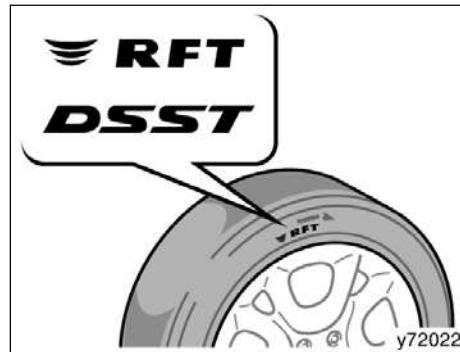
There is an "RFT" or "DSST" mark on the sidewall of the run-flat tire.
