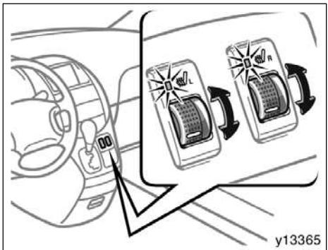
To turn on the seat heater, move the dial upward ("L" dial for the left front seat and "R" dial for the right front seat). At this time, the indicator light will illuminate to indicate the seat heater is operating.
