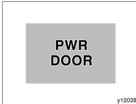
If you shift out of "P" when the power sliding door is opened or in the process of closing with the power sliding door system on, a buzzer will sound and the open power sliding door warning light will flash. This is a warning that the sliding door is not completely closed.
