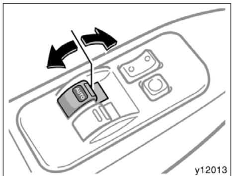
**The windows can be operated with the switch on each front door.**
