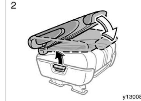
2. Lift the seatback angle adjusting lever and fold the seatback down.
