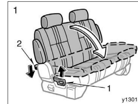
1. Lift the seatback angle adjusting lever (1) or press the lever (2) behind the seatback and fold the seatback down.
