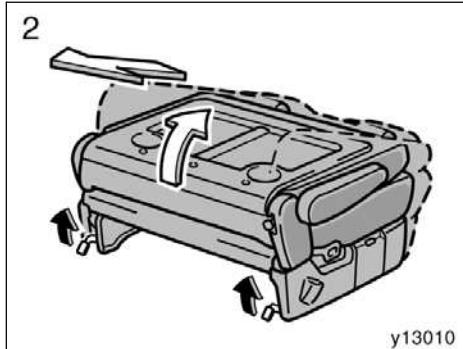
2. Pull the seat lock release lever. Lift the seat and remove the seat toward you.
