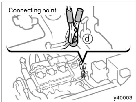
Do not connect the cable to or near any part that moves when the engine is cranked.
