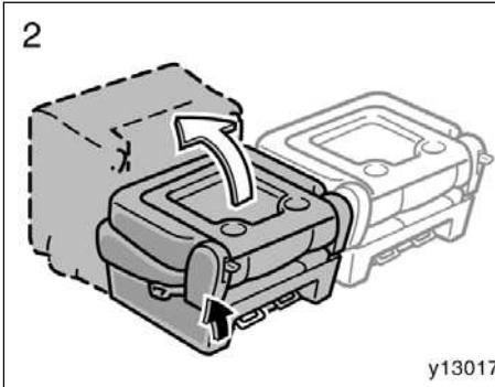
2. Remove the head restraint. Unlock the seat legs by pulling up the left side handle under the seat, and swing the whole seat up and forward.
