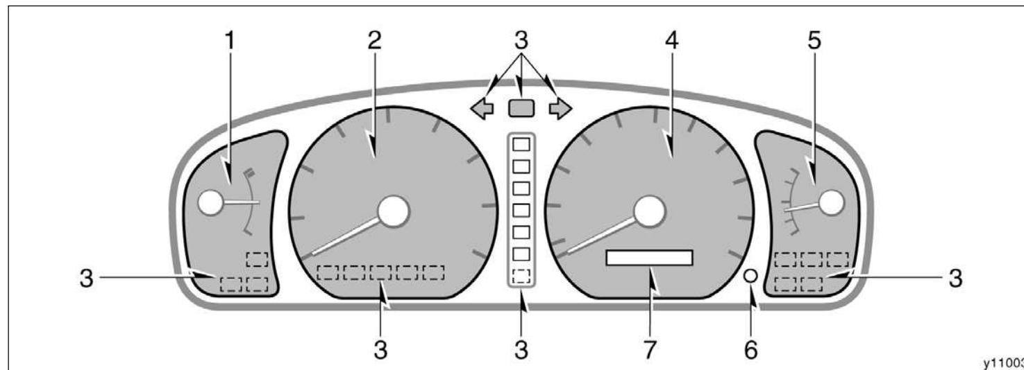
1. Engine coolant temperature gauge
