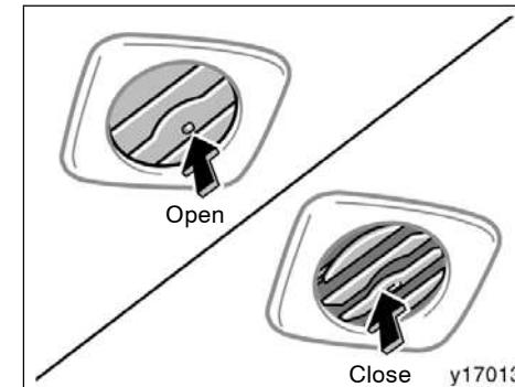
If air flow control is not satisfactory, check the roof vents. The roof vents may be opened or closed as shown.
