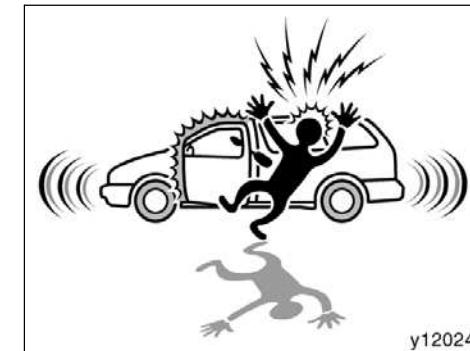
To deter the vehicle theft, the system is designed to give an alarm and keep the engine from being started if any of the front, sliding or back doors or hood is forcibly unlocked or the battery terminal is disconnected and then reconnected when the vehicle is locked.
