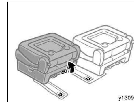
If the seat legs are locked in the wrong position, pull up the right side handle under the seat. Then lift and remove the seat.
