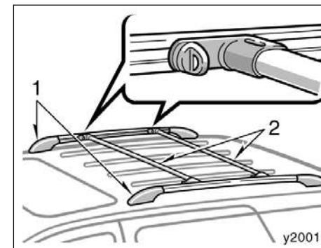
The roof luggage carrier consists of roof rails (1) attached to the roof and sliding crossrails (2).
