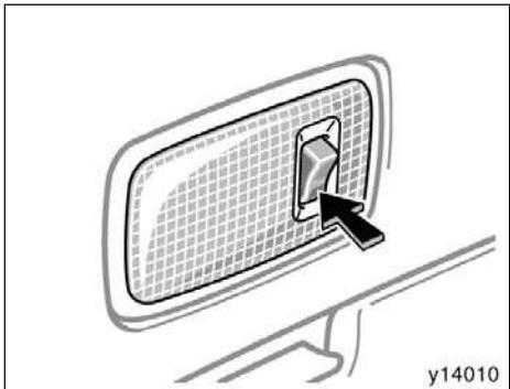
To turn the luggage compartment light on, open the back door and push the switch downwards. To turn it off, push the switch upwards or close the back door.
