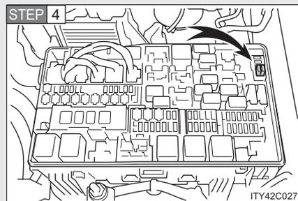
Remove the fuse with the pull-out tool.
