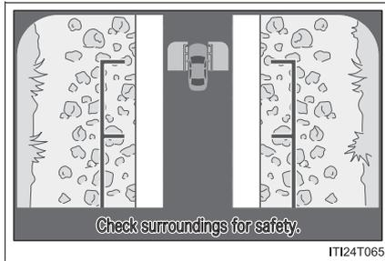
The image from both side cameras is displayed. Use this monitor to help check the area on both sides of the vehicle at the same time, and to check for objects near the tires or the sides of the vehicle. Guidelines showing an image of the vehicle width and the position of the front tires are displayed.
