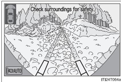
The image from the front camera is displayed. Use this monitor to help check the area in front of the vehicle for safety. Guidelines are shown to help determine the course.
