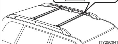
Slide the cross rails to the appropriate position for loading luggage and turn the knobs clockwise to tighten the cross rails securely.
