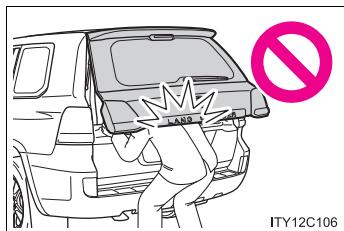
● The back door may fall if it is not opened fully. It is more difficult to open or close the back door on an incline than on a level surface, so beware of the back door unexpectedly opening or closing by itself. Make sure that the back door is fully open and secure before using the luggage compartment.
