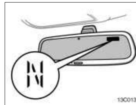
The compass indicates the direction in which the vehicle is heading. The illustration shown above indicates the vehicle is heading north.
