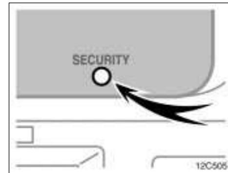
The engine immobilizer system is a theft prevention system. When you insert the key in the ignition switch, the transponder chip in the key's head transmits an electronic code to the vehicle. The engine will start only when the electronic code in the chip corresponds to the registered ID code for the vehicle.
