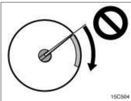
The tachometer indicates engine speed in thousands of rpm (revolutions per minute). Use it while driving to prevent engine over-revving.
