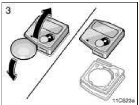
3. Open and remove the battery case cover using a coin. Remove the discharged battery and put in a new battery with the positive side up.
