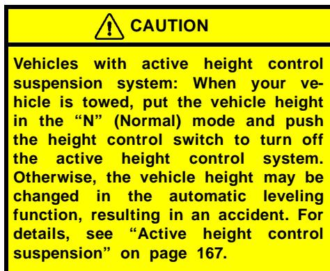
**(a) Towing with wheel lift type truck**
