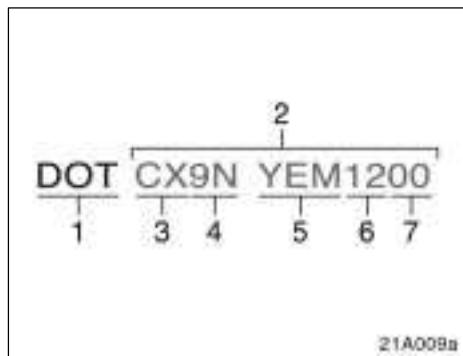
The “DOT” symbol certifies that the tire conforms to applicable Federal Motor Vehicle Safety Standards.
