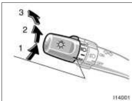
Manually twist the knob to the position 2 to turn on the headlights if they are needed immediately when entering a dark tunnel, parking structure, etc.
