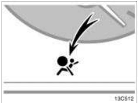
**The indicator comes on when the ignition key is turned to the "ON" position. It goes off after about 6 seconds. This means the SRS side airbags and curtain shield airbags are operating properly.**
