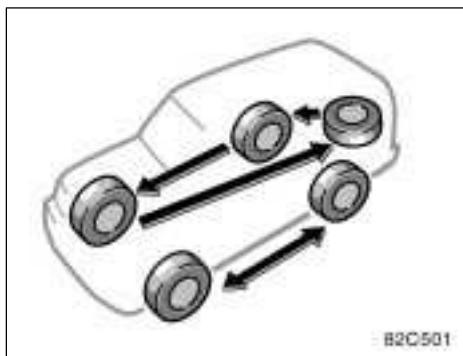
To equalize tire wear and help extend tire life, Toyota recommends that you rotate your tires according to the maintenance schedule. (For scheduled maintenance information, please refer to the "Scheduled Maintenance Guide" or "Owner's Manual Supplement".) However, the most appropriate timing for tire rotation may vary according to your driving habits and road surface conditions.
