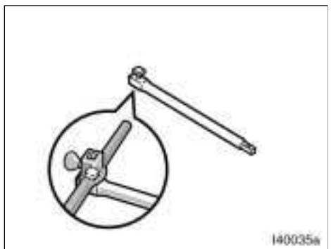
When connecting a jack handle extension with another extension and a jack handle end, use a jack handle to tighten the bolts on the joints as shown in the illustration. When connecting the jack handle with extension, tighten the wing bolt on the jack handle securely. Make sure the hollow meets the bolt on any joint when you tighten the bolts.
