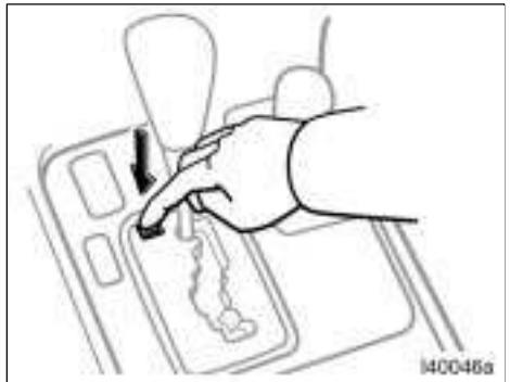
3. Insert your finger into the hole to push down the shift lock override button. You can shift out of "P" position only while pushing the button.
