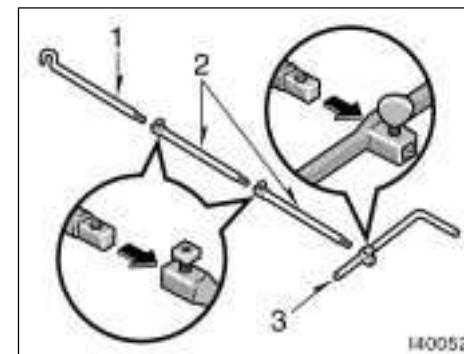
Put a jack handle, jack handle extensions, and jack handle end together as shown in the illustration.
