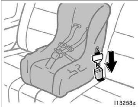
1. Run the center lap belt through or around the convertible seat following the instructions provided by its manufacturer and insert the tab into the buckle taking care not to twist the lap belt.
