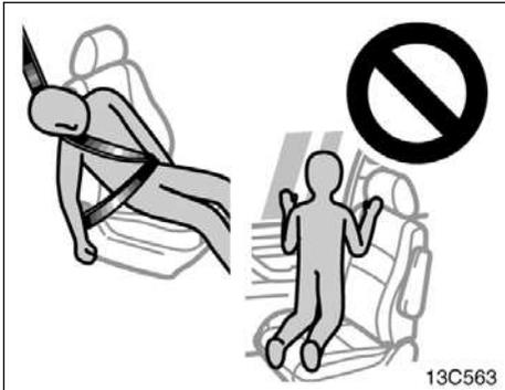
● Do not allow anyone to kneel on the passenger seat, facing the passenger's side door, since the side airbags and curtain shield airbags could inflate with considerable speed and force. Otherwise, he/she may be killed or seriously injured. Special care should be taken especially when you have a small child in the vehicle.
