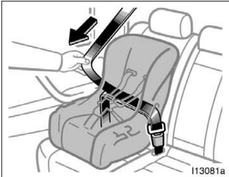
2. Fully extend the shoulder belt to put it in the lock mode. When the belt is then retracted even slightly, it cannot be extended.
