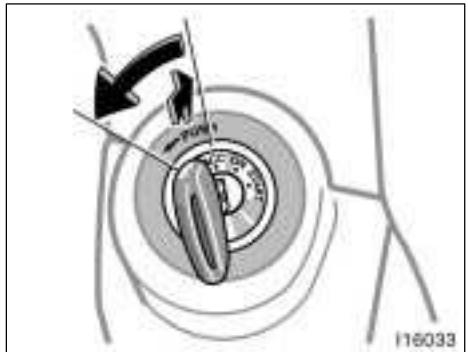
**"START"**—Starter motor on. The key will return to the "ON" position when released.
