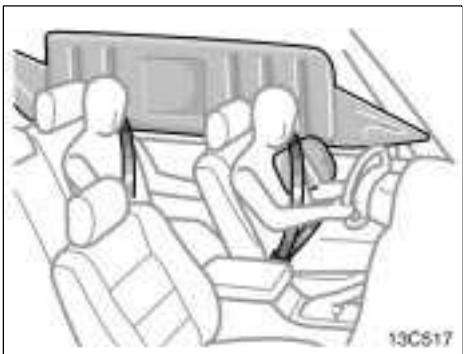
The SRS (Supplemental Restraint System) side and curtain shield airbags are designed to provide further protection for the driver, front and second seat passengers in addition to the primary safety protection provided by the seat belts.
