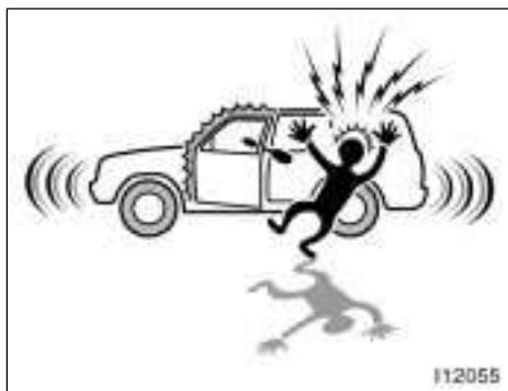
To deter vehicle theft, the system is designed to sound an alarm if any of the side doors, back door or hood is forcibly unlocked or opened or the battery terminal is disconnected and then reconnected when the vehicle is locked.
