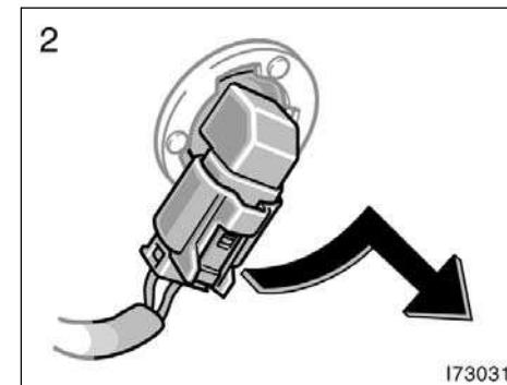
**2. Turn the bulb base counterclockwise to the front of the vehicle as shown.**
