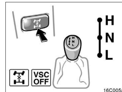
Use the four-wheel drive control lever and center differential lock button to select the transfer and center differential modes.
