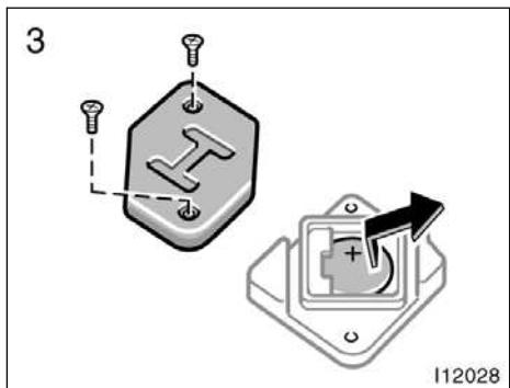
3. Remove the 2 screws to take out the lid of the module. Take out the discharged battery and put a new battery with the positive side up.
