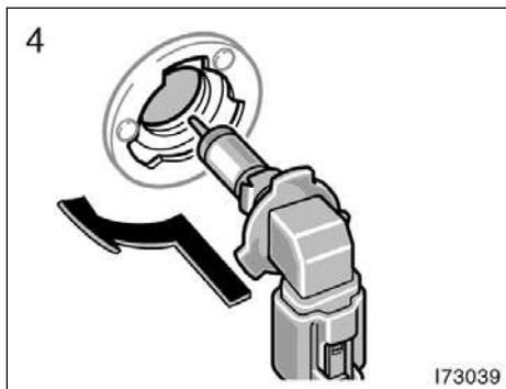
4. Install a new bulb base by turning it clockwise to the front of the vehicle.
