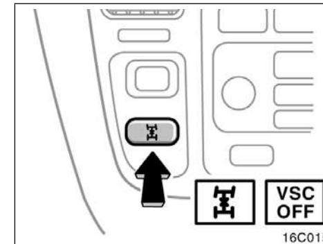
Pushing the center differential lock button automatically turns the vehicle skid control system off. At this time, the "VSC OFF" indicator comes on with the center differential lock indicator light. (For details, see "Four-wheel drive system—(a)Four-wheel drive control" in this section.)
