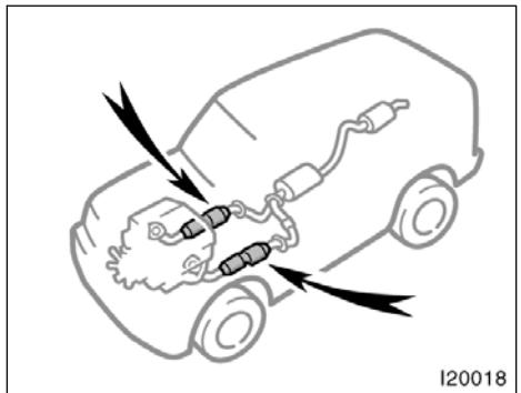
The three-way catalytic converter is the emission control device installed in the exhaust system.
