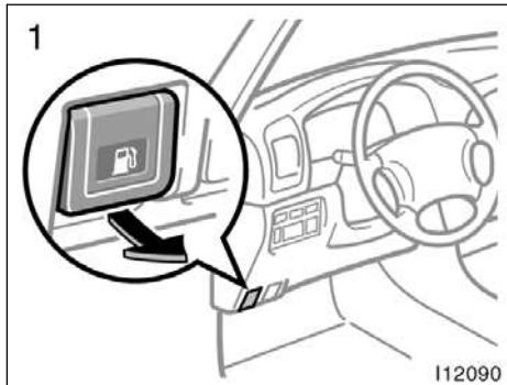
1. To open the fuel filler door, pull the lever.
