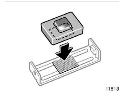
3. Remove Velcro loop on the stay. Remove the paper strip covering the adhesive on back side of Velcro loop and adhere it just behind the button to back side of the transmitter near center.
