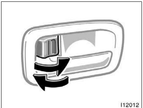
**LOCKING AND UNLOCKING WITH INSIDE LOCK KNOB**
