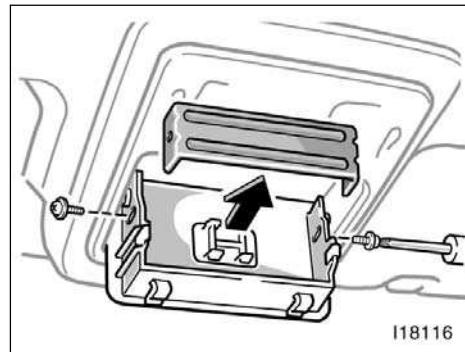
2. Unscrew the screws on both sides and remove the stay.
