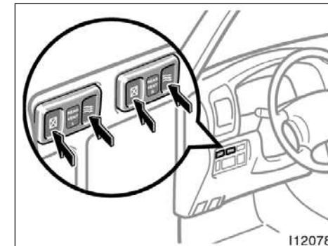
The rear quarter windows can be operated with the "REAR VENT" switches on the instrument panel.
