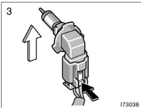
3. Pull the bulb out of the bulb base.
