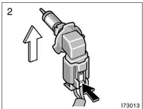
**2. Pull the bulb out of the bulb base.**
