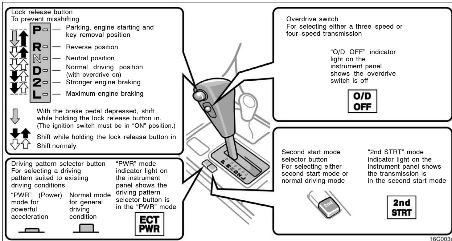
When the cruise control is being used, even if you downshift the transmission by turning off the overdrive switch, engine braking will not be enabled because the cruise control is not cancelled. For ways to decrease the vehicle speed, see "Cruise control" in this section.
