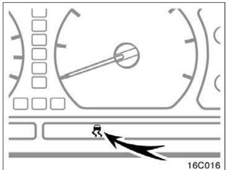
**The vehicle skid control system helps provide comprehensive control of systems such as anti-lock brake, traction control, engine control, etc. This system automatically controls the output of the brakes or engine to help prevent the vehicle from skidding under adverse conditions.**
