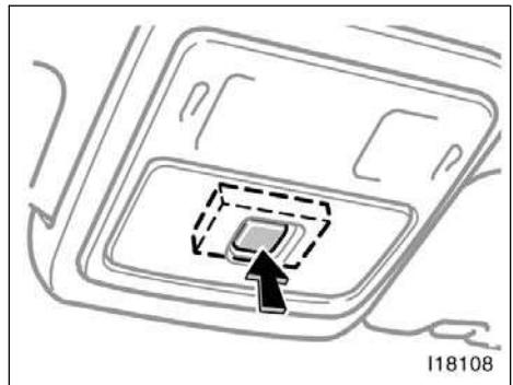
Your vehicle is equipped with a box designed to store a garage door opener transmitter. You can operate the stored garage door opener through the hole on the lid.
