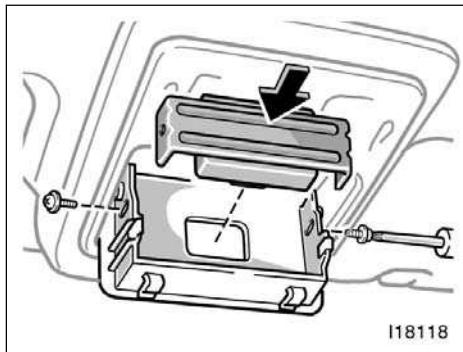
6. Reinstall the stay and secure it with the screws. Before fixing it with the screws, adjust the position of the transmitter as it can be operated through the opening on the lid.
