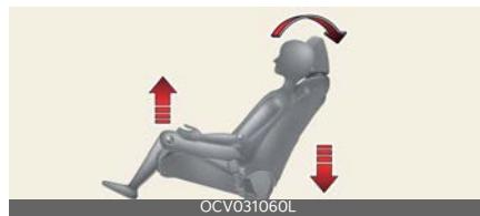
Relaxion comfort seats distribute body pressure and concentrated weight on specific body parts that occur whilst sitting in the same position for a long period of time. The seat relieves fatigue and discomfort by providing the optimal sit position.
