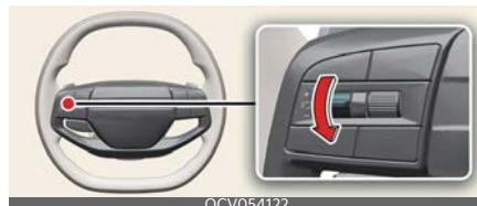
Push the (-) switch down and release it immediately. The set speed will decrease by 1 km/h (1 mph) each time the switch is operated in this manner.
