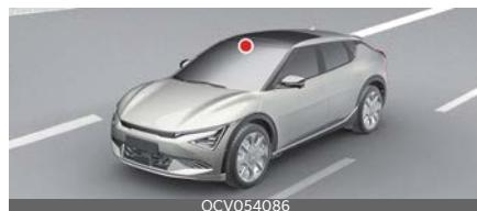
The front view camera is used as a detecting sensor to detect lane markings and front vehicles.
