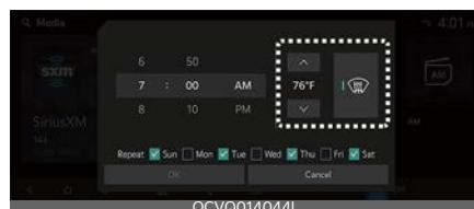
If the target temperature is set with the cable connected, the cabin temperature will be adjusted to the target temperature at departure time. In cold weather, pre-scheduled heating helps enhance electric vehicle performance by heating the vehicle in advance.
