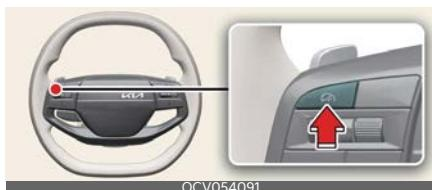
Press the Driving Assist button to turn on Smart Cruise Control. The speed will be set to the current speed on the cluster.
