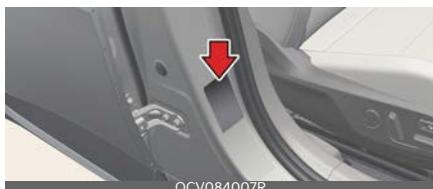
The tyre label located on the centre pillar as shown gives the tyre pressures recommended for your vehicle. The tyres supplied on your new vehicle are chosen to provide the best performance for normal driving.
