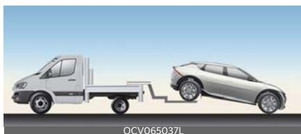
2-wheel drive vehicle can be towed with the opposite tyres on the ground (without dollies) and parking brake released before turning off the vehicle.
