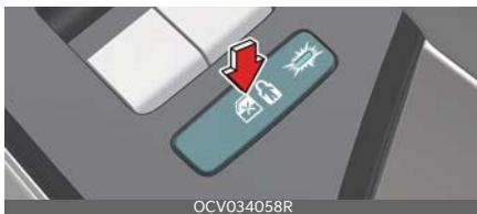
When the electronic child safety lock button is in the LOCK position and an approaching vehicle from the rear area is detected, the electronic child safety lock button will not unlock even if the driver presses the button to prevent the rear doors from opening.
