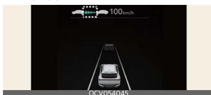
When the Based on Driving Style is enabled, the cluster will show the set vehicle distance level and target vehicle distance in white. It will also display the distance level and target distance based on the driver's driving behavior.
