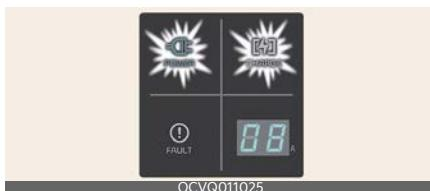
9. Check if the charging indicator light (⚡) of the high voltage battery in the instrument cluster is turned ON. Charging is not active when the charging indicator light (⚡) is off. If the charging connector is not connected properly, reconnect the charging cable to charge it again.
