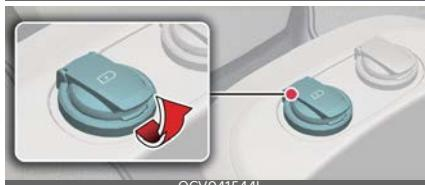
The USB charger allows drivers and passengers to charge their digital devices such as smartphones and tablets.
