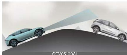
When driving on an uphill or downhill, the system may not detect the vehicle in your lane and the regenerative braking level will reduce automatically, making you feel that the vehicle is accelerating. Also, if the system suddenly recognises the vehicle in front, the regenerative braking level will increase automatically, making you feel that the vehicle is decelerating.
