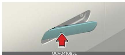
The outside door handle will slide out and the doors will unlock when the driver approaches the vehicle possessing the smart key. (Approach unlock system)
