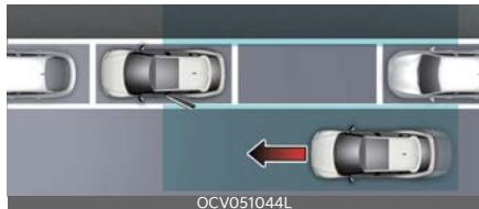
Whilst your vehicle is stopped, and if Safe Exit Warning detects a vehicle approaching the rear corner of your vehicle and a passenger opens a door, Safe Exit Warning may warn you with a warning message and a warning sound to help avoid a collision.
