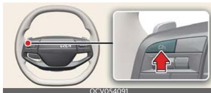
Press the Driving Assist (⌚) button to turn Manual Speed Limit Assist off. The Speed Limit indicator (⌚ LIMIT) will go off.
