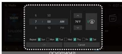
You can set the date and time of when to charge the battery and the climate control temperature. Also, you may select the time to start charging using the Off-peak time settings.
