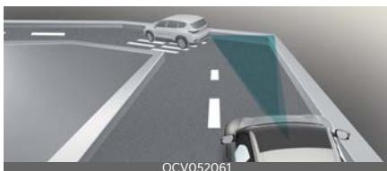
On curves, Smart Cruise Control may not detect a vehicle in the same lane, and may accelerate to the set speed. The vehicle speed may rapidly decrease when the vehicle ahead is detected suddenly.
