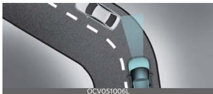
When driving on the curve, the system may not detect the vehicle in your lane and the regenerative braking level will reduce automatically, making you feel that the vehicle is accelerating.
