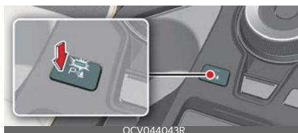
Press the Parking Safety (P) button to turn on Forward/Side/Reverse Parking Distance Warning. Press the button again to turn off the function.
