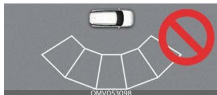
Remote Smart Parking Assist does not work normally in places where parking lines are not parallel. Even if a parking space is recognised, do not use it.
