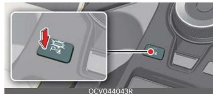
Press the Parking Safety (P) button to turn on Forward/Reverse Parking Distance Warning. Press the button again to turn off the function.
