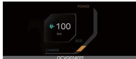
The Power/Charge Gauge shows the energy consumption rate of the vehicle and the charge/discharge status of the regenerative brakes.
