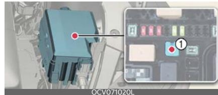
4. Check the removed fuse; replace it if it is blown. Spare fuses are provided in the instrument fuse panel (or in the motor compartment fuse panel).
