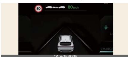
When operating Manual Speed Limit Assist or Smart Cruise Control, if the speed set by the driver is the same as the speed limit on the road, the set speed is automatically adjusted accordingly the speed limit afterwards. The auto set speed change function operates on roads with a speed limit of above 70 km/h (45 mph). When the function is activated, the set speed on the instrument cluster is displayed in green.
