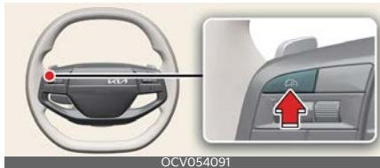
Press the Driving Assist button to turn Cruise Control off. The Cruise ( ) indicator will go off.
