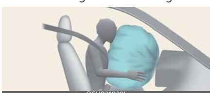
The air bag modules are located both in the centre of the steering wheel and in the front passenger's panel above the glove box. When the SRSCM detects a sufficiently severe impact to the front of the vehicle, it will automatically deploy the front air bags.
