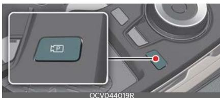
Press the Parking/View button (1) to turn on Rear View Monitor.
