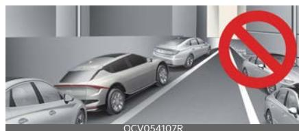
For your safety, Remote Smart Parking Assist does not search for parking spaces at areas with narrow parking spaces that are narrower than the minimum space required for parking.
