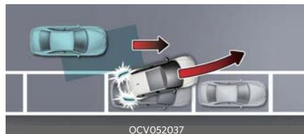
When you are driving forward out of a parking space, if Blind-Spot Collision-Avoidance Assist judges that there is a collision risk with an approaching vehicle in the blind spot, it can help avoid collision by applying the brake.
