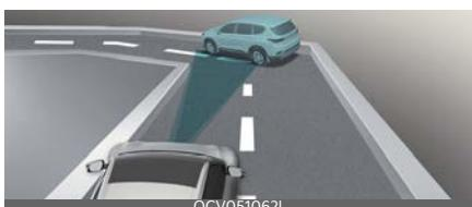
Your vehicle speed can be reduced due to a vehicle in the adjacent lane. Check to be sure that the road conditions permit safe operation of Smart Cruise Control and if necessary, depress the brake pedal to reduce your driving speed in order to maintain a safe distance
