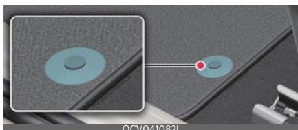
Make sure the floor mat is attached to the anchors to keep it from sliding forward.
