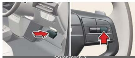
Press the (OFF) switch or depress the brake pedal to temporarily cancel Smart Cruise Control.
