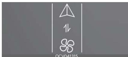
Press the icon on the switchable controller to switch between infotainment system or climate control panel.
