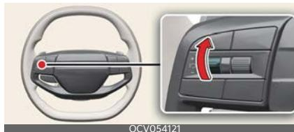
Push the (+) switch up and release it immediately. The set speed will increase by 1 km/h (1 mph) each time the switch is operated in this manner.
