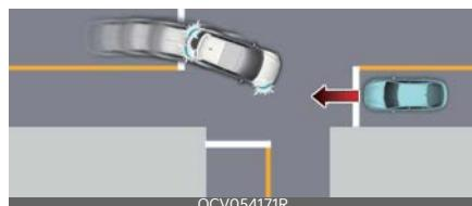
Junction Turning function can help avoid a collision with an oncoming vehicle, powered two-wheeler and cyclist in an adjacent lane when turning left (left-hand drive) or right (right-hand drive) at a crossroad with the turn signal on by applying emergency braking.
