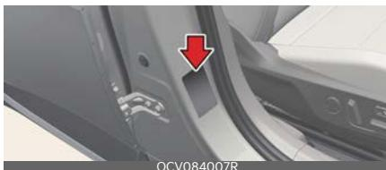
All specifications (sizes and pressures) can be found on a label attached to the vehicle.
