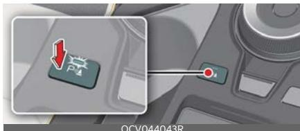
Press and hold the Parking Safety button (P) more than 2 seconds to turn the Parking Collision-Avoidance Assist on or off.
