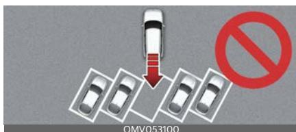
Remotely moving forward or backward function may not operate properly in a diagonal parking space.
