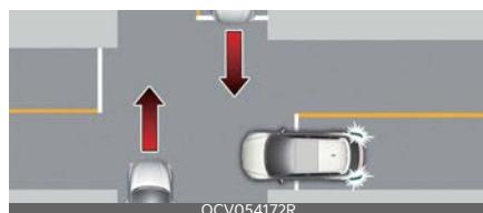
Junction Crossing function will help avoid a collision with oncoming vehicles on the left or right side when crossing an intersection by applying emergency braking.
