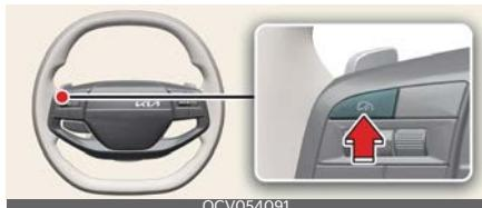
2. Push the (+) switch up or (-) switch down, and release it at the desired speed. The set speed will increase by 1 km/h (1 mph) increments.
