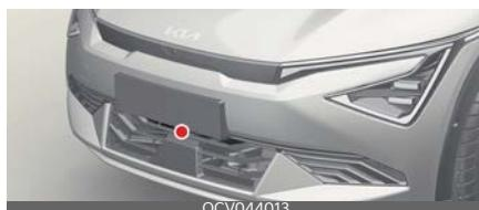
Active air flap system controls the air flap below the front bumper to cool the vehicle parts and improve energy efficiency.
