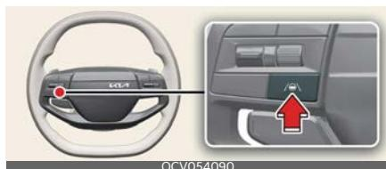
With the vehicle on, shortly press the Lane Driving Assist button located on the steering wheel to turn on Lane Following Assist. The gray or green (Ⓐ) indicator light will appear on the cluster. Press the Lane Driving Assist button again to turn off Lane Following Assist.
