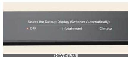
Press and hold the icon to select the default mode for the control panel.
