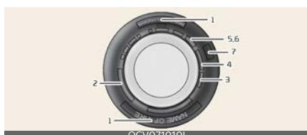
This information identifies and describes the fundamental characteristics of the tyre and also provides the tyre identification number (TIN) for safety standard certification. The TIN can be used to identify the tyre in case of a recall.
