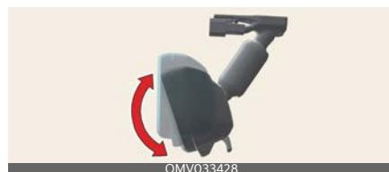
The height of the rearview mirror can be adjusted to suit your driving posture. Change to optical mirror mode, adjusting the rearview mirror angle by moving it up and down.
