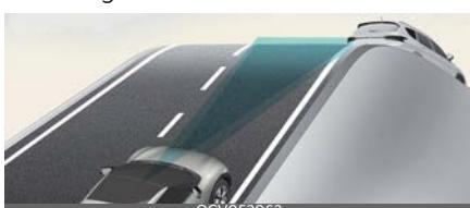
During uphill or downhill driving, the Smart Cruise Control may not detect a moving vehicle in your lane, and
