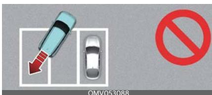
If Remote Smart Parking Assist is used, In a parking space where the alignment of the adjacent vehicle is not correct, your vehicle may cross the parking line to avoid the parked vehicle. However, if the parking lines are present and properly recognised, Remote Smart Parking Assist helps the driver park in parallel along the parking lines.
