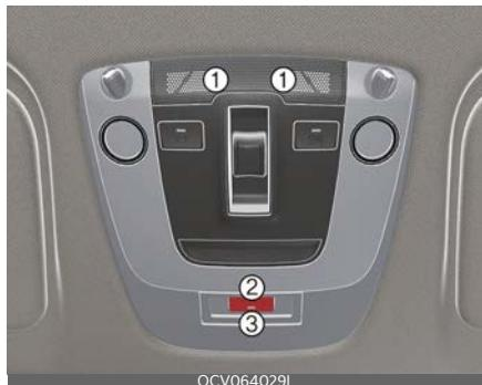
Elements of the UAE eCall system, installed in passenger compartment:
