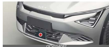
Always make sure the radar sensor cover is clean and free of dirt, snow, and debris.
