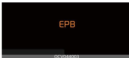
If the EPB malfunction indicator remains on, turns on whilst driving, or does not turn on when the vehicle is in the POWER ON position, this indicates that the EPB may be malfunctioning.
