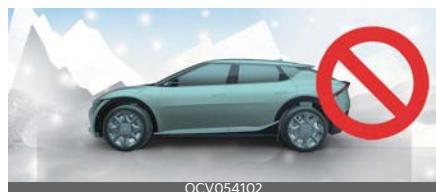
Snow may interfere with sensor operation, or Remote Smart Parking Assist may cancel if the road is slippery whilst parking.
