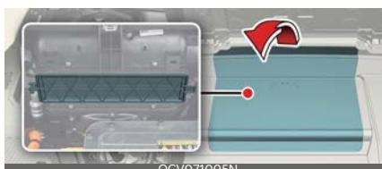
3. Remove the climate control air filter cover (2) by pulling out both sides of the cover (1).
