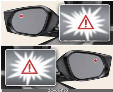
The warning light on the cluster, outside rearview mirror and head-up display (if equipped) will appear when the vehicle on both lanes is detected from the rear. A vehicle is detected in the following conditions.
