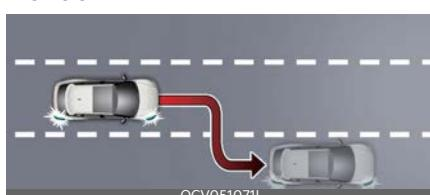
Highway Lane Change Assist function helps change lanes to the direction you operate the turn signal switch if the function judges that lane change is possible.
