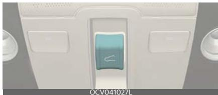
The sunroof can only be operated when the EV button is in the POWER ON or DRIVE READY position.
