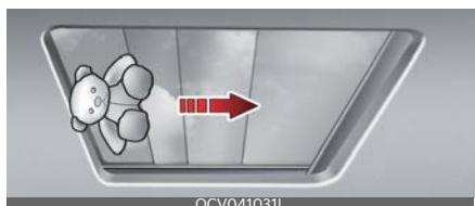
If the power sunshade or sunroof glass senses any obstacle whilst it is closing automatically, it will reverse direction then stop at a certain position.
