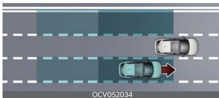
Blind-Spot Collision-Avoidance Assist helps detect and informs the driver that a vehicle is in the blind spot.
