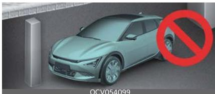
Remote Smart Parking Assist performance may reduce or collision with an obstacle may occur when there is a narrow object, circular pillar, square pillar, or a pillar surrounded by objects such as a fire extinguisher, etc. near the parking space. The driver should park the vehicle manually.
