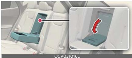
Additional cargo space is provided to accommodate long/narrow cargo (skis, poles, etc.) not able to fit properly in the trunk when closed.
