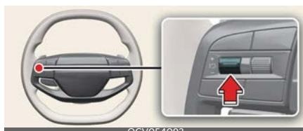
Press the (II) switch to temporarily pause the set speed limit. The set speed limit will turn off but the Speed Limit indicator (➋) will stay on.
