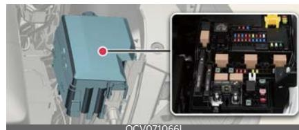
When the blade type fuse is disconnected, remove it by using the clip designed for changing fuses located in the motor room fuse box. Upon
