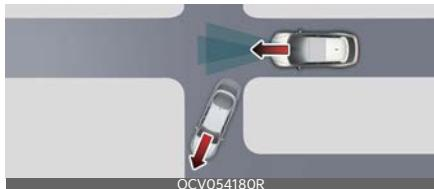
When a vehicle ahead disappears at an intersection, your vehicle may accelerate.
