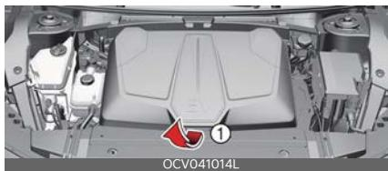
2. Remove the cover by pulling the upper part of the cover.
