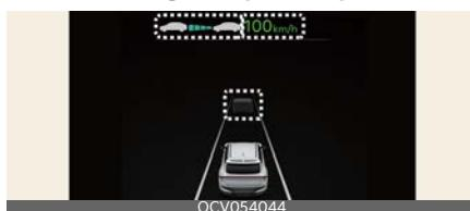
If you want to speed up temporarily without altering the set speed whilst Smart Cruise Control is operating, depress the accelerator pedal. Whilst the accelerator pedal is depressed, the set speed, distance level and target distance will blink on the cluster.
