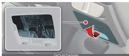
3. Pull the suspected fuse straight out. Use the removal tool (1) provided in the main fuse box in the motor compartment.
