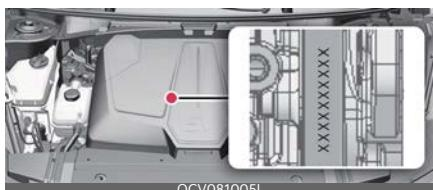
The motor number is stamped on the motor as shown.
