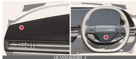
The indications of the system's presence are the words **AIR BAG** intagliated on the air bag pad cover in the steering wheel, and the passenger's side front panel pad above the glove box.
