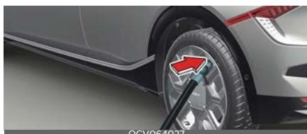
4. Unscrew the valve cap and screw the filling hose onto the tyre valve.
