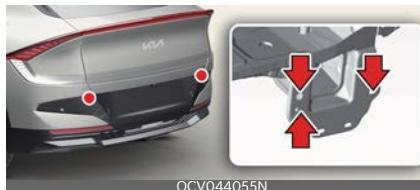
The mounting hole for hitches are located on both sides of the underbody behind the rear tyres.
