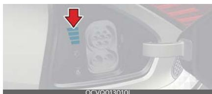
When scheduled charging is set, charging is not initiated immediately when the AC charger or portable charger (ICCB: In-Cable Control Box) is connected.
