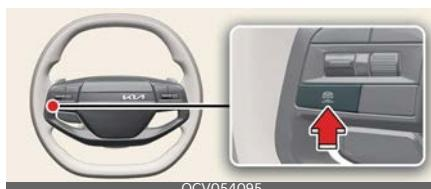
Each time the button is pressed, the headway changes as follows:
