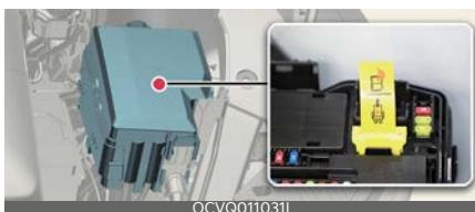
The service interlock connector, located within the motor compartment, is a safety device that disables the high voltage of the battery. It's for vehicle inspections at a professional workshop. Kia
