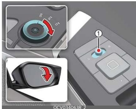
With the outside rearview mirror switch (1) positioned to the left or right, the left and right outside rearview mirrors automatically move to the default provision position to improve driver visibility when the vehicle is in reverse.
