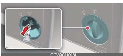
If the charging cable does not detach due to battery discharge and failure of the electric wires, open the tailgate and slightly pull the emergency cable as shown above. The charging connector will then unlock.
