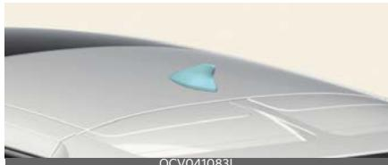
Shark-fin antenna transmit and receive signals such as AM/FM and GPS. Additional signals are sent and received according to vehicle options.
