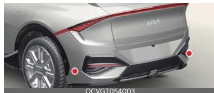
Blind-Spot Collision-Avoidance Assist helps detect and informs the driver that a vehicle is approaching at high speed from the blind spot area.
