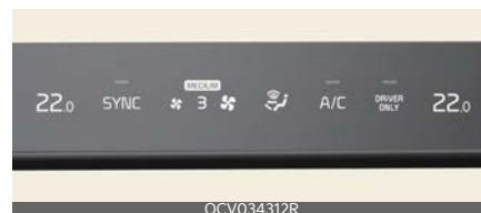
Press the button on the switchable controller to select the desired control panel. The selected control panel icon will be illuminated and the control panel will be changed.
