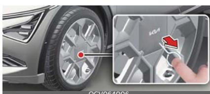
For 20 and 21 inch wheel, take out the remover tool in the Tyre Mobility Kit. Insert the tool to the hole and pull out the wheel cover.
