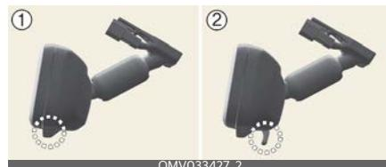
1. Pull the mode select lever to all the way switch to the DCM mode (camera view mode).
