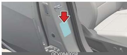
The vehicle certification label attached on the centre pillar as shown gives the vehicle identification number (VIN).
