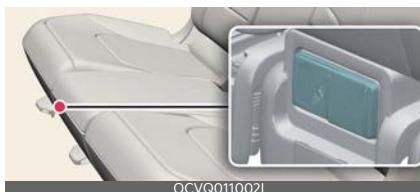
2. Use the mechanical key to unlock the power outlet cover.
