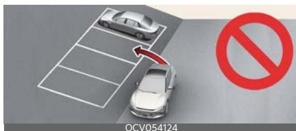
Remote Smart Parking Assist does not work properly on sloped or curved road surfaces even if there are parking lines. Even if a parking space is recognised, do not use it.
