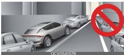
Remote Smart Parking Assist may not operate properly when leaving a parking space that is narrow and near a wall. Always check for pedestrians, animals, objects whilst leaving.
