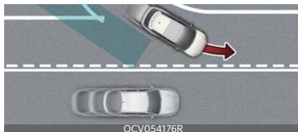
Blind-Spot Collision-Avoidance Assist may not operate properly when driving where the road merges or divides. The function may not detect the vehicle in the next lane.
