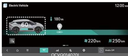
Select vehicle image from the infotainment system screen. You can check battery discharging level.
