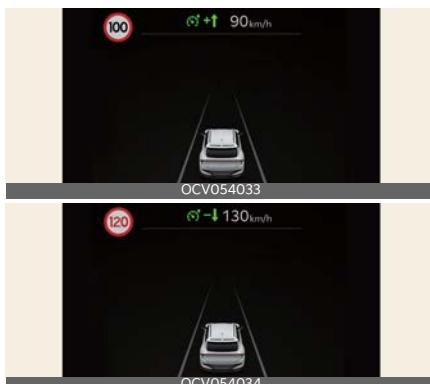
If the speed limit of the road changes during the operation of Manual Speed Limit Assist or Smart Cruise Control, an arrow in the direction of up or down is displayed to inform the driver that the set speed needs to be changed. At this time, the driver can change the set speed according to the speed limit by
