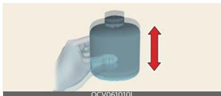
2. Remove the sealant bottle cap and sealant bottle holder cap and screw the bottle onto the sealant bottle holder.
