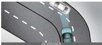
The smart regeneration system may recognise a vehicle in an adjacent lane when driving on a curved road. In this case, the system increase the braking level and slow the vehicle.
