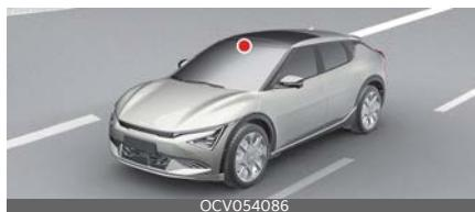
The front view camera is used as a detecting sensor to detect ambient light and brightness whilst driving. Refer to the picture above for the detailed location of the detecting sensor.
