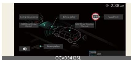
Select **Settings** → **Vehicle** → **Driver Assistance** on the infotainment system screen to set the Driver Assistance function.
