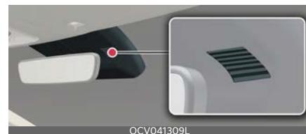
The auto defogging system operates when the heater or air conditioning is on.
