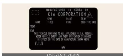
This label shows the maximum allowable weight of the fully loaded vehicle. This is called the GVWR (Gross Vehicle Weight Rating). The GVWR includes the weight of the vehicle, all occupants and cargo.
