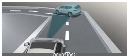
Your vehicle speed can be reduced due to a vehicle in the adjacent lane. Check to be sure that the road conditions permit safe operation of the Smart Cruise Control and if necessary, depress the brake pedal to reduce your driving speed in order to maintain a safe distance.
