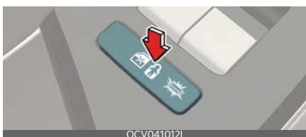
In addition, when the electronic child safety lock button is in the LOCK position and an approaching vehicle from the rear area is detected, the electronic child safety lock button will not unlock even if the driver presses the button to prevent the rear doors from opening.
