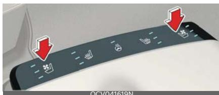
The temperature setting of the seat changes according to the button indicator.
