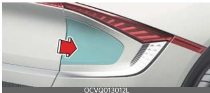
You cannot open the charging door when the vehicle's doors are locked.
