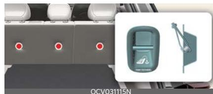
First secure the child restraint with the LATCH lower anchors or the seat belt. If the child restraint manufacturer recommends that the top tether strap be attached, attach and tighten the top tether strap to the top tether strap anchor.
