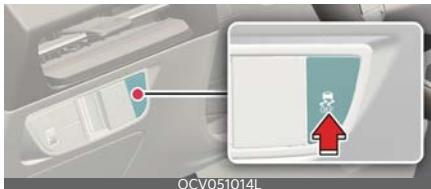
ESC checks where you are steering and where the vehicle is actually going. ESC applies the brakes on individual wheels and intervenes with the vehicle management system to stabilize the vehicle.
