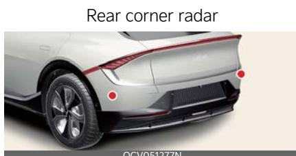
Refer to the picture above for the detailed location of the detecting sensors.
