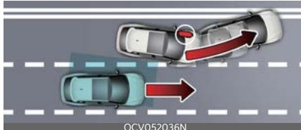
When changing lanes by detecting the lane ahead, if Blind-Spot Collision-Avoidance Assist judges that there is a collision risk with an approaching vehicle in the blind spot, it will help avoid collision by applying the brake.
