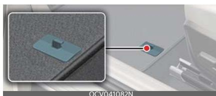
When using a floor mat on the front floor carpet, make sure it attaches to the floor mat anchor(s) in your vehicle. This keeps the floor mat from sliding forward.
