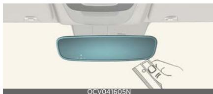
3. While the HomeLink indicator light (7) is flashing orange, press and hold the hand-held remote button. Continue pressing the hand-held remote button until the HomeLink indicator light (7) light changes from orange to green. You may now release the hand-held remote button.
