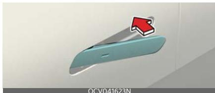
When all doors are closed, touch the touch sensor on the front outside door handle (the engraved part) while carrying the smart key with you, outside door handle will return and doors will be locked.
