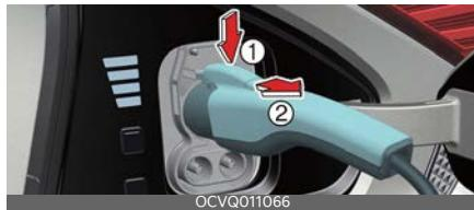
Before disconnecting the charging connector, make sure the vehicle's doors are unlocked. When the doors are locked, the charging connector lock system will be triggered. And the
