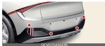
The rear ultrasonic sensors are located inside the rear bumper to detect objects in the rear area. If the sensors are covered with foreign material, such as snow or rain, it may adversely affect sensor performance and Reverse Parking Collision-Avoidance Assist may not operate normally. Always keep the rear bumper clean.
