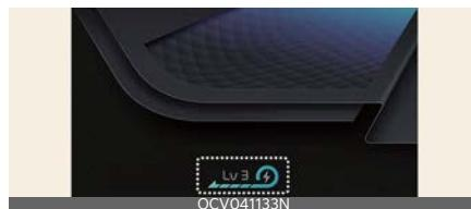
The regenerative brake indicates the level of the regenerative braking that you set. And it also indicates Smart regenerative system's operation status.
