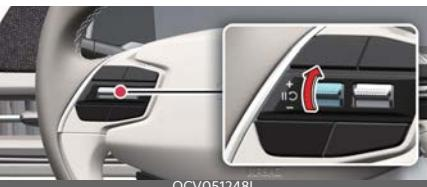
Push the + switch up and release it immediately. The set speed will increase by 1 mph (1 km/h) each time the switch is operated in this manner.
