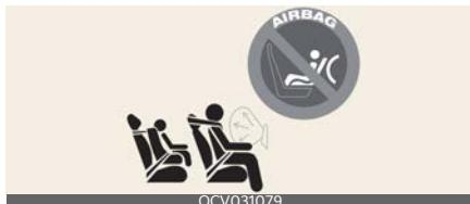
If the air bag deploys, it would impact the rear-facing child restraint, causing serious or fatal injury.
