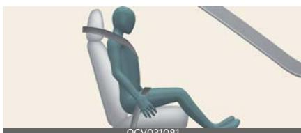
When an adult is seated in the front passenger seat, if the PASSENGER AIR BAG OFF indicator is on, change EV button to the OFF position and ask the passenger to sit properly (sitting upright with the seatback in an upright position, centered on the seat cushion with their seat belt on, legs comfortably extended and their feet on the floor). Restart the vehicle and have the person remain in that position. This will allow the system to detect the
