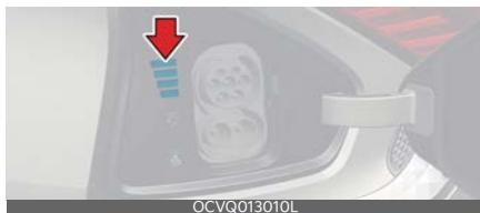
When scheduled charging is set, charging is not initiated immediately when the AC charger or Portable Charging Cable (ICCB: In-Cable Control Box) is connected. When immediate charging is required, use the infotainment system or the Kia Connect application on your smart phone to deactivate the scheduled charging or press and hold the charging button on the charging door for 2 seconds.
