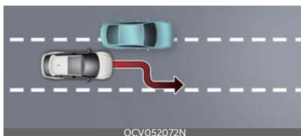
When vehicle speed is above 40 mph (60 km/h), if a vehicle around you is driving at a close distance, your vehicle will control steering in the opposite direction of the vehicle to assist in safe driving. If there are vehicles in both sides of the lane that are driving close to you, the function will not veer to the opposite side of the lane.
