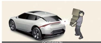
After the hazard warning lights blink and the chime sounds 6 times, the smart liftgate will open.
