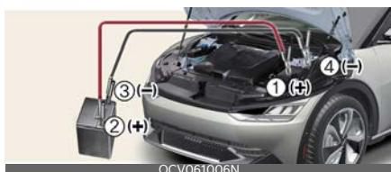
Jump starting can be dangerous if done incorrectly. Therefore, to avoid harm to yourself or damage to your vehicle or battery, follow these jump starting procedures. If in doubt, we strongly recommend that you have a competent technician or towing service jump start your vehicle.
