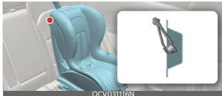
1. Route the child restraint tether strap over the child restraint seatback. Route the tether strap under the head restraint and between the head restraint posts, or route the tether strap over the top of the vehicle seatback. Make sure the strap is not twisted.
