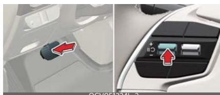
Press the ( ) switch or depress the brake pedal to temporarily cancel Smart Cruise Control.
