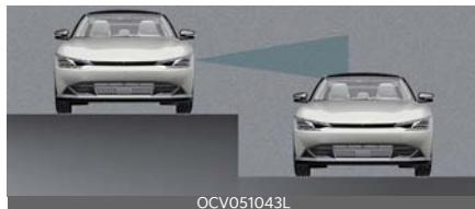
Blind-Spot Collision-Avoidance Assist may not operate properly when driving where the heights of the lanes are different. Blind-Spot Collision-Avoidance Assist may not detect the vehicle on a road with different lane heights. Always pay attention to road and driving conditions while driving.
