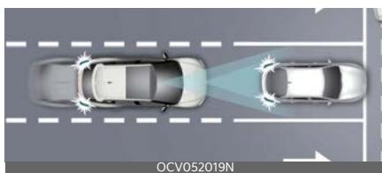
Forward Collision-Avoidance Assist is designed to help detect and monitor the vehicle ahead or help detect a pedestrian or cyclist in the roadway and warn the driver that a collision is imminent with a warning message and an audible warning apply emergency braking.
