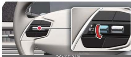
Push the - switch down and release it immediately. The set speed will decrease by 1 mph (1 km/h) each time the switch is operated in this manner.
