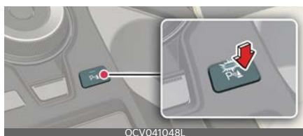
Press the Parking Safety (P) button to turn on or off Reverse Parking Distance Warning.
