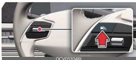
Press the Driving Assist (i) button to turn Manual Speed Limit Assist off. The Speed Limit indicator (LIMIT) will go off.
