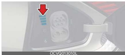
When charging the high voltage battery, the charge level can be checked from inside the charging door.
