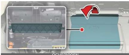
3. Remove the climate control air filter case (2) by pulling out left side of the cover (1).
