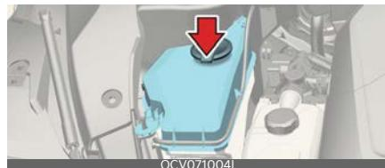
The reservoir is translucent so that you can check the level with a quick visual inspection.
