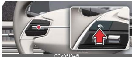
The speed limit indicator (LIMIT) light will appear and the set speed limit will be displayed on the cluster.
