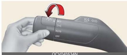
When the light switch is in the headlamp (Low beam) position, the head, tail, license lights will turn ON.
