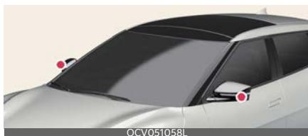
(camera located at bottom of the mirror)
