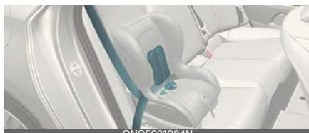
Since all passenger seat belts move freely under normal conditions and only lock under extreme or emergency conditions (emergency locking mode), you must manually pull the seat belt all the way out to shift the retractor to the "automatic locking" mode to secure a child restraint.
