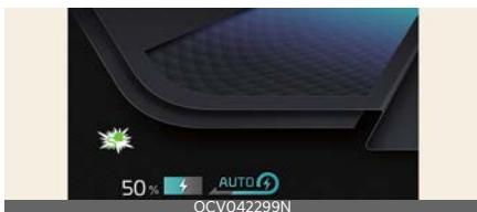
Charging doesn't start when the charging indicator lamp is OFF.
