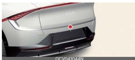
The wide-rear view camera is used as a detecting sensor to detect pedestrians. If the camera lens is covered with foreign material, such as snow or rain, it may adversely affect camera performance
