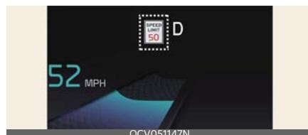
When driving at a speed higher than the displayed speed limit, the red speed limit indicator will blink.
