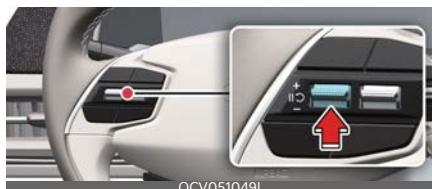
Press the (II) switch to temporarily pause the set speed limit. The set speed limit will turn off but the Speed Limit indicator (LIMIT) will stay on.
