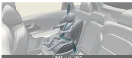
A forward-facing child seat provides restraint for the child's body with a harness. Keep children in a forward-facing child seat with a harness until they reach the top height or weight limit allowed by your child restraint's manufacturer.
