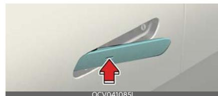
To lock your vehicle using the door handle touch sensor or the smart key:
