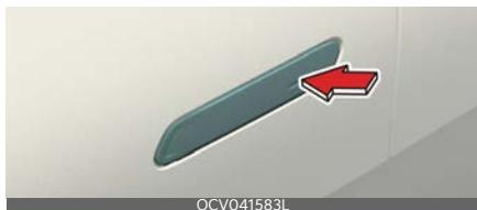
Push the button on the front outside door handle (the engraved part) while carrying the smart key with you, all doors will lock.
