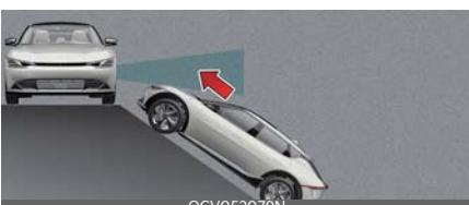
Rear Cross-Traffic Collision-Avoidance Assist may be limited when the vehicle is on an uphill or downhill slope, or near it, and may not detect the vehicle approaching from the blind spot area. If this occurs, the function may not warn the driver or control the brakes when necessary.
