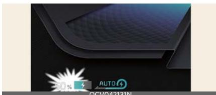
The SOC gauge shows the charging status of the high voltage battery.
