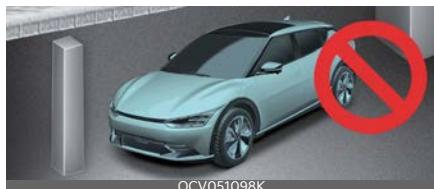
Remote Smart Parking Assist performance may reduce or collision with an obstacle may occur when there is a narrow object, circular pillar, square pillar, or a pillar surrounded by objects such as a fire extinguisher, etc. near the parking space. The driver should park the vehicle manually.
