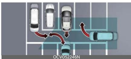
Rear Cross-Traffic Collision-Avoidance Assist may detect vehicles which are parking or pulling out near your vehicle (for example: a vehicle leaving beside your vehicle, a vehicle parking or pulling out in the rear area, a vehicle approaching your vehicle making
