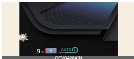
When the remaining battery is lower than 10% (15% for GT) on the SOC gauge, the warning light (✉) turns ON to alert you of the battery level.
