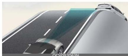
During uphill or downhill driving, the Smart Cruise Control may not detect a moving vehicle in your lane, and cause your vehicle to accelerate to the set speed. Also, vehicle speed will rapidly decrease when the vehicle ahead is detected suddenly.
