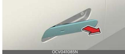
If you approach (within 1 ft. (30 cm)) the driver or front passenger's door handle possessing the smart key, the outside door handles slide out and the doors are unlocked. In this case, Hazard Warning
