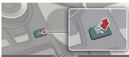
Press the Parking Safety (P) button to turn on or off Forward/Reverse Parking Distance Warning.
