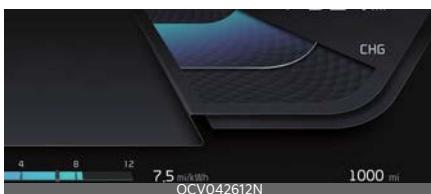
The odometer indicates the total distance that the vehicle has been driven
