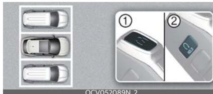
1. Within a certain range from the vehicle press the door lock (🔒) button on the smart key and lock all doors.
