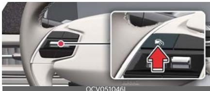
Press the Driving Assist (SCC) button to turn on the function. The speed will be set to the current speed on the cluster.
