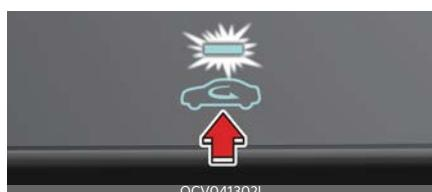
With the recirculated air position selected, air from the passenger compartment will be drawn through the heating system and heated or cooled according to the function selected.
