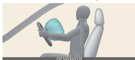
Upon deployment, tear seams molded directly into the pad covers will separate under pressure from the expansion of the air bags. Further opening of the covers then allows full inflation of the air bags.
