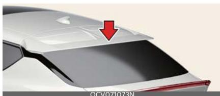
If the high mounted stop lamp (LED) does not operate, have your vehicle checked by an authorized Kia dealer.
