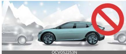
Snow may interfere with sensor operation, or Remote Smart Parking Assist may cancel if the road is slippery while parking.
