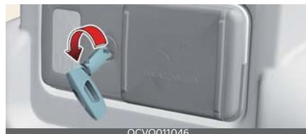
2. Connect to the power outlet located in the base of the rear seat with the EV button in the ON position.
