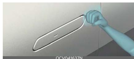
2. If necessary, increase the intensity of tapping to remove ice, and repeat until the door handle protrudes when unlocking the door.
