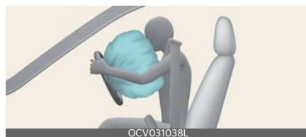
A fully inflated air bag, in combination with a properly worn seat belt, slows the driver's or the passenger's forward motion, reducing the risk of head and chest injury.
