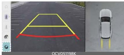
With the vehicle on, select the setup icon (⚙) on the screen or **Setup** → **Vehicle** → **Driver Assistance** → **Parking Safety** → **Camera Settings** from the infotainment system screen to change the Rear View Monitor settings.
