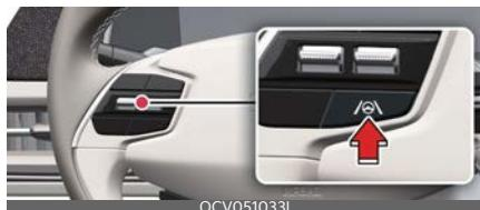
With the vehicle on, shortly press the Lane Driving Assist button located on the steering wheel to turn on Lane Following Assist. The gray or green (Ⓐ) indicator light will appear on the cluster. Press the button again to turn off the function.
