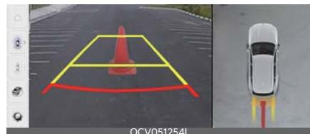
Parking distance warning is displayed on the right side of the Surround View Monitor top view screen when the **Parking Distance Warning** is selected.
