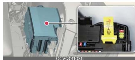
The high voltage cut-off switch is located in the motor room compartment fuse box.
