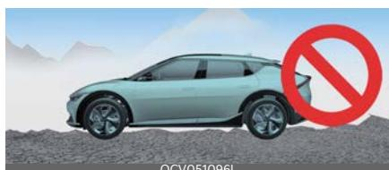
Remote Smart Parking Assist may cancel when the vehicle slips, or the vehicle cannot move due to road conditions such as pebbles or fragmented stones.
