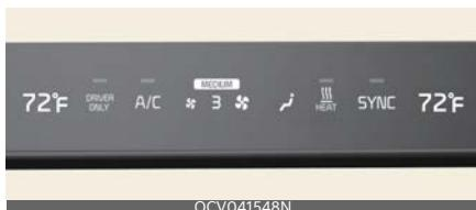
Press the button on the switchable controller to select the desired control panel. The selected control panel icon will appear and the control panel will be changed.
