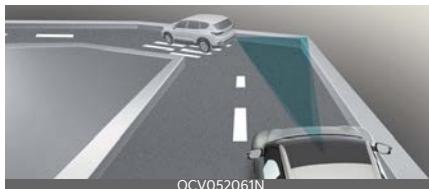
On curved roads, Smart Cruise Control may not detect a vehicle in the same lane, and may accelerate to the
