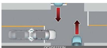
Junction Crossing function may help avoid a collision with oncoming vehicles on the left or right side when crossing an intersection by applying emergency braking.
