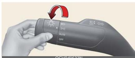
When the light switch is in the parking light position, the tail, license and instrument panel lights will turn ON.
