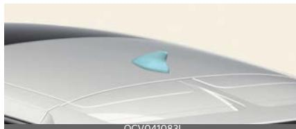
The sharkfin antenna transmits and receives wireless signals such as AM/FM, Sirius XM, GNSS, etc. \* The signals which antenna can transmit and receive vary by the vehicle option.
