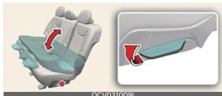
5. To use the rear seat, lift and unfold the seatback to the upright position by pulling up the folding lever. Push the seatback firmly until it clicks into place. Make sure the seatback is locked in place.
