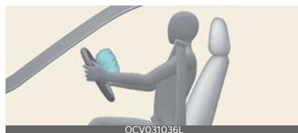
The front air bag modules are located both in the center of the steering wheel and in the front passenger's panel above the glove box. When the SRSCM detects a sufficiently severe impact to the front of the vehicle, it will automatically deploy the front air bags.
