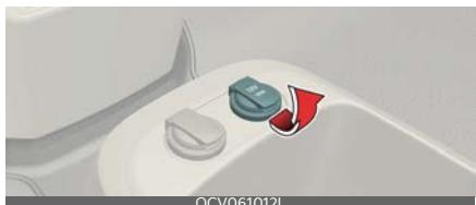
7. With the EV button ON, switch on the compressor and let it run for approximately 5~7 minutes to fill the sealant up to cold tire recommended pressure. (refer to "Tires and wheels" on page 10-4). Be careful not to overinflate the tire and stay away from the tire when filling it.
