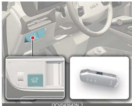
When the liftgate is closed, press the power liftgate open/close button for 1 second. The power liftgate opens with a warning sound.
