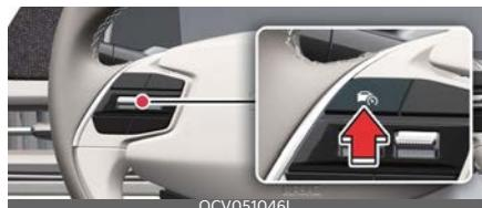
Press the Driving Assist ( ) button to turn Smart Cruise Control off.
