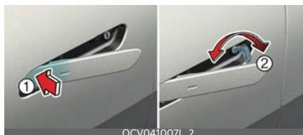
Press the front part (1) of the door handle to pull out the rear part of the door handle. While keep pressing the front part of the door handle, insert the mechanical key (2) to the lock with the key handle facing the ground as shown.
