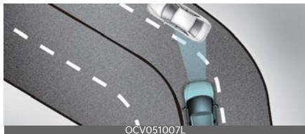
The smart regeneration system may recognize a vehicle in an adjacent lane when driving on a curved road. In this case, the system increases the braking level and slows the vehicle.
