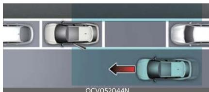
After the vehicle stops, when an approaching vehicle from the rear area is detected as soon as a passenger opens a door, Safe Exit Warning will warn the driver with a warning message and an audible warning to help prevent a collision.
