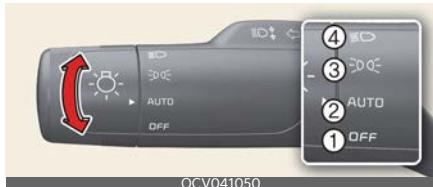
To operate the lights, turn the knob at the end of the control lever to one of the following positions:
