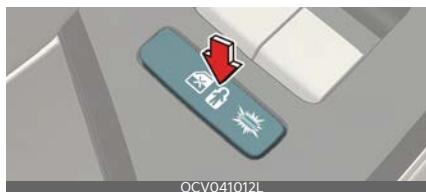
If you push the electronic child safety lock switch and the indicator appears, rear passengers cannot open the rear door from inside the vehicle.
