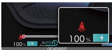
If the driver continues not to fasten the seat belt, the warning light will stay on and the warning chime will sound for approximately 6 seconds until the belt is fastened each time the EV button is in ON. This will happen every time the EV button is in ON.
