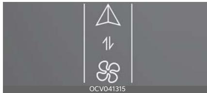
Press the button on the switchable controller to switch between infotainment system or climate control panel.
