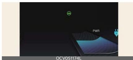
If the vehicle ahead and/or both lane markings are detected and your vehicle speed is below 110 mph (180 km/h), Lane Following Assist will help center the vehicle in the lane by assisting the steering wheel. The green (Ⓐ) indicator light will appear on the cluster.
