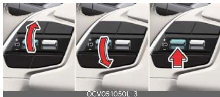
To resume Manual Speed Limit Assist after the function was paused, operate the +, -, (i) switch.
