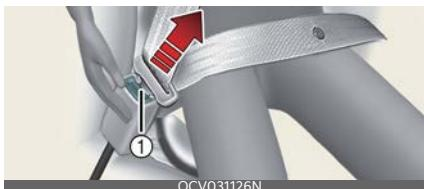
The seat belt is released by pressing the release button (1) on the locking buckle. When it is released, the belt should automatically draw back into the retractor.
