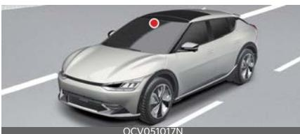
The front view camera is used to detect driving patterns and front vehicle departure while vehicle is being driven.
