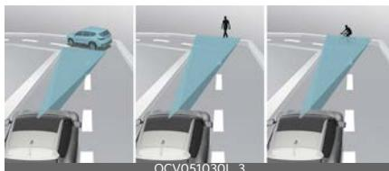
Forward Collision-Avoidance Assist may detect a vehicle, pedestrian or cyclist in the next lane or outside the lane when driving on a curved road. If this occurs, Forward Collision-Avoidance Assist may unnecessarily warn the driver and control the brake or steering wheel (if equipped). Always check the traffic conditions around the vehicle.
