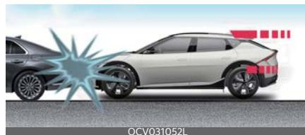
Front air bags are designed to inflate in a frontal collision depending on the severity of impact of the front collision.
