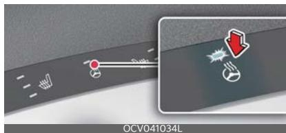
To turn the heated steering wheel off, press the button once again. The indicator on the button will turn off.
