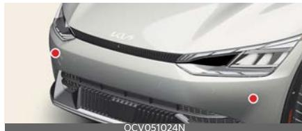
The front view camera, front radar, and front corner radars (if equipped) are used as a detecting sensor to detect the vehicles in front.
