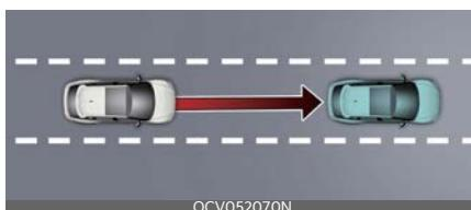
Highway Driving Assist is designed to help detect vehicles and lanes ahead, and help maintain distance from the vehicle ahead, maintain the set speed, and keep the vehicle between lanes while driving on the highway (or motorway).
