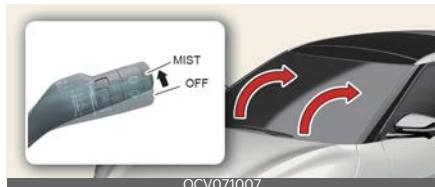
After turning off the vehicle, move the wiper switch to the single wiping (MIST) position within 20 seconds and hold the switch more than 2 seconds until the wiper blade is in the fully up position.
