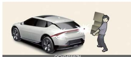
If you are positioned in the detecting area (20~40 inches [50~100 cm] behind the vehicle) carrying a smart key, the hazard warning lights will blink and chime will sound to alert you the smart key has been detected and the liftgate will open.
