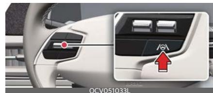
With the vehicle on, press and hold the Lane Driving Assist button located on the steering wheel to turn on Lane Keeping Assist. The gray (/
