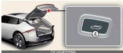
Press the power liftgate open/close button. The liftgate opens or closes with a warning sound.
