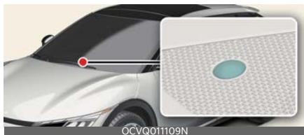
The high voltage indicator is located on bottom of the windshield. When the 12V auxiliary battery is discharged, it is charged from the high voltage battery of the vehicle. When the high voltage electricity flow in the vehicle, the color of the indicator changes to amber and turns off after charging is finished.
