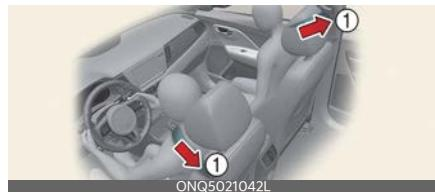
The pre-tensioner seat belts may be activated when a frontal collision is severe enough, together with the air bags.
