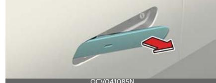
The handle does not slide out even when you approach with the smart key in possession. The doors are unlocked if you press the outside handle as the handles slide out.
