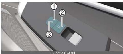
Operate by pressing the central door lock switch.
