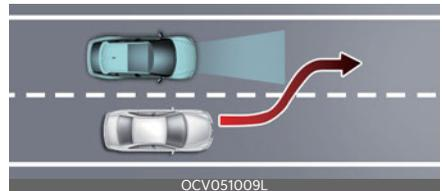
When a vehicle changes lanes in front of you, the smart regeneration system may not immediately detect the vehicle, especially if the vehicle changes lanes abruptly. In this case, you must maintain a safe braking distance, and if necessary, depress the brake pedal to reduce
