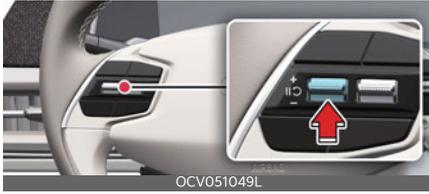
Press the (||) switch to temporarily pause the set speed limit. The set speed limit will turn off but the Speed Limit indicator (LIMIT) will stay on.
