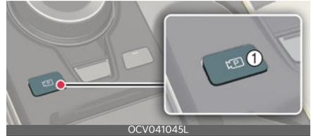
Press the Parking/View button (1) to turn on or off Rear View Monitor while P (Park) position is selected.
