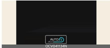
If the front radar recognizes the vehicle in front, 'AUTO' is displayed in blue. The regenerative braking level is automatically controlled depending on the driving condition of the vehicle in front and the level is indicated with arrows.
