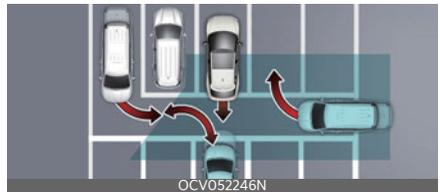
Rear Cross-Traffic Collision-Avoidance Assist may detect vehicles which
