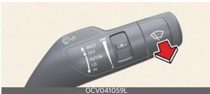
1. Move the wiper speed control switch to the OFF position.
