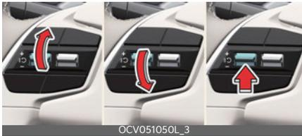
To resume Manual Speed Limit Assist after the function was paused, operate the +, -, (||) switch.
