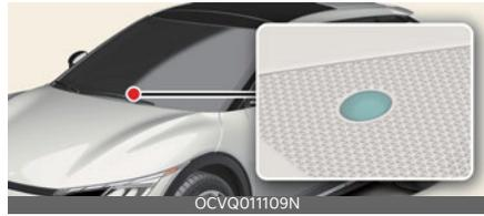
The high voltage indicator is located on top of the crash pad. When the 12V auxiliary battery is discharged, it is charged from the high voltage battery of the vehicle. When the high voltage electricity flow in the vehicle, the color of the indicator changes to amber and turns off after charging is finished.
