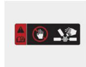
The electric motor (cooling fan) is controlled by coolant temperature, refrigerant pressure and vehicle speed. It may sometimes operate even when the vehicle is not operating. Use extreme caution when working near the blades of the cooling fan so that you are not injured by a rotating fan blades. As the coolant temperature decreases, the electric motor will automatically shut off. This is a normal condition.
