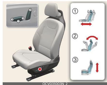
The front seat can be adjusted by using the control switches located on the outside of the seat cushion.
