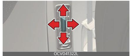
The outlet vents can be opened or closed by moving the vent left or right. Also, you can adjust the direction of air delivery from these vents using the vent control lever as shown.
