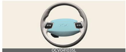
The horn will operate only when this area is pressed. Check the horn regularly to be sure it operates properly.
