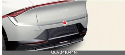
The wide-rear view camera is used as a detecting sensor to detect pedestrians. If the camera lens is covered with foreign material, such as snow or rain, it may adversely affect camera performance and Reverse Parking Collision-Avoidance Assist may not operate normally. Always keep the camera lens clean.
