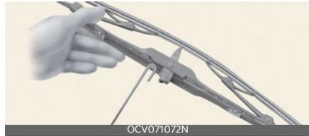
4. Install the blade assembly in the reverse order of removal.
