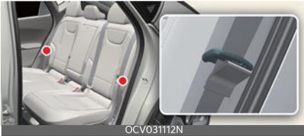
4. Pull on the seatback folding lever, then fold the seat toward the front of the vehicle. When you return the seatback to its upright position, always be sure it has locked into position by pushing on the top of the seatback.
