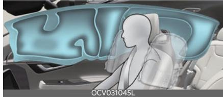
Side and/or curtain air bags are designed to inflate when an impact is detected by side collision sensors
