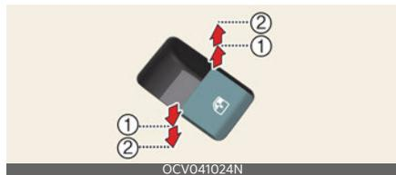
Pressing or pulling up the power window switch momentarily to the second detent position (2) completely lowers or raises the window even when the switch is released. To stop the window at the desired position while the window is in operation, pull up or press down and release the switch.
