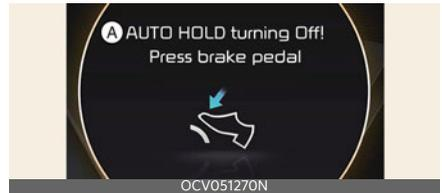
**A: AUTO HOLD turning Off! Press brake pedal**
