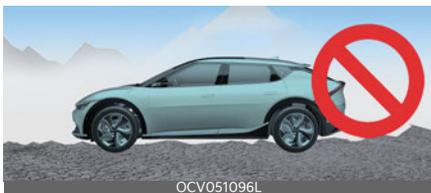
Remote Smart Parking Assist may cancel when the vehicle slips, or the vehicle cannot move due to road conditions such as pebbles or fragmented stones.
