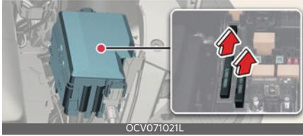
If the multi fuse is blown, it must be removed as follows:
