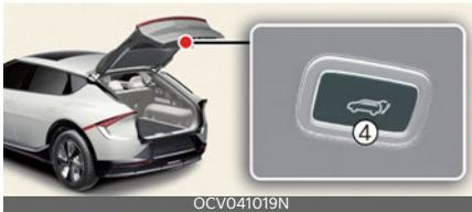
Press the power liftgate open/close button. The liftgate opens or closes with a warning sound.
