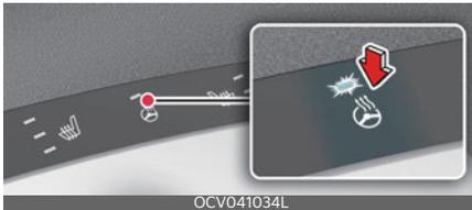
To turn the heated steering wheel off, press the button once again. The indicator on the button will turn off.
