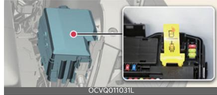
The high voltage cut-off switch is located in the motor room compartment fuse box.
