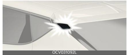
When all doors are locked and closed, the body silhouette lamp will come on for 15 seconds if any of the below is performed.
