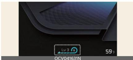
Initial setting of the regenerative braking level and adjustable range vary according to the selected Drive mode.
