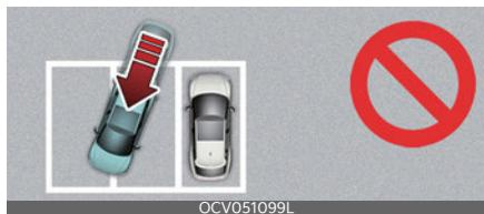
If Remote Smart Parking Assist is used, when parking in a parking space with a vehicle only on one side, your vehicle may cross the parking line to avoid the parked vehicle.
