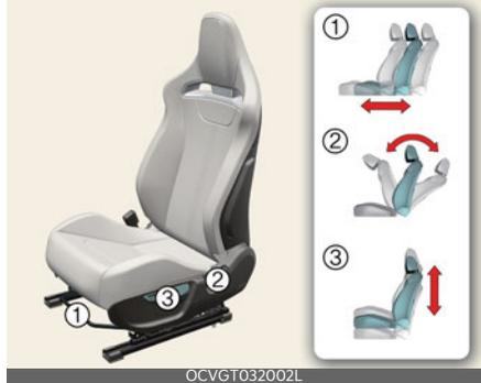
The front seat can be adjusted by using the control levers located on the outside of the seat cushion.
