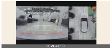
1. Press the Parking/View (P) button when the vehicle is stopped by depressing the brake pedal.
