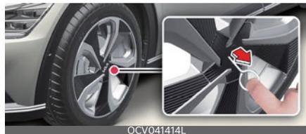
For 20 inch wheel, take out the remover tool in the Tire Mobility Kit. Insert the tool to the hole and pull out the wheel cover.
