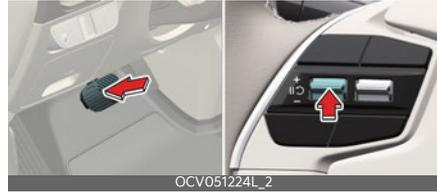
Press the (||) switch or depress the brake pedal to temporarily cancel Smart Cruise Control.
