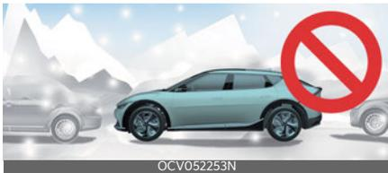
Snow may interfere with sensor operation, or Remote Smart Parking Assist may cancel if the road is slippery while parking.
