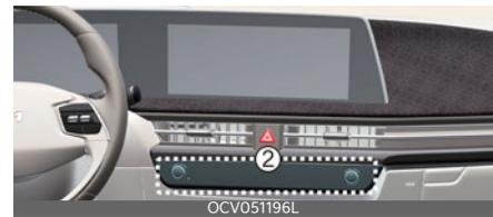
Front view function is displayed on the screen when the gear is in N (Neutral) or D (Drive) to assist in parking. The front view has a top view, front view, side view and 3D view. Also, other view modes can be selected by pressing the view icons on the Surround View Monitor screen.
