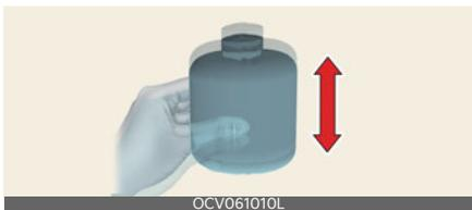
2. Remove the sealant bottle cap and sealant bottle holder cap and screw the bottle onto the sealant bottle holder.
