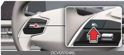
Press the Driving Assist (Ⓜ) button to turn on the function. The speed will be set to the current speed on the cluster.
