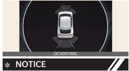
Reverse Parking Collision-Avoidance Assist operates only once after the gear is shifted to R (Reverse). To reactivate Reverse Parking Collision-Avoidance Assist, shift the gear from another gear to R (Reverse).
