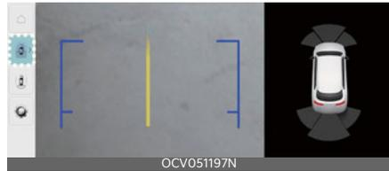
Rear top view shows the distance from the vehicle or the object in the back of your vehicle while parking.
