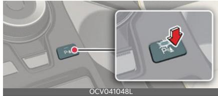
Press and hold the Parking Safety (P) button for more than 2 seconds to turn Active rear assist or Rear Warning Only on or off.
