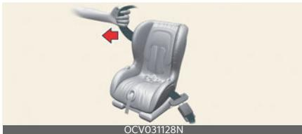
4. Slowly allow the shoulder portion of the seat belt to retract and listen for an audible "clicking" or "ratcheting" sound. This indicates that the retractor is in the "automatic locking" mode. If no distinct sound is heard, repeat steps 3 and 4.
