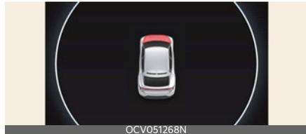
The warning chime will operate when the vehicle is being driven above 2 mph (3 km/h) with the hood open.
