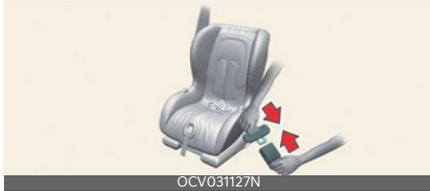
3. Pull the shoulder portion of the seat belt all the way out. When the shoulder portion of the seat belt is fully extended, it will shift the retractor to the "automatic locking" (child restraint) mode.
