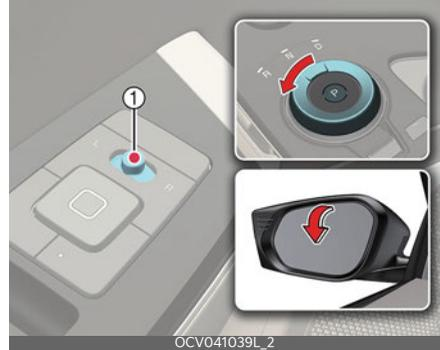
The position of the outside rear view mirror switch (1) determines whether or not the mirrors will move:
