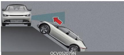
Rear Cross-Traffic Collision-Avoidance Assist may be limited when the vehicle is on an uphill or downhill slope, or near it, and may not detect the vehicle approaching from the blind spot area. If this occurs, the function
