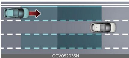
Blind-Spot Collision-Avoidance Assist helps detect and inform the driver that a vehicle is approaching at high speed from the blind spot area.
