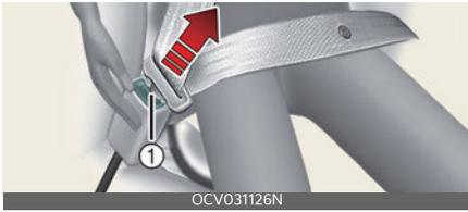
The seat belt is released by pressing the release button (1) on the locking buckle. When it is released, the belt should automatically draw back into the retractor. If this does not happen, check the belt to make sure it is not twisted, then try again.
