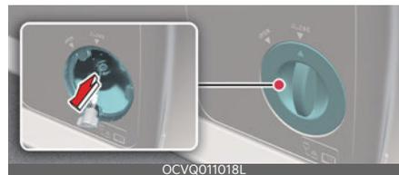
If the charging cable does not detach due to battery discharge and failure of the electric wires, open the liftgate and slightly pull the emergency cable on the right side area as shown above. The charging connector will then unlock.
