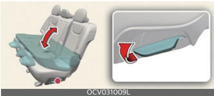
5. To use the rear seat, lift and unfold the seatback to the upright position by pulling up the folding lever. Push the seatback firmly until it clicks into place. Make sure the seatback is locked in place.
