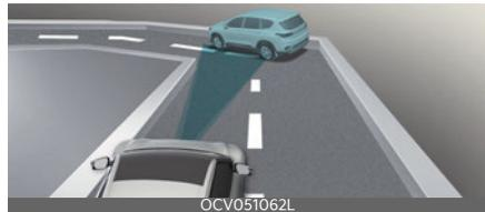
Your vehicle speed can be reduced due to a vehicle in the adjacent lane. Check to be sure that the road conditions permit safe operation of the Smart Cruise Control and if necessary, depress the brake pedal to reduce your driving speed in order to maintain a safe distance.
