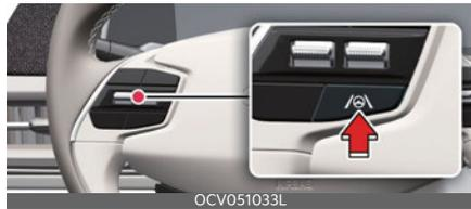
With the vehicle on, press and hold the Lane Driving Assist button located on the steering wheel to turn on Lane Keeping Assist. The gray ( / ) indicator light will appear on the cluster.
