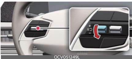
Push the - switch down and release it immediately. The set speed will decrease by 1 mph (1 km/h) each time the switch is operated in this manner.
