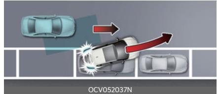
When you are driving forward out of a parking space, if Blind-Spot Collision-Avoidance Assist judges that there is a collision risk with an approaching vehicle in the blind spot, it will help avoid collision by applying the brake.
