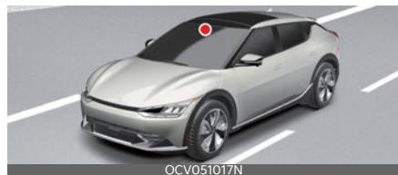
The front view camera is used as a detecting sensor to detect ambient light and brightness while driving. Refer to the picture above for the detailed location of the detecting sensor.
