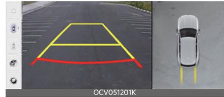
Surround View Monitor can assist in parking by allowing the driver to see around the vehicle.
