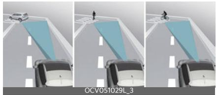
Forward Collision-Avoidance Assist may not detect other vehicles, pedestrians or cyclists in front of you on curved roads adversely affecting the performance of the sensors. This may result in no warning, braking assist or steering assist (if equipped) when necessary.
