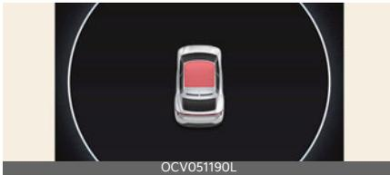
If the driver turns off the vehicle when the sunroof is not fully closed, the warning chime will sound for several seconds and the sunroof open warning will appear on the cluster LCD display.
