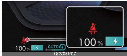
If the driver continues not to fasten the seat belt, the warning light will stay illuminated and the warning chime will sound for approximately 6 seconds until the belt is fastened each time the EV button is in ON. This will happen every time the EV button is in ON.
