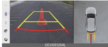
Parking distance warning is displayed on the right side of the Surround View Monitor top view screen when the **Parking Distance Warning** is selected.
