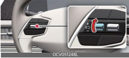
Push the + switch up and release it immediately. The set speed will increase by 1 mph (1 km/h) each time the switch is operated in this manner.
