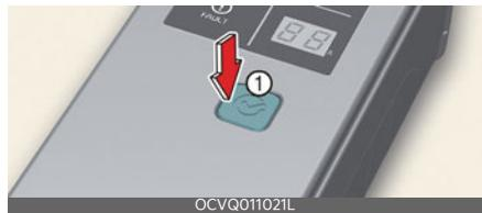
5. Each time the button (1) is pressed, the control box display is sequentially changed to 12 A, 10 A and 8 A. Once the charging current setting is complete, start charging (refer to "Portable charge (sold separately)" on page 1-32 for more information).
