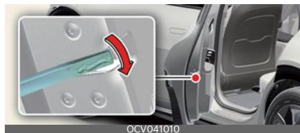
In case of emergency such as when the battery is discharged, the only way to lock the door(s) is with the mechanical key from the outside key hole. Doors without an outside key hole can be locked as follows:
