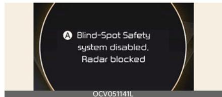
**A: Blind-Spot Safety system disabled. Radar blocked**
