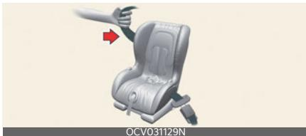
5. Remove as much slack from the belt as possible by pushing down on the child restraint system while feeding the shoulder belt back into the retractor.
