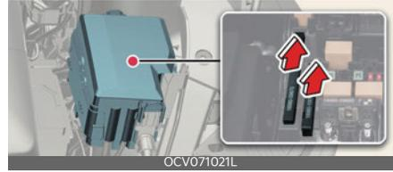
If the main fuse is blown, it must be removed as follows:
