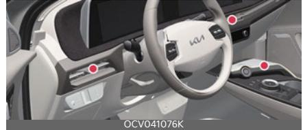
The ambient lights are installed in the front crash pad, front doors, and the top/bottom of the center console.
