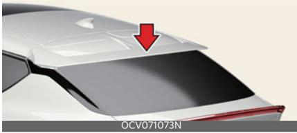
If the high mounted stop lamp (LED) does not operate, have your vehicle checked by an authorized Kia dealer. The LED lamp cannot be replaced as a single component because it is an integrated unit. The LED lamp has to be replaced with the unit.
