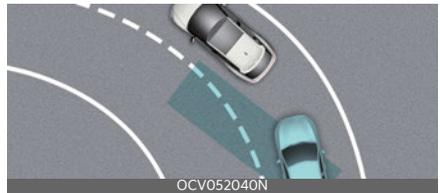
Blind-Spot Collision-Avoidance Assist may not operate properly when driving on a curved road. Blind-Spot Collision-Avoidance Assist may detect a vehicle in the same lane.
