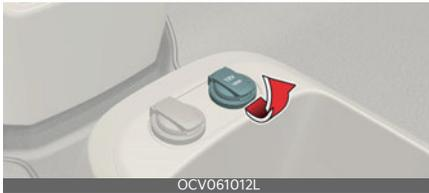
7. With the EV button ON, switch on the compressor and let it run for approximately 5~7 minutes to fill the sealant up to cold tire recommended pressure. (refer to "Tires and wheels" on page 9-4). Be careful not to overinflate the tire and stay away from the tire when filling it.
