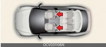
The headrest not only provides comfort for the driver and front passenger, but also helps protect the head and neck in the event of a rear collision.
