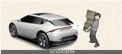
If you are positioned in the detecting area (20~40 inches [50~100 cm] behind the vehicle) carrying a smart key, the hazard warning lights will blink and chime will sound to alert you the smart key has been detected and the liftgate will open.
