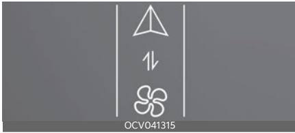
Press the button on the switchable controller to switch between infotainment system or climate control panel. Press and hold the button to select the default mode for the control panel.
