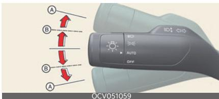
Highway Lane Change Assist function will operate, when you push the turn signal lever up or down while the function is in the ready state (( ) indicator is green), and all of the following conditions are satisfied:
