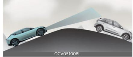
When driving uphill or downhill, the system may not detect the vehicle in your lane and the regenerative braking level will reduce automatically, making you feel that the vehicle is accelerating.
