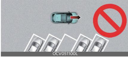
Remote Smart Parking Assist does not provide diagonal parking. Even if your vehicle was able to enter the parking space, do not use the function because the function cannot operate normally.
