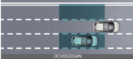
Blind-Spot Collision-Avoidance Assist helps detect and inform the driver that a vehicle is in the blind spot.
