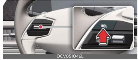
Press the Driving Assist (DA) button to turn Manual Speed Limit Assist off. The Speed Limit indicator (LIMIT) will go off.
