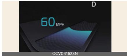
The speedometer indicates the speed of the vehicle and is calibrated in miles per hour (mph) and/or kilometers per hour (km/h).
