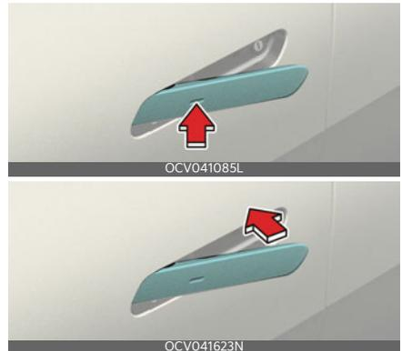
When all doors are closed, touch the touch sensor on the front outside door handle (the engraved part) while carrying the smart key with you, outside door handle will return and doors will be locked.
