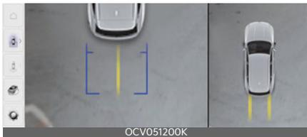
Parking guidance is displayed on the right side of the Surround View Monitor screen when the **Front or Rear Top View Parking Guidance** is selected.
