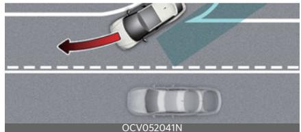
Blind-Spot Collision-Avoidance Assist may not operate properly when driving where the road merges or divides. Blind-Spot Collision-Avoidance Assist
