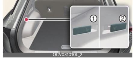
Pull the rear seatback folding switch (1, 2) located on both sides of the cargo area.
