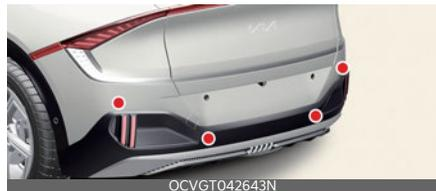
The rear ultrasonic sensors are located inside the rear bumper to detect objects in the rear area. If the sensors are covered with foreign material, such as snow or rain, it may adversely affect sensor performance and Reverse Parking Collision-Avoidance Assist may not operate normally. Always keep the rear bumper clean.
