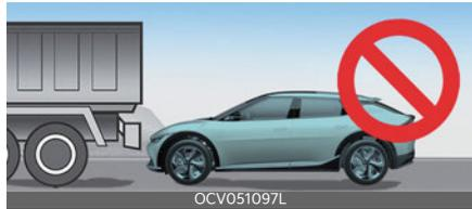
Do not use Remote Smart Parking Assist around vehicles with higher ground clearance, such as a bus, truck, etc. It may lead to an accident.
