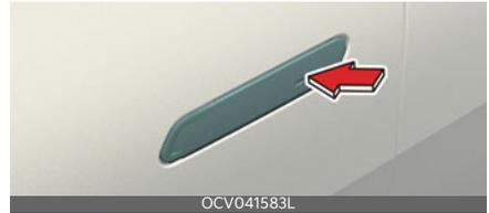
Push the button on the front outside door handle (the engraved part) while carrying the smart key with you, all doors will lock.
