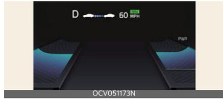
If temporary deceleration is required in the standby state and Navigation-based Smart Cruise Control is operating, the green (NAV) symbol will appear on the cluster.
