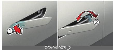
Press the front part (1) of the door handle to pull out the rear part of the door handle. While keep pressing the front part of the door handle, insert the mechanical key (2) to the lock with the key handle facing the ground as shown. To lock the door, turn the key toward the front (left side) of the vehicle. To unlock, turn the key toward the rear (right side) of the vehicle.
