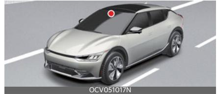
The front view camera is used as a detecting sensor to detect lane markings (or road edges).
