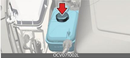
Replace any swollen or deteriorated hoses. The coolant level should be filled between F (MAX) and L (MIN) marks on the side of the coolant reservoir when motor compartment is cool. When the coolant level (in the reservoir) is low, have your vehicle inspected by an authorized Kia dealer. Use only designated coolant water for electric vehicles, adding other types of water or anti-freeze can damage the vehicle.
