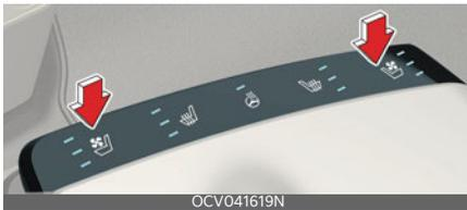
The temperature setting of the seat changes according to the button indicator.
