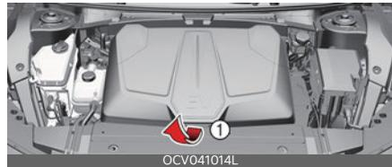
2. Remove the cover by pulling the upper part of the cover.
