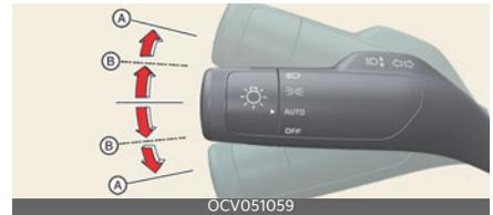
Blind-Spot View Monitor will turn on and off when the turn signal is turned on and off.
