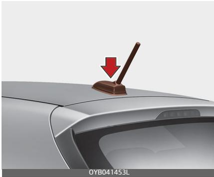
The micro pole antenna transmits and receives wireless signals such as AM/FM, DAB, GNSS, etc. The antenna pole is a removable type. To remove the antenna pole, turn it counterclockwise. To install the antenna, turn it clockwise.
