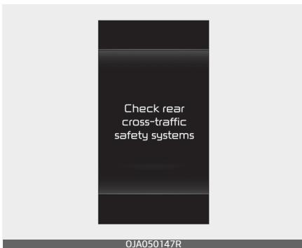
When Rear Cross-Traffic Safety system is not working properly, the 'Check Rear cross-traffic safety system' warning message will appear on the cluster, and the function will turn off automatically or the function will be limited. In this case, have your vehicle inspected by a professional workshop. Kia recommends to contact an authorised Kia dealer/service partner.
