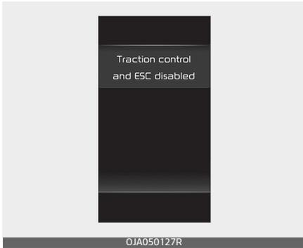
Press the ESC OFF button for more than 3 seconds. ESC OFF indicator light and message illuminate and ESC OFF warning chime will sound. At this state, the engine control function and brake control function does not operate. In other words, the vehicle stability control function does not operate any more.
