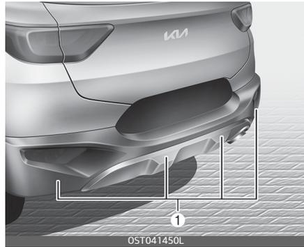
Reverse Parking Distance Warning assists the driver during backward movement of the vehicle by chiming if any object is sensed within a distance of 120 cm (48 inches) behind the vehicle.
