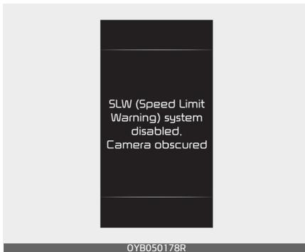
The message will appear when camera's field of view is covered by some objects. The function stops until the field of view is normal. Check the windscreen around the camera view area. If the function does not work normally even though camera's field of view is cleared, have the function checked by a professional workshop. Kia recom-
