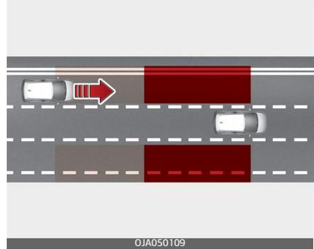
Blind-Spot Collision Warning help detects and informs the driver that a vehicle is approaching at high speed from the blind spot area.
