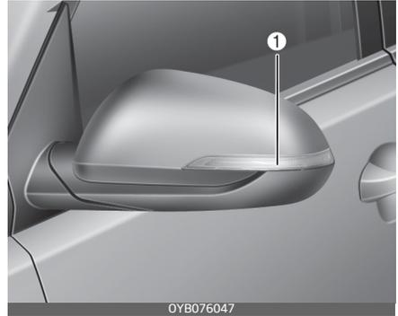
If the side repeater lamp (LED) (1) does not operate, have your vehicle checked by a professional workshop.
