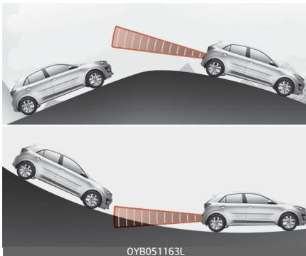
Blind-Spot Safety system may not operate properly when driving on a slope. The function may not detect the vehicle in the next lane or may
