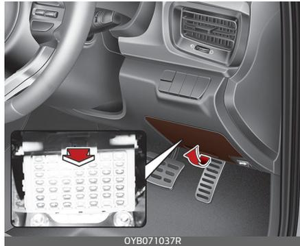
Your vehicle is equipped with a memory fuse to prevent battery discharge if your vehicle is parked without being operated for prolonged periods. Use the following procedures before parking the vehicle for prolonged periods.
