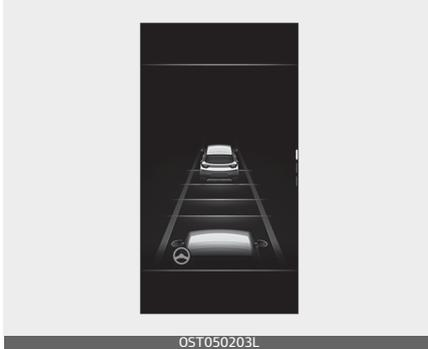
If the vehicle ahead or both lane markings are detected and your vehicle speed is below 200 km/h (120 mph), the green (🚗) indicator light will illuminate on the cluster, and the function will help the vehicle stay in lane by controlling the steering wheel.
