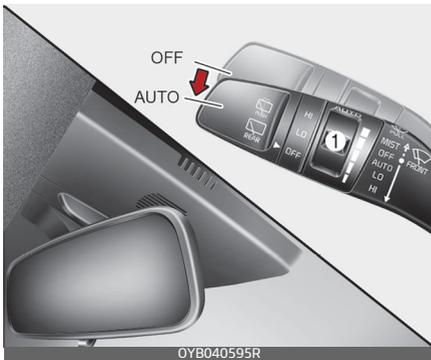
The rain sensor located on the upper end of the windscreen glass senses the amount of rainfall and controls the wiping cycle for the proper interval. The more it rains, the faster the wiper operates. When the rain stops, the wiper stops.
