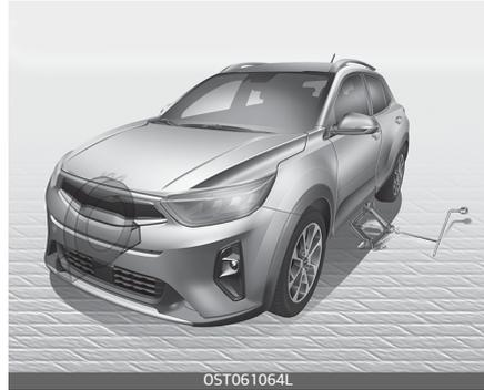
5. Block both the front and rear of wheel that is diagonally opposite the jack position.
