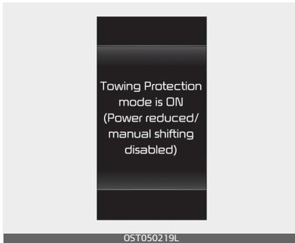
If the above warning message appears during towing of the trailer, to prevent overheating of the engine/transmission, power may be limited or manual transmission may not be available.
