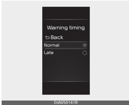
The driver can select the initial warning activation time in the User Settings in the LCD display by selecting 'User settings → Driver assistance → Warning timing'. The options for the initial Inattentive Driving Warning includes the following:
