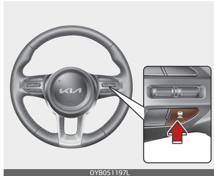
Each time the Vehicle Distance button is pressed, the Vehicle Distance changes as follows:
