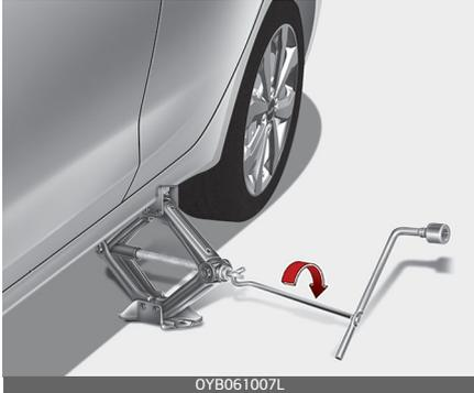
9. Loosen the wheel nuts and remove them with your fingers. Slide the wheel off the studs and lay it flat so it cannot roll away. To put the wheel on the hub, pick up the spare tyre, line up the holes with the studs and slide the wheel onto them. If this is difficult, tip the wheel slightly and get the top hole in the wheel lined up with the top stud. Then jiggle the wheel back and forth until the wheel can be slid over the other studs.
