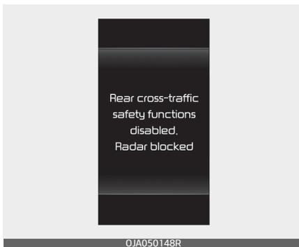
When the rear bumper around the rear-side radar or sensor is covered with foreign matters, such as snow or rain, or installing a trailer or carrier, it can reduce the detecting per-
