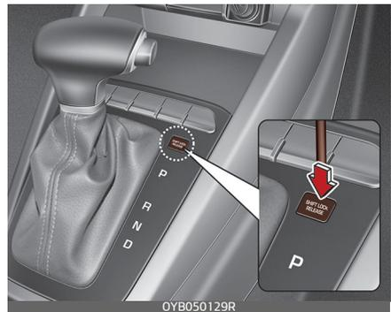
If the shift lever cannot be moved from the P (Park) or N (Neutral) position into R (Reverse) position with the brake pedal depressed, continue depressing the brake, then do the following:
