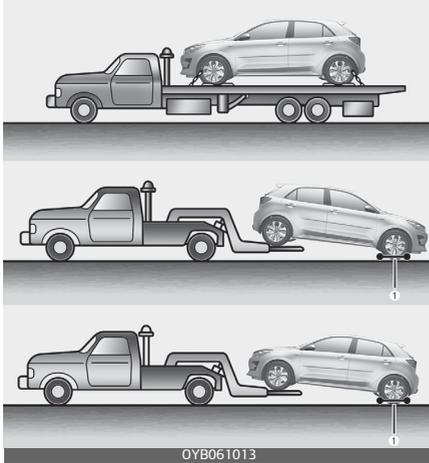
If emergency towing is necessary, we recommend having it done by an authorised Kia dealer or a commercial tow-truck service. Proper lifting and towing procedures are necessary to prevent damage to the vehicle. The use of wheel dollies (1) or flatbed is recommended.
