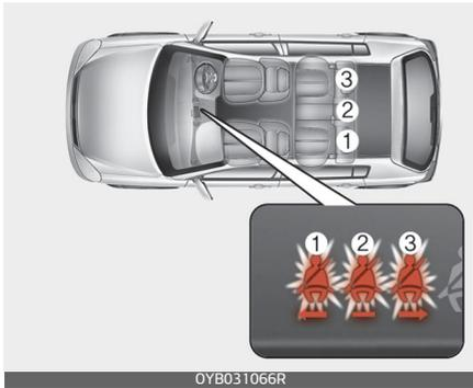
As a reminder to the rear passenger, the rear passenger's seat belt warning lights will illuminate for approximately 6 seconds each time you turn the ignition switch ON regardless of belt fastening.
