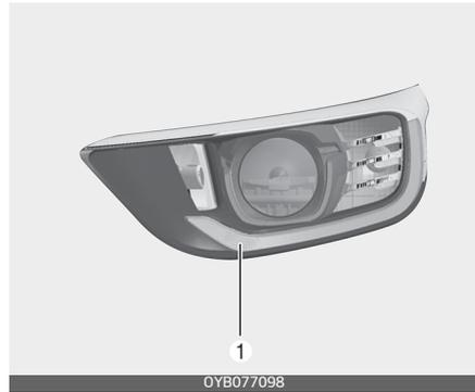
If the position lamp/daytime running lamp (LED) (1) does not operate, have your vehicle checked by a professional workshop.
