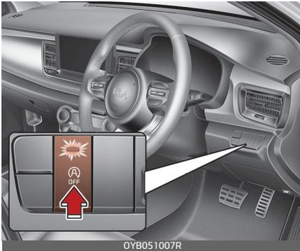
The engine will not start if the shift lever is moved from the N (neutral) stage to the D (driving) stage, manual mode, or R (reverse) stage without stepping on the brake pedal whilst the engine is stopped automatically. At this time, if you press the brake it will be restarted.
