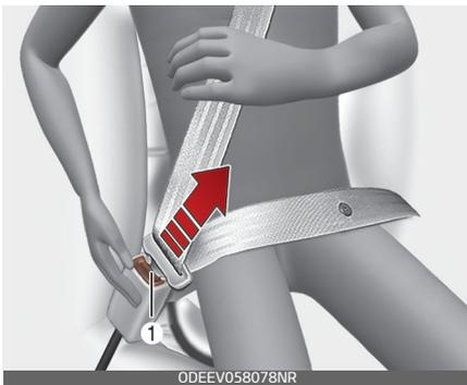
The seat belt is released by pressing the release button (1) on the locking buckle. When it is released, the belt should automatically draw back into the retractor.
