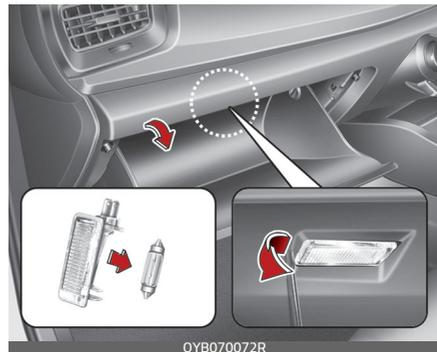
1. Using a flat-blade screwdriver, gently pry the lamp assembly from interior.
