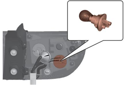
8. Install the socket in the assembly by aligning the tabs on the socket with the slots in the assembly. Push the socket into the assembly and turn the socket clockwise.
