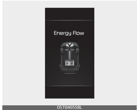
Both the motor and the engine power are used to drive the vehicle. (Battery & Engine → Wheel)
