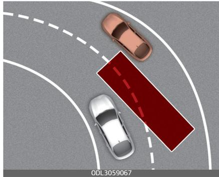
Blind-Spot Safety system may not operate properly when driving on a curved road. The function may not detect the vehicle in the next lane. Always pay attention to road and driving conditions whilst driving.
