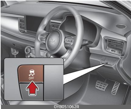
Electronic Stability Control (ESC) is designed to stabilize the vehicle during cornering manoeuvres. ESC checks where you are steering and where the vehicle is actually going.
