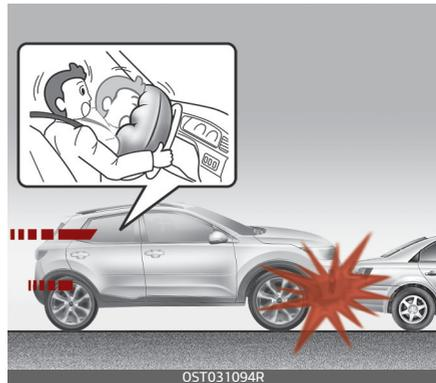
Front air bags are designed to inflate in a frontal collision depending on the intensity, speed or angles of impact of the front collision.
