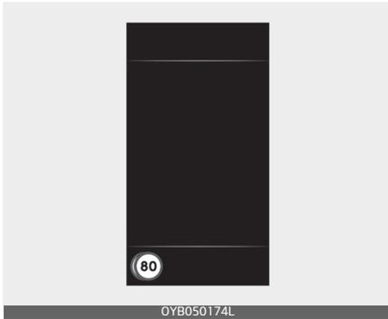
If ISLW detects a conditional road sign, the symbol of road sign is overlapped at the bottom or left of the speed limit on the cluster. There may be signs with different speed limits on the same road. For example, normally, the speed limit is 120 km/h (75 mph), however the speed limit is 90 km/h (55 mph) when it is raining or snowing. The conditional road sign means that you observe the speed limit and overtaking prohibition on certain conditions, such as when rain or snow.
