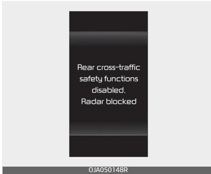
When the rear bumper around the rear-side radar or sensor is covered with foreign matters, such as snow or rain, or installing a trailer or carrier, it can reduce the detecting performance and temporarily limit or disable Rear Cross-Traffic Safety system.
