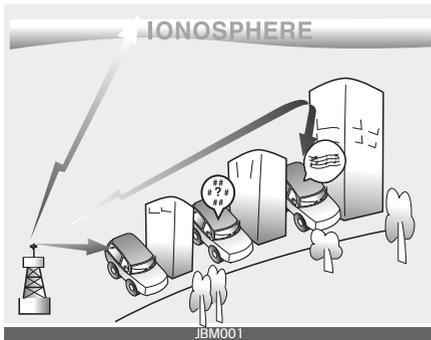
AM and FM radio signals are broadcast from transmitter towers located around your city. They are intercepted by the radio antenna on your vehicle. This signal is then
