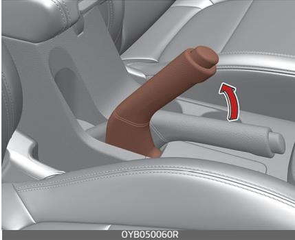
Check the stroke of the parking brake by counting the number of “clicks” heard whilst fully applying it from the released position. Also, the parking brake alone should securely hold the vehicle on a fairly steep grade. If the stroke is more or less than specified, have the system serviced by a professional workshop. Kia recommends to visit an authorised Kia dealer/service partner.
