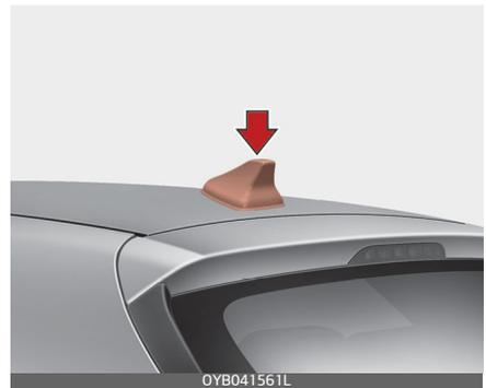
The shark fin antenna transmits and receives wireless signals such as AM/FM, DAB, GNSS, etc.
