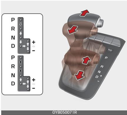
➡ Depress the brake pedal and the lock release button when shifting.
