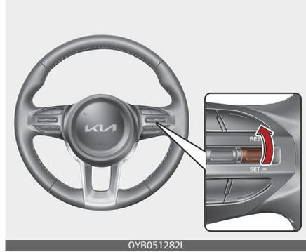
If any method other than the switch was used to cancel cruising speed and the function is still activated, the cruising speed will automatically resume when you move the switch up. If you move up the RES+ switch, the speed will resume to the recently set speed. Vehicle speed must be above 10 km/h (5 mph) for the function to resume.
