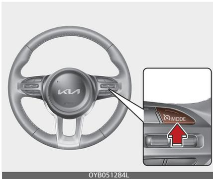
Press the Driving Assist button to turn Smart Cruise Control off.
