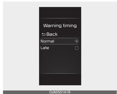
With the ignition switch or ENGINE START/STOP button in the ON position, select 'Driver assistance → Warning timing' from the Settings menu to change the initial warning activation time for Blind-Spot Safety system.
