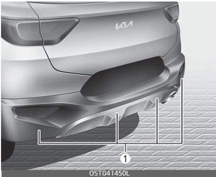
Forward/Reverse Parking Distance Warning assist the driver during movement of the vehicle by chiming if any object is sensed within the distance of 100 cm (40 inches) in front and 120 cm (48 inches) behind the vehicle.
