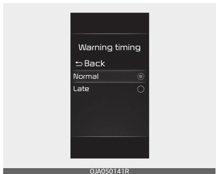
With the ignition switch or ENGINE START/STOP button in the ON position, select 'Driver assistance → Warning timing' from the Settings menu to change the initial warning
