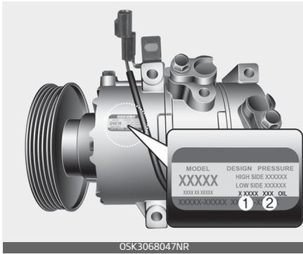
A compressor label informs you the type of compressor your vehicle is equipped with such as model, supplier part number, production number, refrigerant (1) and refrigerant oil (2).
