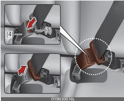
Pull the metal tab (3) and insert it (3) into the buckle (4). There will be an audible “click” when the tab locks into the buckle. Make sure the belt is not twisted. When using the rear centre seat belt the buckle with the “CENTER” mark must be used.
