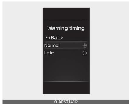
The driver can select the initial warning activation time in the User Settings in the instrument cluster LCD display.
