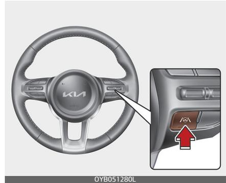
With the ignition switch or ENGINE-START/STOP button in the ON position, press and hold the Lane Driving Assist button (LKA) located on the steering wheel to turn on Lane Keeping Assist.
