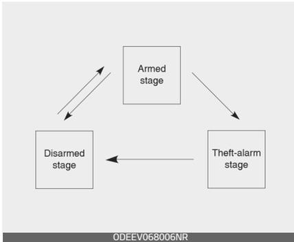
This system is designed to provide protection from unauthorised entry into the car. This system is operated in three stages: the first is the “Armed” stage, the second is the “Theft-alarm” stage, and the third is the “Disarmed” stage. If triggered, the system provides an audible
