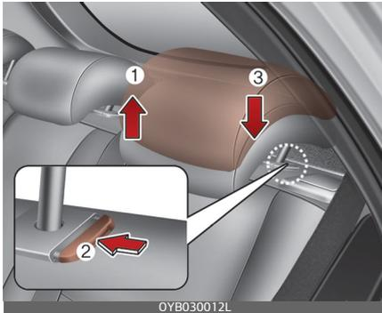
To raise the headrest, pull it up to the desired position (1). To lower the headrest, push and hold the release button (2) on the headrest support and lower the headrest to the desired position (3).
