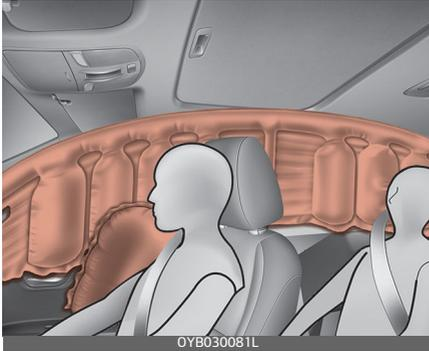
Side and curtain air bags are designed to inflate when an impact is detected by side collision sensors depending on the strength, speed or angles of impact resulting from a side impact collision.
