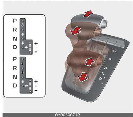
Whether the vehicle is stationary or in motion, sports mode is selected by pushing the shift lever from the D (Drive) position into the manual gate. To return to D (Drive) range operation, push the shift lever back into the main gate.
