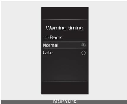
With the ignition switch or ENGINE START/STOP button in the ON position, select 'Driver assistance → Warning timing' from the Settings menu to change the initial warning activation time for Rear Cross-Traffic Safety system.
