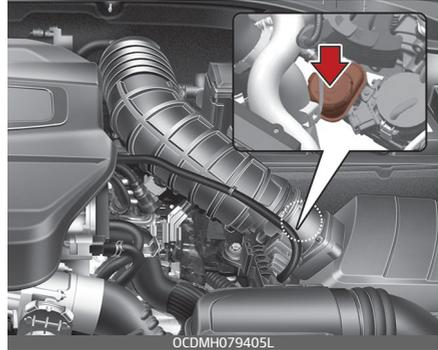
In normal driving conditions, the actuator fluid level does not go down rapidly.
