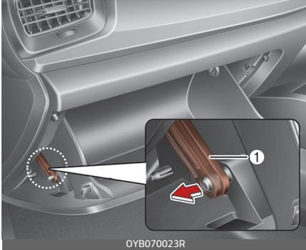
3. Remove the climate control air filter cover whilst pressing the lock on the right side of the cover.
