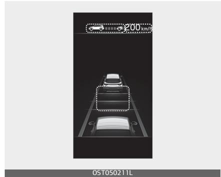
If you want to speed up temporarily when Smart Cruise Control is on, depress the accelerator pedal. Whilst the speed is increasing, the set speed, distance level and target distance will blink on the cluster.
