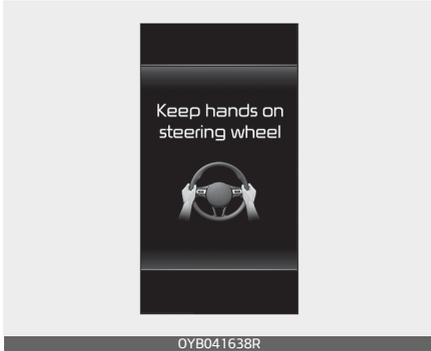
If the driver takes hands off the steering wheel for several seconds whilst LKA is activated, the function will warn the driver.
