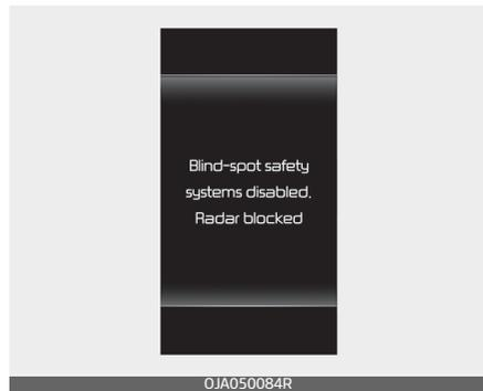
When the rear bumper around the rear corner radar or sensor is covered with foreign material, such as snow or rain, or installing a trailer or carrier, it can reduce the detecting performance and temporarily limit or disable Blind-Spot Safety system.
