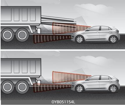
When the vehicle in front has heavy loading extended rearward, or when the vehicle in front has higher ground clearance, it may induce a hazardous situation. Always pay attention to road and driving conditions, whilst driving and, if necessary, depress the brake pedal to reduce your driving speed in order to maintain distance.
