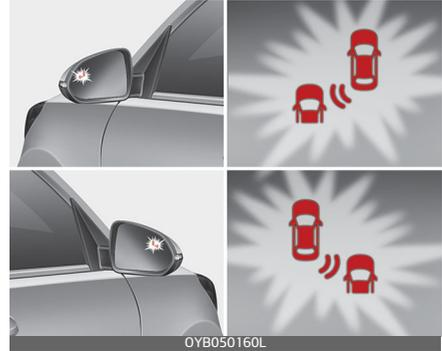
To warn the driver of an approaching vehicle from the rear left/right side of your vehicle, the outside rearview mirror will blink and a warning will appear on the cluster. At the same time, an audible warning will sound and the steering wheel will vibrate. If Rear View Monitor is operating, a warning will also appear on the infotainment screen.
