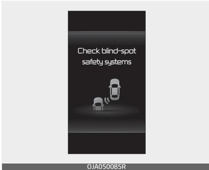
When Blind-Spot Safety system is not working properly, the 'Check blind-spot safety systems' warning message will appear on the cluster, and the function will turn off automatically, or the function will be limited. In this case, have your vehicle inspected by a professional workshop. Kia recommends to contact an authorised Kia dealer/service partner.
