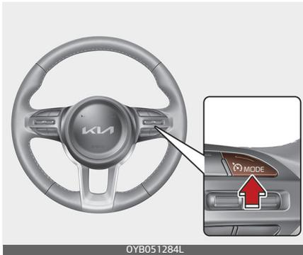
Press the Driving Assist button to turn Cruise Control off. The Cruise (Ⓢ) CRUISE) indicator will go off.
