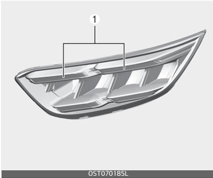
If the daytime running lamp/front turn signal lamp (LED) (1) does not operate, have your vehicle checked by a professional workshop.
