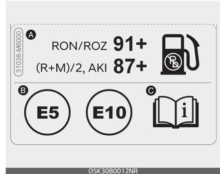
The fuel label is attached on the fuel filler door.
