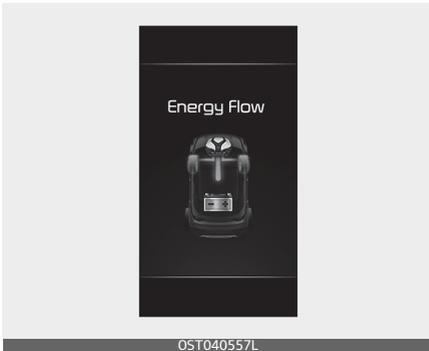
The engine and regenerative brake system charges up the high-voltage battery. (Engine & Wheel → Battery)
