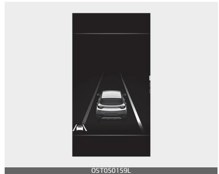
If the vehicle leaves a lane, the lane marker you cross will blink on the LCD display and the warning sound is provided.
