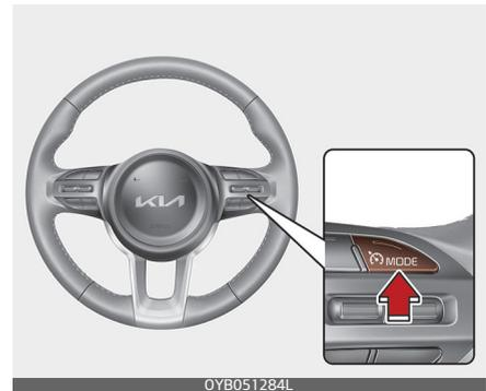
1. Press the Driving Assist button to turn the function on. The CRUISE indicator in the instrument cluster will illuminate.
