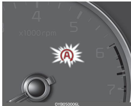
ISG System is indicated by lamp on the instrument cluster. If your vehicle is equipped with a supervision cluster, the notice will illuminate on the LCD display.
