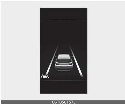
If the speed of the vehicle is over 60 km/h (37 mph) and the function detects lane markers, the colour changes from gray to white.
