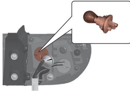
8. Install the socket in the assembly by aligning the tabs on the socket with the slots in the assembly. Push the socket into the assembly and turn the socket clockwise.
