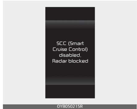
When the front radar cover or sensor is covered with snow, rain, or foreign matters, it can reduce the detecting performance and temporarily limit or disable Smart Cruise Control.
