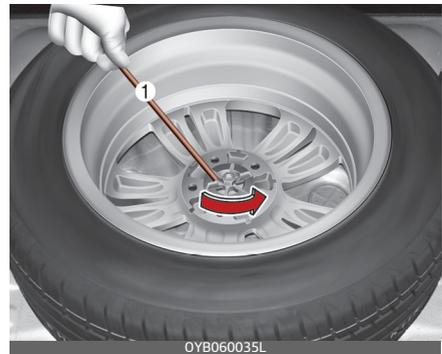
If it is hard to loosen the tyre hold-down wing bolt by hand, you can loosen it easily using the jack handle.
