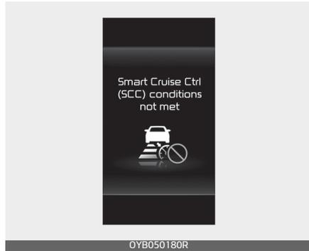
If the Driving Assist button, RES+ or SET- switch is pushed when the function's operating conditions are not satisfied, the 'Smart Cruise Ctrl (SCC) conditions not met' will appear on the cluster, and an audible warning will sound.
