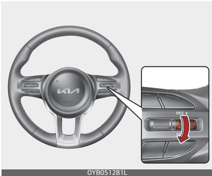
3. Move the switch up (to RES+) or down (to SET-), and release it at the desired speed. Move the switch up (to RES+) or down (to SET-) and hold it. The speed will increase or decrease by 5 km/h (3 mph).
