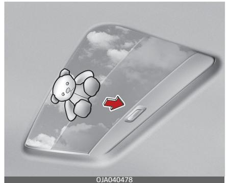
If the sunroof glass senses any obstacle whilst it is closing automatically, it will reverse direction then stop at a certain position.
