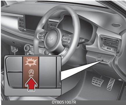
If you want to deactivate the ISG system, press the ISG OFF button. The light on the ISG OFF button will illuminate. If you press the ISG OFF button again, the function will be activated and the light on the ISG OFF button will turn off.
