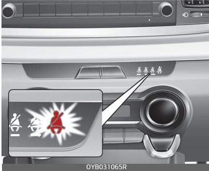
As a reminder to the front passenger, the front passenger's seat belt warning lights will illuminate for approximately 6 seconds each time you turn the ignition switch or ENGINE START/STOP button ON regardless of belt fastening.
