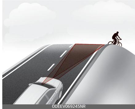
The performance of Forward Collision-Avoidance Assist may be decreased whilst driving upward or downward on a slope. The front view camera or front radar sensor recognition may not detect the vehicle, pedestrian or cyclist in front.
