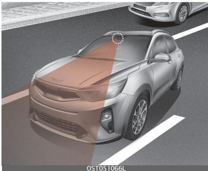
The front view camera is used as a detecting sensor to detect driving patterns and front vehicle departure whilst vehicle is being driven.
