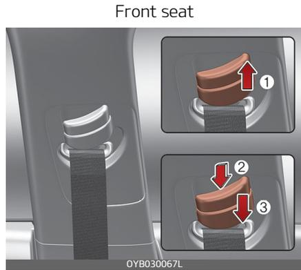
You can adjust the height of the shoulder belt anchor to one of the 3 positions for maximum comfort and safety.
