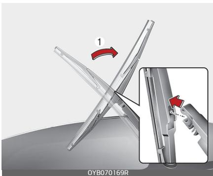
2. Install the new blade assembly by inserting the centre part into the slot in the wiper arm until it clicks into place.
