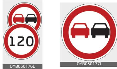
The symbol is displayed on the instrument cluster and the navigation, when ISLW detects a no overtaking sign.
