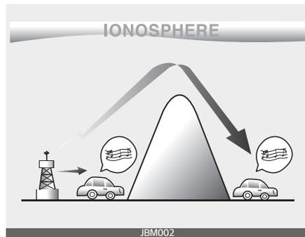
AM broadcasts can be received at greater distances than FM broadcasts. This is because AM radio waves are transmitted at low frequencies. These long, low frequency radio waves can follow the curvature of the earth rather than traveling straight out into the
