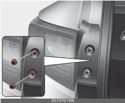
3. Remove the rear combination lamp assembly from the body of the vehicle.
