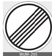
The symbol, 'end of limitation', is displayed on the instrument cluster for the roads in Germany, which have no speed limit applicable. It is displayed, until the vehicle passes by another speed limit sign.
