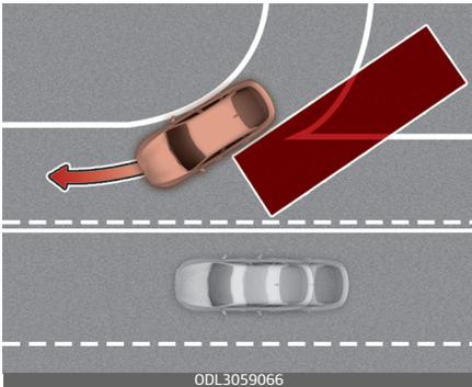
Blind-Spot Safety system may not operate properly when driving where the road merges or divides. The function may not detect the vehicle in the next lane. Always pay
