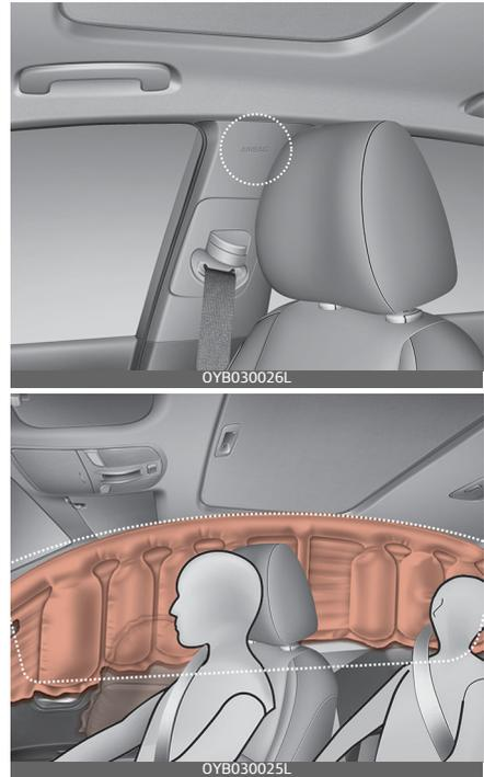
Curtain air bags are located along both sides of the roof rails above the centre pillar.
