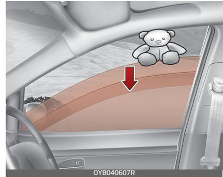
If the upward movement of the window is blocked by an object or part of the body, the window will detect the resistance and will stop upward movement. The window will then lower approximately 30 cm (11.8 inches) to allow the object to be cleared.
