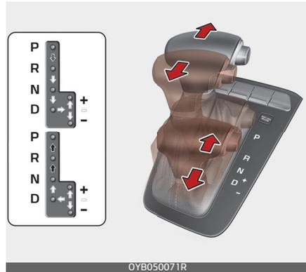
➡ To shift, depress the brake pedal and press the button.
