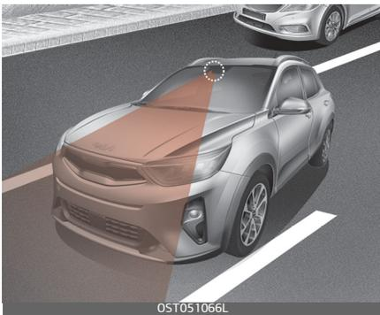
The front view camera is used as a detecting sensor to detect lane markings (or road edges). Refer to the picture above for the detailed location of the detecting sensor.
