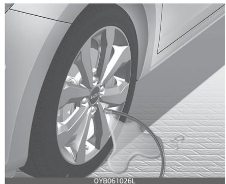
Securely install the sealant filling hose to the valve. If not, sealant
