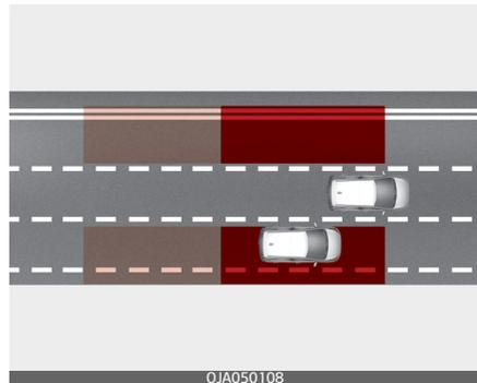
Blind-Spot Collision-Avoidance Assist help detects and informs the driver that a vehicle is in the blind spot.
