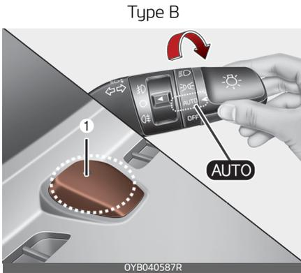
When the light switch is in the AUTO light position, the taillights and headlights will be turned ON or OFF automatically depending on the amount of light outside the vehicle.
