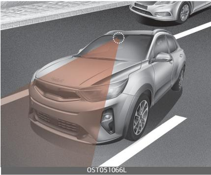
Intelligent Speed Limit Warning displays the speed limit information and overtaking restriction of the current road through the instrument cluster and the navigation. ISLW reads the traffic signs through the front view camera, which is attached on the upper part of the inner front windscreen. ISLW also utilizes the navigation and vehicle information to display the speed limit information.
