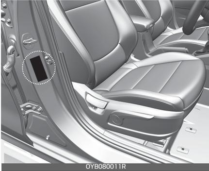
The vehicle certification label attached on the driver's (or front passenger's) side centre pillar gives the vehicle identification number (VIN).
