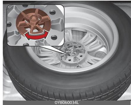
Turn the tyre hold-down wing bolt counterclockwise.
