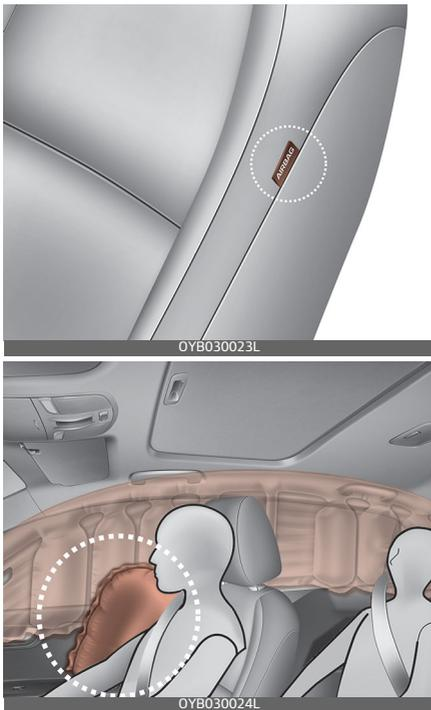
Your vehicle is equipped with a side impact air bag in each front seat. The purpose of the air bag is to provide the vehicle's driver and the front passenger with additional pro-
