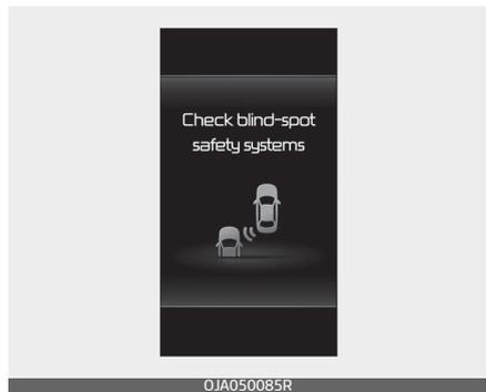
When Blind-Spot Safety system is not working properly, the 'Check blind-spot safety systems' warning
