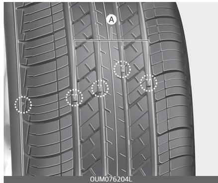
If the tyre is worn evenly, a tread wear Indicator (A) will appear as a solid band across the tread. This shows there is less than 1.6 mm (1/16 in.) of tread left on the tyre. Replace the tyre when this happens.
