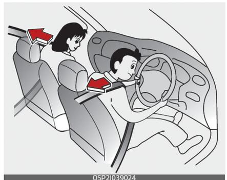
Your vehicle is equipped with pre-tensioner seatbelts at the front and rear outboard seating positions. The purpose of the pre-tensioner is to
