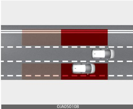
Blind-Spot Collision Warning help detects and informs the driver that a vehicle is in the blind spot.
