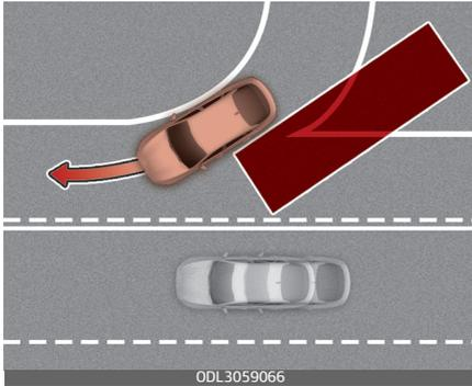
Blind-Spot Safety system may not operate properly when driving where the road merges or divides. The function may not detect the vehicle in the next lane.
