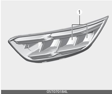
If the headlamp (Low beam) (LED) (1) does not operate, have your vehicle checked by a professional workshop.
