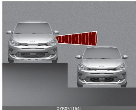
Blind-Spot Safety system may not operate properly when driving where the heights of the lanes are different. The function may not detect the vehicle on a road with different lane heights (underpass joining section, grade separated intersections, etc.).
