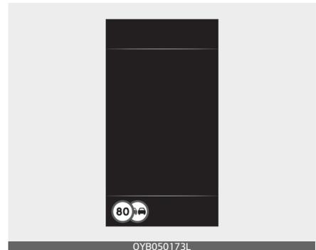
The cluster displays the speed limit information, overtaking restriction and conditional road sign.
