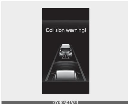
Whilst Smart Cruise Control is operating, when the collision risk with the vehicle ahead is high, the 'Collision warning!' warning message will appear on the cluster, and an audible warning will sound to warn the driver. Always have your eyes on the road whilst driving, and if necessary, depress the brake pedal to reduce your driving speed in order to maintain a safe distance.
