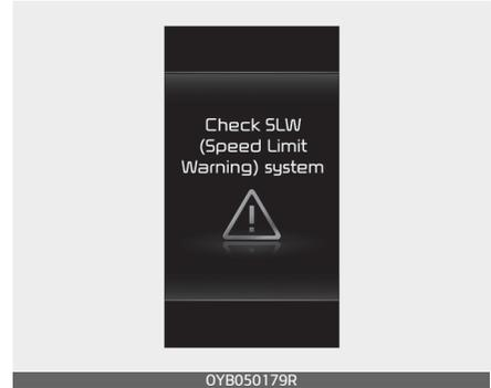
When ISLW is not working properly, the warning message will come on for a few second. After the message disappears, the master warning light will illuminate.
