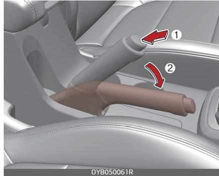
To release the parking brake, first apply the foot brake and pull up the parking brake lever slightly. Secondly depress the release button (1) and lower the parking brake lever (2) whilst holding the button.
