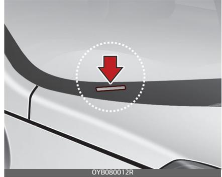
The VIN is also on a plate attached to the top of the dashboard. The number on the plate can easily be seen through the windscreen from outside.
