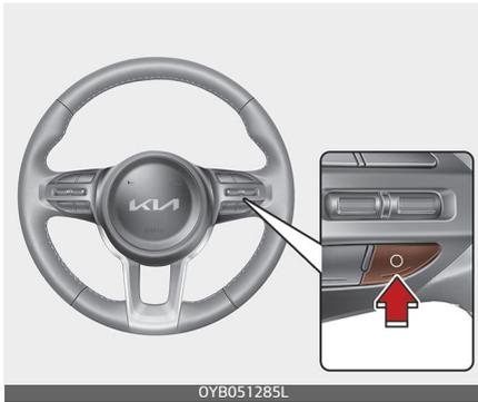
Press the (O) button or depress the brake pedal temporarily to cancel Smart Cruise Control.
