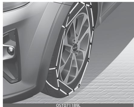
Since the sidewalls of radial tyres are thinner, they can be damaged by mounting some types of snow chains on them. Therefore, the use
