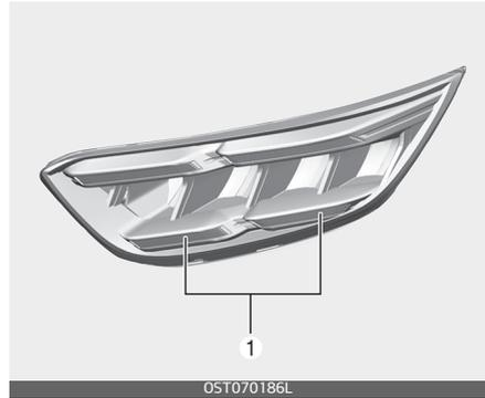
If the daytime running lamp/position lamp (LED) (1) does not operate, have your vehicle checked by a professional workshop.
