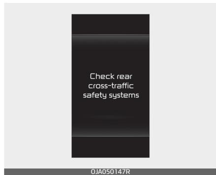
When Rear Cross-Traffic Safety system is not working properly, the 'Check rear cross-traffic safety systems' warning message will appear on the cluster, and the function will turn off automatically, or the function will be limited. In this case, have your vehicle inspected by a professional workshop. Kia recommends to contact an authorised Kia dealer/ service partner.
