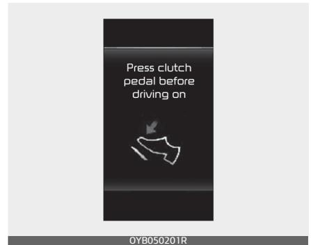
Unintentionally, when the engine is turned off or the vehicle is moving, if the gear is engaged and the clutch pedal is not pressed, the system displays the warning message as shown above. At this time, if the driver presses the clutch pedal all the way, the engine restarts automatically. (Only with Late Restart equipped ISG system, except MHEV)
