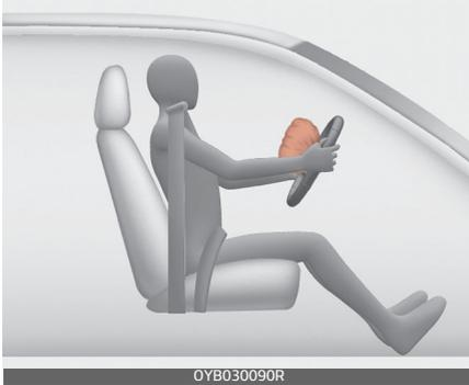
The air bag modules are located both in the centre of the steering wheel and in the front passenger's panel above the glove box. When the SRSCM detects a sufficiently severe impact to the front of the vehicle, it will automatically deploy the front air bags.
