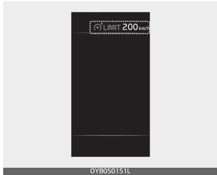
To drive over the preset speed limit you must depress hard on the accelerator pedal (more than approximately 80%) until the kick down mechanism works with a clicking noise. Then the set speed limit will blink and chime will sound until you return the vehicle speed within the speed limit.
