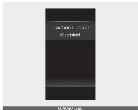
Press the ESC OFF button shortly (ESC OFF indicator light and message illuminates). At this state, the engine control function does not operate. In other words, the traction control function does not operate but only the brake control function operates.
