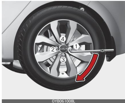
Then position the wrench as shown in the drawing and tighten the wheel nuts. Be sure the socket is seated completely over the nut. Do not stand on the wrench handle or use an extension pipe over the wrench handle. Go around the wheel tightening every other nut until they are all tight. Then double-check each nut for tightness. After
