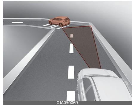
On curves, Smart Cruise Control may not detect a vehicle in the same lane, and may accelerate to the set speed. Also, vehicle speed may rapidly decrease when the vehicle ahead is detected suddenly.
