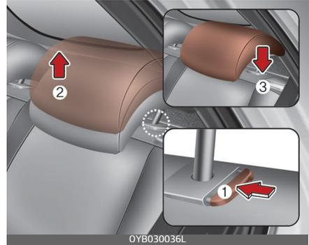
To remove the headrest, raise it as far as it can go then press the release button (1) whilst pulling upward (2).
