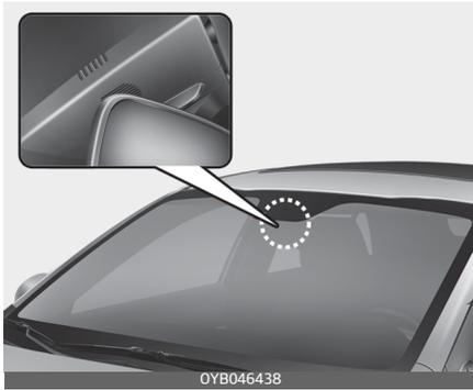
Auto defogging reduces the possibility of fogging up the inside of the windscreen by automatically sensing the moisture of inside the windscreen and air flow toward the windscreen can increase.
