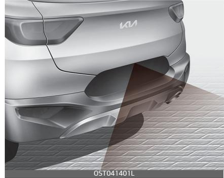
Rear View Monitor will activate when the engine is running and the shift lever is in the R (Reverse) position.
