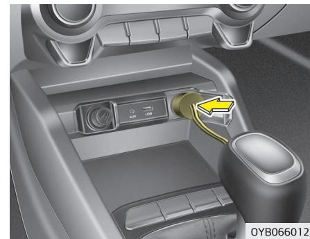
9. Connect between compressor and the vehicle power outlet using the cable and connectors.
