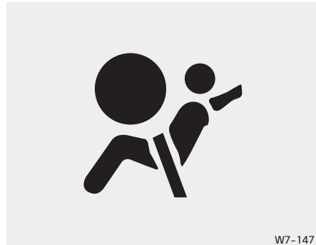
The purpose of the air bag warning light in your instrument panel is to alert you of a potential problem with your air bag - Supplemental Restraint System (SRS). When the ignition switch is turned ON, the warning light should illuminate for approximately 6 seconds, then go off. Have the system checked if:
