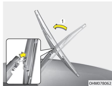
1. Raise the wiper arm (1) and pull out the wiper blade assembly.
