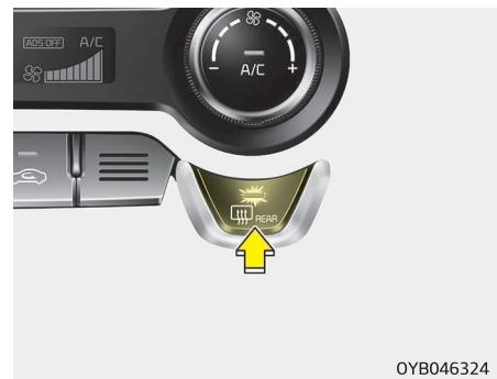
The rear window defroster automatically turns off after approximately 20 minutes or when the ignition switch is turned off. To turn off the defroster, press the rear window defroster button again.
