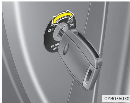
The passenger's front air bag can be deactivated by the passenger's front air bag ON/OFF switch if a child restraint is installed on the front passenger's seat or if the front passenger's seat is unoccupied by a person.
