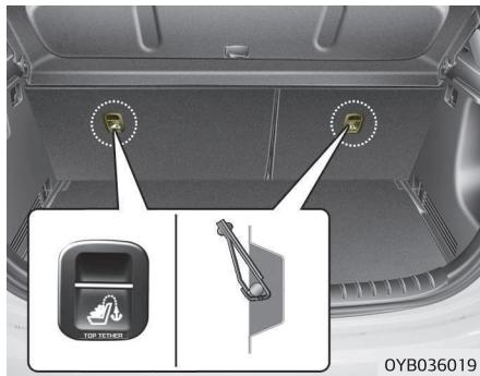
Child restraint system top tether anchorages are located on the back of the rear seatbacks.
