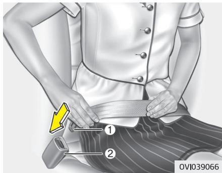
To fasten a 2-point static type belt, insert the metal tab (1) into the locking buckle (2). There will be an audible "click" when the tab locks into the buckle. Check to make sure the belt is properly locked and that the belt is not twisted.
