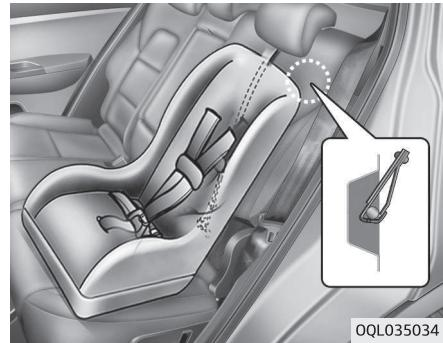
1. Route the Child Restraint System top-tether strap over the seatback. Placing the top tether strap, please follow the instructions of the Child Restraint System manufacturer.
