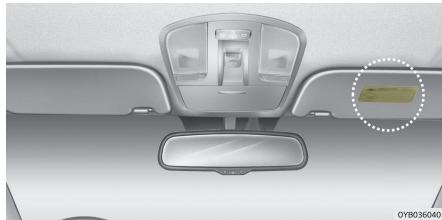
Air bag warning labels are attached to alert the driver and passengers of potential risk of air bag system.
