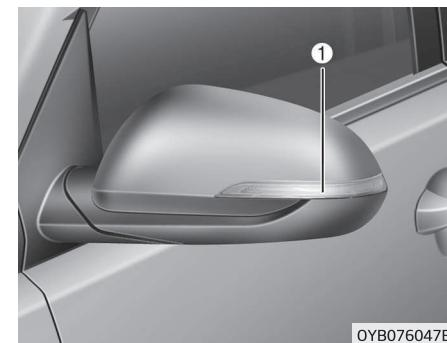
If the side repeater lamp (LED) (1) does not operate, have your vehicle checked by a professional workshop. Kia recommends to visit an authorized Kia dealer/service partner. The LED lamps cannot be replaced as a single unit because it is an integrated unit. The LED lamps has to be replaced with the unit. A skilled technician should check or repair side repeater lamp (LED), for it may damage related parts of the vehicle.
