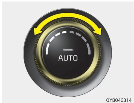
The temperature will increase to the maximum (HI) by turning the knob to the right extremely.
