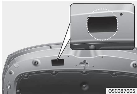
The refrigerant label is located on the underside of the hood.
