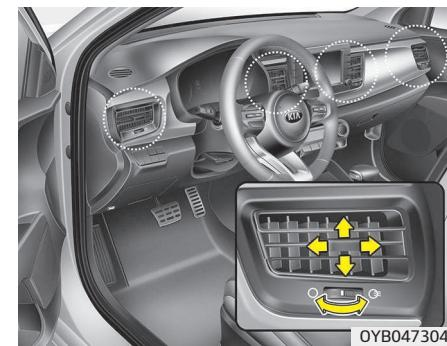
The outlet vents can be opened or closed separately using the thumb-wheel. To close the vent, rotate it downward to the maximum position. Also, you can adjust the direction of air delivery from these vents using the vent control lever as shown.
