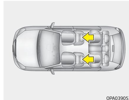
The driver's and front passenger's seats are equipped with a headrest for the occupant's safety and comfort. The headrest not only provides comfort for the driver and front passenger, but also helps to protect the head and neck in the event of a collision.
