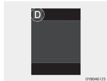
This indicator displays which automatic transaxle shift lever is selected.
