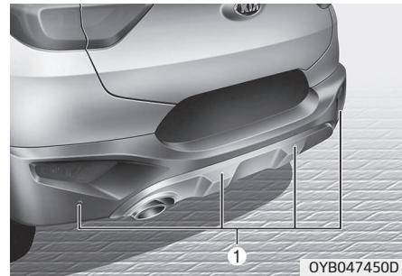
The rear parking assist system assists the driver during backward movement of the vehicle by chiming if any object is sensed within a distance of 120 cm (47 in.) behind the vehicle.
