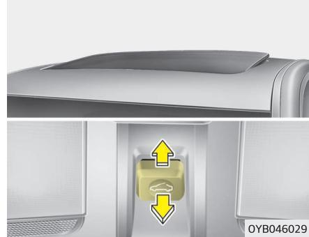
To open the sunroof, push the sunroof control lever upward until the sunroof moves to the desired position. To close the sunroof, push the sunroof lever forward until the sunroof moves to the desired position.
