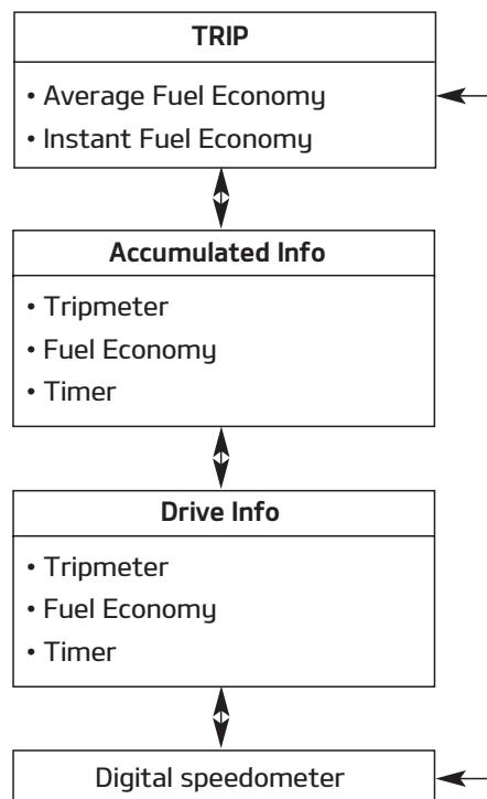
To change the trip mode, scroll the MOVE scroll switch (^/v) in the trip computer mode.
