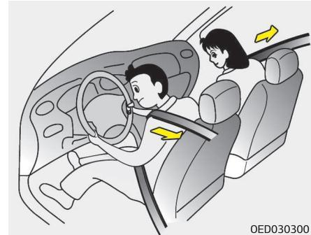
Your vehicle is equipped with pre-tensioner seatbelts at the front and rear outboard seating positions. The purpose of the pre-tensioner is to make sure that the seat belts fit tightly against the occupant's body in certain collisions. The pre-tensioner seat belts may be activated in crashes where the collision is severe enough.
