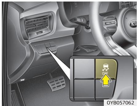
The Electronic Stability Control (ESC) system is designed to stabilize the vehicle during cornering maneuvers. ESC checks where you are steering and where the vehicle is actually going. ESC applies the brakes at individual wheels and intervenes in the engine management system to stabilize the vehicle.
