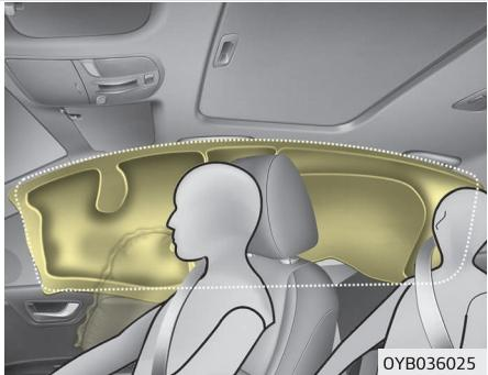
Curtain air bags are located along both sides of the roof rails above the center pillar.
