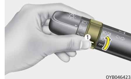
Fog lights are used to provide improved visibility when visibility is poor due to fog, rain or snow, etc. The fog lights will turn on when the fog light switch (1) is turned on after the parklight is turned on.
