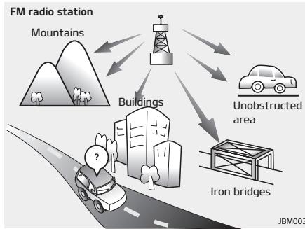
FM broadcasts are transmitted at high frequencies and do not bend to follow the earth's surface. Because of this, FM broadcasts generally begin to fade at short distances from the station. Also, FM signals are easily affected by buildings, mountains, or other obstructions. These can result in certain listening conditions which might lead you to believe a problem exists with your radio. The following conditions are normal and do not indicate radio trouble:
