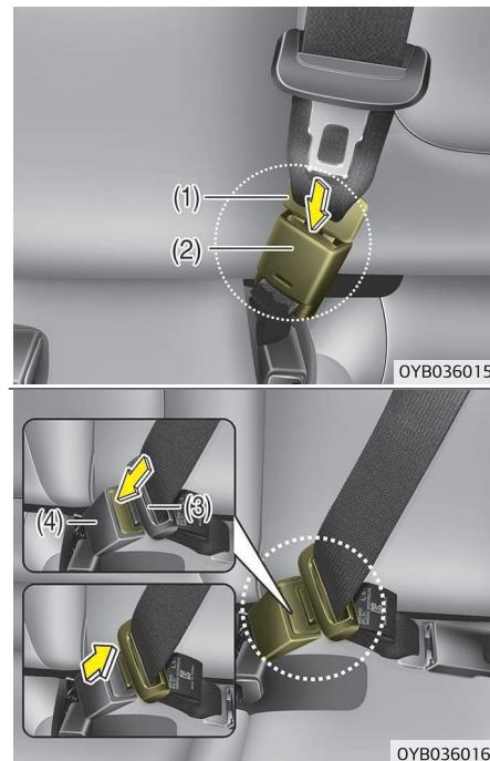
Pull the metal tab (3) and insert it (3) into the buckle (4). There will be an audible "click" when the tab locks into the buckle. Make sure the belt is not twisted. When using the rear center seat belt the buckle with the "CENTER" mark must be used.
