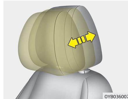
The headrest may be adjusted forward to 4 different positions by pulling the headrest forward to the desired detent. To adjust the headrest to its furthest backwards position, pull it fully forward to the farthest position and release it. Adjust the headrest so that it properly supports the head and neck.
