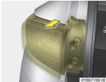
3. Remove the rear combination lamp assembly from the body of the vehicle.
