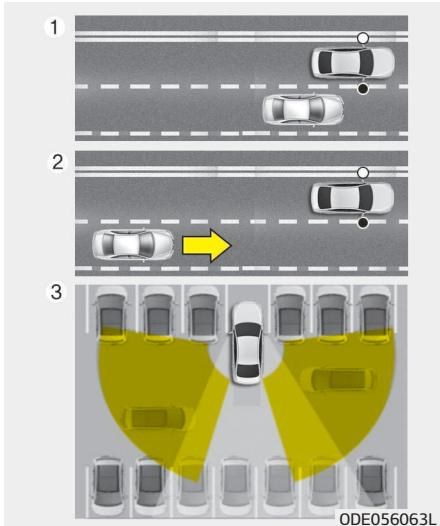
The Blind-Spot Collision Warning (BCW) system uses a radar sensor to alert the driver while driving. It senses the rear side territory of the vehicle and provides information to the driver.
