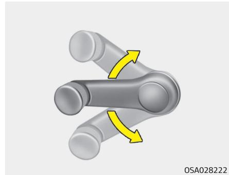
To raise or lower the window, turn the window regulator handle clockwise or counterclockwise.
