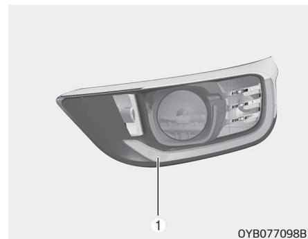
If the position lamp + DRL (LED) (1) does not operate, have your vehicle checked by a professional workshop. Kia recommends to visit an authorized Kia dealer/service partner. The LED lamps cannot be replaced as a single unit because it is an integrated unit. The LED lamps has to be replaced with the unit. A skilled technician should check or repair the position lamp + DRL (LED), for it may damage related parts of the vehicle.
