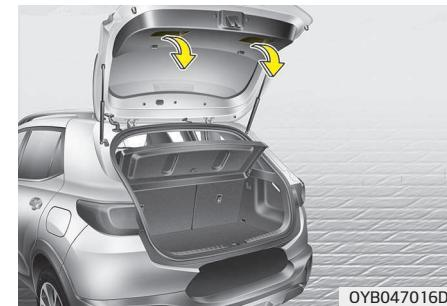
To close the tailgate, lower and push down the tailgate firmly. Make sure that the tailgate is securely latched.
