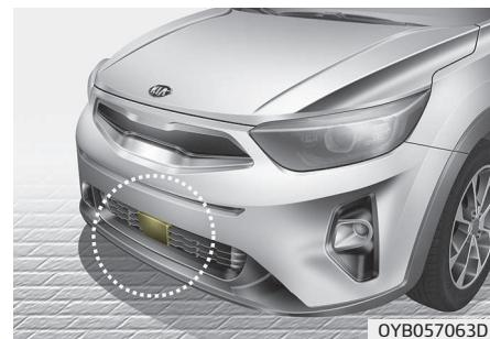
The sensor is to maintain a certain distance from the vehicle in front. However, the smudged sensor lens with foreign substances, such as snow and rain, adversely affects the sensing performance. It may even temporarily cancel the FCA. Always keep the sensor lens clean.
