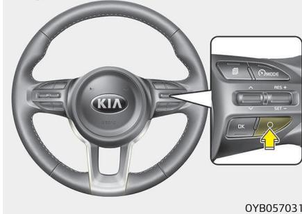
*Each of these actions will cancel cruise control operation (the cruise set indicator light will go off), but it will not turn the system off. If you wish to resume cruise control operation, move up the lever (to RES+) located on your steering wheel. You will return to your previously preset speed.*
