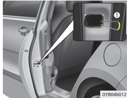
If the power door lock switch does not operate electrically, the only way to lock the door(s) is with the mechanical key from the outside key hole. Doors without the outside key hole, you can lock the door as follows:
