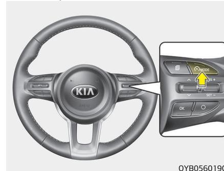
1. Press the speed limit
