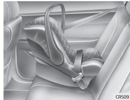
A rearward-facing Child Restraint System provides restraint with the seating surface against the back of the child. The harness system holds the child in place, and in an accident, acts to keep the child positioned in the Child Restraint Systems and reduce the stress to the fragile neck and spinal cord.
