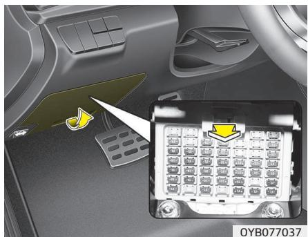
Your vehicle is equipped with a memory fuse to prevent battery discharge if your vehicle is parked without being operated for prolonged periods. Use the following procedures before parking the vehicle for prolonged periods.
