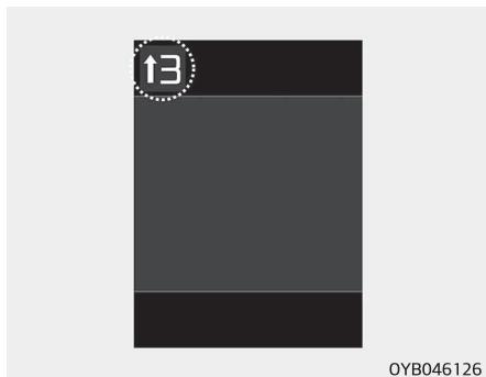
In the Sports Mode, this indicator informs which gear is desired while driving to save fuel.
