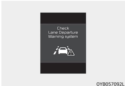
When the Lane Departure Warning (LDW) System is not working properly, the warning light will illuminate and the warning message will come on for a few second. After the message disappears, the master warning light will illuminate.
