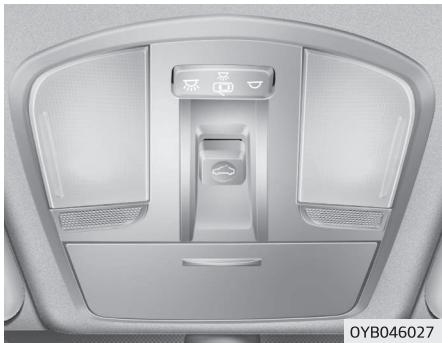
If your vehicle is equipped with a sunroof, you can slide or tilt your sunroof with the sunroof control lever located on the overhead console. The sunroof can only be opened, closed, or tilted when the ignition switch is in the ON position.
