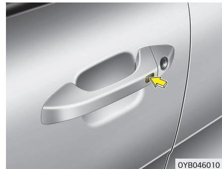
Carrying the smart key, you may lock and unlock the vehicle doors (and tailgate). Also, you may start the engine. Refer to the following, for more details.
