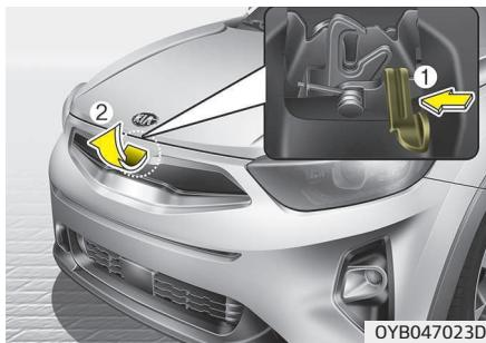
2. Go to the front of the vehicle, raise the hood slightly, push the secondary latch (1) inside of the hood center and lift the hood (2).
