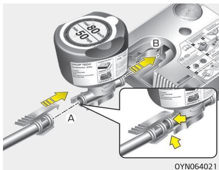
4. Connect the filling hose (3) onto the connector of the sealant bottle (A).
