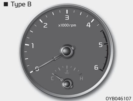
The tachometer indicates the approximate number of engine revolutions per minute (rpm).
