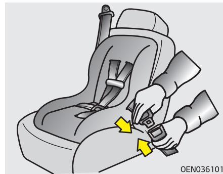
2. Fasten the lap/shoulder belt latch into the buckle. Listen for the distinct "click" sound. Position the release button so that it is easy to access in case of an emergency.
