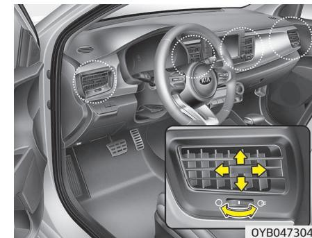
The outlet port can be opened or closed separately using the horizontal thumb-wheel. To close the vent, rotate it downward to the maximum position. To open the vent, rotate it upward to the desired position.
