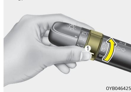
To turn the rear fog lights on, turn the rear fog light switch (1) to the on position when the headlight is turned on.
