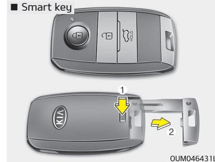
To remove the mechanical key, press and hold the release button and remove the mechanical key.
