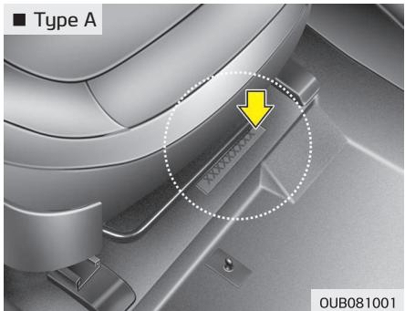
The vehicle identification number (VIN) is the number used in registering your car and in all legal matters pertaining to its ownership, etc. The number is punched on the floor under the passenger seat. To check the number, remove the cover (1).
