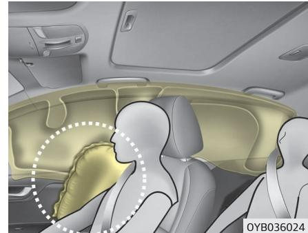
Your vehicle is equipped with a side impact air bag in each front seat. The purpose of the air bag is to provide the vehicle's driver and the front passenger with additional protection than that offered by the seat belt alone.
