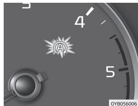
The engine will stop and the green AUTO STOP indicator ((A)) on the instrument cluster will illuminate. If your vehicle is equipped with a supervision cluster, the notice will illuminate on the LCD display.
