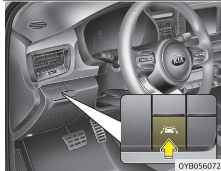
This system detects the lane with the sensor at the front windshield and warns you when your vehicle leaves the lane.
