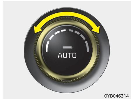
2. Set the temperature control knob to set the desired temperature.
