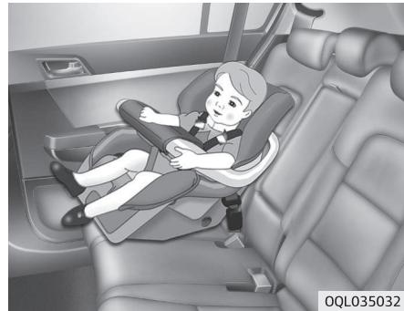
A forward-facing Child Restraint System provides restraint for the child's body with a harness. Keep children in a forward-facing Child Restraint System with a harness until they reach the top height or weight limit allowed by your Child Restraint System's manufacturer. Once your child outgrows the forward-facing Child Restraint System, your child is ready for a booster seat.
