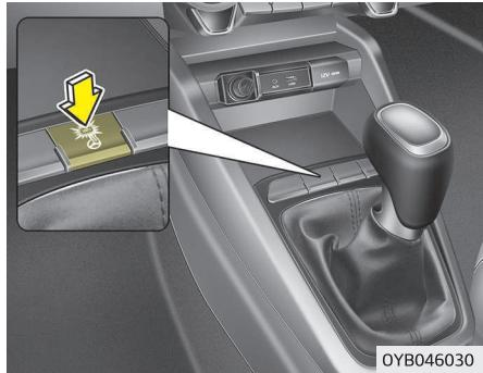
When the ignition switch is in the ON position, pressing the heated steering wheel button warms the steering wheel. The indicator on the button will illuminate.
