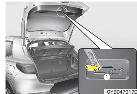
Your vehicle is equipped with the emergency tailgate safety release lever located on the bottom of the tailgate. When someone is inadvertently locked in the luggage compartment.
