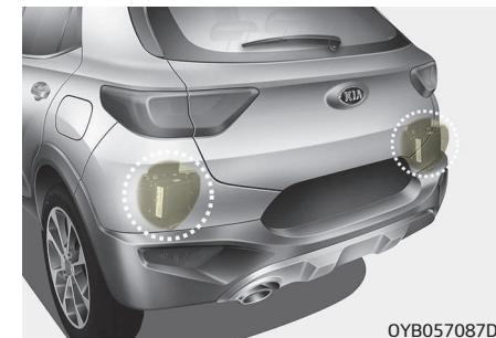
The sensors are located inside the rear bumper.
