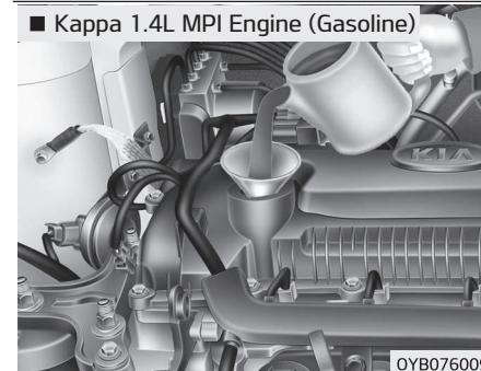
If it is near or at L (Low), add enough oil to bring the level to F (Full). **Do not overfill.**
