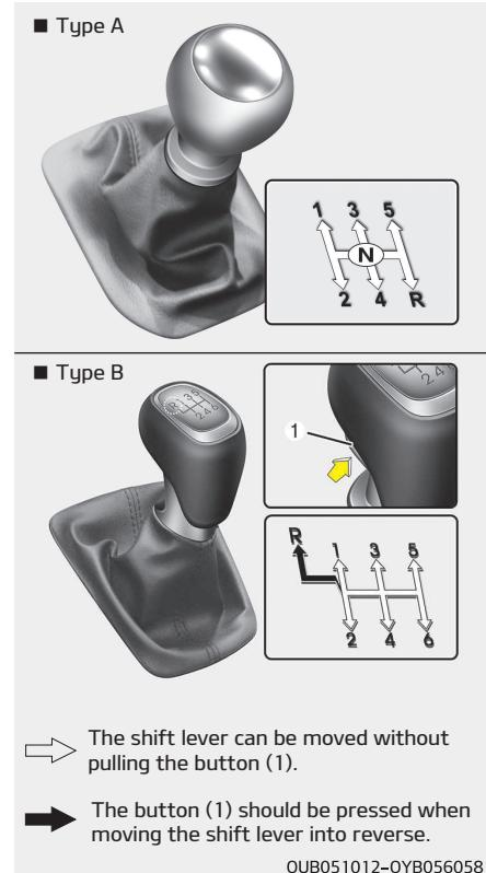
This shift pattern is imprinted on the shift knob. The transaxle is fully synchronized in all forward gears so shifting to either a higher or a lower gear is easily accomplished.
