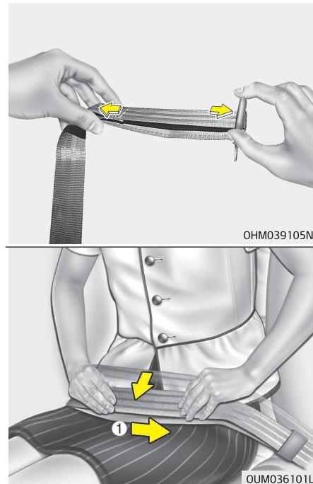
With a 2-point static type seat belt, the length must be adjusted manually so it fits snugly around your body. Fasten the belt and pull on the loose end to tighten.
