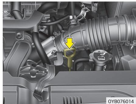
The automatic transaxle fluid level should be checked regularly. Keep the vehicle on level ground with the parking brake applied and check the fluid level according to the following procedure.
