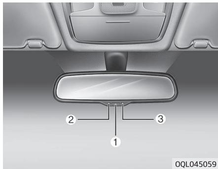
The electric rearview mirror automatically controls the glare from the headlights of the vehicles behind you in nighttime or low light driving conditions. The sensor (3) mounted in the mirror senses the light level around the vehicle, and automatically controls the headlight glare from the vehicles behind you.
