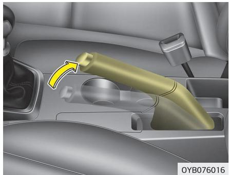
Check the stroke of the parking brake by counting the number of "clicks" heard while fully applying it from the released position. Also, the parking brake alone should securely hold the vehicle on a fairly steep grade. If the stroke is more or less than specified, have the system serviced by a professional workshop. Kia recommends to visit an authorized Kia dealer/service partner.
