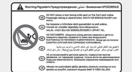
Never place a rear-facing child restraint in the front passenger's seat. If the air bag deploys, it would impact the rear-facing child restraint, causing serious or fatal injury.
