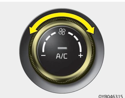
The fan speed can be set to the desired speed by operating the fan speed control knob.
