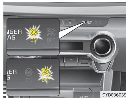
To deactivate the passenger's front air bag, insert the master key into the passenger's front air bag ON/OFF switch and turn it to the OFF position. The passenger's front air bag OFF indicator (※) will illuminate and stay on until the passenger's front air bag is reactivated.
