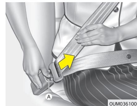
The seat belt is released by pressing the release button (A) on the locking buckle. When it is released, the belt should automatically draw back into the retractor.
