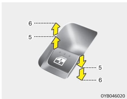
Pressing or pulling up the power window switch momentarily to the second detent position (6) completely lowers or lifts the window even when the switch is released. To stop the window at the desired position while the window is in operation, pull up or press and release the switch to the opposite direction of the movement.
