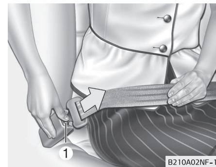
When you want to release the seat belt, press the button (1) in the locking buckle.
