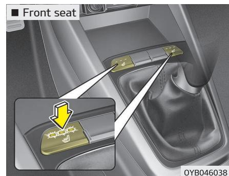
The seat warmer is provided to warm the front seats during cold weather. With the ignition switch in the ON position, push either of the switches to warm the driver's seat or the front passenger's seat. During mild weather or under conditions where the operation of the seat warmer is not needed, keep the switches in the "OFF" position.
