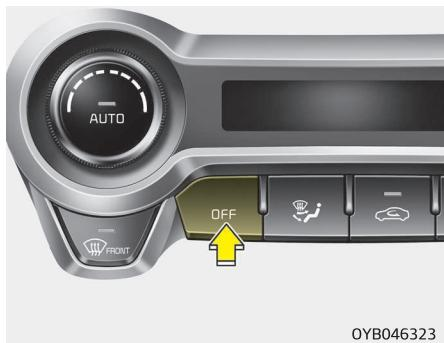
Press the OFF button to turn off the air climate control system. However, you can still operate the air intake buttons as long as the ignition switch is in the ON position.
