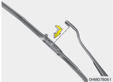
2. Lift up the wiper blade clip. Then pull down the blade assembly and remove it.
