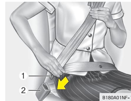
To fasten your seat belt, pull it out of the retractor and insert the metal tab (1) into the buckle (2). There will be an audible "click" when the tab locks into the buckle.
