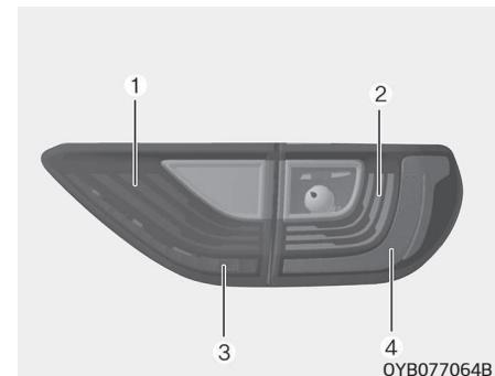
If the stop and tail lamp (LED) (1,2,3,4) does not operate, have your vehicle checked by a professional workshop. Kia recommends to visit an authorized Kia dealer/service partner. The LED lamps cannot be replaced as a single unit because it is an integrated unit. The LED lamps has to be replaced with the unit. A skilled technician should check or repair the stop and tail lamp (LED), for it may damage related parts of the vehicle.
