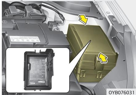
■ Engine compartment fuse panel
