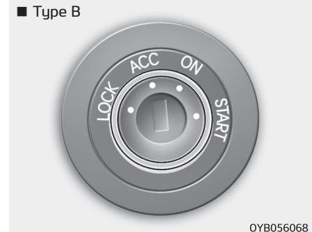
The steering wheel locks to protect against theft. The ignition key can be removed only in the LOCK position.
