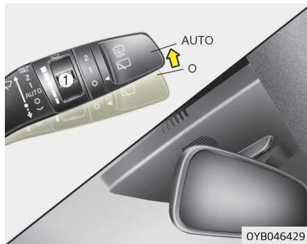
The rain sensor located on the upper end of the windshield glass senses the amount of rainfall and controls the wiping cycle for the proper interval. The more it rains, the faster the wiper operates. When the rain stops, the wiper stops.
