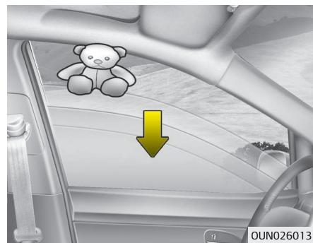
If the upward movement of the window is blocked by an object or part of the body, the window will detect the resistance and will stop upward movement. The window will then lower approximately 30 cm (11.8 in.) to allow the object to be cleared.
