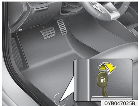
The fuel-filler lid must be opened from inside the vehicle by pulling up on the fuel-filler lid opener located on the front floor area on the driver's seat.
