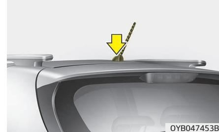
To remove the antenna, turn it counterclockwise. To install the antenna, turn it clockwise.
