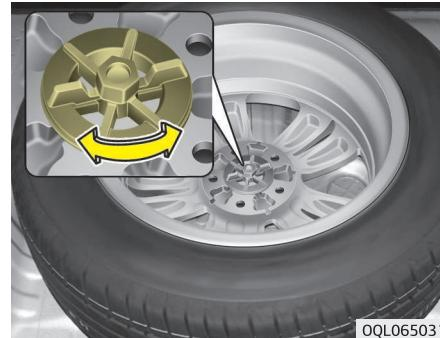
Turn the tire hold-down wing bolt counterclockwise.
