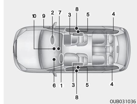
The SRS consists of the following components:
