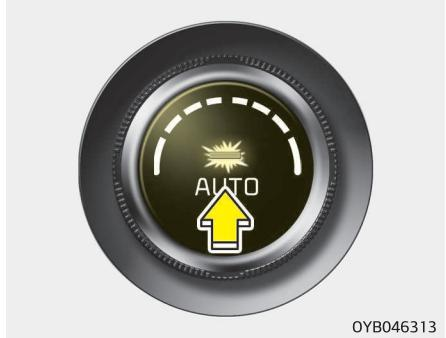
1. Push the AUTO button. The modes, fan speeds, air intake and air-conditioning will be controlled automatically according to the temperature setting.
