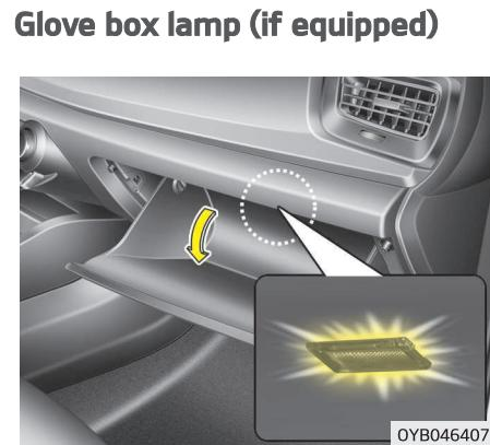
The glove box lamp comes on when the glove box is opened.
