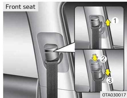
You can adjust the height of the shoulder belt anchor to one of the 3 positions for maximum comfort and safety. The height of the adjusting seat belt should not be too close to your neck. The shoulder portion should be adjusted so that it lies across your chest and midway over your shoulder near the door and not your neck.
