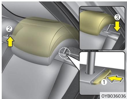
To remove the headrest, raise it as far as it can go then press the release button (1) while pulling upward (2).
