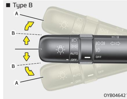
The ignition switch must be on for the turn signals to function. To turn on the turn signals, move the lever up or down (A).
