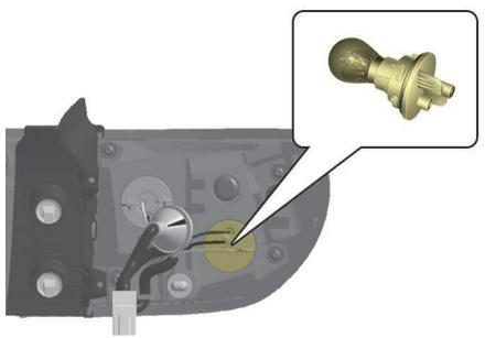
5. Remove the socket from the assembly by turning the socket counterclockwise until the tabs on the socket align with the slots on the assembly.
