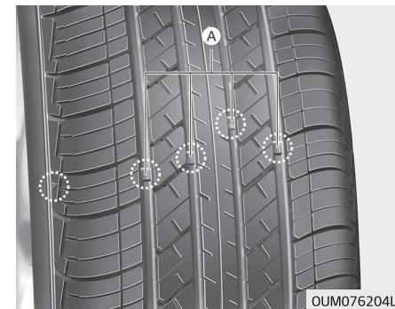
If the tire is worn evenly, a tread wear Indicator (A) will appear as a solid band across the tread. This shows there is less than 1.6 mm (1/16 in.) of tread left on the tire. Replace the tire when this happens.
