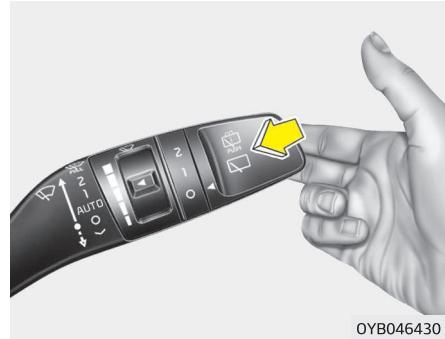
In the 0 (Off) position, pull the lever gently toward you to spray washer fluid on the windshield and to run the wipers 1-3 cycles.
