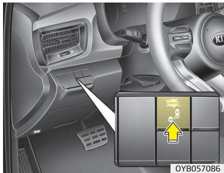
The indicator on the switch will illuminate when the Blind-Spot Collision Warning (BCW) system switch is pressed with the ignition switch ON. If the vehicle speed exceeds 30 km/h (18.6 mph), the system will activate. If you press the switch again, the switch indicator and system will be turned off. If the ignition switch is turned OFF and ON the system returns to the previous state.
