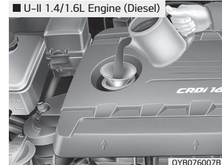
If it is near or at L (Low), add enough oil to bring the level to F (Full). **Do not overfill.**
