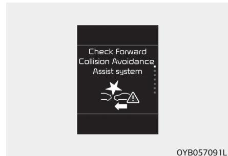
When the FCA is not working properly, the FCA warning light (✽) will illuminate and the warning message will appear for a few seconds. After the message disappears, the master warning light (Δ) will illuminate. In this case, have the vehicle inspected by a professional workshop. Kia recommends to visit an authorized Kia dealer/service partner.
