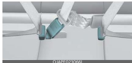
The rear seat belt buckles can be stowed in the pocket between the rear seatback and cushion when not in use.
