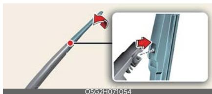
2. Install the new blade assembly by inserting the centre part into the slot in the wiper arm until it clicks into place.
