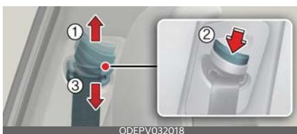
Release the button to lock the anchor into position. Try sliding the height adjuster to make sure that it has locked into position.
