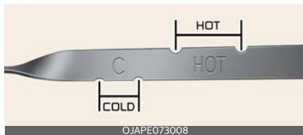
4. If the fluid level is checked in cold condition [fluid temperature 20~30°C (68~86°F)], add the fluid to the "COLD" line and then recheck the fluid level according to the above step 2.
