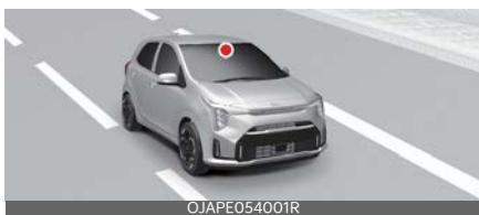
The front view camera is used as a detecting sensor to detect lane markings (or road edges).
