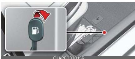
The fuel filler door must be opened from inside the vehicle by pulling up on the fuel-filler lid opener located on the front floor area on the driver's seat.
