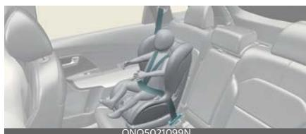
A forward-facing Child Restraint System provides restraint for the child's body with a harness. Keep children in a forward-facing Child Restraint System with a harness until they reach the top height or weight limit allowed by your Child Restraint System's manufacturer.
