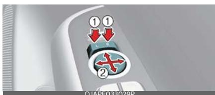
The electric remote control mirror switch allows you to adjust the position of the left and right outside rearview mirrors. To adjust the position of either mirror, the ignition switch should be in the ACC position.
