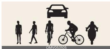
The illustration above shows the image the front view camera and front radar are capable of detecting as a vehicle, powered two-wheeler, pedestrian and cyclist.
