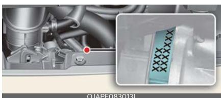
The engine number is stamped on the engine block as shown in the drawing.
