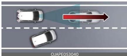
If the vehicle in front abruptly departs, Leading Vehicle Departure Alert may not operate properly.
