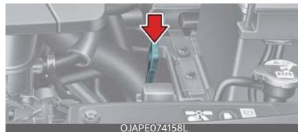
The automatic transmission fluid level should be checked regularly.
