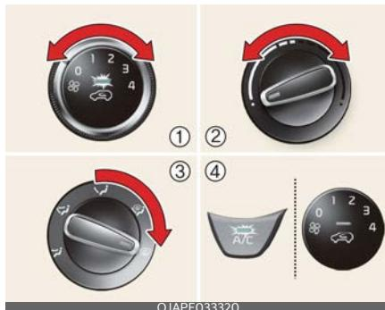
If the air conditioning and outside (fresh) air position are not selected automatically, press the corresponding button manually.
