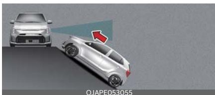
Rear Cross-Traffic Collision-Avoidance Assist may be limited when the vehicle is on an uphill or downhill slope, or near it, and may not detect the vehicle approaching from the left or right. If this occurs, the function may not warn the driver or control the brakes when necessary.
