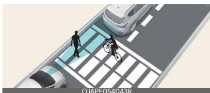
If there is a pedestrian(s) or bicycle(s) in between you and the vehicle in front, Leading Vehicle Departure Alert may not operate properly.
