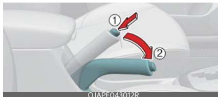
To release the parking brake, first apply the foot brake and pull up the parking brake lever slightly. Secondly depress the release button (1) and lower the parking brake lever (2) whilst holding the button.
