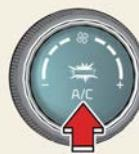
Press the A/C button to turn the air conditioning system on (indicator light will illuminate).
