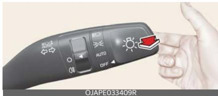
To flash the headlights, pull the lever towards you. It will return to the normal (low beam) position when released. The headlight switch does not need to be on to use this flashing feature.
