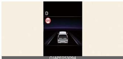
If you exceed the displayed speed limit, the sign will blink and an audible warning will be triggered.
