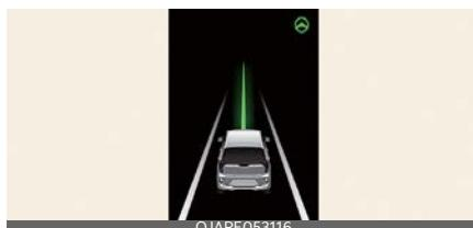
If the vehicle ahead and/or both lane markings are detected and Your driving speed is below 150 km/h (95 mph), the green (Ⓐ) indicator light appears on the cluster, and Lane Following Assist helps centre the vehicle in the lane by assisting the steering wheel.
