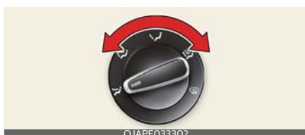
The mode selection knob controls the direction of the air flow through the ventilation system.
