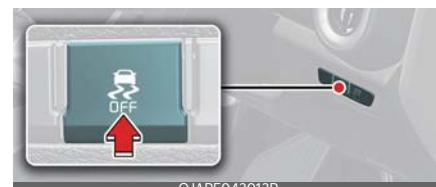
The Electronic Stability Control (ESC) system is designed to stabilize the vehicle during cornering manoeuvres. ESC checks where you are steering and where the vehicle is actually going. ESC applies the brakes at individual wheels and intervenes in the engine management system to stabilize the vehicle.
