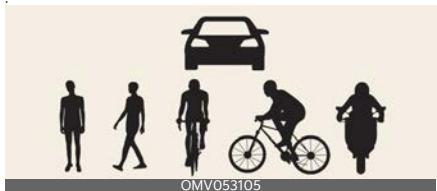
The illustration above shows the image the front view camera and front radar are capable of detecting as a vehicle, powered two-wheeler, pedestrian and cyclist.
