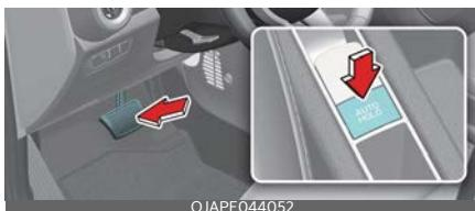
Before the Auto Hold will engage, the driver's door, tailgate and engine bonnet must be closed.
