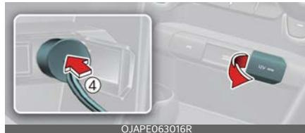
9. With the ENGINE START/STOP button position on or ignition switch position on, switch on the compressor and let it run for approximately 5~7 minutes to fill the sealant up to proper pressure. The inflation pressure of the tyre after
