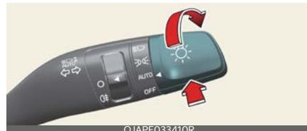
High Beam Assist is a function that automatically adjusts the headlamp range (switches between high beam and low beam) depending on the brightness of detected vehicles and certain road conditions.
