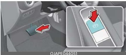
Releasing the parking brake with EPB switch,
