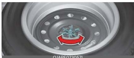
If it is hard to loosen the tyre holdown wing bolt by hand, you can loosen it easily using the jack handle.
