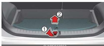
3. Pull the luggage board hinge(3) to the end of sliding slot and it will fall down lower to increase cargo space.
