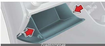
2. Remove the climate control air filter cover whilst pressing the lock on the right side of the cover.
