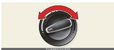
The temperature control knob allows you to control the temperature of the air flowing from the ventilation system. To change the air temperature in the passenger compartment, turn the knob to the right position for warm and hot air or left position for cooler air.
