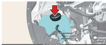
The coolant level should be filled between MAX and MIN (F and L) marks on the side of the coolant reservoir when the engine is cool. If the coolant level is low, add enough distilled (deionized) or soft water. Bring the level to MAX (F), but do not overfill.
