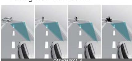
Forward Collision-Avoidance Assist may not detect other vehicle, powered two-wheeler, pedestrians or cyclists in front of you when driving on curved roads adversely affecting the performance of the sensors. This may result in no warning, braking assist when necessary.
