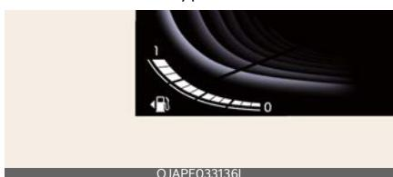
This gauge indicates the approximate amount of fuel remaining in the fuel tank.
