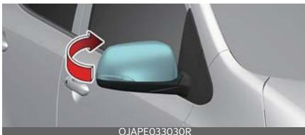
To fold outside rearview mirror, grasp the housing of mirror and then fold it toward the rear of the vehicle.
