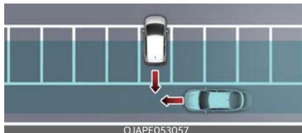
Rear Cross-Traffic Collision-Avoidance Assist may detect vehicles passing by behind you when parking in reverse into a parking space. If this occurs, the function may unnecessarily warn the driver and control the brake.
