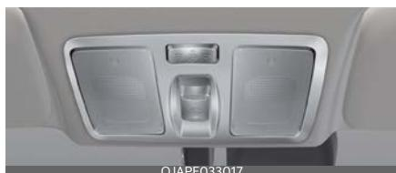
If your vehicle is equipped with a sunroof, you can slide or tilt your sunroof with the sunroof switch located on the overhead console.
