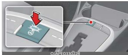
When the ignition switch is in the ON position, pressing the steering wheel heater button warms the steering wheel. The indicator on the button will illuminate.
