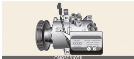
A compressor label informs you the type of compressor your vehicle is equipped with such as model, supplier part number, production number, refrigerant (1) and refrigerant oil (2).
