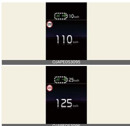
During the operation of Manual Speed Limit Assist, if the speed limit of the road changes, an arrow pointing up or down is displayed to indicate the need to change the set speed. Raise or lower the (+) or (-) switch in the arrow direction to adjust the set speed according to the speed limit.
