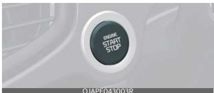
Whenever the front door is opened, the ENGINE START/STOP button will illuminate for your convenience. The light will go off after about 30 seconds when the door is closed. It will also go off immediately when the theft-alarm system is armed.
