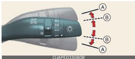
The ignition switch must be on for the turn signals to function. To turn on the turn signals, move the lever up or down (A).
