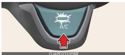
Press the A/C button to turn the air conditioning system on (indicator light will illuminate). Press the button again to turn the air conditioning system off.
