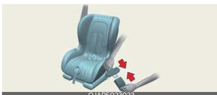
3. Remove as much slack from the belt as possible by pushing down on the Child Restraint System whilst feeding the shoulder belt back into the retractor.
