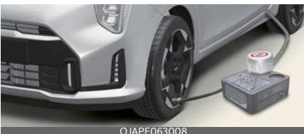
The system of compressor and sealing compound effectively and comfortably seals most punctures in a passenger car tyre caused by nails or similar objects and reinflates the tyre.
