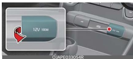
The power outlet is designed to provide power for mobile telephones or other devices designed to operate with vehicle electrical systems. The devices should draw less than 10 amps with the engine running.
