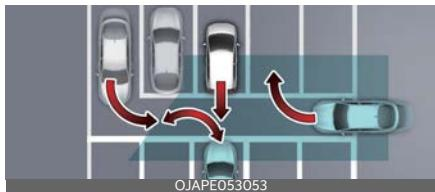
Rear Cross-Traffic Collision-Avoidance Assist may detect vehicles which are parking or pulling out near your vehicle (example, a vehicle leaving beside your vehicle, a vehicle parking or pulling out in the rear area, a vehicle approaching your vehicle making a turn, etc.).
