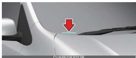
The VIN is also on a plate attached to the top of the dashboard. The number on the plate can easily be seen through the windscreen from outside.
