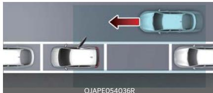
Whilst your vehicle is stopped, and if Safe Exit Warning detects a vehicle approaching the rear corner of your vehicle and a passenger opens a door, Safe Exit Warning may warn you with a warning message and a warning sound to help avoid a collision.
