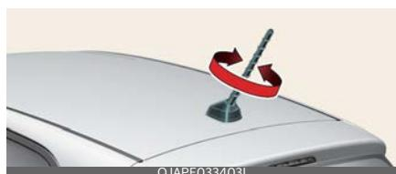
The micro-pole antenna receives an AM/FM signal. This antenna is a removable type.
