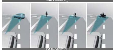
Forward Collision-Avoidance Assist may not detect other vehicles, powered two-wheelers, pedestrians or cyclists in front of you when driving on curved roads adversely affecting the performance of the sensors. This may result in no warning, or braking assist when necessary.
