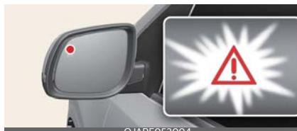
The warning light on the cluster, the outside rear view mirror will appear when the vehicle on both lanes is detected from the rear.
