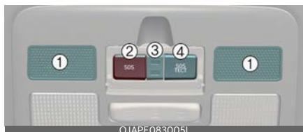
Elements of the system ERA-GLONASS, installed in passenger compartment:
