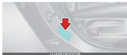
The vehicle certification label attached on the driver's (or front passenger's) side centre pillar gives the vehicle identification number (VIN).
