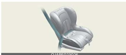
2. Fasten the lap/shoulder belt latch into the buckle. Listen for the distinct "click" sound. Position the release button so that it is easy to access in case of an emergency.
