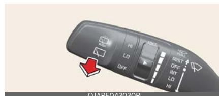
In the O (Off) position, pull the lever gently toward you to spray washer fluid on the windscreen and to run the wipers 1-3 cycles.
