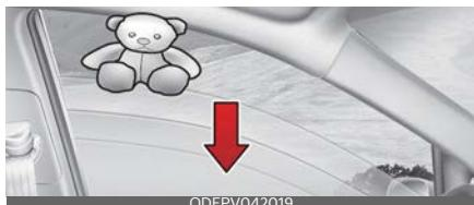
If the upward movement of the window is blocked by an object or part of the body, the window will detect the resistance and will stop upward movement. The window will then lower approximately 30 cm (11.8 in) to allow the object to be cleared.
