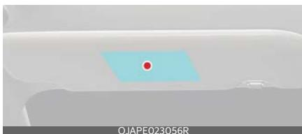
Air bag warning labels are attached to alert the driver and passengers of potential risk of air bag system.
