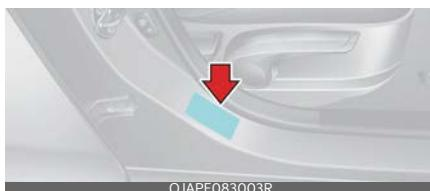
The Certification/Tyre label is found on the front edge of the RH (or LH) "B" pillar. The label shows the size of your original tyres and inflation pressures needed to obtain the gross weight capacity of your vehicle.
