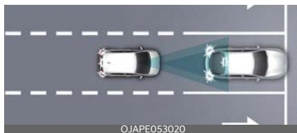
Forward Collision-Avoidance Assist detects a vehicle, a powered two-wheeler, a pedestrian, or a cyclist ahead on the road and may warn you of a possible collision with a warning message on the instrument cluster and a warning sound. Also, Forward Collision-Avoidance Assist may assist with braking your vehicle to help reduce collision speed or avoid a collision.
