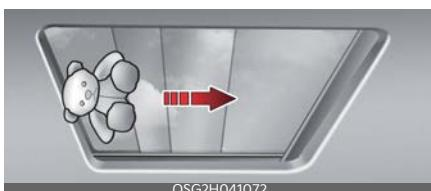
If the sunroof glass senses any obstacle whilst it is closing automatically, it will reverse direction then stop at a certain position.
