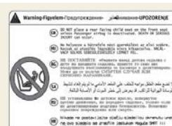
Never place a rear-facing child restraint in the front passenger's seat. If the air bag deploys, it would impact the rear-facing child restraint, causing serious or fatal injury.
