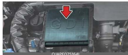
1. Loosen the air cleaner cover attaching clips.
