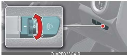
To adjust the headlight beam level according to the number of the passengers and loading weight in the luggage area, turn the beam levelling switch.
