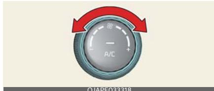
The fan speed can be set to the desired speed by operating the fan speed control knob.
