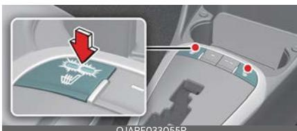
The seat warmer is provided to warm the front seats during cold weather. With the ignition switch in the ON position, push either of the switches to warm the driver's seat or the front passenger's seat.
