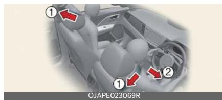
When the vehicle stops suddenly, or if the occupant tries to lean forward too quickly, the seat belt retractor will lock into position. In certain frontal collisions, the pre-tensioner will activate and pull the seat belt into tighter contact against the occupant's body.
