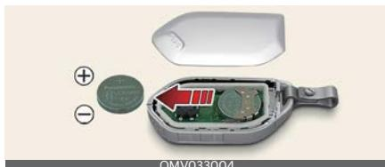
The transmitter uses a 3 volt lithium battery which will normally last for several years. When replacement is necessary, use the following procedure.
