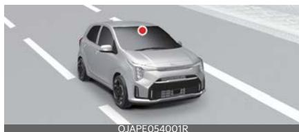
The front view camera is used as a detecting sensor to help detect driving patterns and front vehicle departure whilst vehicle is being driven. Refer to the picture above for the detailed location of the detecting sensor.
