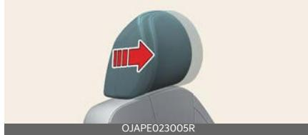
The headrest may be adjusted forward to 4 different positions by pulling the headrest forward to the desired detent. To adjust the headrest to its rearmost position, pull it fully forward to the foremost position and release it. Adjust the headrest so that it properly supports the head and neck.
