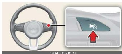
1. Accelerate to the desired speed, which must be more than 30 km/h (20 mph).
