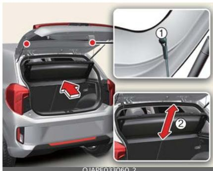
2. Whilst lifting the cover up, hold the area near the front slots. Then, pull up the cover (2) at approximately 50° angle.
