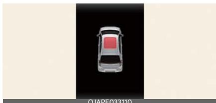
If the driver turns off the engine when the sunroof is not fully closed, the warning chime will sound for several seconds and the sunroof open warning will appear on the cluster LCD display.
