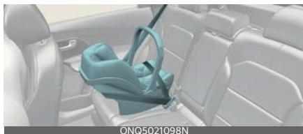
A rearward-facing Child Restraint System provides restraint with the seating surface against the back of the child. The harness system holds the child in place, and in an accident, acts to keep the child positioned in the Child Restraint Systems and reduce the stress to the fragile neck and spinal cord.
