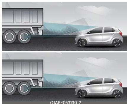
If the vehicle in front of you has cargo that extends rearward from the cab, or when the vehicle in front of you has higher ground clearance, additional special attention is required. Forward Collision-Avoidance Assist may not be able to detect the cargo extending from the vehicle. In these instances, you must maintain a safe braking distance from the rearmost object, and if necessary, steer your vehicle and depress the brake pedal to reduce
