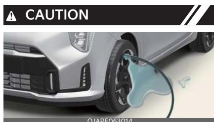
Securely install the sealant filling hose to the valve. If not, sealant may flow backward, possibly clogging the filling hose.
