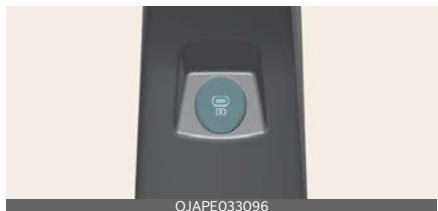
The USB charger allows drivers and passengers to charge their digital devices such as smartphones and tablets.
