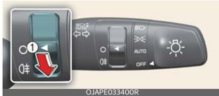
To turn the rear fog lights on, turn the rear fog light switch (1) to the on position when the headlight is turned on.
