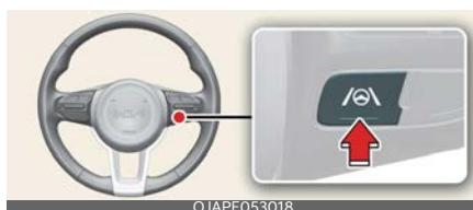
With the vehicle on, shortly press the Lane Driving Assist button located on the steering wheel to turn on Lane Following Assist. The grey or green (Ⓐ) indicator light will appear on the cluster.
