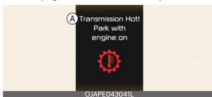
A: Transmission Hot! Park with engine on
