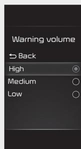
With the ignition switch or ENGINE-START/STOP button in the ON position, select 'Driver Assistance → Warning volume' from the Settings menu to change the Warning volume to 'High', 'Medium', 'Low' for Rear Cross- Traffic Safety system.
