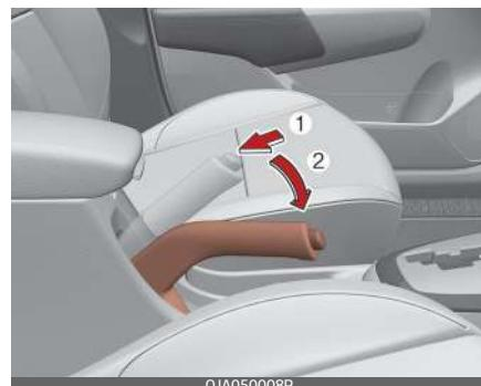
To release the parking brake, first apply the foot brake and pull up the
