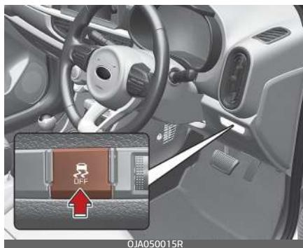
The Electronic Stability Control (ESC) system is designed to stabilize the vehicle during cornering manoeuvres. ESC checks where you are steering and where the vehicle is actually going.
