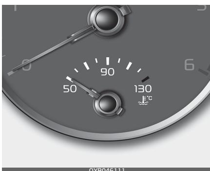
This gauge indicates the temperature of the engine coolant when the ignition switch or ENGINE START/STOP button is ON.
