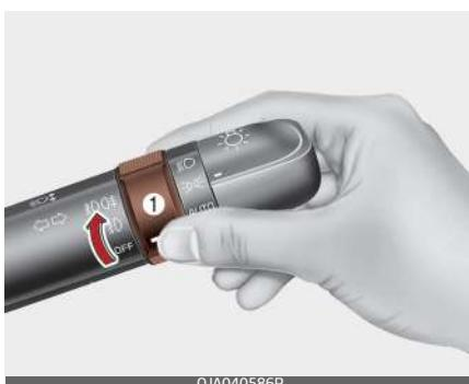
Fog lights are used to provide improved visibility when visibility is poor due to fog, rain or snow, etc. The fog lights will turn on when the fog light switch (1) is turned on after the parklight is turned on.
