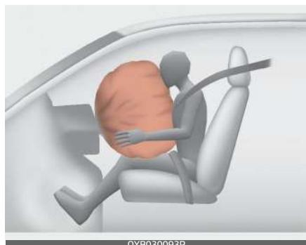
After complete inflation, the air bag immediately starts deflating, enabling the driver to maintain forward visibility and the ability to steer or operate other controls.
