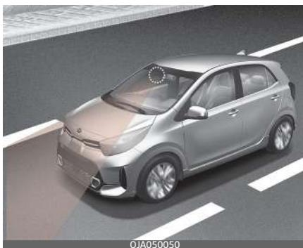
The front view camera is used as a detecting sensor to detect driving patterns whilst vehicle is being driven.
