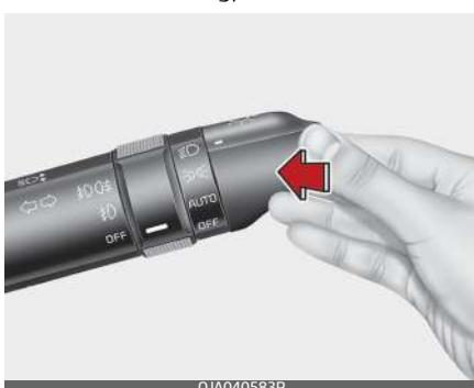
To turn on the high beam headlights, push the lever away from you when the headlight is on. Pull it back for low beams.
