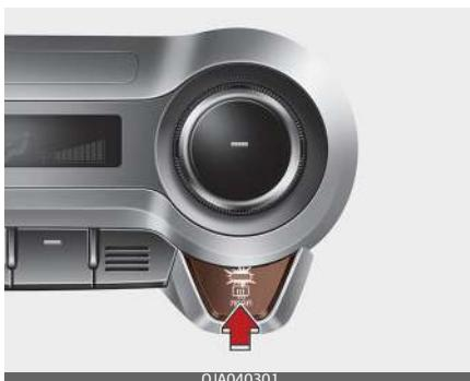
The defroster heats the window to remove frost, fog and thin ice from the rear window, whilst the engine is running.
