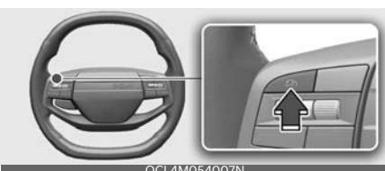
Press the Driving Assist button to turn Smart Cruise Control off.
