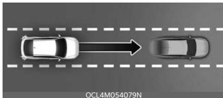
Highway Driving Assist detect lanes and vehicles ahead and help maintain the distance from the vehicle ahead and the set speed and center your vehicle in the lane while driving on the highway.
