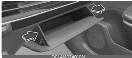
4. Remove the climate control air filter cover by pulling out right side of the cover.
