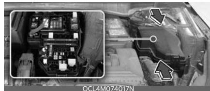
3. Check the removed fuse; replace it if it is blown. To remove or insert the fuse, use the fuse puller in the engine compartment fuse panel.
