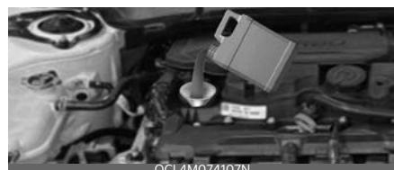
**Use a funnel to help prevent oil from being spilled on engine components.** Use only the specified engine oil. (Refer to "Recommended lubricants and capacities" on page 9-9.)
