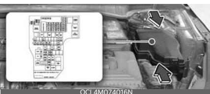
4. Check the removed fuse; replace it if it is blown.
