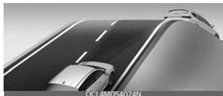
During uphill or downhill driving, the Smart Cruise Control may not detect a moving vehicle in your lane and cause your vehicle to accelerate to the set speed. Vehicle speed will rapidly decrease when a vehicle ahead is detected suddenly.
