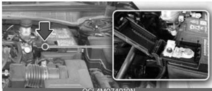
3. Replace the fuse with a new one of the same rating.
