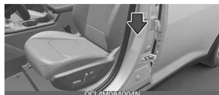
The vehicle certification label attached on the driver's (or front passenger's) side center pillar gives the vehicle identification number (VIN).
