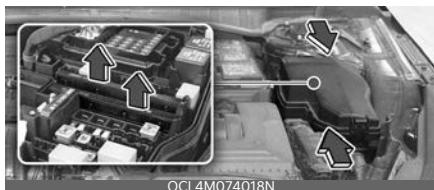
If the multi fuse is blown, it must be removed as follows:
