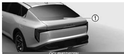
If the high-mounted stop lamp (LED) (1) is not functioning, please have your vehicle inspected by an authorized Kia dealer. The LED lamp cannot be replaced as a single unit because it is an integrated component. Instead, the entire LED lamp unit must be replaced. It's essential to have a skilled technician check or repair the high-mounted stop lamp (LED) to prevent any damage to related vehicle parts.
