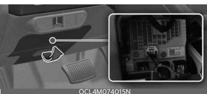
3. Pull the suspected fuse straight out. Use the removal tool provided on the engine fuse panel cover.
