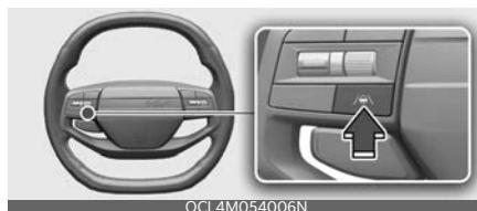
With the vehicle on, shortly press the Lane Driving Assist button located on the steering wheel to turn on Lane Following Assist. The gray or green (Ⓐ) indicator light will appear on the cluster.
