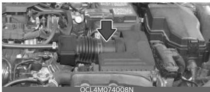
You can clean the filter when inspecting the air cleaner compartment. Clean the filter by using compressed air.
