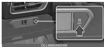
ESC applies the brakes on individual wheels and intervenes with the vehicle management system to stabilize the vehicle.
