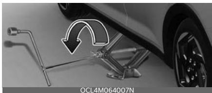
Before removing the wheel lug nuts, make sure the vehicle is stable and that there is no chance for movement or slippage.
