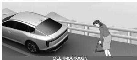
4. Remove the wheel lug nut wrench, jack and spare tire from the vehicle.
