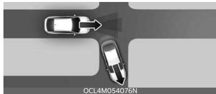
When a vehicle ahead disappears from view at an intersection, your vehicle may accelerate.
