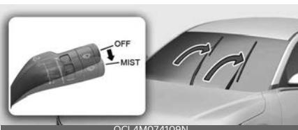
This vehicle has a "hidden" wiper design which means that the wipers cannot be lifted when they are in their bottom resting position.
