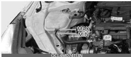
8. If the coolant level is low, add enough specified coolant to provide protection against freezing and corrosion. Bring the level to MAX, but do not overfill.
