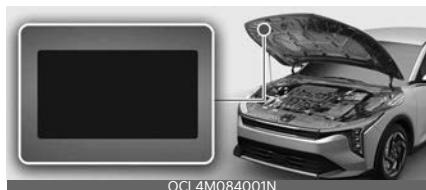
The refrigerant label is located on the underside of the hood.
