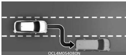
Highway Lane Change Assist function can help change lanes to the direction you operate the turn signal switch if the function determines that lane change is possible.
