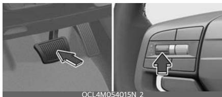
Press the (II) switch or depress the brake pedal to temporarily cancel Smart Cruise Control.
