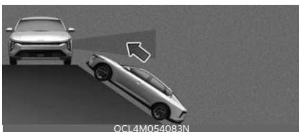
Rear Cross-Traffic Collision-Avoidance Assist may be limited when the vehicle is on an uphill or downhill road, or near it, and may not detect the vehicle approaching from the left or right. If this occurs, the function may not warn the driver or control the brakes when necessary.
