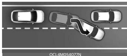
When a vehicle in front of you merges out of the lane, Smart Cruise Control may not immediately detect the new vehicle that is now in front of you.
