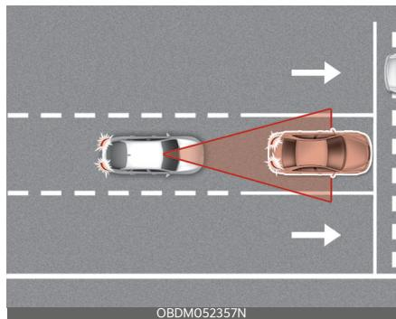
Forward Collision-Avoidance Assist is designed to detect and monitor a vehicle ahead or detect a pedestrian in the roadway through front view camera recognition to warn the driver that a collision is imminent, and if necessary, apply emergency braking.
