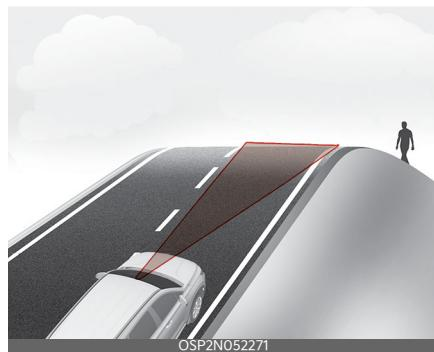
Forward Collision-Avoidance Assist may recognize a vehicle or pedestrian in the next lane or outside the lane when driving on a curved road.
