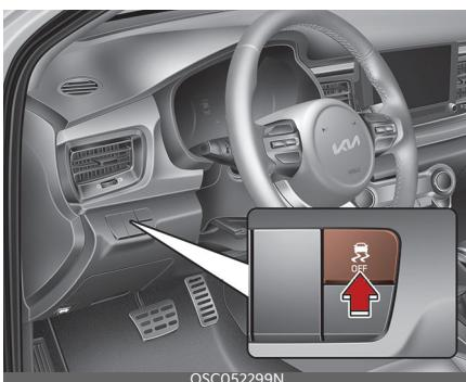
The Electronic Stability Control (ESC) system is designed to stabilize the vehicle during cornering maneuvers. ESC
