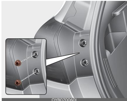
2. Loosen the light assembly retaining screws with a cross-tip screw-driver.
