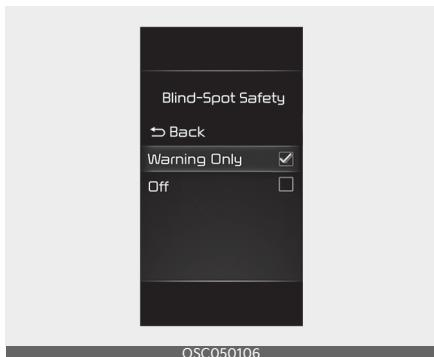
With the ignition switch or ENGINE START/STOP button in the ON position, select or deselect "User Settings → Driver Assistance → Blind-Spot Safety" to set whether to use each function.
