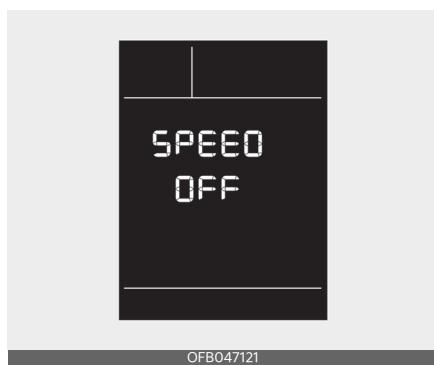
Switch to Speed Mode using the trip switch in Trip mode, and press and hold the RESET button for more than 1 second. Then it will be switched from SPEED ON to SPEED OFF or the other way around.
