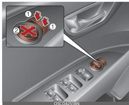
The electric remote control mirror switch allows you to adjust the position of the left and right outside rearview mirrors. To adjust the position of either mirror, the ignition switch or ENGINE START/
