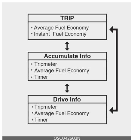
To change the trip mode, scroll the MOVE scroll switch ( $\swarrow/\searrow$ ) in the trip computer mode.
