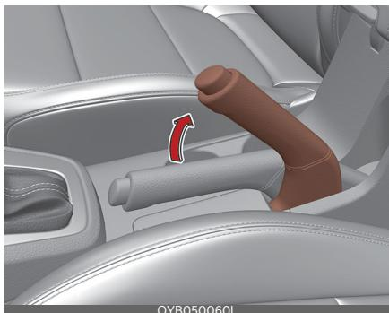
To engage the parking brake, first apply the foot brake and then without pressing the release button in, pull the parking brake lever up as far as possible. In addition it is recommended that when parking the vehicle on a gradient, the shift lever should be positioned in the appropriate low gear for Manual Transmission vehicles or in the P (Park) position for Intelligent Variable Transmission vehicles.
