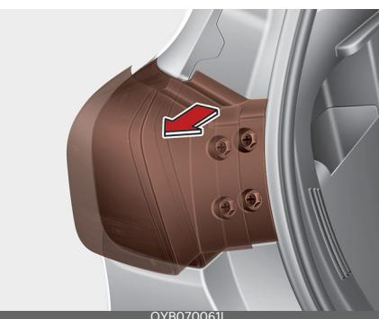
4. Disconnect the rear combination lamp connector.
