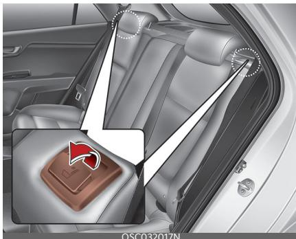
4. Pull the lock release lever and fold the rear seatback forward and down firmly.
