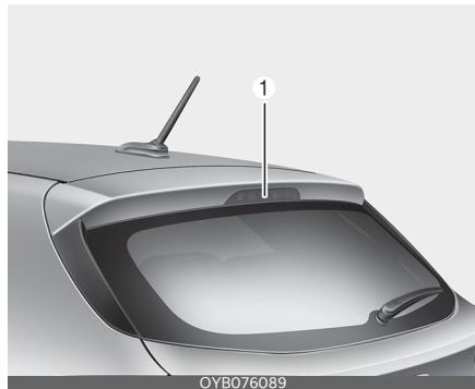
If the high mounted stop lamp (1) does not operate, have the vehicle checked by an authorized Kia dealer.
