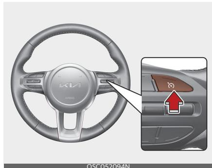
1. Press the Driving Assist (Ⓐ) button on the steering wheel to turn Cruise Control on. The CRUISE indicator will illuminate.
