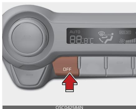
Press the OFF button to turn off the air climate control system. However you can still operate the mode and air intake buttons as long as the ignition switch is in the ON position.
