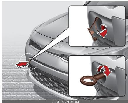
1. Remove the towing hook from the tool case located in the trunk/liftgate.
