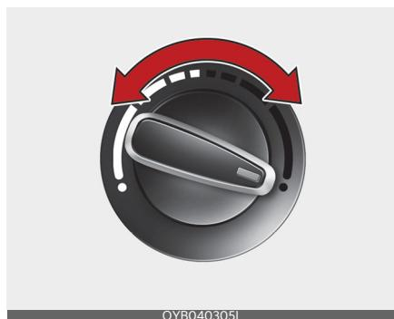
The temperature control knob allows you to control the temperature of the air flowing from the ventilation system. To change the air temperature in the passenger compartment, turn the knob to the right for warmer and hot air, or to the left for cooler air.
