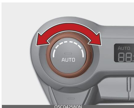
The temperature control knob allows you to control the temperature of the air flowing from the ventilation system. To change the air temperature in the passenger compartment, turn the knob to the right for warm air or left for cooler air.
