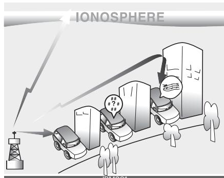
AM and FM radio signals are broadcast from transmitter towers located around your city. They are intercepted by the
