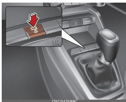
With the ignition switch or ENGINE START/STOP button in the ON position, pressing the heated steering wheel button warms the steering wheel. The indicator on the button will illuminate.
