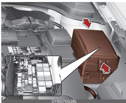
2. Remove the fuse panel cover by pressing the tab and pulling the cover up. When the blade type fuse is disconnected, remove it by using the clip designed for changing fuses located in the engine compartment fuse box. Upon removal, securely insert reserve fuse of the same rating.
