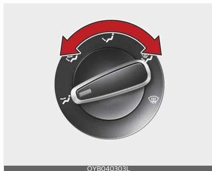
The mode selection knob controls the direction of the air flow through the ventilation system. Five symbols are used to represent Face, Bi-Level, Floor, Floor-Defrost and Defrost air position.
