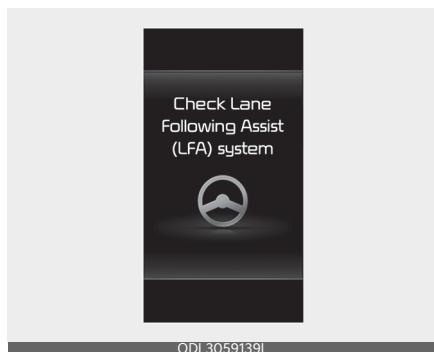
When Lane Following Assist is not working properly, the 'Check Lane Following Assist (LFA) system' warning message will appear on the cluster.
