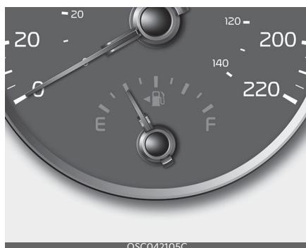
The fuel gauge indicates the approximate amount of fuel remaining in the fuel tank.
