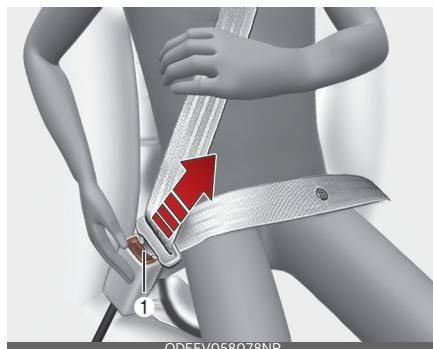
The seat belt is released by pressing the release button (1) of the locking buckle. When it is released, the belt should automatically draw back into the retractor. If this does not happen, check the belt to be sure it is not twisted, then try again.
