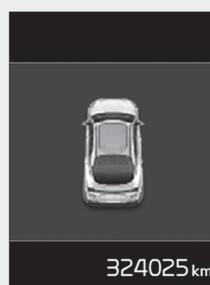
If the driver turns off the engine when the sunroof is not fully closed, the warning chime will sound for several seconds and the sunroof open warning will appear on the cluster LCD display.
