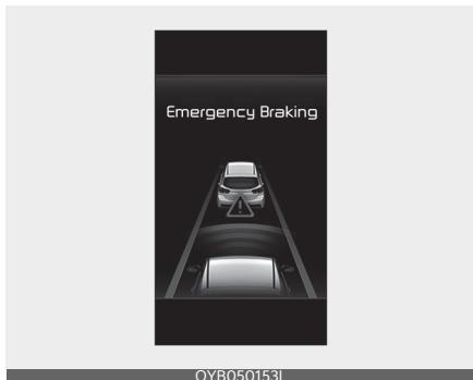
Additionally, some vehicle function intervention occurs by the engine management function to help decelerate the vehicle.
