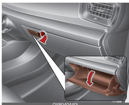
To open the glove box, pull the handle, and the glove box will automatically open. Close the glove box after use. Always keep the glove box closed while the vehicle is in motion.
