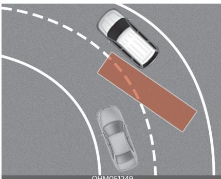
Blind-Spot Collision Warning may not operate properly when driving on a curved road. Blind-Spot Collision Warning may not detect the vehicle in the next lane.
