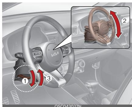
To change the steering wheel angle, pull down the lock release lever (1), adjust the steering wheel to the desired angle (2), then pull up the lock-release lever to lock (3) the steering wheel in place. Be sure to adjust the steering wheel to the desired position before driving.
