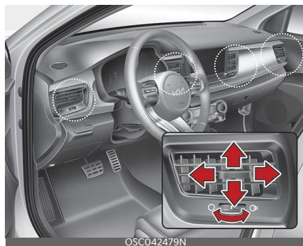
The outlet vents can be opened or closed separately using the thumbwheel. Also, you can adjust the direction of air delivered from these vents using the vent control lever as shown.
