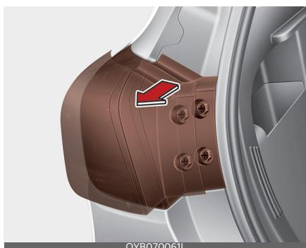
4. Disconnect the rear combination lamp connector.
