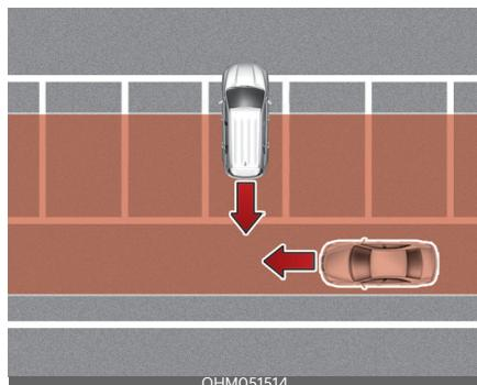
Rear Cross-Traffic Collision Warning may detect vehicles passing by behind you when parking backwards into a parking space. If this occurs, Rear Cross-Traffic Collision Warning may unnecessarily warn the driver. Always check your surroundings while backing up.
