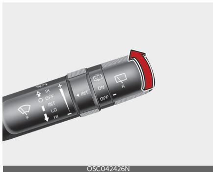
Push the lever away from you or turn the wiper lever switch upwards fully to spray rear washer fluid and to run the rear wipers 1~3 cycle. The spray and wiper operation will continue until you release the lever.
