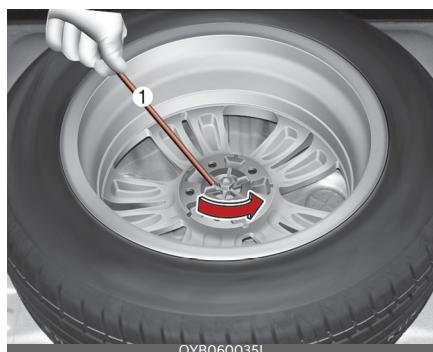
If it is hard to loosen the tire holddown wing bolt by hand, you can loosen it easily using the jack handle.
