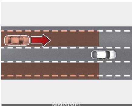
Blind-Spot Collision Warning helps detect and informs the driver that a vehicle is approaching at high speed from the blind spot area.
