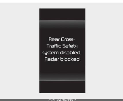
When the rear bumper around the rear-side radar or sensor is covered with foreign matters, such as snow or rain, or if you have installed a trailer or carrier, it can reduce the detecting performance and temporarily limit or disable Rear Cross-Traffic Collision Warning.
