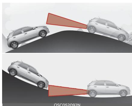
Blind-Spot Collision Warning may not operate properly when driving on a slope. Blind-Spot Collision Warning may not detect the vehicle in the next lane or may incorrectly detect the ground or structure.
