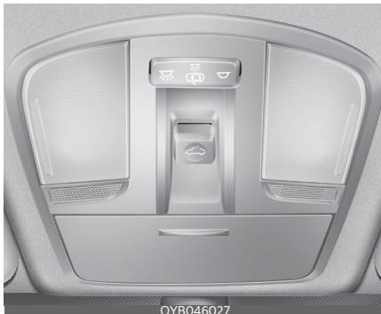
If your vehicle is equipped with a sunroof, you can slide or tilt your sunroof with the sunroof switch located on the overhead console.
