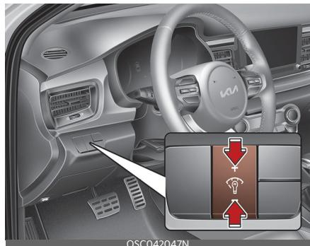
The instrument panel illumination intensity can be adjusted by pressing the control switch with the headlight switch in any position when the ignition or ENGINE START/STOP button is in the ON position.
