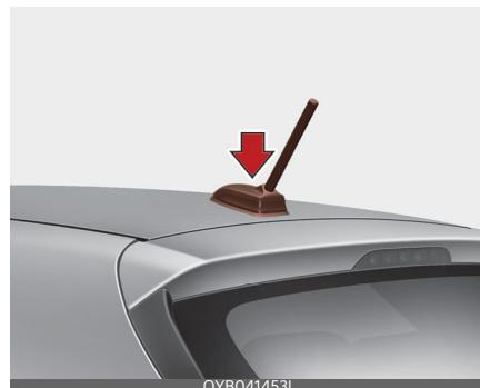
The micro pole antenna receives data transmitted from base stations and satellites (e.g. AM/FM, SXM, GPS, LTE) and also transmits to base stations (e.g. LTE). The antenna pole is removable type.
