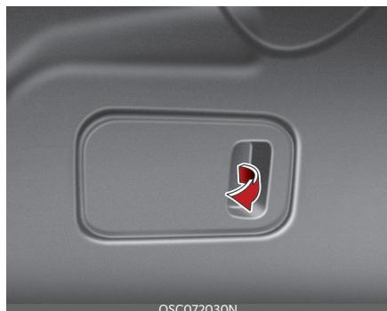
2. Remove the service cover by pulling out the service cover.
