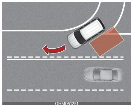
Blind-Spot Collision Warning may not operate properly when driving where the road merges or divides. Blind-Spot Collision Warning may not detect the vehicle in the next lane.
