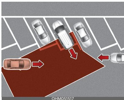
Rear Cross-Traffic Collision Warning may detect vehicles which are parking or pulling out near your vehicle (e.g. a vehicle leaving beside your vehicle, a vehicle parking or pulling out in the rear area, a vehicle approaching your vehicle making a turn, etc.). If this occurs, Rear Cross-Traffic Collision Warning may unnecessarily warn the driver.
