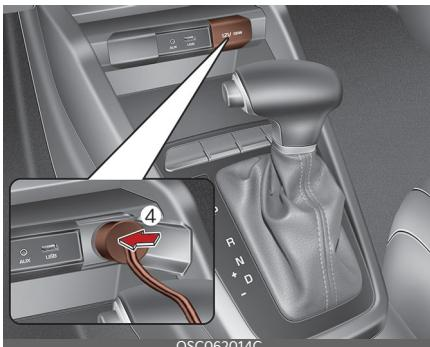
9. Connect between compressor and the vehicle power outlet (4) using the cable and connectors.
