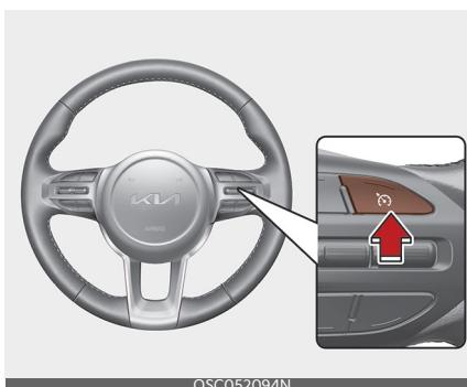
Press the Driving Assist
