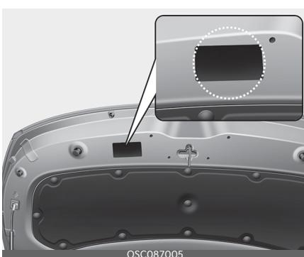
The refrigerant label is located on the underside of the hood.
