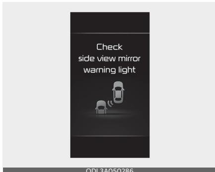
When the outside rearview mirror warning light is not working properly, the 'Check side view mirror warning light' warning message will appear on the cluster for several seconds, and the master (⚠) warning light will appear on the cluster. If this occurs, have your vehicle inspected by an authorized Kia dealer.
