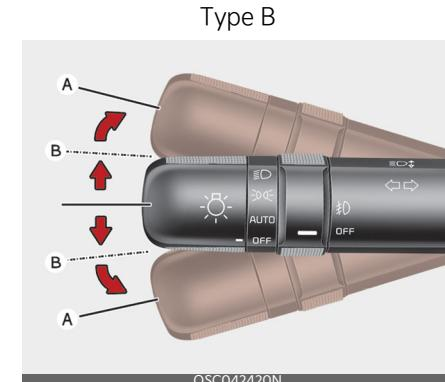
The ignition switch must be on for the turn signals to function. To turn on the turn signals, move the lever up or down (A). The green arrow indicators on the instrument panel indicate which turn signal is operating.
