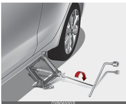
8. Insert the jack handle into the jack and turn it clockwise, raising the vehicle
