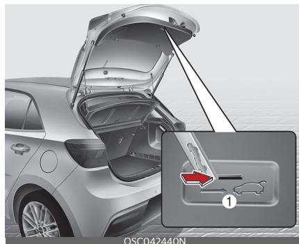
Your vehicle is equipped with the emergency liftgate safety release lever located on the bottom of the liftgate. If someone is inadvertently locked in the luggage compartment.
