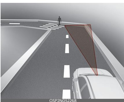
Forward Collision- Avoidance Assist may be limited when driving on a curved road.
