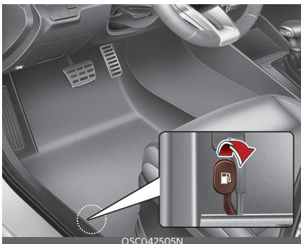
The fuel filler door must be opened from inside the vehicle by pulling up the fuel filler door opener.
