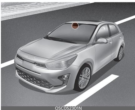
The front view camera is used to help detect driving patterns and front vehicle departure while vehicle is being driven.
