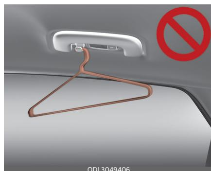
Do not hang other objects such as hangers or hard objects except clothes. Also, do not put heavy, sharp or breakable objects in clothing pockets. In an accident or when the curtain air bag is inflated, it may cause vehicle damage or personal injury.
