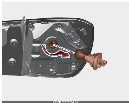
6. Remove the bulb from the socket by pressing it in and rotating it counterclockwise until the tabs on the bulb align with the slots in the socket. Pull the bulb out of the socket.
