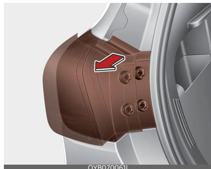
5. Disconnect the rear combination lamp connector.
