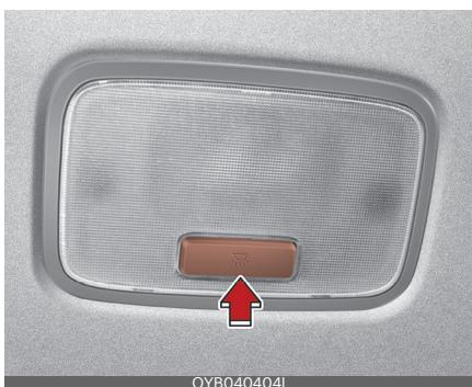
To turn the room lamp ON or OFF, push the switch.
