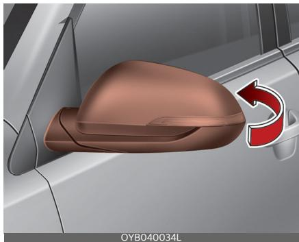
To fold the outside review mirror, grasp the housing of the mirror and then fold it toward the rear of the vehicle.
