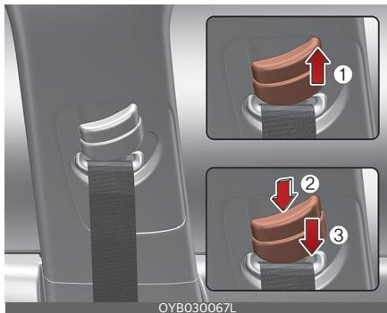
You can adjust the height of the shoulder belt anchor to one of the 3 positions for maximum comfort and safety.
