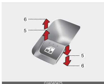
Pressing or pulling up the power window switch momentarily to the second detent position (6) completely lowers or lifts the
