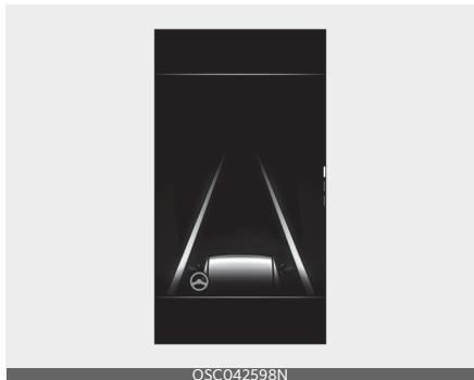
If the vehicle ahead or both lane markings are detected and your driving speed is below 190 km/h (120 mph), the green (Ⓐ) indicator light will illuminate on the cluster, and Lane Following Assist will help center the vehicle in the lane by assisting the steering wheel.
