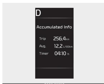
Displays accumulated information starting from a mileage/fuel efficiency/time default point.
