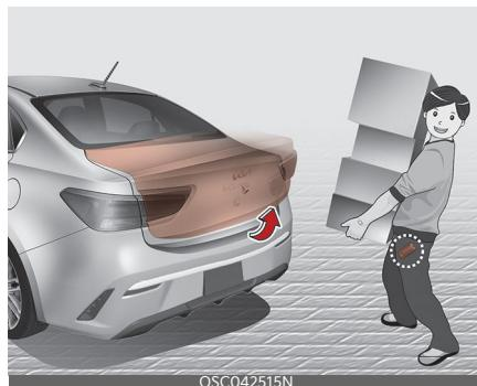
On a vehicle equipped with a smart key, the trunk can be opened with no-touch activation using the Smart Trunk Release system.
