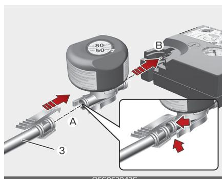
4. Connect the filling hose (3) onto the connector of the sealant bottle (A).
