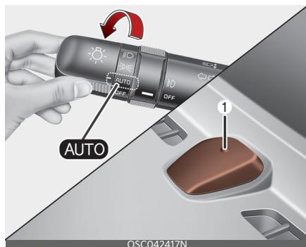
The parking lamp and headlamp will be turned ON or OFF automatically depending on the amount of daylight as measured by the ambient light sensor on the center dash.
