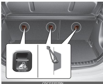
Child restraint hook holders are located on the package tray (4 Door) or the floor behind the rear seat (5 Door).
