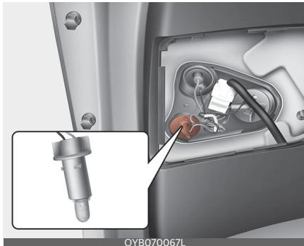
4. Remove the bulb from bulb-socket by pulling it out.
