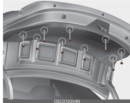
2. Loosen the retaining screw of the trunk lid cover and then remove the cover.
