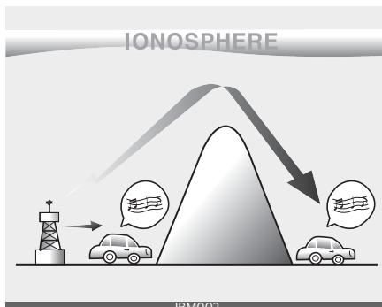
AM broadcasts can be received at greater distances than FM broadcasts. This is because AM radio waves are transmitted at low frequencies. These long, low frequency radio waves can follow the curvature of the earth rather than travelling straight out into the atmosphere. In addition, they curve around obstructions so that they can provide better signal coverage.
