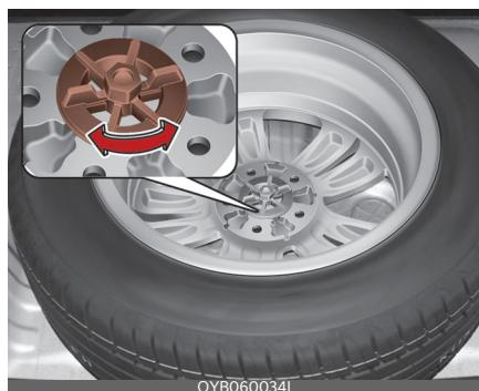
Turn the tire hold-down wing bolt counterclockwise to remove the spare tire.
