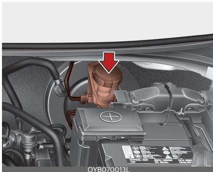
Check the fluid level in the reservoir periodically. The fluid level should be between the MAX (Maximum) and MIN (Minimum) marks on the side of the reservoir.
