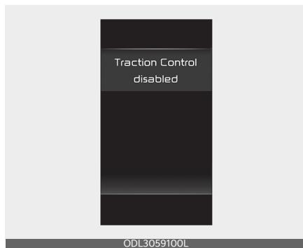
To turn off the traction control function and only operate the brake control function of the ESC, press the ESC OFF button (OFF) for less than 3 seconds and the ESC OFF indicator light (OFF) will illuminate. At this state, only the brake function will operate.
