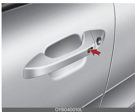
Pressing the button of the front outside door handles with all doors (and trunk,
