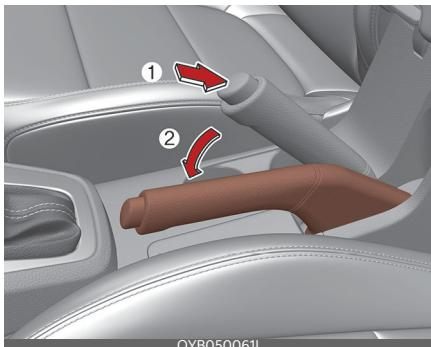
To release the parking brake, first apply the foot brake and pull up the parking brake lever slightly. Secondly, press the release button (1) and lower the parking brake lever (2) while holding the button.
