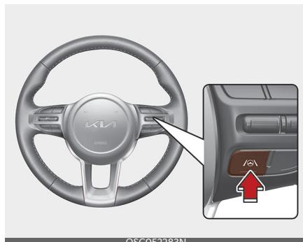
With the ignition switch or ENGINE START/STOP button in the ON position, press the Lane Driving Assist button (LFA) located on the steering wheel to turn on Lane Following Assist. The white or green (LFA) indicator light will illuminate on the cluster.
