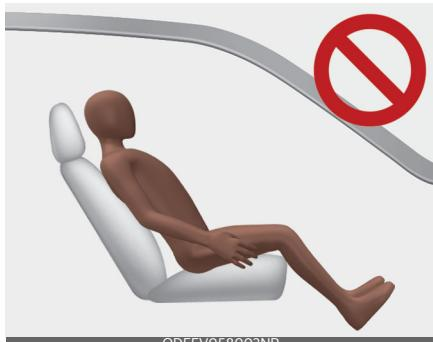
The driver must advise the passenger to keep the seatback in an upright position whenever the vehicle is in motion. If a
