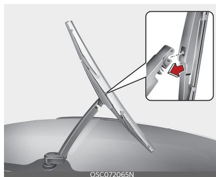
2. Compress the clip (1) and slide the blade assembly downward (2).
