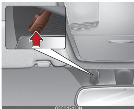
Auto defogging reduces the possibility of fogging up the inside of the windshield by automatically sensing the moisture inside the windshield and air flow toward the windshield can increase. The auto defogging system operates when the AUTO mode is on.
