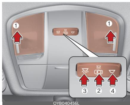
Push the lens (1) to turn the map lamp on or off. This light produces a spot beam for convenient use as a map lamp at night or as a personal lamp for the driver and front passenger.
