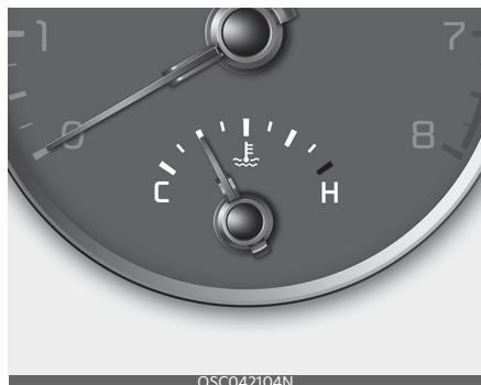
This gauge shows the temperature of the engine coolant when the ignition switch or ENGINE START/STOP button is ON.
