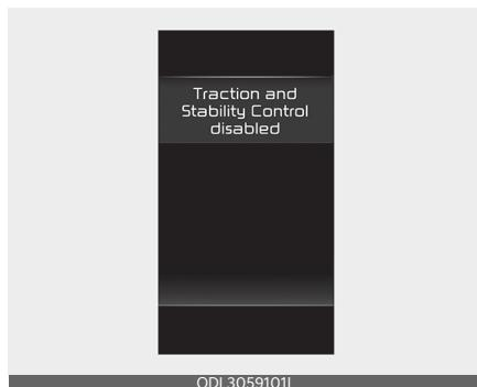
To turn off the traction control function and the brake control function of the ESC, press the ESC OFF button (OFF) for more than 3 seconds. ESC
