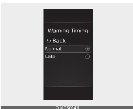
With the ignition switch or ENGINE START/STOP button in the ON position, select 'Driver Assistance → Warning Timing' from the User Settings menu to change the initial warning activation time for Rear Cross-Traffic Collision Warning.
