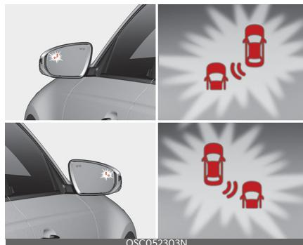
To warn the driver of an approaching vehicle from the rear left/right side of your vehicle, the outside rearview mirror will blink and a warning will appear on the cluster. At the same time, an audible warning will sound. If Rear View Monitor is operating, a warning will also appear on the infotainment screen.
