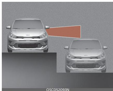
Blind-Spot Collision Warning may not operate properly when driving where the heights of the lanes are different. Blind-Spot Collision Warning may not detect the vehicle on a road with different lane heights (underpass joining section, grade separated intersections, etc.).
