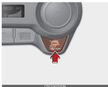
The defroster heats the window to remove frost, fog and thin ice from the interior and exterior of the rear window, while the engine is running.
