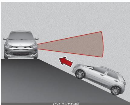
Rear Cross-Traffic Collision Warning may be limited when the vehicle is on an uphill or downhill slope, or near it, and may not detect the vehicle approaching from the left or right. If this occurs, Rear Cross-Traffic Collision Warning may not warn the driver when necessary.
