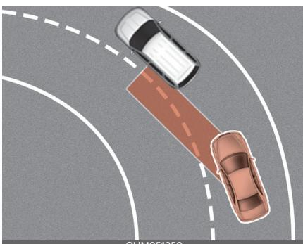
Blind-Spot Collision Warning may not operate properly when driving on the curved road. Blind-Spot Collision Warning may recognize the vehicle in the same lane.
