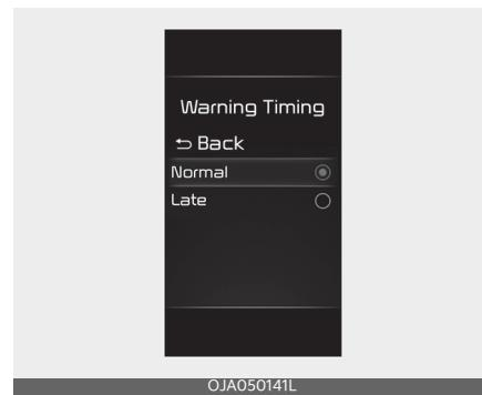
The driver can select the initial warning activation time in the User Settings in the LCD display by selecting "User Settings → Driver Assistance → Warning Timing". When the vehicle is first delivered, Warning Timing is set to 'Normal'. If you change the Warning Timing, the Warning Timing of other Driver Assistance functions may change. Make sure to check the Warning Timing before changing it.
