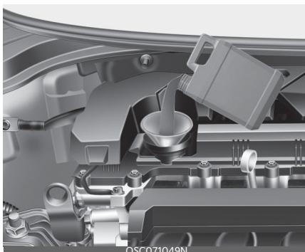
Use a funnel to help prevent oil from being spilled on engine components. Use only the specified engine oil. (Refer to "Recommended lubricants and capacities" on page 8-6.)
