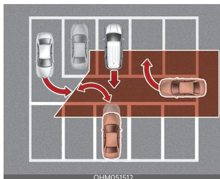
Rear Cross-Traffic Collision Warning may detect vehicles which are parking or pulling out near your vehicle (e.g. a
