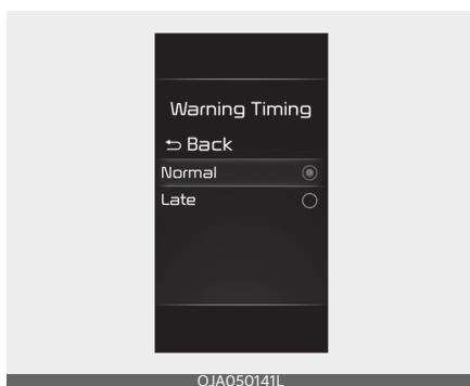
With the ignition switch or ENGINE START/STOP button in the ON position, select 'Driver Assistance → Warning Timing' from the User Settings to change the initial warning activation time for Blind-Spot Collision Warning. When the vehicle is first delivered, Warning Timing is set to 'Normal'. If you change the Warning Timing, the Warning Timing of other Driver Assistance functions may change.
