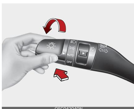
High Beam Assist is a function that automatically adjusts the headlamp range (switches between high beam and low beam) according to the brightness of other vehicles and road conditions.
