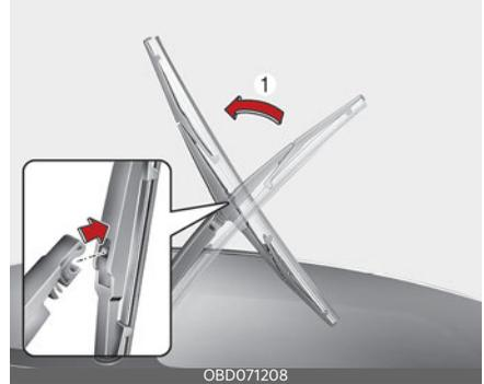
2. Install the new blade assembly by inserting the center part into the slot in the wiper arm until it clicks into the place.
