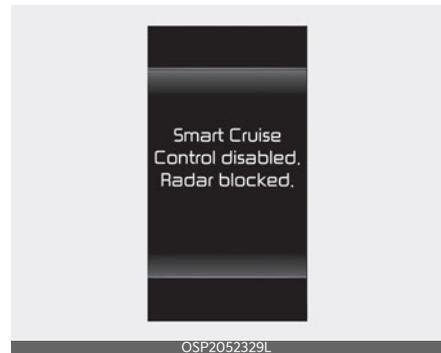
When the front radar cover or sensor is covered with snow, rain, or foreign matters, it can reduce the detecting performance and temporarily limit or disable SCC.
