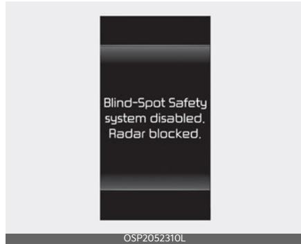
When the rear bumper around the rear-side radar or sensor is covered with foreign matters, such as snow or rain, or installing a trailer or carrier, it can reduce the detecting performance and temporarily limit or disable SEW.
