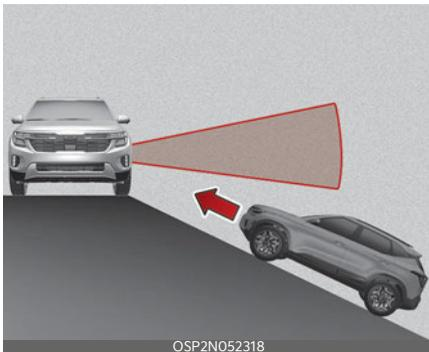
RCCA may be limited when the vehicle is on an uphill or downhill slope, or near it, and may not detect a vehicle approaching from the left or right. RCCA may not warn you or control the brakes when necessary.
