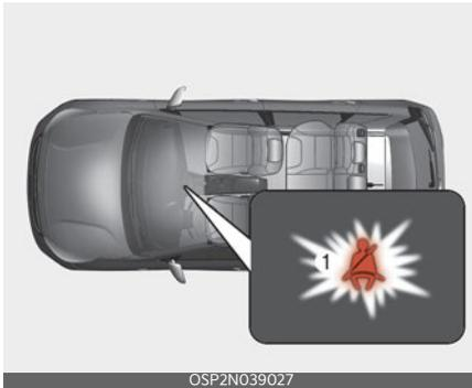
If you start to drive without the passenger seat belt fastened or you unfasten the seat belt when you drive 12 mph (20 km/h) and faster, the warning light will blink and the warning chime will sound for approximately 100 seconds. When the passenger seat belt is unfastened during driving, the warning light will appear when the speed is under 12 mph (20 km/h). When the speed is 12 mph (20 km/h) and faster, the warning light
