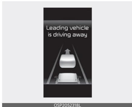
When a detected vehicle in front departs from a stop, Leading Vehicle Departure Alert will inform you by displaying the warning message on the instrument cluster and an audible warning will sound.
