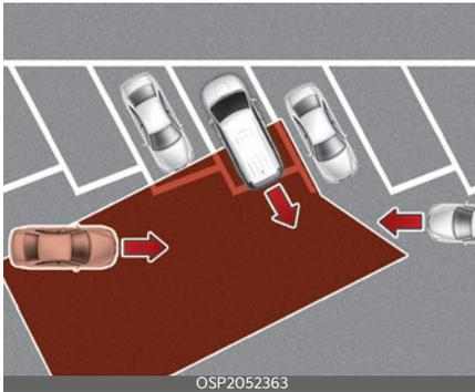
RCCA may be limited when backing up diagonally and may not detect a vehicle approaching from the left or right. If this occurs, RCCA may not warn you or control the brakes when necessary.
