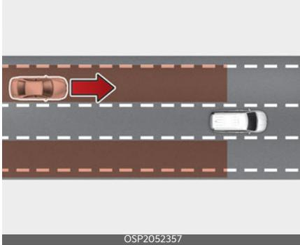
BCA helps detect and informs the driver that a vehicle is approaching at high speed from the blind spot area.
