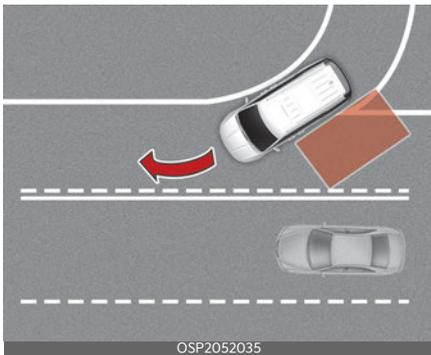
BCA may not operate properly when driving where the road merges or divides. BCA may not detect the vehicle in the next lane. Always pay attention to road and driving conditions.
