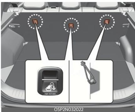
First secure the child restraint with the LATCH lower anchors or the seat belt. If the child restraint manufacturer recommends that the top tether strap be
