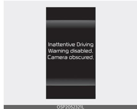
When the front view camera is located is covered with foreign material, such as snow or rain, it can reduce the detecting performance and temporarily limit or disable DAW. The warning message, and (⚠) warning light will appear on the instrument cluster. DAW will operate normally when snow, rain or foreign material is removed. Always keep it clean.
