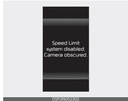
When the windshield where the front view camera is located is covered with foreign material, such as snow or rain, it can reduce the detecting performance and temporarily limit or disable ISLA. The warning message and speed limit warning light (⚠) will appear on the instrument cluster.
