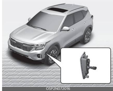
1. Remove the lamp assembly from the vehicle by prying the cover and pulling the assembly out.
