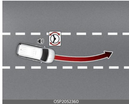
LKA is designed to help detect lane markings (or road edges) while driving over a certain speed. Lane Keeping Assist will warn the driver if the vehicle leaves the lane without using the turn signal, or will automatically assist the driver's steering to help prevent the vehicle from departing the lane.
