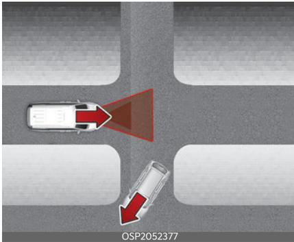
When a vehicle ahead disappears from an intersection, your vehicle may accelerate. Always pay attention to road and driving conditions.
