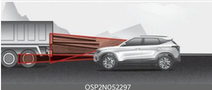
When the vehicle in front has heavy loading extended rearward, or when the vehicle in front has higher ground clearance, it may induce a hazardous situation. Always pay attention to road and driving conditions, while driving and, if necessary, depress the brake pedal to reduce your driving speed in order to maintain distance.
