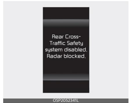
When the rear bumper around the rear corner radar or sensor is covered with foreign matters, such as snow or rain, or installing a trailer or carrier, it can reduce the detecting performance and temporarily limit or disable RCCA.
