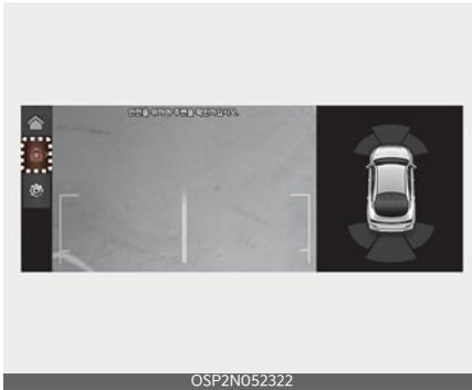
When you touch the
