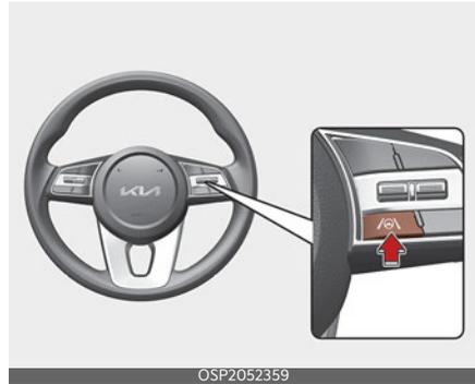
With the ignition switch or ENGINE START/STOP button in the ON position, press the Lane Driving Assist button located on the steering wheel to turn on LFA. The white or green (🚗) indicator light will appear on the cluster. Press the LFA button again to turn off the function.
