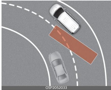
BCA may not operate properly when driving on a curved road. BCA may not detect the vehicle in the next lane.
