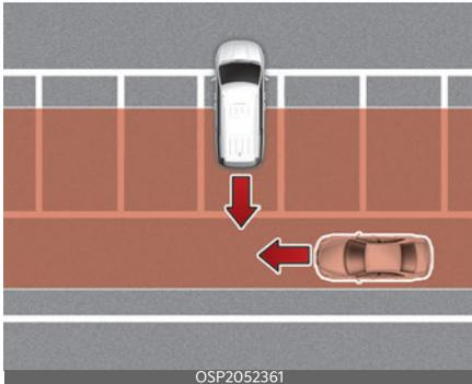
RCCA may detect vehicles passing by behind you when parking backwards into a parking space. If this occurs, RCCA may unnecessarily warn the driver and control the brake.
