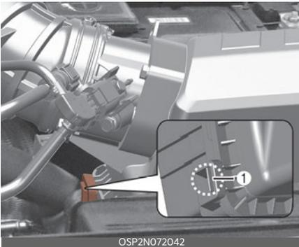
5. Check that the cover is firmly installed.
