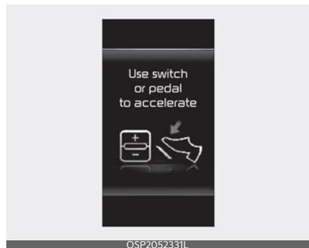
In traffic, your vehicle will stop if a vehicle ahead of you stops. If a vehicle ahead of you starts moving, your vehicle will start as well. After your vehicle has stopped and a certain time has passed, the warning message will appear on the
