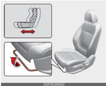
Adjust the seat before driving, and make sure the seat is locked securely by trying to move forward and backward without using the lever. If the seat moves, it is not locked properly.
