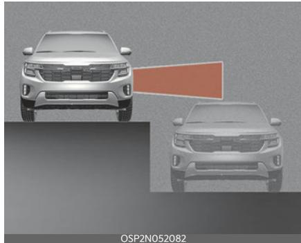
BCA may not operate properly when driving where the heights of the lanes are different. BCA may not detect the vehicle on a road with different lane heights (underpass joining section, grade separated intersections, etc.). Always pay attention to road and driving conditions.
