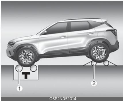
1. Place the front wheels on the roll tester (1) for a speedometer test as shown in the illustration.
