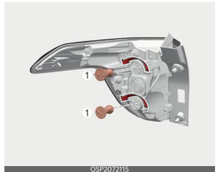
8. Install the socket in the assembly by aligning the tabs on the socket with the slots in the assembly.
