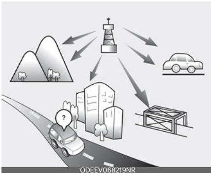
FM broadcasts are transmitted at high frequencies and do not bend to follow the earth's surface. Because of this, FM broadcasts generally begin to fade within short distances from the station. FM signals are easily affected by buildings, mountains, and obstructions. This can lead to unpleasant listening conditions which might lead you to believe a problem exists with your radio.
