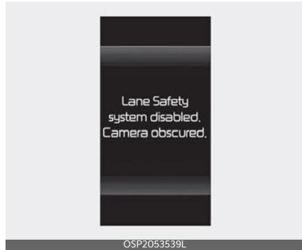
If foreign materials such as snow or rain block the sensors or the windshield where the front view camera is located, the detecting performance may be reduced, resulting in Lane Keeping Assist temporarily limited or disabled.
