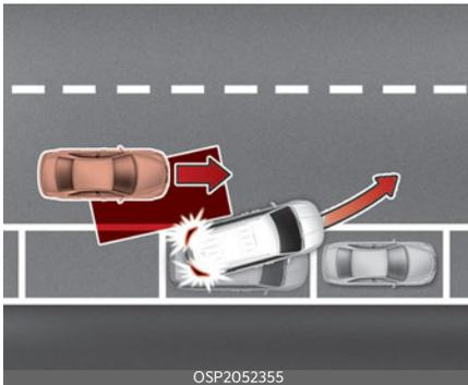
When you are driving forward out of a parking space, if BCA determines that there is a collision risk with an approaching vehicle in the blind spot, it can help avoid collisions by applying the brake.
