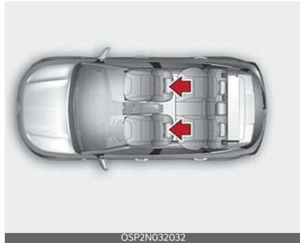
The headrest not only provides comfort for the driver and front passenger, but also helps protect the head and neck in the event of a rear collision.
