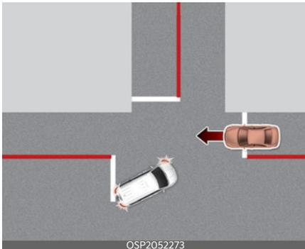
Junction Turning function can help avoid or mitigate a collision with an oncoming vehicle in an adjacent lane when turning left at a crossroad with the turn signal on by applying emergency braking.
