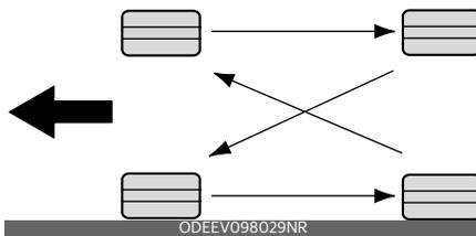
Rotate radial tires that have an asymmetric tread pattern only from front to rear and not from right to left.
