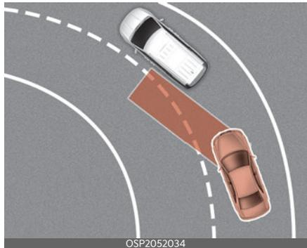
BCA may not operate properly when driving on the curved road. BCA may recognize the vehicle in the same lane.
