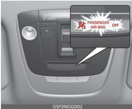
The ODS is designed to detect the presence of a properly seated front passenger and determine if the passenger's front air bag should be activated (may inflate) or not. Only the front passenger front air bag is controlled by the ODS.
