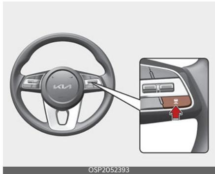
Each time the Vehicle Distance button is pressed, the Vehicle Distance changes as follows. Stage 1 indicates the nearest distance.
