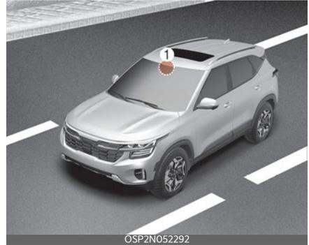
The front view camera is used as a detecting sensor to detect lane markings and front vehicles. Refer to the picture above for the detailed location of the detecting sensor.
