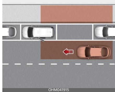
After the vehicle stops, when an approaching vehicle from the rear area is detected as soon as a passenger opens a door, SEW will warn the driver with a warning message and an audible warning to help prevent a collision.
