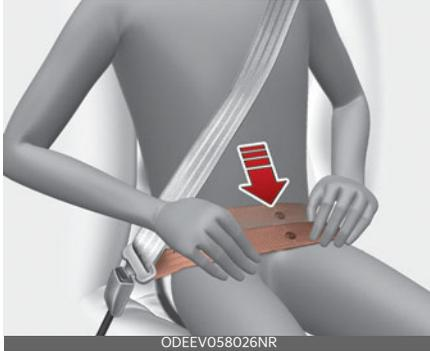
The arm closest to the seat belt buckle should be over the belt while the other arm should be under the belt as shown in the illustration. Never wear the seat belt under the arm closest to the door.
