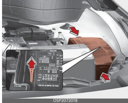
4. Check the removed fuse; replace it if it is blown.
