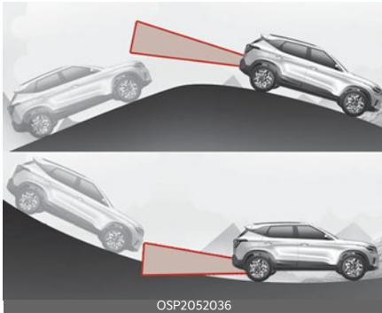
BCA may not operate properly when driving on a slope. BCA may not detect a vehicle in the next lane or may incorrectly detect the ground or structure. Always pay attention to road and driving conditions.
