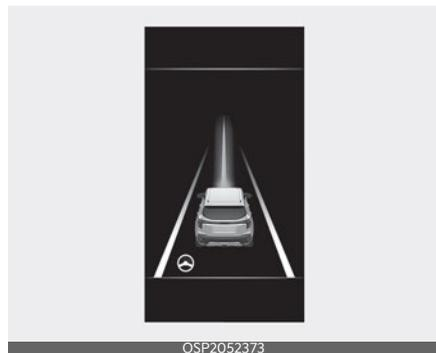
If a vehicle ahead or both lane markings are detected and your speed is below 110 mph (180 km/h), the green (🚗)
