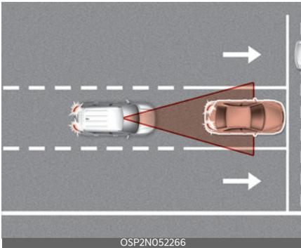
FCA is designed to help detect and monitor the vehicle ahead or help detect a pedestrian or cyclist in the roadway and warn the driver that a collision is imminent with a warning message, audible warning and emergency braking.
