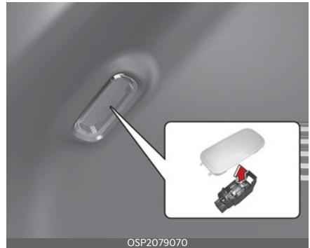
1. Using a flat-blade screwdriver, gently pry the lens cover from lamp housing.
