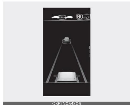
If you want to speed up temporarily when SCC is on, depress the accelerator pedal for a certain amount. While depressing the accelerator pedal for a certain amount, the set speed, distance level and target distance will blink on the instrument cluster. If the accelerator pedal is insufficiently depressed, the vehicle may slow down.
