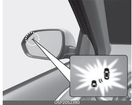
The warning light on the outside rear view mirror and head-up display (if equipped) will appear when the vehicle on both lanes is detected from the rear. A Vehicle detection will operate in the following conditions.
