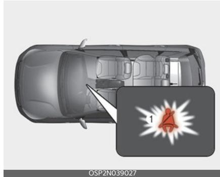
If you start to drive without the seat belt fastened over 5 mph (9 km/h) and less than 12 mph (20 km/h), the corresponding warning light will appear. The warning light will turn off when the vehicle speed drops below 5 mph (9 km/h).
