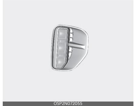
If the LED (1) lamp is not functioning, please have your vehicle inspected by an authorized Kia dealer. The LED lamp cannot be replaced as an individual component since it is an integrated unit. Instead, the entire LED lamp unit must be replaced.
