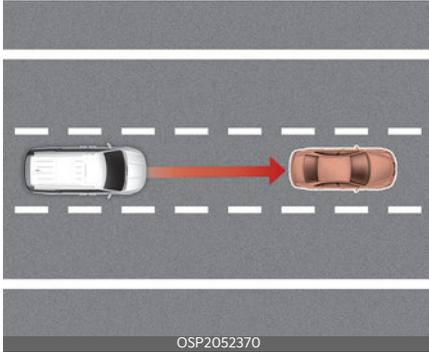
HDA is designed to help detect vehicles and lanes ahead, and help maintain distance from a vehicle ahead, maintain the set speed, help center your vehicle in the lane while driving on the highway.
