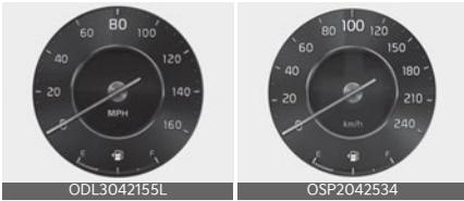
The speedometer indicates the speed of the vehicle and is calibrated in miles per hour (mph) and/or kilometers per hour (km/h).
