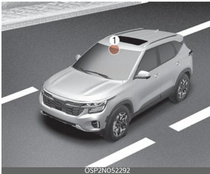
The front view camera is used as a detecting sensor to help detect driving patterns and front vehicle departure while your vehicle is being driven. Refer to the picture above for the detailed location of the detecting sensor.
