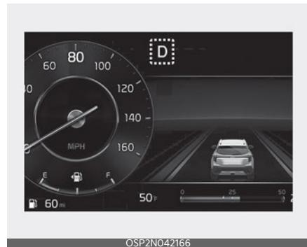
This indicator displays which Automatic Transmission/Intelligent Variable Transmission shift lever is selected.
