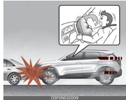
Front air bags may inflate in a frontal collision depending on several factors, including the severity of impact of the front collision.
