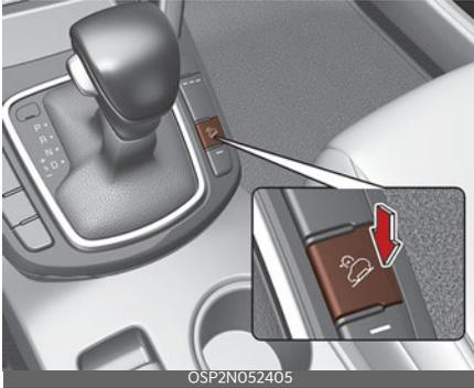
The DBC assists the driver to descend down a steep hill without having to depress the brake pedal.
