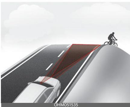
Forward Collision-Avoidance Assist may not detect other vehicle, pedestrian or cyclist in front while driving uphill or downhill and this may result
