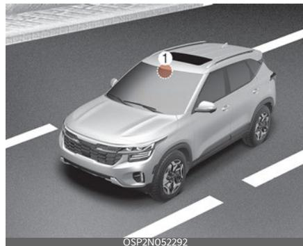
The front view camera is used as a detecting sensor to detect lane markings (or road edges).
