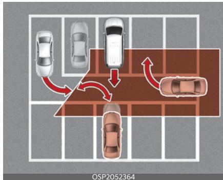
RCCA may detect vehicles which are parking or pulling out near your vehicle (for example, a vehicle leaving beside
