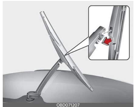
3. Make sure the blade assembly is installed firmly by trying to pull it slightly. To prevent damage to the wiper arms or other components, have the wiper blade replaced by an authorized Kia dealer.
