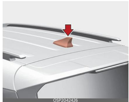
Shark-fin antenna transmit and receive signals such as AM/FM and GPS. Addi-
