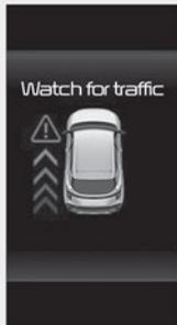
The warning light on the side view mirror will blink and the warning message will appear on the instrument cluster, and an audible warning will sound.
