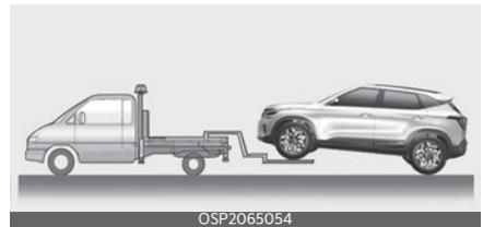
2-wheel drive vehicle can be towed with the opposite tires on the ground (without dollies) and parking brake released before turning off the vehicle.
