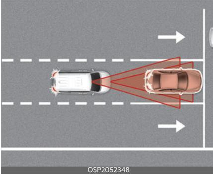
FCA is designed to help detect and monitor the vehicle ahead or help detect a pedestrian or cyclist in the roadway and warn the driver that a collision is imminent with a warning message, audible warning and apply emergency braking.
