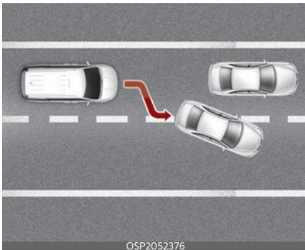
When a vehicle in front of you merges out of the lane, SCC may not immediately detect the new vehicle that is now in front of you. Always pay attention to road and driving conditions while driving.
