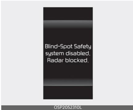
When the rear bumper around the rear corner radar or sensor is covered with foreign material, such as snow or rain, or installing a trailer or carrier, it can reduce the detecting performance and temporarily limit or disable BCA.
