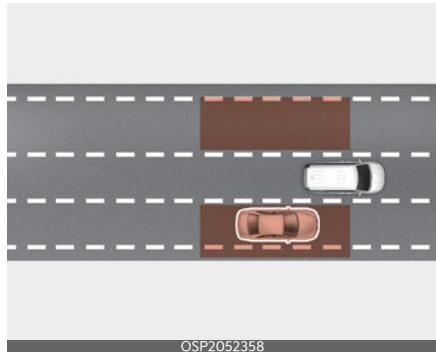
BCA helps detect and informs the driver that a vehicle is in the blind spot.
