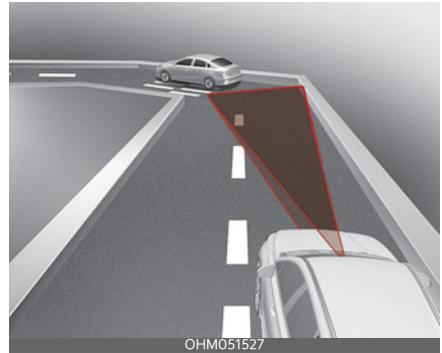
On curves, SCC may not detect a vehicle in the same lane, and may accelerate to the set speed. Vehicle speed may rapidly decrease when the vehicle ahead is detected suddenly.
