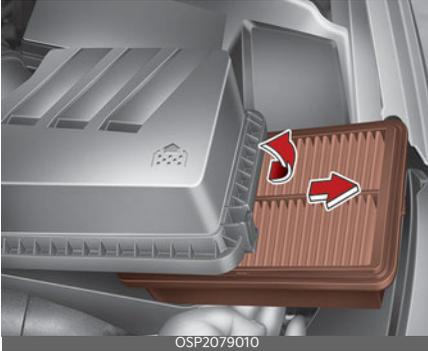
4. Insert the air cleaner cover in the hinge (1) and close the cover, then lock the cover with attaching clips.
