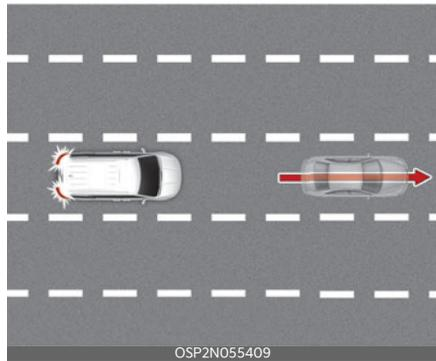
If a vehicle in front abruptly departs, Leading Vehicle Departure Alert may not operate properly.
