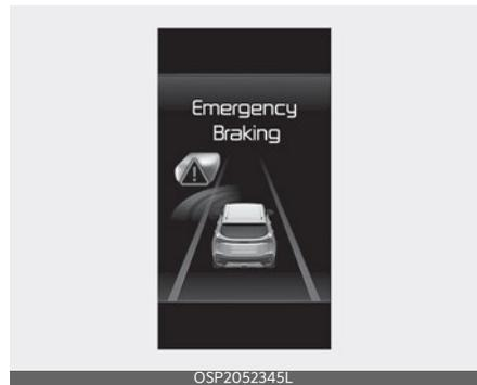
The warning message and an audible warning to warn the driver that emergency braking will be assisted. The brake assist will be activated and it helps avoiding collision of a vehicle. Emergency braking will be activated in the following conditions.
