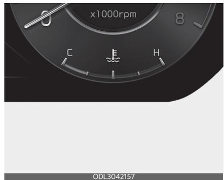
This gauge indicates the temperature of the engine coolant when the ignition
