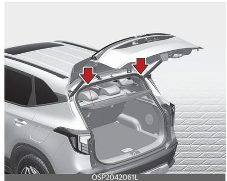
2. Whilst lifting the cover up, hold the area near the front slots. Then, pull up the cover at approximately 45° angle.
