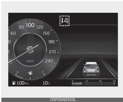
In the Sports Mode, this indicator informs which gear is desired whilst driving to save fuel.
