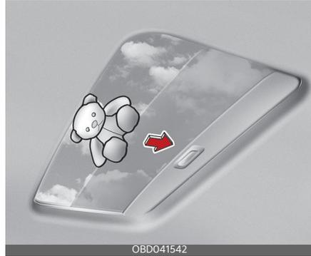
If the sunroof glass senses any obstacle whilst it is closing automatically, it will reverse direction then stop at a certain position. The auto reverse function may not work if an object thin or soft is caught between the sliding sunroof glass and sunroof sash.
