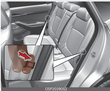
Then, insert the seat belt into the two holes located on both sides.
