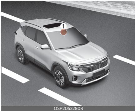
The front view camera is used as a detecting sensor to detect ambient light and brightness whilst driving. Refer to the picture for the detailed location of the detecting sensor.
