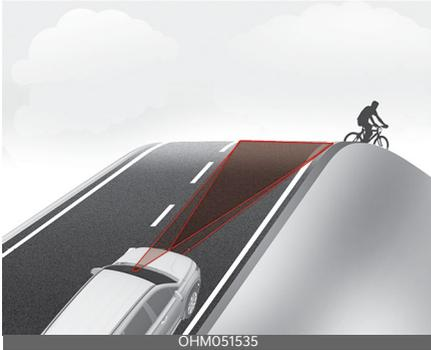
Forward Collision-Avoidance Assist may not detect other vehicle, pedestrian or cyclist in front whilst driving uphill or downhill and this may result in no warning, or braking assist when necessary.
