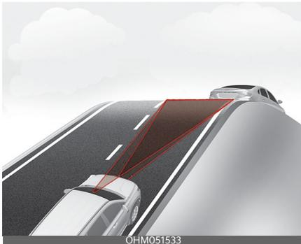
During uphill or downhill driving, Smart Cruise Control may not detect a moving vehicle in your lane, and cause your vehicle to accelerate to the set speed. Also, vehicle speed will rapidly decrease when the vehicle ahead is detected suddenly.
