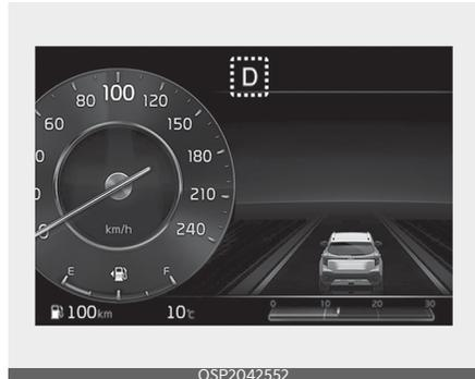
This indicator displays which Automatic Transmission/Intelligent Variable Transmission shift lever is selected.
