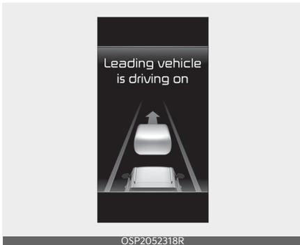
When a detected vehicle in front departs from a stop, Leading Vehicle Departure Alert will inform the driver by displaying the warning message on the cluster and an audible warning will sound.
