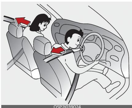
Your vehicle is equipped with pre-tensioner seat belts at the front or front/rear seating positions.
