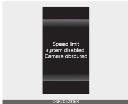
When the front windscreen where the front view camera is located is covered with foreign material, such as snow or rain, it can reduce the detecting performance and temporarily limit or disable Intelligent Speed Limit Assist. If this occurs, the warning message and speed limit warning light (---) will appear on the cluster.
