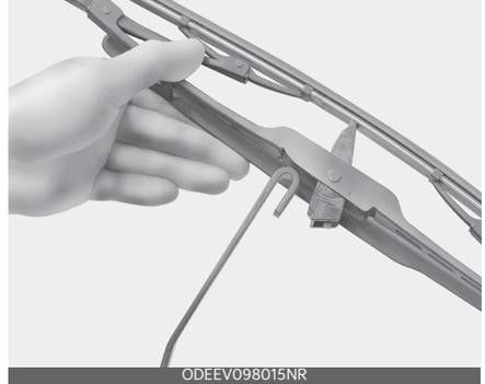
4. Install the blade assembly in the reverse order of removal.
