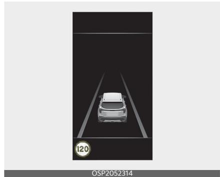
When driving at a speed higher than the displayed speed limit, the road sign indicator will blink and warning will sound.
