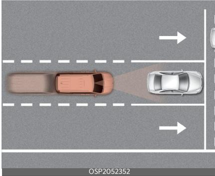
Forward Collision-Avoidance Assist is designed to help detect and monitor the vehicle ahead or help detect a pedestrian or cyclist in the roadway and warn the driver that a collision is imminent with a warning message, audible warning and apply emergency braking.
