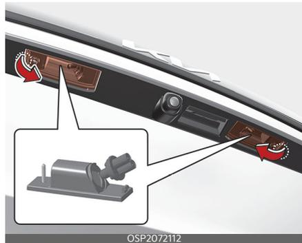
1. Using a screwdriver, gently pry the lamp assembly from interior.
