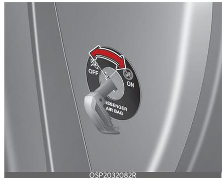
The passenger's front air bag can be deactivated by the passenger's front air bag ON/OFF switch if a child restraint is installed on the front passenger's seat or if the front passenger's seat is unoccupied by a person.
