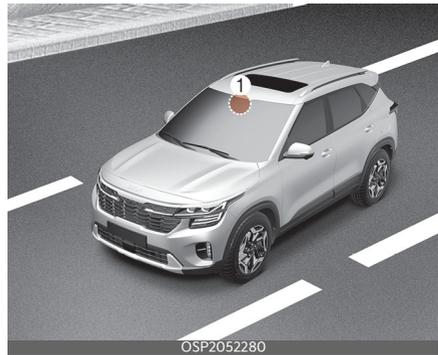
The front view camera is used as a detecting sensor to help detect driving patterns and front vehicle departure whilst vehicle is being driven. Refer to the picture above for the detailed location of the detecting sensor.
