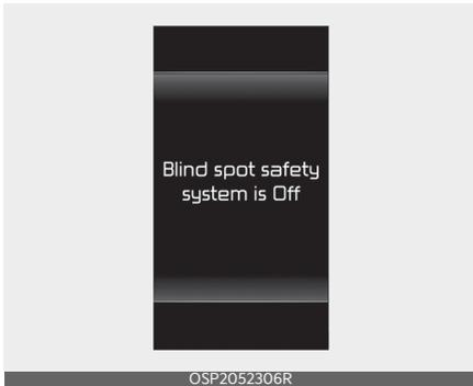
When activating Blind-Spot Collision-Avoidance Assist or restarting the vehicle with this function activated, the warning light on the side mirrors will appear for approximately 3 seconds. When the vehicle is restarted with Blind-Spot Collision-Avoidance Assist inactivated, the warning message will appear on the cluster.
