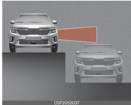
Blind-Spot Collision-Avoidance assist may not operate properly when driving where the heights of the lanes are different. Blind-Spot Collision-Avoidance Assist may not detect the vehicle on a road with different lane heights (underpass joining section, grade separated intersections, etc.).
