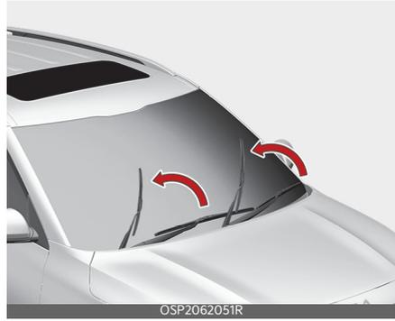
To inspect or replace the windscreen wiper blades and to prevent damaging the bonnet, move the windscreen wiper blades as follows;
