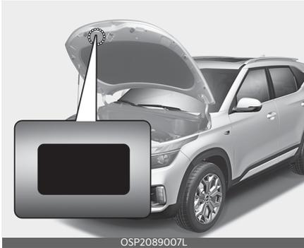
The refrigerant label is located on the underside of the bonnet.
