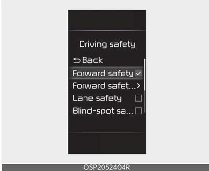
With the ignition switch or ENGINE START/STOP button in the ON position, select 'User settings → Driver assistance → Driving safety' on the LCD display or 'Settings → Vehicle → Driver assistance → Driving safety' on the Infotainment system screen to set whether to use the function.
