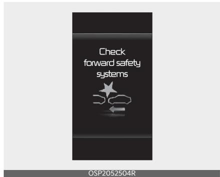
When Forward Collision-Avoidance Assist is not working properly, the warning message will appear and the
