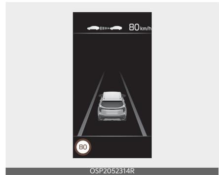
When operating Manual Speed Limit Assist or Smart Cruise Control, if the speed set by the driver is the same as the speed limit on the road, the set speed is automatically adjusted accordingly even if the speed limit changes afterwards. The auto set speed change function operates on roads with a speed limit of above 70 km/h (45 mph). When the function is activated, the set speed on the instrument cluster is displayed in green.
