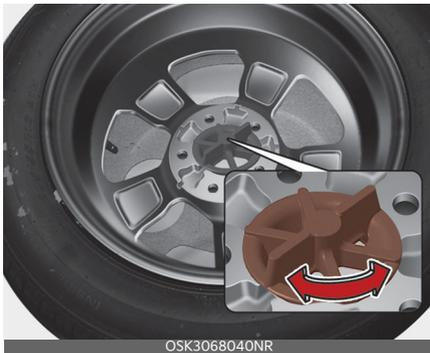
Turn the tyre hold-down wing bolt counterclockwise to remove.
