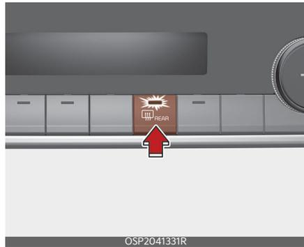
The defroster heats the window to remove frost, fog and thin ice from the rear window, whilst the engine is running. To activate the rear window defroster, press the rear window defroster button.
