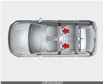
The headrest not only provides comfort for the driver and front passenger, but also helps protect the head and neck in the event of a collision.
