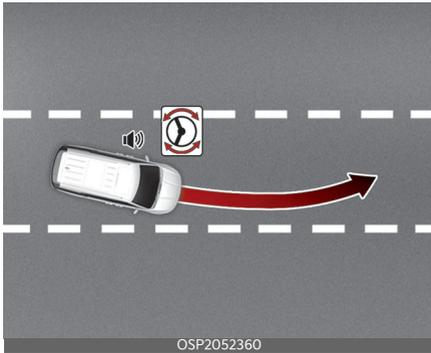
Lane Keeping Assist is designed to help detect lane markings (or road edges) whilst driving over a certain speed. Lane Keeping Assist will warn the driver if the vehicle leaves the lane without using the turn signal, or will automatically assist the driver's steering to help prevent the vehicle from departing the lane.
