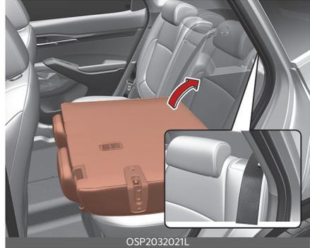
2. Make sure the seatback is locked in place. When you return the seatback to its upright position, always be sure it has locked into position by pushing on the top of the seatback. If you can not see the red line at the bottom of folding lever, it means the seatback is locked completely.
