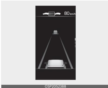
If you want to speed up temporarily when Smart Cruise Control is on, depress the accelerator pedal for a certain amount. Whilst depressing the accelerator pedal for a certain amount, the set speed, distance level and target distance will blink on the cluster. However, if the accelerator pedal is insufficiently depressed, the vehicle may slow down.
