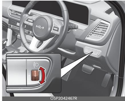
To adjust the headlight beam level according to the number of the passengers and loading weight in the luggage area, turn the beam levelling switch.
