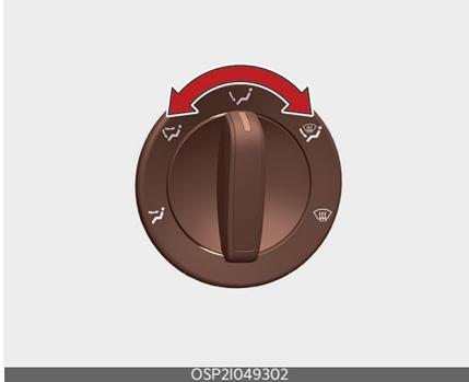
Air can be directed to the floor, dashboard outlets, or windscreen. Five symbols are used to represent Face, Bi-Level, Floor, Floor-Defrost and Defrost air position.
