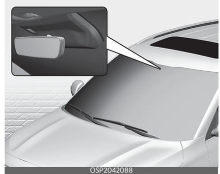
Auto defogging reduces the possibility of fogging up the inside of the windscreen by automatically sensing the moisture of inside the windscreen.
