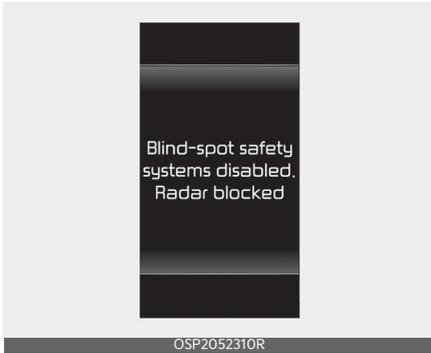
When the rear bumper around the rear-side radar or sensor is covered with foreign matters, such as snow or rain, or installing a trailer or carrier, it can reduce the detecting performance and temporarily limit or disable Safe Exit Warning. If this occurs, the 'Blind-spot safety systems disabled. Radar blocked' warning message will appear on the cluster.
