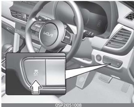
ESC applies the brakes on individual wheels and intervenes with the vehicle management system to stabilize the vehicle.
