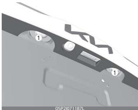
1. Using a screwdriver, gently pry the lamp assembly from interior.
