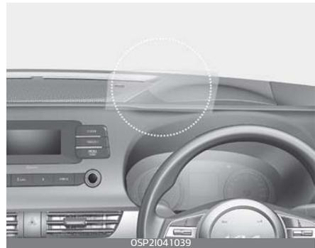
The hidden screen will go up when you press the screen operation switch on the left side of the lower part of crash pad and if you press the switch again, the screen will return to its original hidden position.
