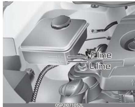
8. If the coolant level is low, add enough specified coolant to provide protection against freezing and corrosion. Bring the level to F, but do not overfill.
