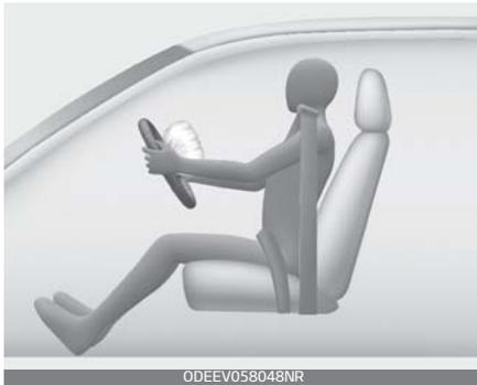
The air bag modules are located both in the center of the steering wheel and in the front passenger's panel above the glove box. When the SRSCM detects a sufficiently severe impact to the front of the vehicle, it will automatically deploy the front air bags.
