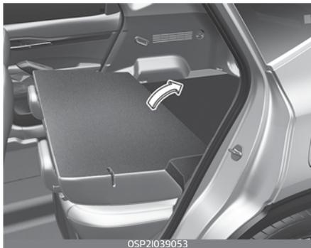
2. Make sure the seatback is locked in place. When you return the seatback to its upright position, always be sure it has locked into position by pushing on the top of the seatback.
