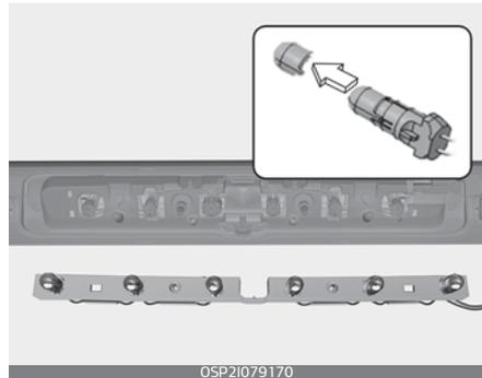
7. Insert a new bulb in the socket.
