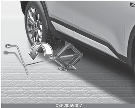
9. Loosen the wheel nuts and remove them with your fingers. Slide the wheel off the studs and lay it flat so it cannot roll away. To put the wheel on the hub, pick up the spare tire, line up the holes with the studs and slide the wheel onto them. If this is difficult, tip the wheel slightly and get the top hole in the wheel lined up with the top stud. Then jiggle the wheel back and forth until the wheel can be slid over the other studs.
