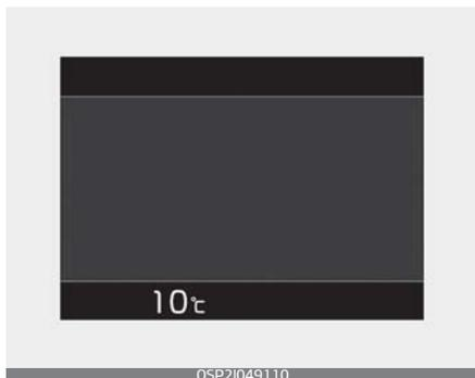
This gauge indicates the current outside air temperatures by 1 °C (1 °F).
