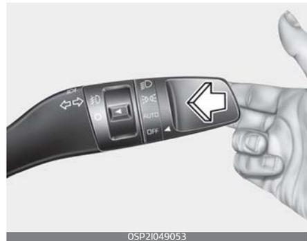
It will return to the normal (low beam) position when released. The headlight switch does not need to be on to use this flashing feature.
