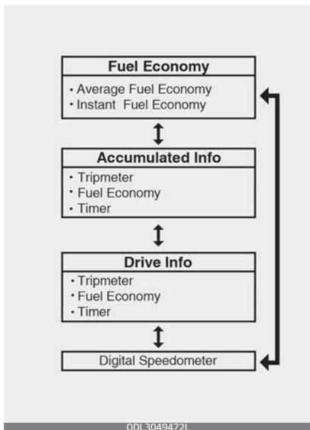
To change the trip mode, scroll the toggle the switch (∧ / ∨) on the steering wheel.
