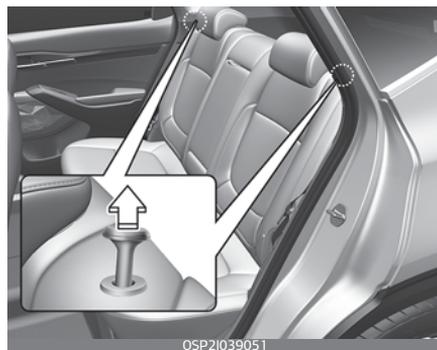
1. Pull up both sides of the seatback folding lever.
