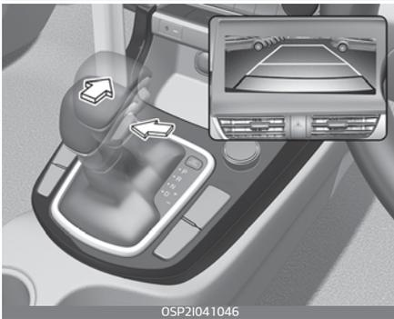
Rear View Monitor with parking guidance will activate when the engine is running and the shift lever is in the R (Reverse) position.
