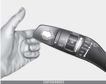
1. Move the wiper speed control switch to In OFF position.
