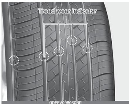
This shows there is less than 1.6 mm of tread left on the tire. Replace the tire when this happens.
