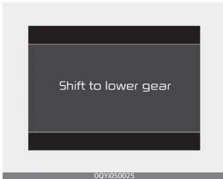
It is possible to drive on a slope with the gear is in first but the following warning message appears when the driver operates while the gear is in above second.
