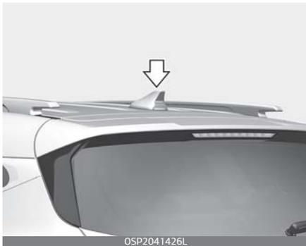
The roof antenna transmits and receives wireless signals such as AM/FM, Sirius XM, GNSS, etc.
