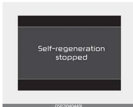
The regeneration operation could be canceled if the driver press the OK button firmly while operating the self regeneration process.
