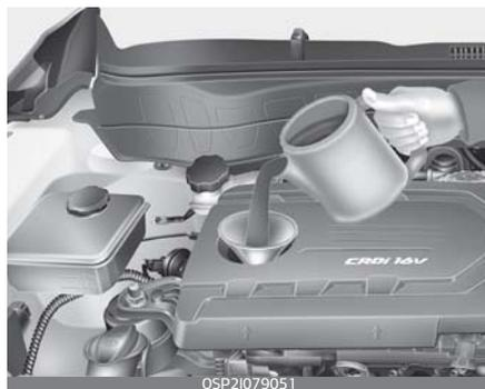
Use only the specified engine oil. (Refer to "Recommended lubricants and capacities" on page 9-7.)
