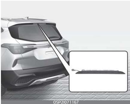
3. Remove the three round head cap nut fixing the high mounted stop lamp using a wrench.
