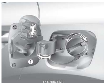
4. To remove the cap, turn the fuel filler cap counterclockwise.
