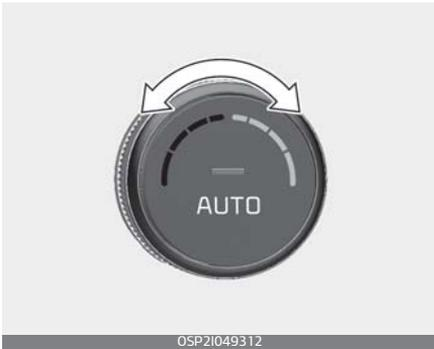
The temperature will increase to the maximum (HI) by rotating the knob clockwise direction. The temperature will decrease to the minimum (Lo) by rotating the knob anti clock wise direction. When rotating the knob, the temperature will increase or decrease by 0.5 °C. When set to the lowest temperature setting, the air
