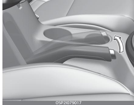
Check the stroke of the parking brake by counting the number of "clicks" heard while fully applying it from the released position. Also, the parking brake alone should securely hold the vehicle on a fairly steep grade. If the stroke is more or less than specified, we recommend that the system be inspected by an authorized kia dealer.
