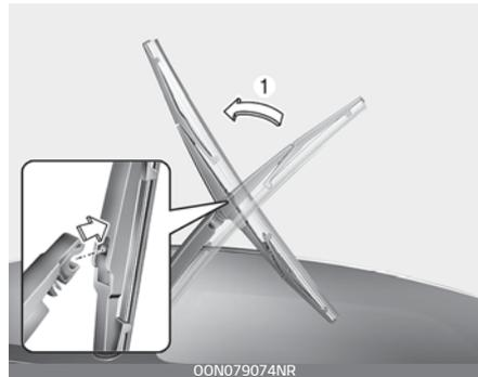
3. Install the new blade assembly by inserting the center part into the slot in the wiper arm until it clicks into place.
