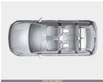
The headrest not only provides comfort for the driver and front passenger, but also helps protect the head and neck in the event of a collision.
