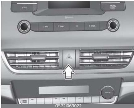
It should be used whenever emergency repairs are being made or when the vehicle is stopped near the edge of a roadway.
