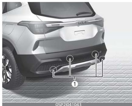
This function is a supplemental function and it is not intended to nor does it replace the need for extreme care and attention of the driver. The sensing range and objects detectable by the back sensors (1) are limited. Whenever backing-up, pay as much attention to what is behind you as you would in a vehicle without a Reverse Parking Distance Warning.
