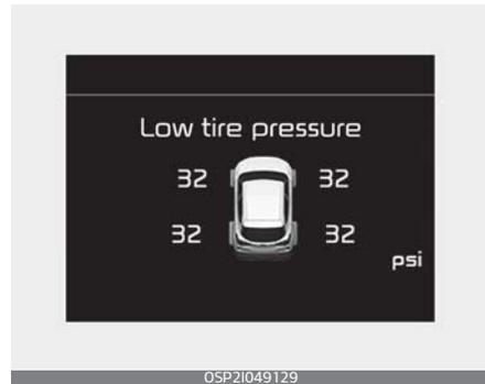
The low tire pressure position telltale light will indicate which tire is significantly under-inflated by illuminating the corresponding position light.
