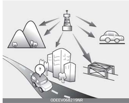
FM broadcasts are transmitted at high frequencies and do not bend to follow the earth's surface. Because of this, FM broadcasts generally begin to fade within short distances from the station. Also, FM signals are easily affected by buildings, mountains, and obstructions. This can lead to undesirable or unpleasant listening conditions which might lead you to believe a problem exists with your radio.
