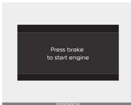
When the shift lever is not placed in N (Neutral), the following pop-up will be displayed on the cluster
