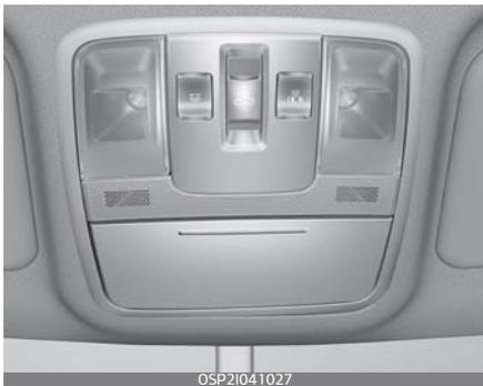
The sunroof can only be operated when the ignition switch or the ENGINE START/STOP button is in the ON position.
