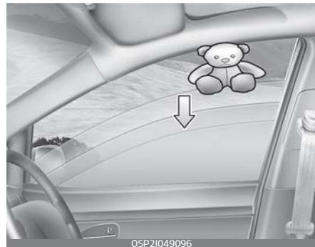
If the upward movement of the window is blocked by an object or part of the body, the window will detect the resistance and will stop upward movement. The window will then lower approximately 30 cm
