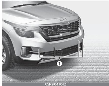
The sensing range and objects detectable by the sensors (1) are limited. Whenever moving while using Forward/Reverse Parking Dis-
