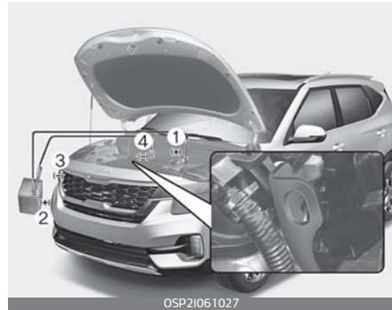
Jump starting can be dangerous if done incorrectly. Therefore, to avoid harm to yourself or damage to your vehicle or battery, follow the jump starting procedures. If in doubt, we strongly recommend that you have a competent technician or towing service jump start your vehicle.
