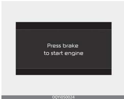
When the shift lever is not placed in N (Neutral), the following pop-up will be displayed on the cluster.
