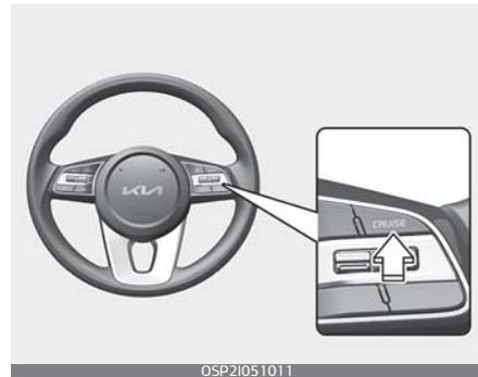
2. Accelerate to the desired speed, which must be more than 30 km/h.
