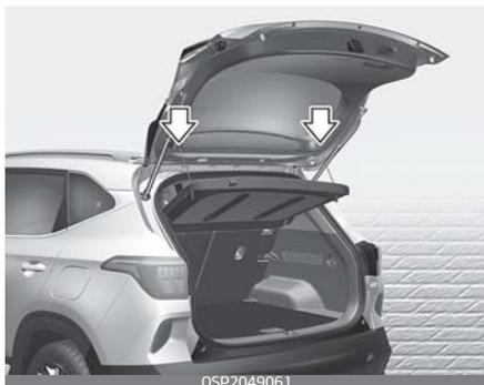
2. While lifting the cover up, hold the area near the front slots. Then, pull up the cover at approximately 45 ° angle.
