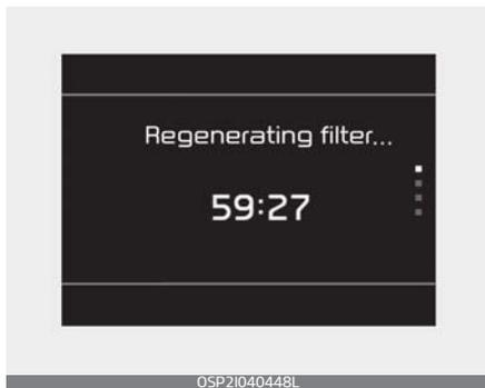
If the self regeneration mode starts, the message "Regenerating filter..." and the remaining time appears. It takes around 30~60 minutes.
