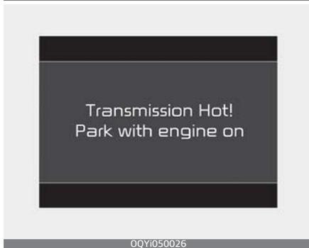
The following extreme cases may damage the clutch due to overheating while driving. Vehicle's own protection system sounds alarm and displays warning messages. Please shift into lower gear or stop the vehicle according to the instruction.
