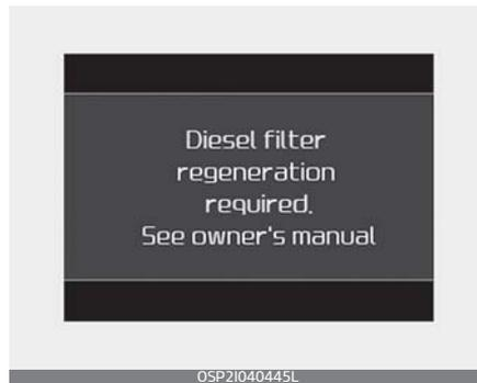
If the system still needs the self regeneration process after canceling the operation, the warning message appears. (Diesel filter regeneration required.) If the driver press the OK button firmly, it can
