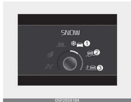
If you press the "DRIVE/TRACTION" mode button, the driving mode is changed from Driving control to Traction control. You can select SNOW (1), MUD (2) or SAND (3) mode by rotation the knob. If you press the "DRIVE/TRACTION" mode button again, the driving mode is changed from Traction Control to previous driving control.
