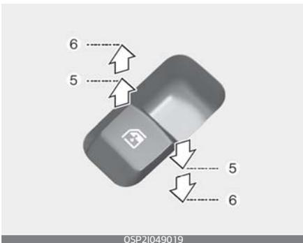
Pressing or pulling up the power window switch momentarily to the
