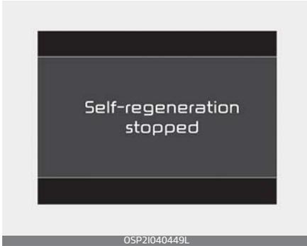
The self regeneration process stops if any of the self regeneration conditions is cancelled. If the self regeneration process is cancelled automatically, the system maintains "Self-regeneration stopped" message. If the driver presses the OK button firmly, it can restart the self regeneration mode again. (Self regeneration conditions should be satisfied.)
