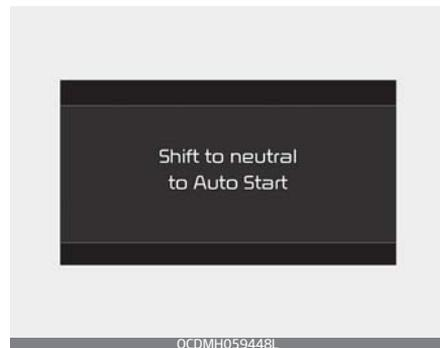
**Automatic Transmission / Dual clutch transmission** - Place the transmission shift lever in P (Park). Depress the brake pedal fully.
