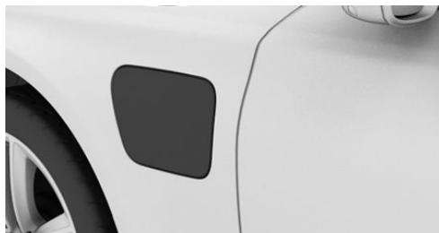
The charging socket flap is located in front on the left side of the vehicle.
