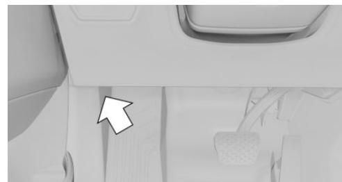
On the left side of the vehicle, there is a diagnostic socket for reading out vehicle data.
