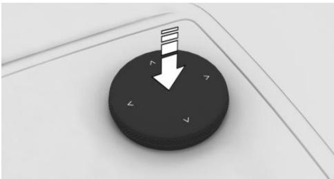
▷ Slide the Controller in four directions to switch between menus, for example.
