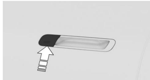
Hold the smartphone NFC antenna directly at the center of the driver's door handle. The po-
