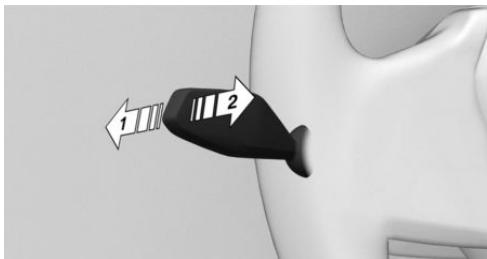
To reactivate the High Beam Assistant, press the turn signal lever up, arrow 1.
