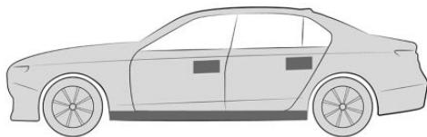
The ultrasonic sensors for the automatic doors are located near the door handles and below the door opening in the sill.
