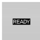
When the drive-ready state is switched on, READY is displayed in the instrument cluster.
