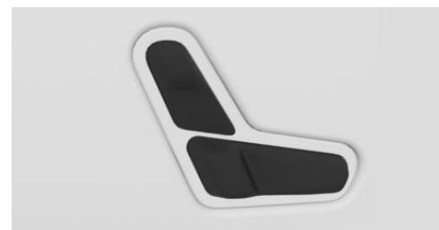
The switches for the seat settings are located at the front doors.
