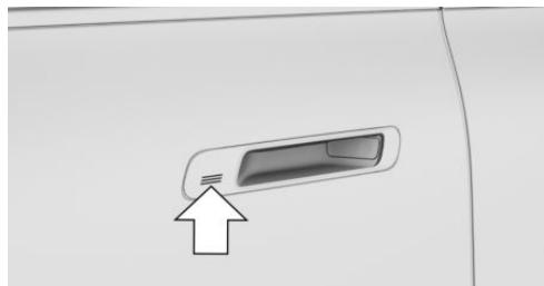
Touch the grooved surface on the door handle of a closed front door with your finger and hold it there without grasping the recessed grip.
