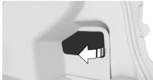
2. Pull the green button with the fuel pump icon. This silently releases the fuel filler flap.
