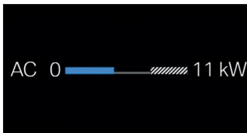
The shaded area indicates a limitation in the charging capacity that can occur, for instance due to the connected charging infrastructure.
