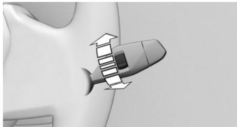
Turn the thumbwheel on the wiper lever.
