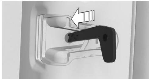
6. Pull the door handles to make sure they are locked. If necessary, repeat the process.
