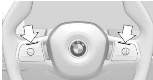
Similar to the instrument cluster views, the two LEDs above the keypads illuminate.
