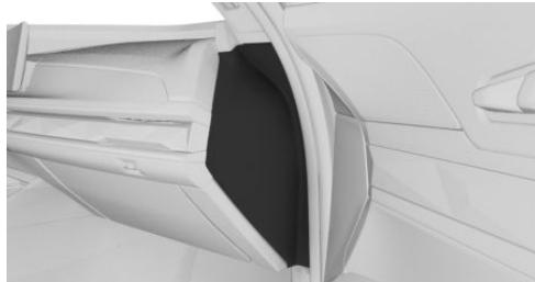
3. Press the sound insulation downward or remove it.
