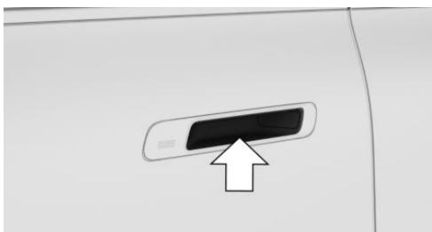
Reach into the recessed grip of the door and pull the door outward.
