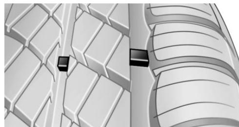
The tire manufacturer's wear indicators are distributed around the tire circumference and have a height of at least 0.06 in/1.6 mm.
