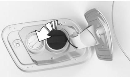
3. Place the fuel filler cap in the bracket on the fuel filler flap.
