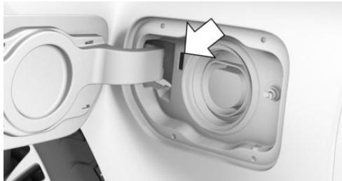
The charging status is shown by the indicator light on the high-voltage charging socket.
