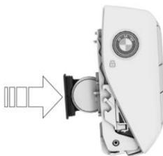
6. Insert the cover into the vehicle key.
