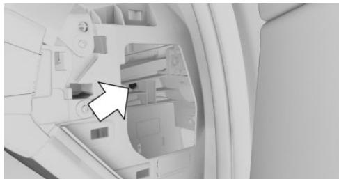
5. Pull the object out of the opening again. The glove compartment opens.
