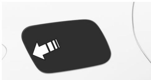
2. Open the fuel filler cap counterclockwise.
