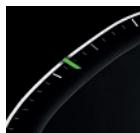
A mark for the set speed appears on the speedometer.
