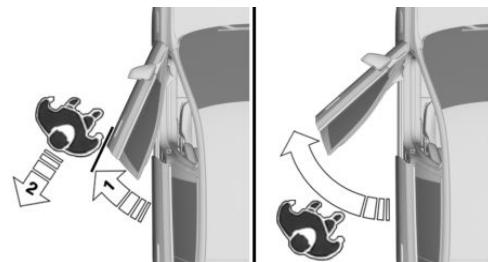
If the person opening the door is detected as an obstacle, the door stops, arrow 1. If the door's travel path is exited immediately, arrow 2, the door continues to move.
