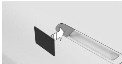
Hold the activated Service Card directly over the middle of the driver's door handle.
