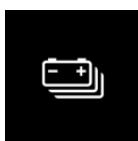
If this icon is displayed, the electric drive is not available because the high-voltage battery is too cold or too warm. A Check Control message is displayed where applicable.
