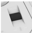
Push the volume button on the center console. The control display and the instrument cluster illuminate.
