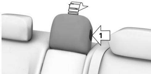
Press button, arrow 1, and fold the head restraint back.
