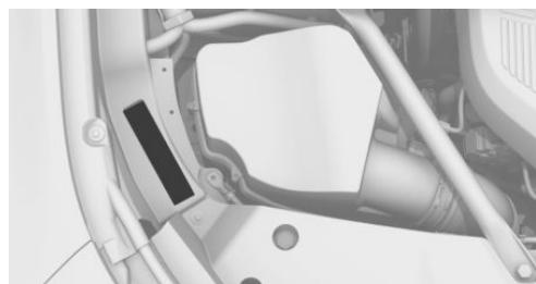
The engraved vehicle identification number can be found in the engine compartment, on the right-hand side of the vehicle.
