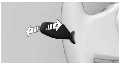
Press the turn signal lever forward, arrow 1, or pull the turn signal lever backward when the high-beam headlights are switched on, arrow 2.
