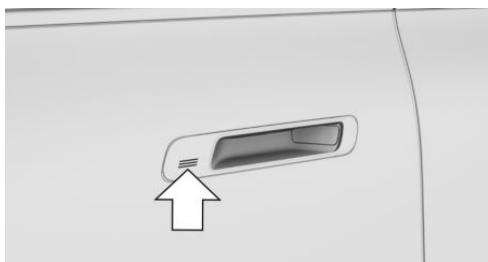
Touch the grooved surface on the door handle of a closed front door with your finger and hold it there without grasping the recessed grip.
