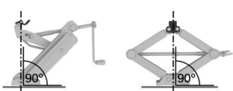
6. Crank the vehicle up until the entire jack surface is on the ground and the corresponding wheel is lifted max. 1.2 inches/3 cm above the ground.
