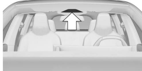
The camera behind the windshield is located near the interior mirror.
