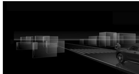
Example of anticipatory hybrid drive before reaching an urban area: The electric drive is prepared. The vehicle switches automatically to electric drive upon reaching an urban area.
