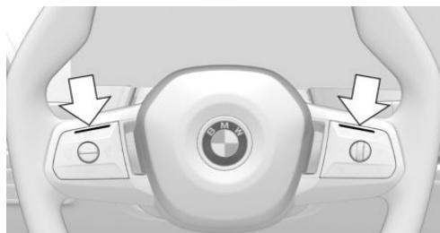
The two LEDs above the keypads illuminate depending on the situation.
