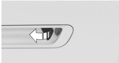
8. Press the central locking button to unlock the other doors.
