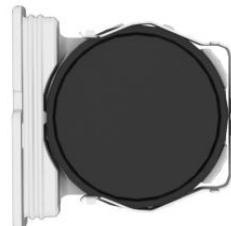
4. Insert a CR2032 3V battery with the positive side facing down.
