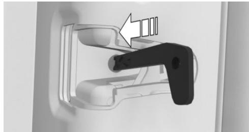
2. Pull the door handles to make sure they are locked. If necessary, repeat the process.
