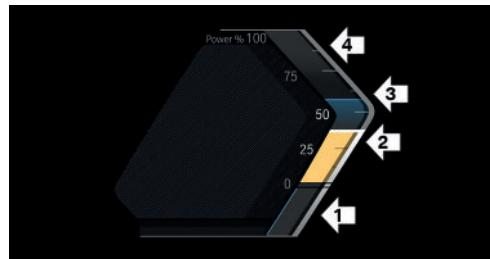
Needle near arrow 1: indicator for energy recovery, e.g., while decelerating.
