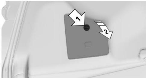
Turn the twist lock in the cover by 90°, arrow 1, and fold down the trim panel, arrow 2.
