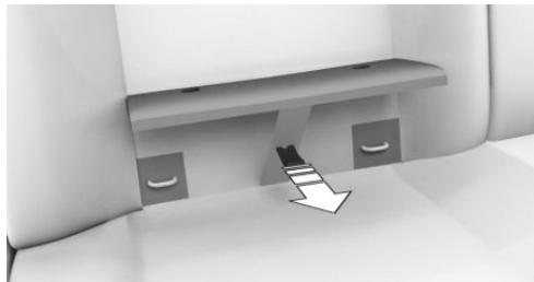
To close the cover, pull the loop forward and release.
