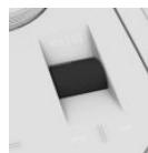
Press and hold the volume button on the center console until all displays go out.
