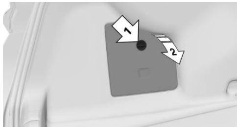
The onboard vehicle tool kit is located in the left storage compartment of the cargo area. Turn the cover lock, arrow 1, and fold out the trim panel, arrow 2.
