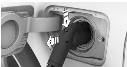
3. Disconnect the charging cable from the high-voltage charging socket, arrow 2.
