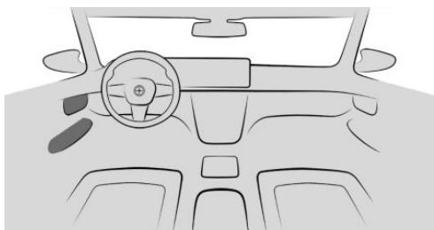
The seat adjustment menu button is located on the front door.
