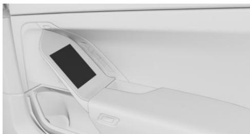
The rear air conditioning system is operated via BMW Touch Command.
