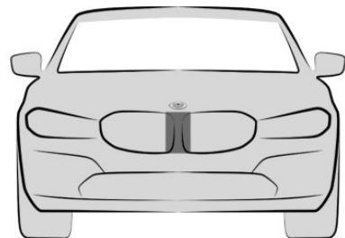
The front camera is located in the radiator grille.
