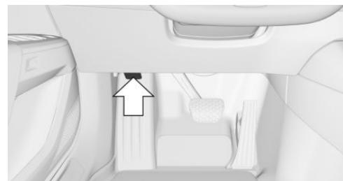
The unlock lever for the hood is located in the driver's footwell.
