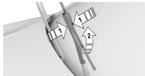
4. Remove the wiper blade forward from the detent.
