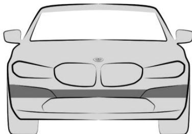
The ultrasonic sensors are located in the front bumper.
