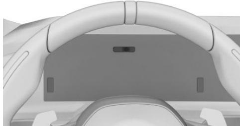
Depending on vehicle equipment, the instrument cluster has one or more infrared light sources. Depending on the light conditions, these light sources can be visible when the vehicle is in standby mode.
