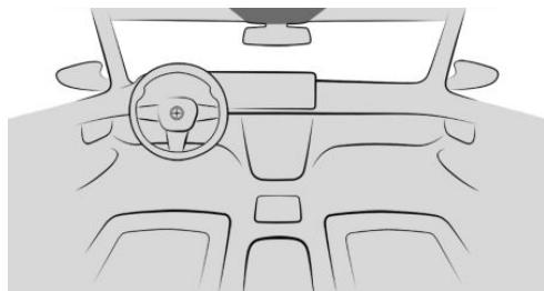
The interior camera is located on the headliner.
