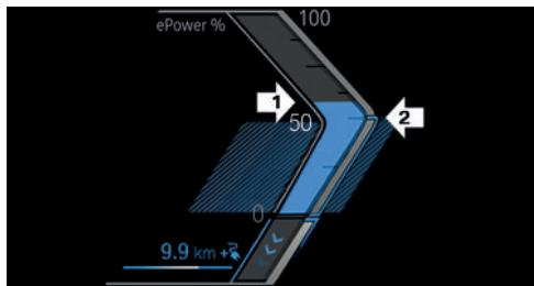
A blue range appears on the power gauge, indicating reduced consumption while driving. Additionally, the bonus range will be displayed. If the blue range turns gray, the fuel consumption has increased.
