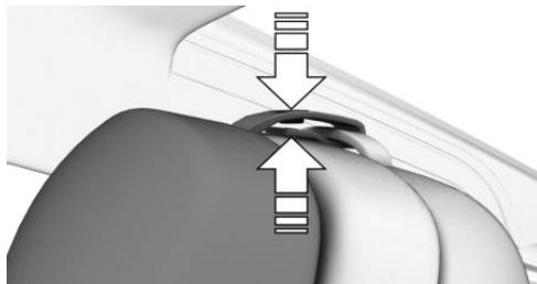
3. The head restraint folds into the topmost position.
