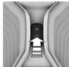
Press the switch up and hold it until initialization is complete.
