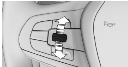
Press the rocker switch up or down once while the system is interrupted.
