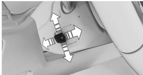
Move the steering wheel to the preferred height and angle to suit your seating position by pressing the switch.
