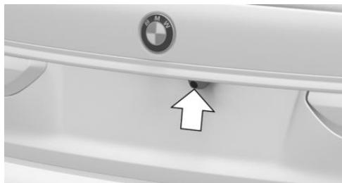
The camera lens is located in the handle of the trunk lid.
