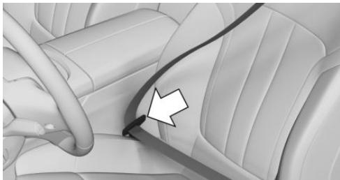
When the safety belt is fastened, the driver's and passenger's belt straps are automatically tightened once after driving away.
