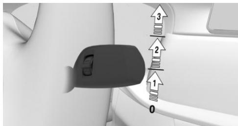
Press the lever up once from its standard position, arrow 1.
