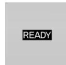
The display in the tachometer indicates that the Auto Start/Stop function is ready for an Automatic engine start.
