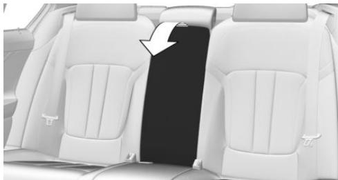
Reach into the recess and fold the center armrest forward.
