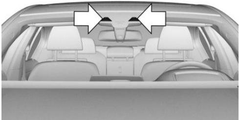
The camera is installed near the interior mirror.
