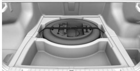
The emergency wheel and the wheel change tools are located in the cargo area under the cargo floor panel.
