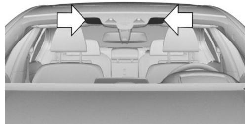
The marked area is not covered with heat reflective coating.
