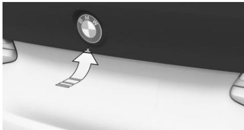
Press the button on the exterior of the trunk lid. This corresponds with pressing the button
