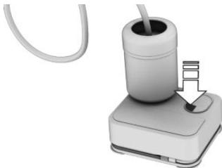
Let the compressor run for max. 10 minutes to fill the tire with sealant and achieve a tire inflation pressure of approx. 2.0 bar.
