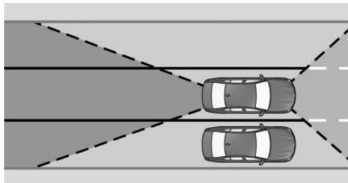
Four radar sensors in the bumpers monitor the area next to the vehicle in the speed range from approx. 45 mph/70 km/h to approx. 130 mph/210 km/h.
