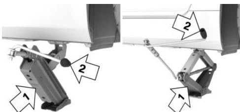
2. Insert the vehicle jack into the rectangular recess of the jacking point closest to the wheel to be changed.
