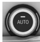
Turn the ring to set the desired temperature.
