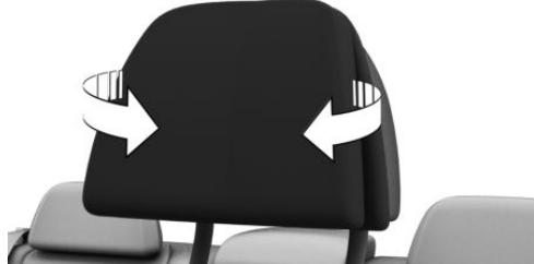
Fold the side extensions on the head restraint forward for increased lateral support in the resting position.
