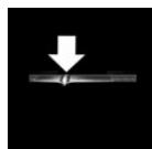
The mark in the consumption display below the tachometer is located at the zero point and is backlit in blue. The tachometer approximately indicates idle speed.
