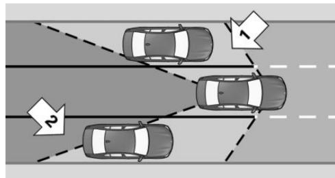
Two radar sensors in the rear bumper monitor the area behind and next to the vehicle when traveling faster than a minimum speed.
