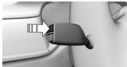
Press and hold the button on the turn signal lever.
