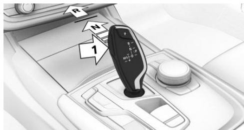
4. Release Start/Stop button and selector lever.
