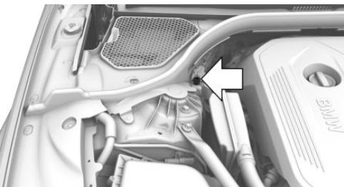
The starting aid terminal in the engine compartment acts as the battery's positive terminal.
