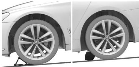
If you need to change a wheel on a slight downhill grade, place chocks and other suitable objects, for instance a rock, under the wheels of both the front and rear axles against the rolling direction.
