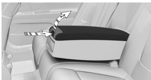
Press the button, arrow 1, and fold the cover up, arrow 2.
