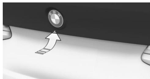
► Unlock the vehicle and then press the button on the outside of the trunk lid.
