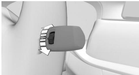
Turn the thumbwheel on the wiper lever.
