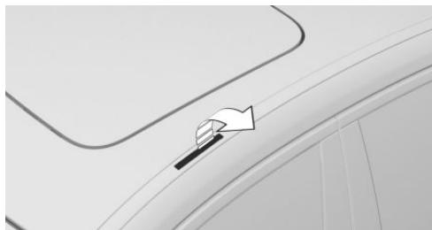
The fixing points are located in the roof drip rail above the doors.
