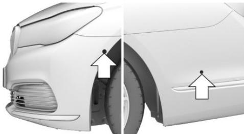
With the four side ultrasound sensors, arrows, and the ultrasound sensors of PDC Park Distance Control in the bumpers, the parking spaces are measured and the distances to obstacles determined.
