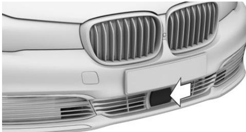
The radar sensor is located in the front bumper. Always keep radar sensor clean and unobstructed.
