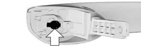
3. Use the thumb of the hand on the door handle to push the cover toward the rear of the vehicle.
