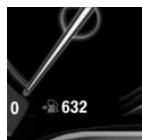
The current range is displayed as numerical value at the bottom of the speedometer.
