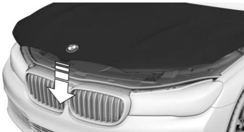
Let the hood drop from a height of approx. 16 inches/40 cm and push down on it to lock it fully.
