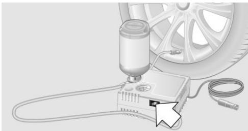
**⚠** Switch off the compressor after 10 minutes
