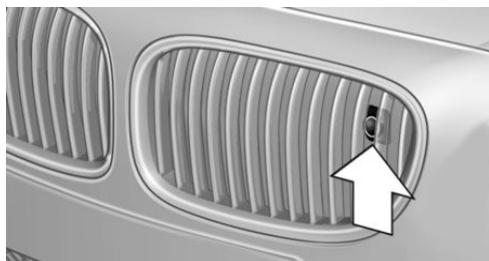
The camera is automatically heated when the external temperatures are low.
