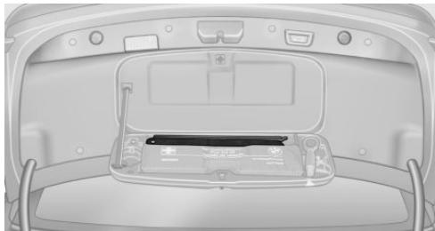
The warning triangle is located in the container on the inside of the trunk lid.
