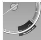
The kinetic energy of the vehicle is converted to electrical energy while coasting. The vehicle battery is partially charged and fuel consumption can be reduced.
