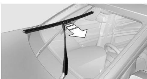
5. Insert the new wiper blade in reverse order of removal until it locks in place.
