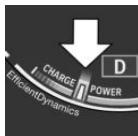
The mark in the efficiency display below the tachometer is backlit in blue and is located at the zero point. The tachometer approximately indicates idle speed.
