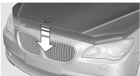
Let the hood drop from a height of approx. 16 in/40 cm and push down on it to lock it fully.
