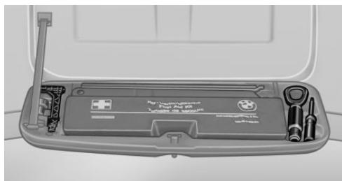
The onboard vehicle tool kit is located in a fold-down cover in the trunk lid.
