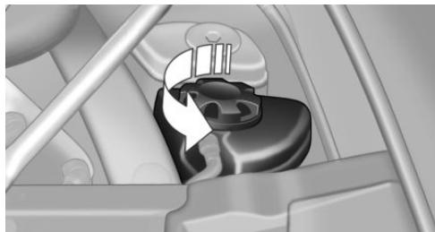
3. If the coolant is low, slowly add coolant up to the specified level; do not overfill.
