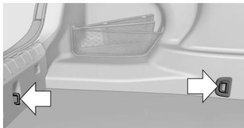
To secure the cargo there are four lashing eyes in the cargo area.
