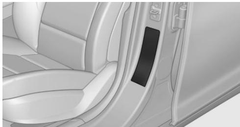
These pressure values can also be found on the tire inflation pressure label on the driver's door pillar.
