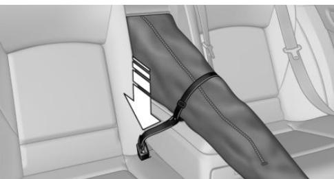
6. Tighten the retaining strap.
