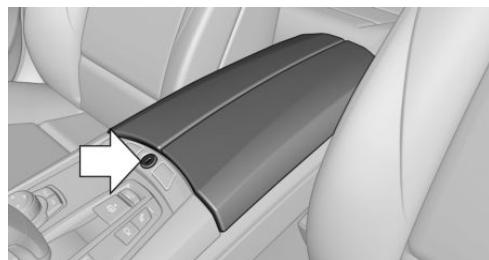
The storage compartment in the armrest can be locked with an integrated key to separately secure the trunk lid, refer to page 43, e.g.
