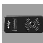
An external audio device, e.g., an MP3 player, can be connected via the AUX-IN port or the USB audio interface in the center armrest.
