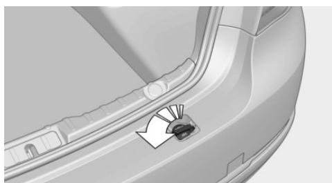
The tank lid for the reducing agent is located in the rear bumper under a cover.
