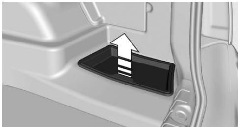
Under the cover on the side of the cargo area is a storage compartment that can be used to store the printed Owner's Manual, e.g.
