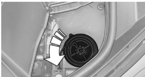
3. Pull the connector off the bulb.
