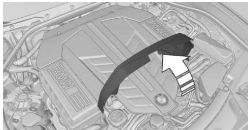
When the flap is closed, it must latch.
