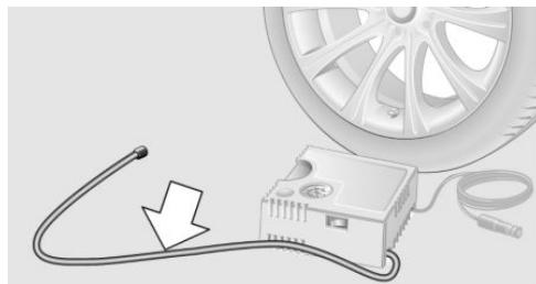
3. Screw the connection hose onto the connector of the sealant container.
