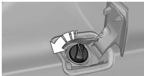
3. Place the tank lid in the bracket attached to the fuel filler flap.
