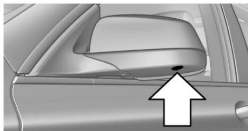
The lenses of the Top View camera are located at the bottom in the mirror housings. The image quality may be impaired by dirt.
