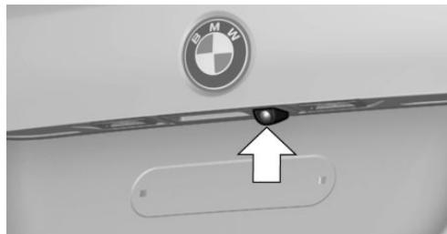
The camera lens is located in the handle of the tail gate. The image quality may be impaired by dirt.
