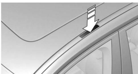
On the roof drip rail, press on the outside of the flap.
