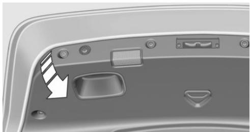
3. Replace the defective bulb.
