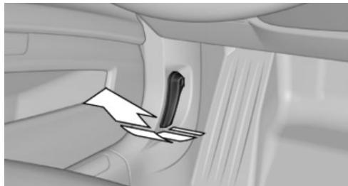
2. Press the release handle and open the hood.
