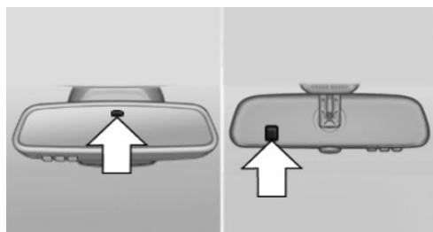
Photocells are used for control:
