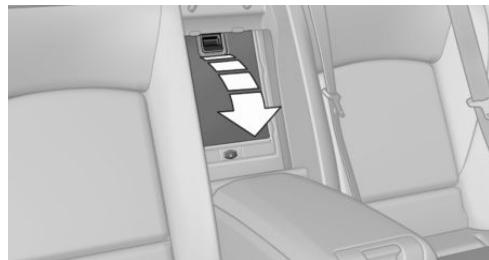
Pull on the opener and fold the cooler forward.
