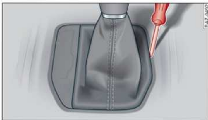
Fig. 76 Selector lever: Removing the boot
