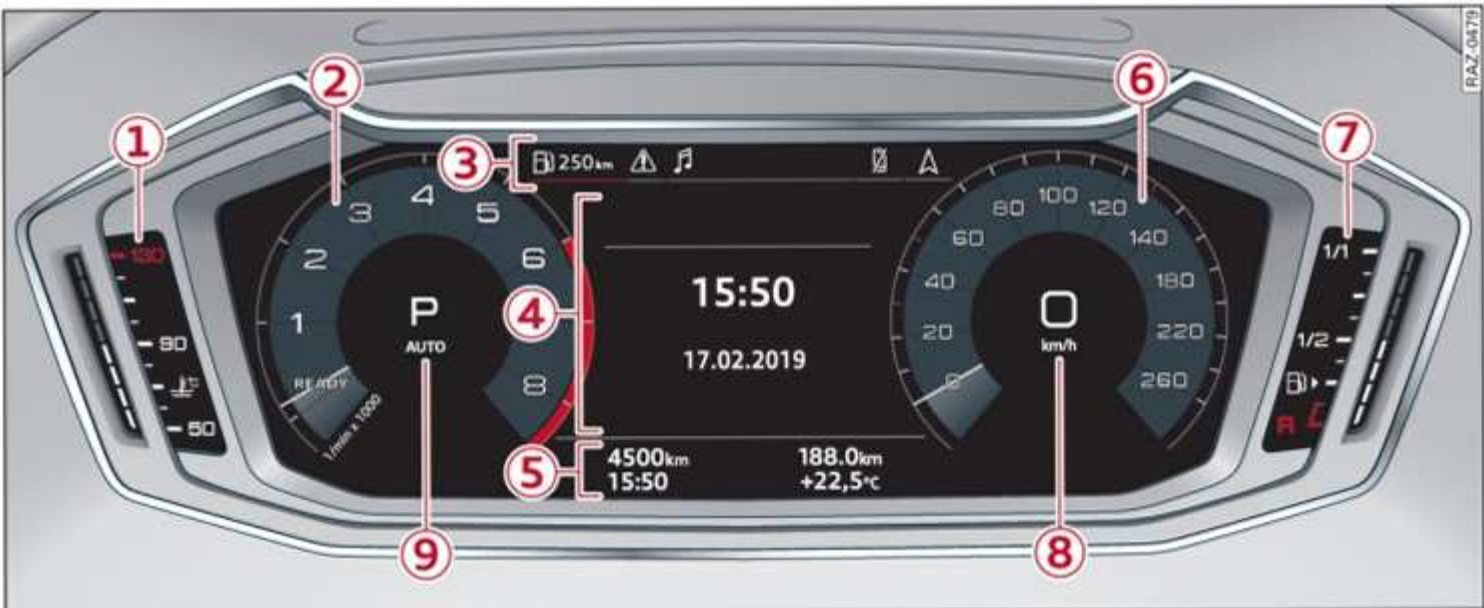
Fig. 3 Overview of digital instrument cluster / Audi virtual cockpit
