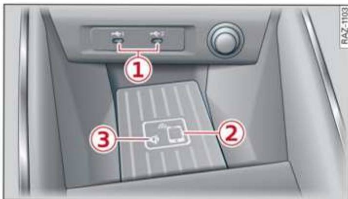
Fig. 114 Front centre console: Audi phone box with connections
