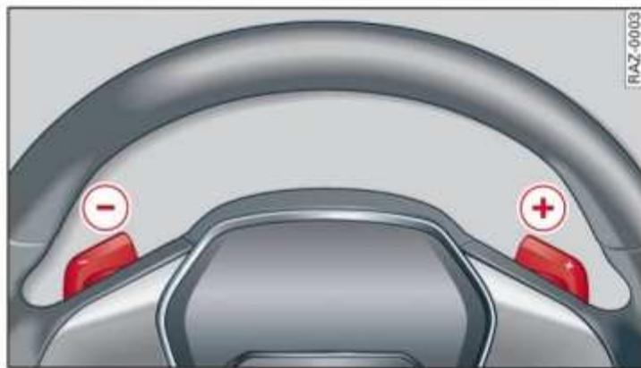
Fig. 75 Steering wheel: Paddle levers*
