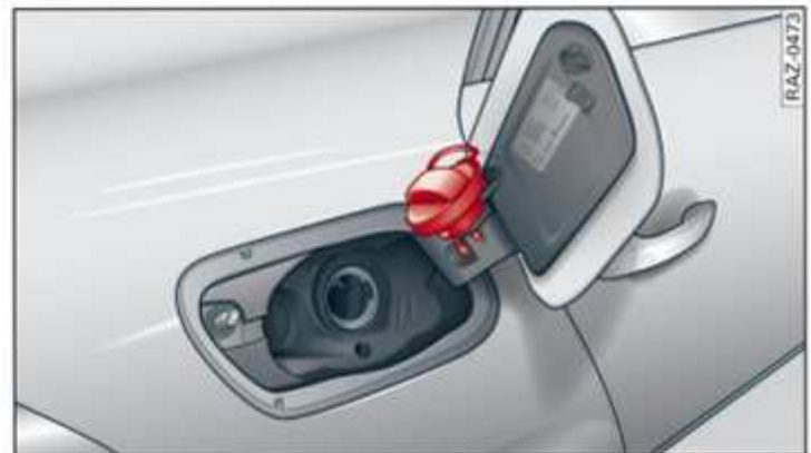
Fig. 134 Fuel tank flap with tank cap attached
