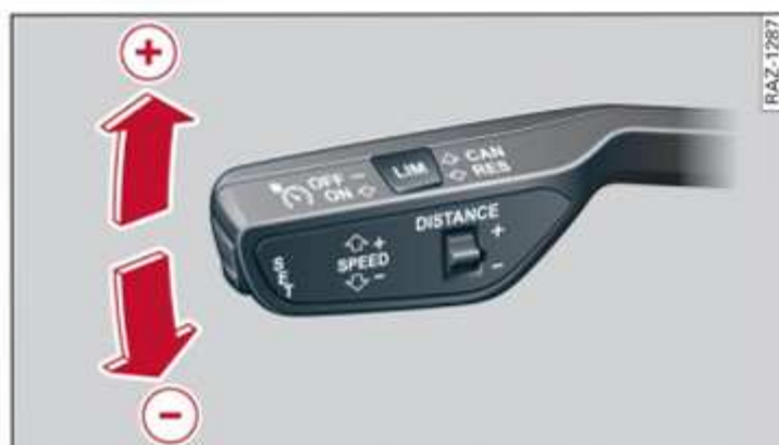
Fig. 93 Control lever: Setting a new speed
