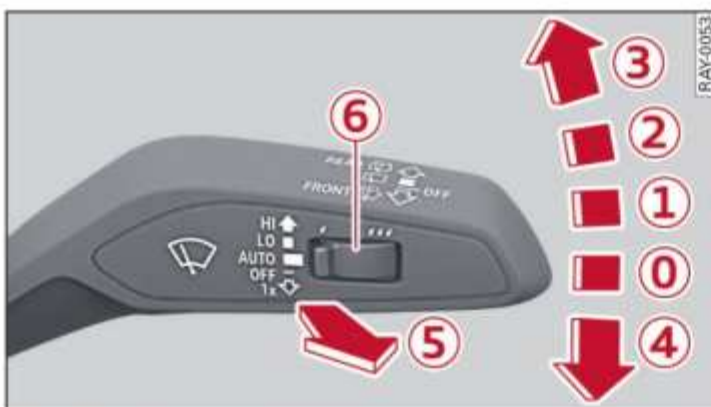
Fig. 39 Control lever: Windscreen wipers
