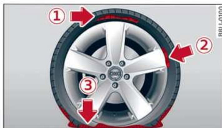
Fig. 150 Tyres: Irreparable tyre damage
