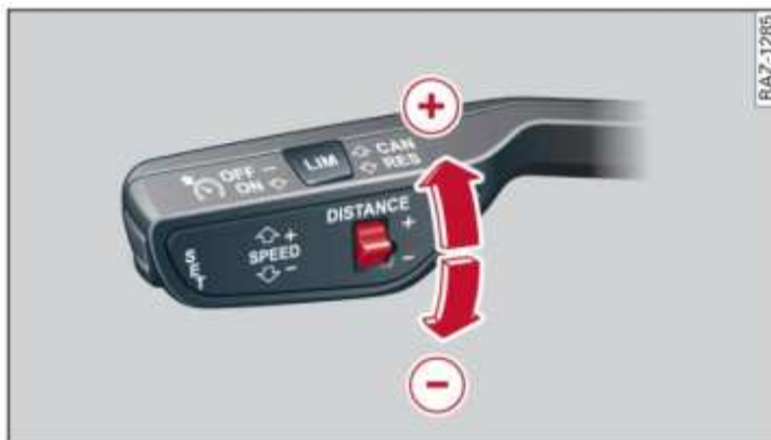
Fig. 96 Control lever: Setting the distance
