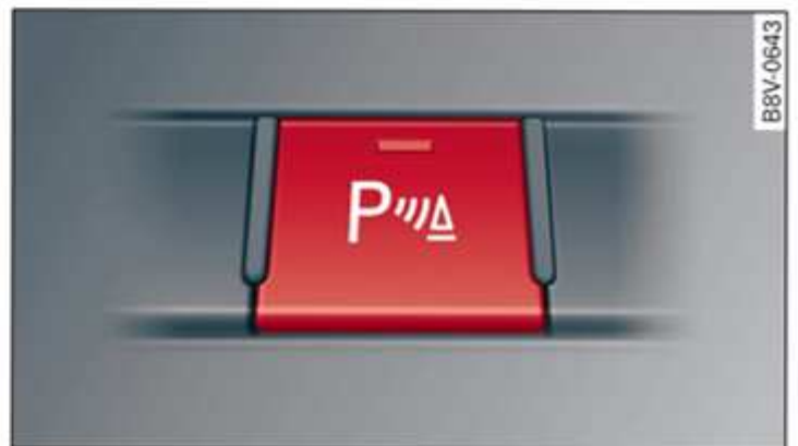
Fig. 107 Centre console: Button for parking aid
