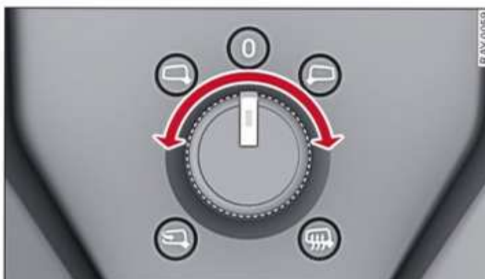
Fig. 37 Driver's door: Adjuster knob for exterior mirrors
