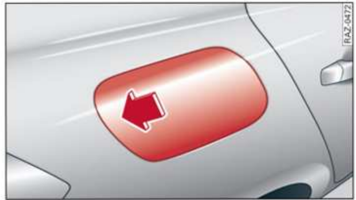
Fig. 133 Vehicle as seen from the rear right: Opening fuel tank flap
