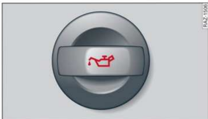
Fig. 140 Engine compartment: Engine oil filler cap (example)
