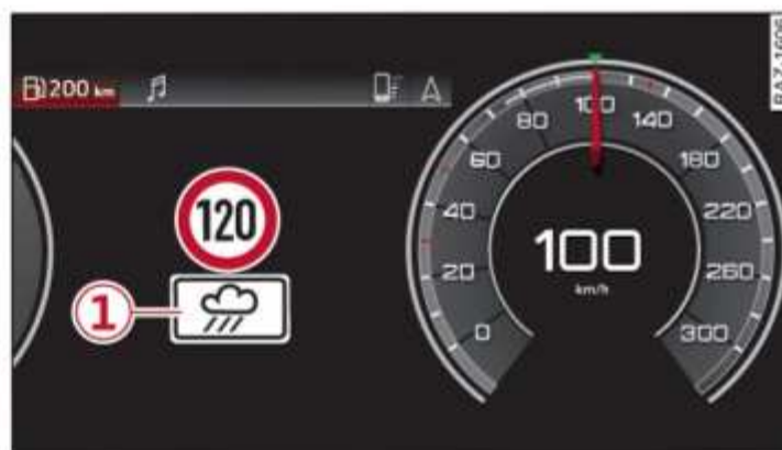
Fig. 85 Instrument cluster: Traffic sign recognition
