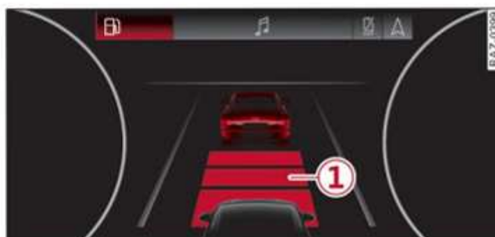
Fig. 95 Instrument cluster: Take over braking prompt
