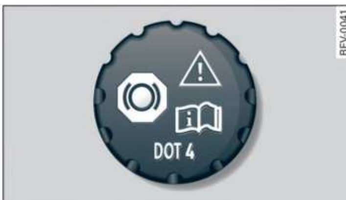
Fig. 142 Engine compartment: Cap of brake fluid reservoir
