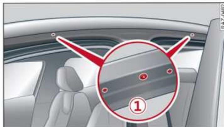
Fig. 68 Roof: Attachment points
