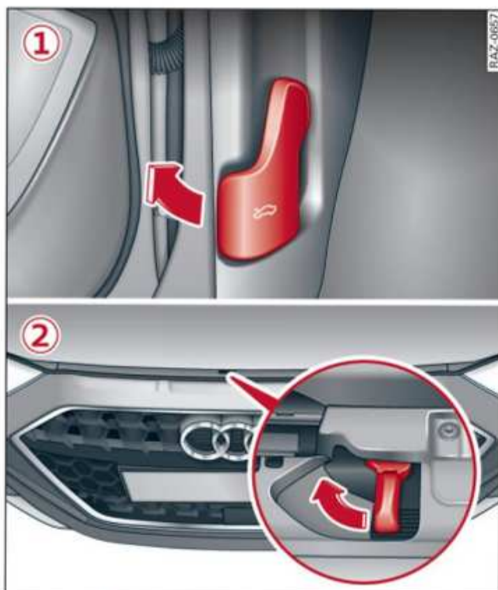
Fig. 135 ① Footwell: Release lever. ② Engine compartment: Lever for releasing bonnet
