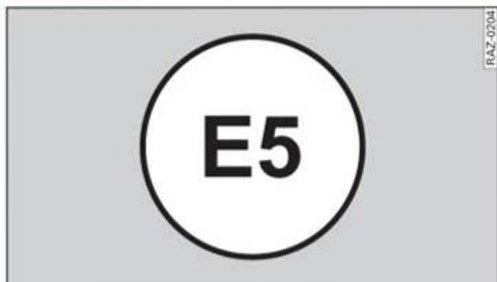
Fig. 132 Tank flap sticker: Identification of fuels (examples)
