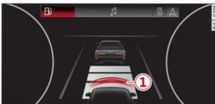
Applies to: vehicles with safe start monitor Fig. 98 Instrument cluster: Safe start monitor
