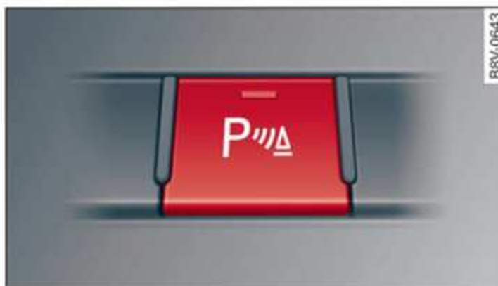
Fig. 84 Centre console: Button for parking aid
