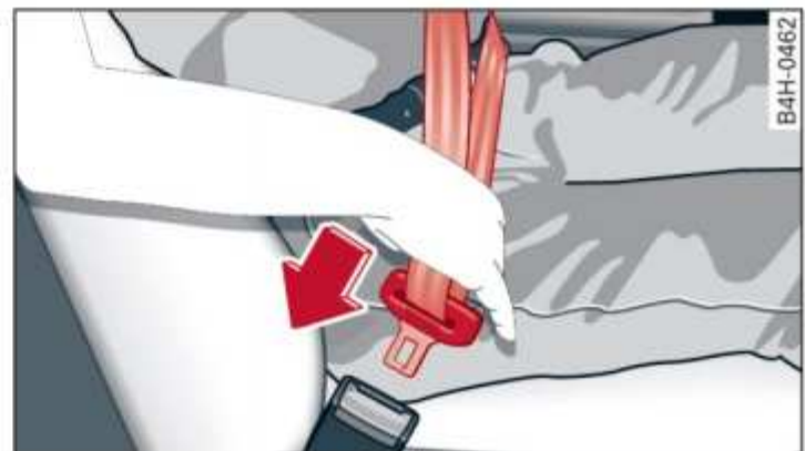
Fig. 50 Latch plate and buckle
