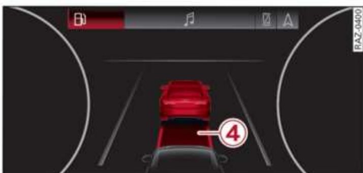
Fig. 100 Instrument cluster: Distance warning
