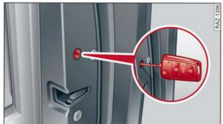
Fig. 23 Door: Locking the door manually
