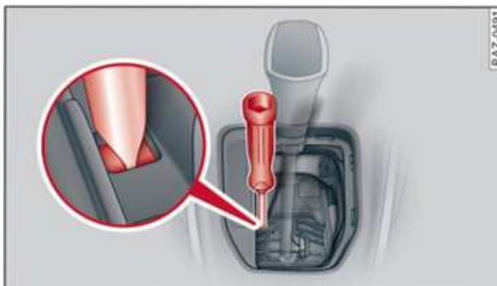
Fig. 77 Manual release mechanism (bottom left)
