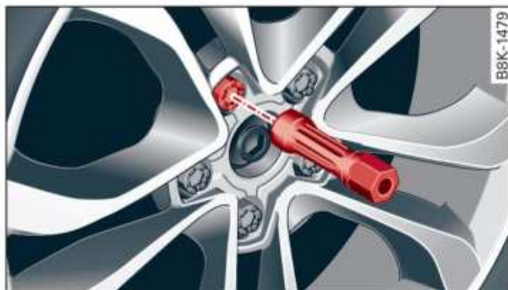
Fig. 157 Wheel: Hexagonal socket for turning wheel bolts
