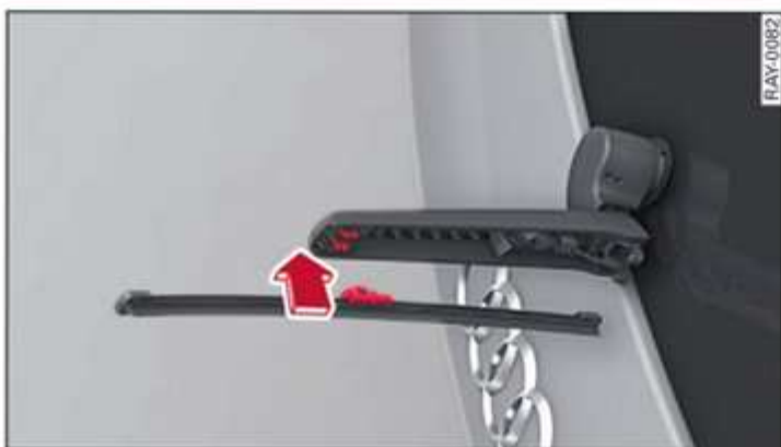
Fig. 42 Rear window wiper: Attaching the wiper blade
