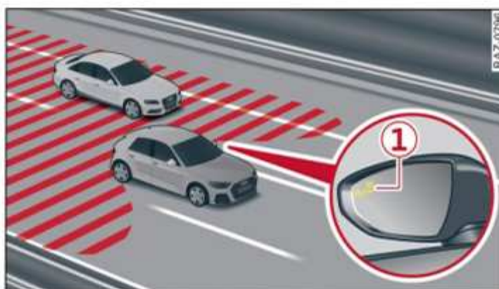
Fig. 103 Driving situation and warning signal on exterior mirror
