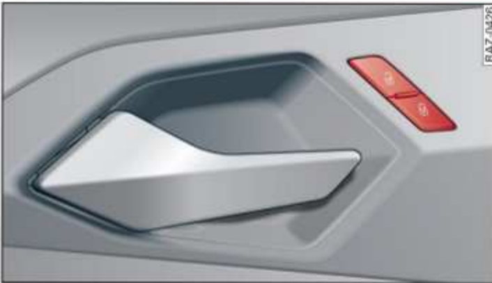
Fig. 21 Driver's door: Central locking switch
