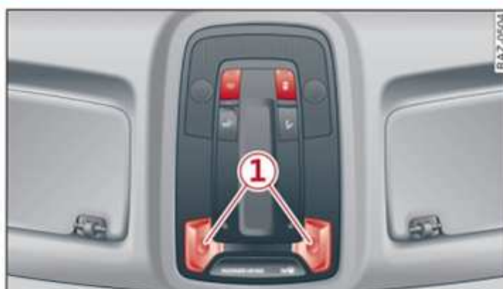
Fig. 35 Headliner: Interior lights
