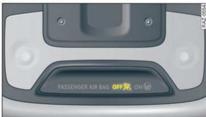
Fig. 55 Headliner: Indicator lamp for status of front passenger's airbag
