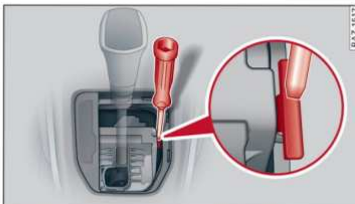
Fig. 78 Manual release mechanism (top right)
