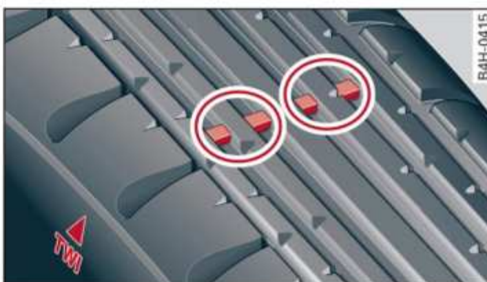
Fig. 146 Tyre tread: Tread wear indicators
