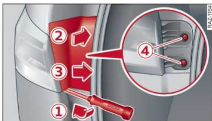
Fig. 175 Side panel: Removing cover
