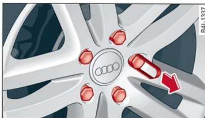
Fig. 152 Wheel: Wheel bolts with caps
