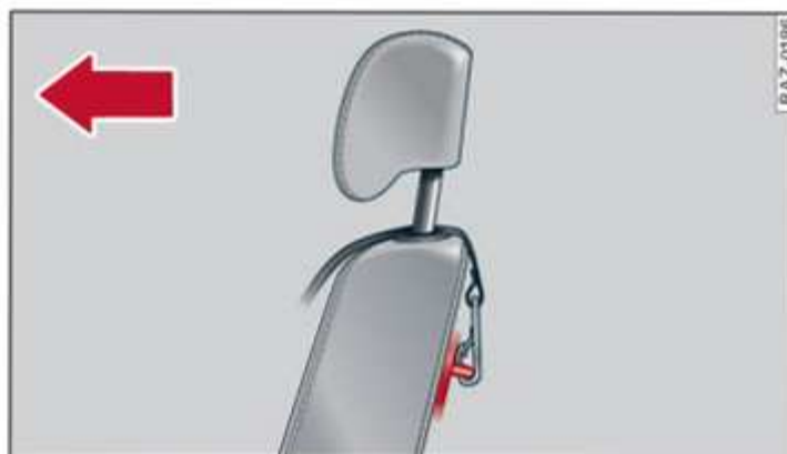
Fig. 59 Rear backrest: Hooking strap into top tether anchorage
