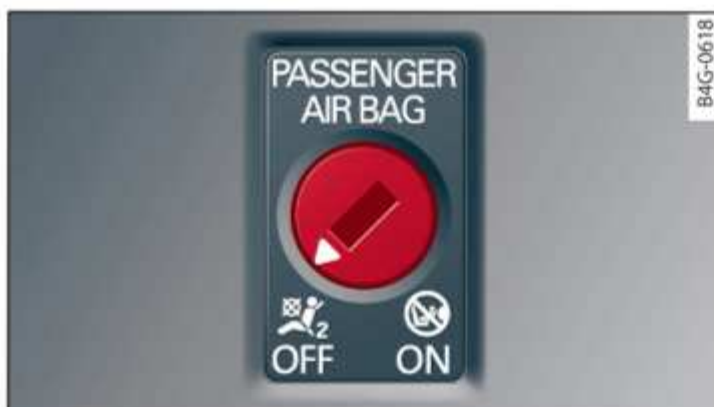
Fig. 54 Glove box: Key-operated switch for deactivating front passenger's airbag
