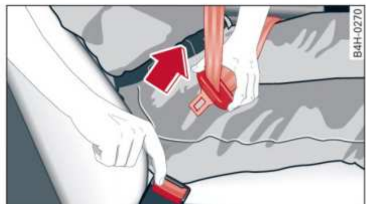
Fig. 51 The latch plate of the belt springs out of the buckle
