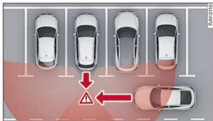
Fig. 109 Areas covered by sensors for rear cross-traffic assist
