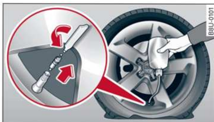
Fig. 151 Tyres: Filling the tyre
