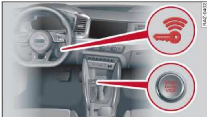
Fig. 71 Centre console: Starting the engine
