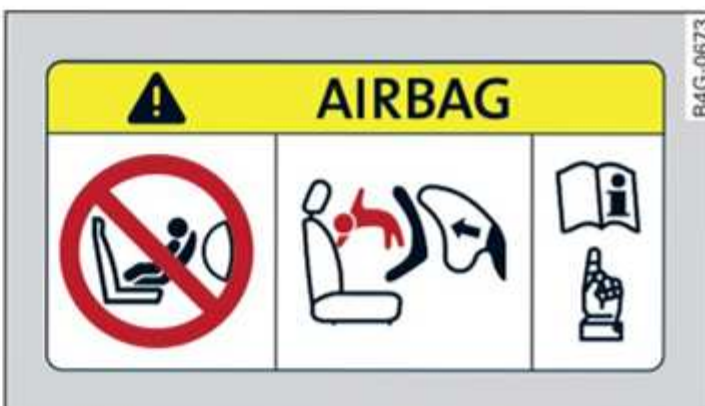
Fig. 56 Passenger's sun visor: Airbag sticker
