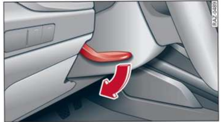
Fig. 44 Steering column: Lever for adjusting the steering wheel position
