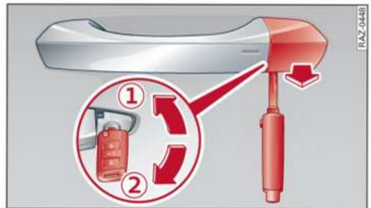
Fig. 22 Driver's door lock
