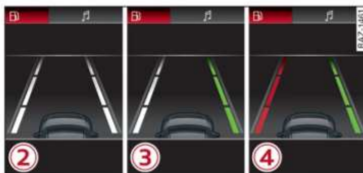
Fig. 101 Instrument cluster: Display showing driver assist system
