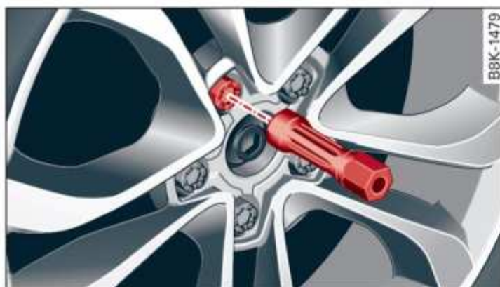
Fig. 155 Wheel: Hexagonal socket for turning wheel bolts
