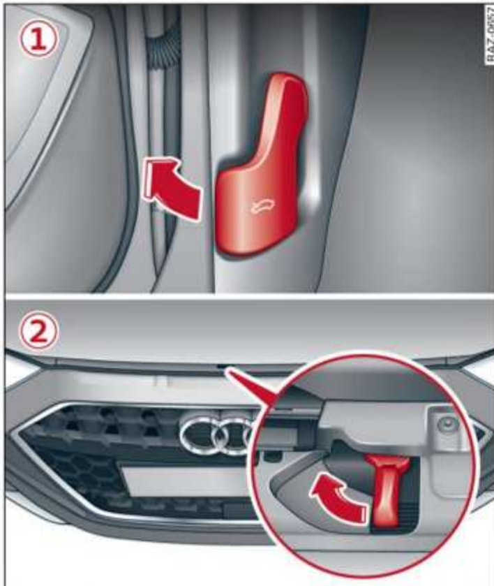
Fig. 133 ① Footwell: Release lever. ② Engine compartment: Lever for releasing bonnet
