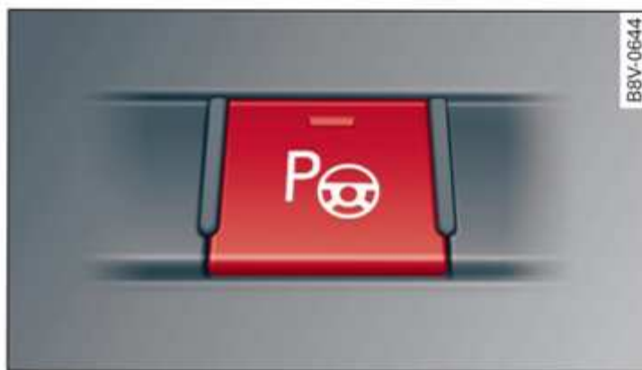
Fig. 111 Centre console: Button for park assist
