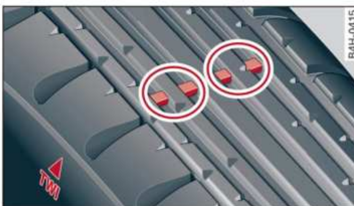
Fig. 144 Tyre tread: Tread wear indicators
