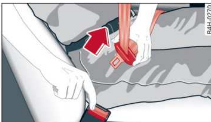
Fig. 51 The latch plate of the belt springs out of the buckle
