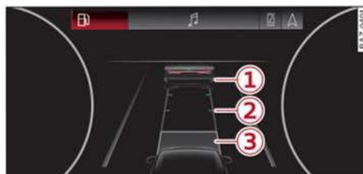
Fig. 98 Instrument cluster showing the current distance
