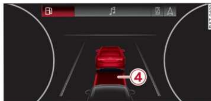
Fig. 99 Instrument cluster: Distance warning
