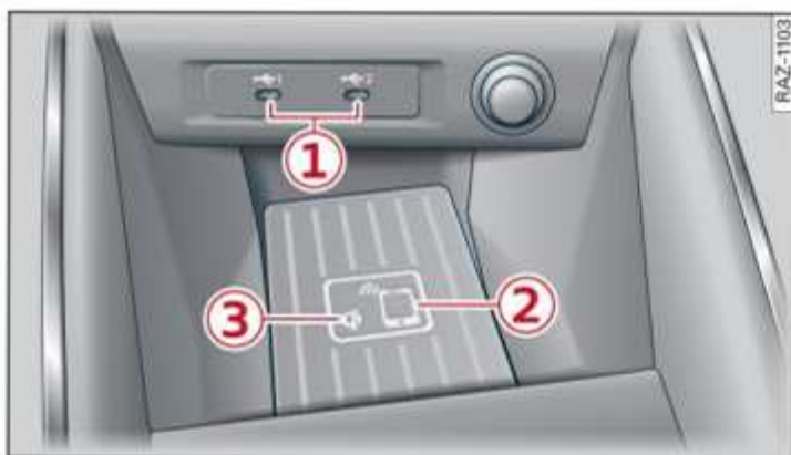
Fig. 113 Front centre console: Audi phone box with connections
