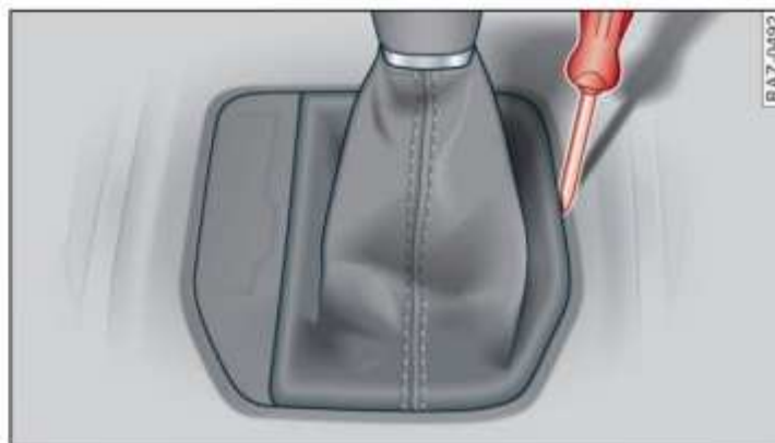
Fig. 76 Selector lever: Removing the boot
