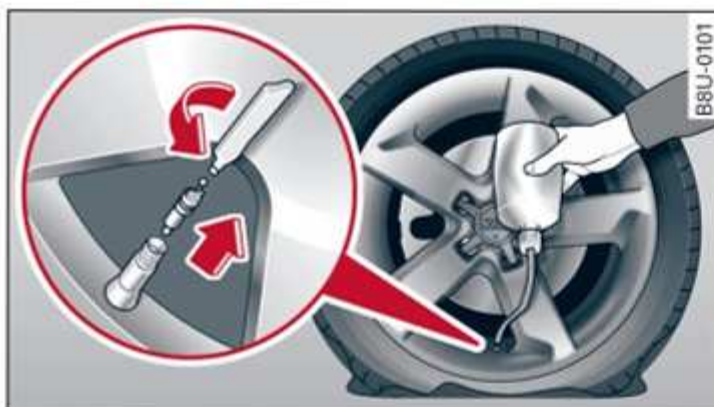
Fig. 149 Tyres: Filling the tyre
