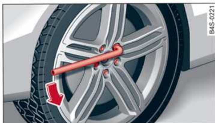
Fig. 152 Wheel: Loosening the wheel bolts
