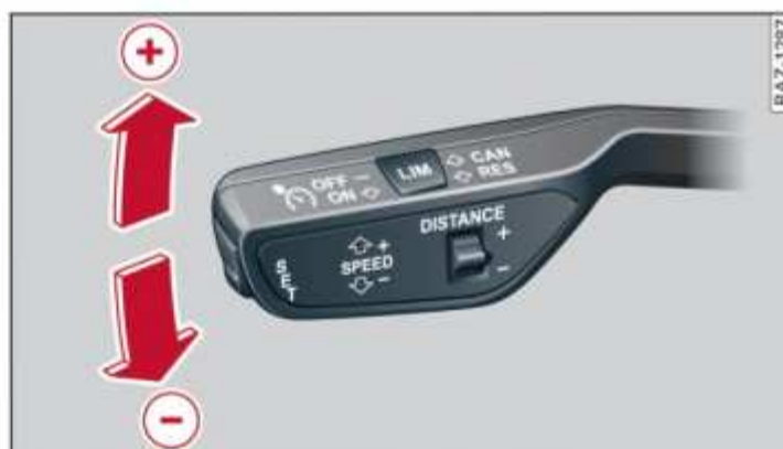
Fig. 92 Control lever: Setting a new speed
