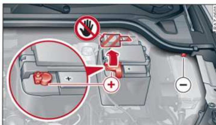
Fig. 141 Engine compartment with battery: Terminals for battery charger or jump leads
