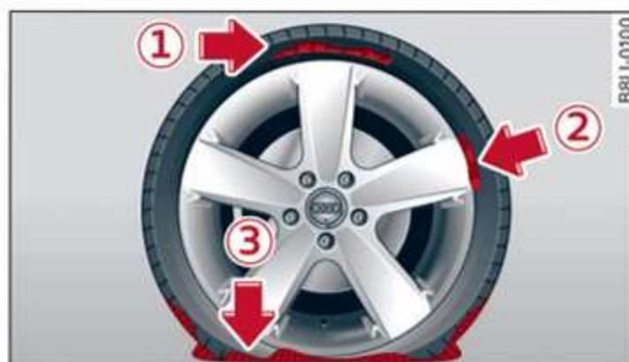
Fig. 148 Tyres: Irreparable tyre damage
