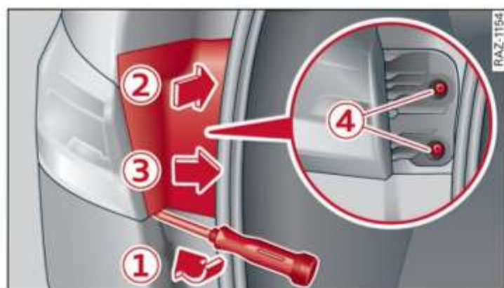
Fig. 173 Side panel: Removing cover
