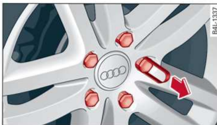
Fig. 150 Wheel: Wheel bolts with caps
