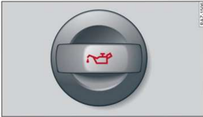
Fig. 138 Engine compartment: Engine oil filler cap (example)
