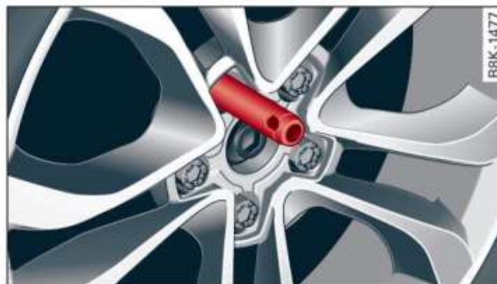
Fig. 156 Wheel: Mounting pin in wheel bolt hole nearest to the top
