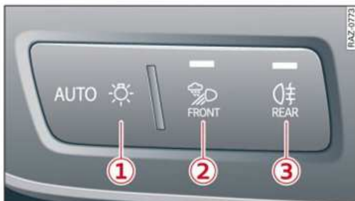
Fig. 32 Dashboard: Light switch module
