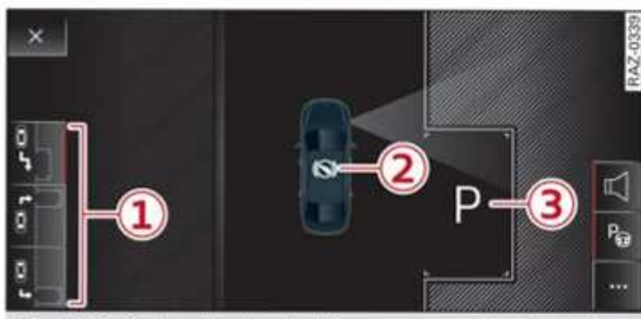
Fig. 112 Centre display: Parking space search activated
