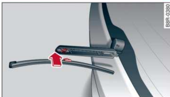
Fig. 42 Rear window wiper: Attaching the wiper blade
