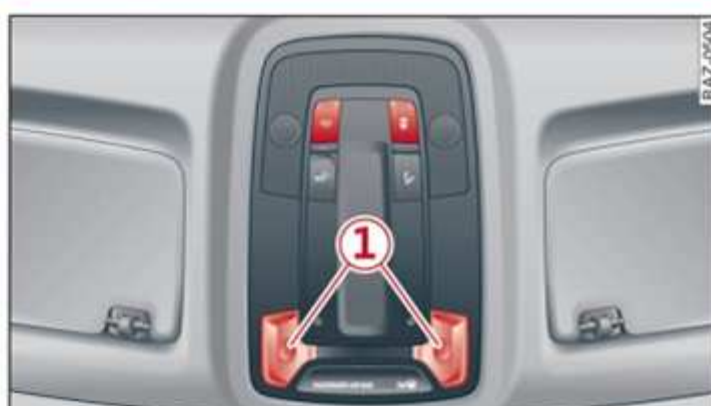
Fig. 35 Headliner: Interior lights
