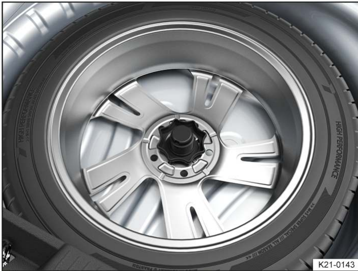
Fig. 1 Under the luggage compartment floor: handwheel for securing the spare wheel.
