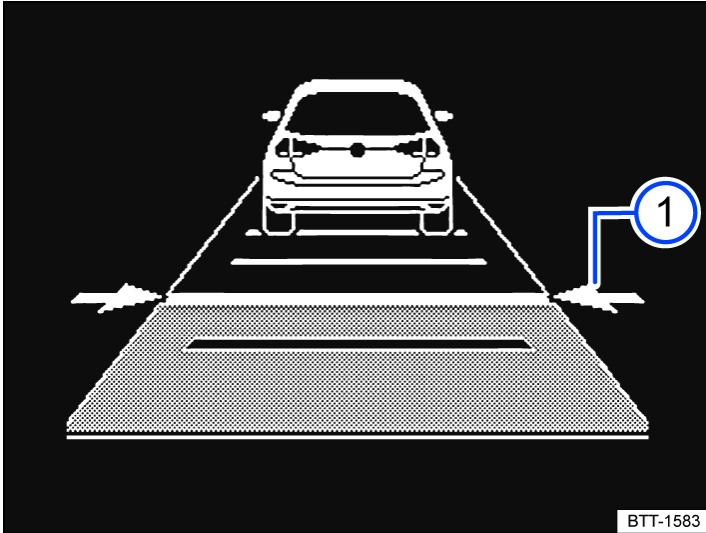
Fig. 1 On the instrument cluster display: set distance for control (illustration).
