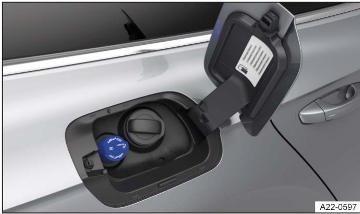
Fig. 1 Behind the tank flap: tank cap for AdBlue (illustration).
