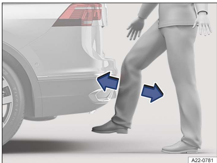
Fig. 1 Illustration of the boot lid with sensor-controlled opening (Easy Open).
