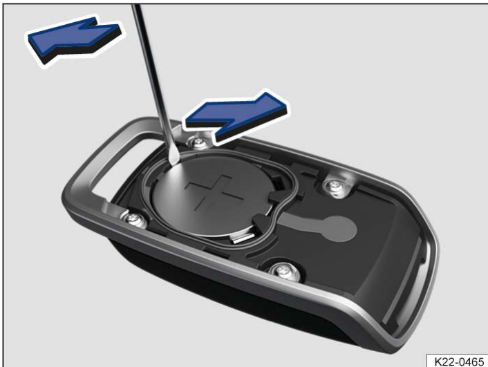
Fig. 2 Replacing the button cell in the remote control.
