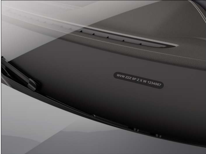
Fig. 1 In the windscreen: vehicle identification number.
