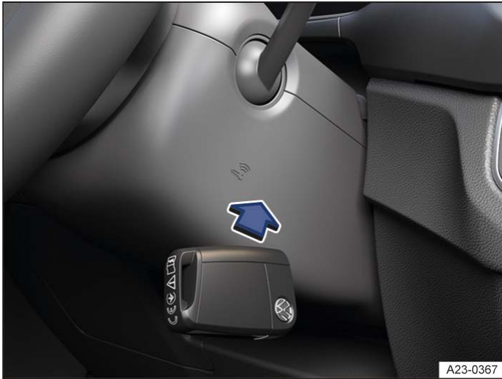
Fig. 1 On the right-hand side of the steering column: emergency start function in vehicles with the keyless locking and starting system Keyless Access (illustration).
