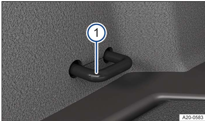
Fig. 1 In the luggage compartment: fastening ring (illustration).
