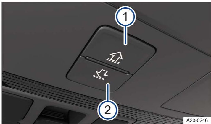
Fig. 1 In the roof: button for controlling the sun blind.
