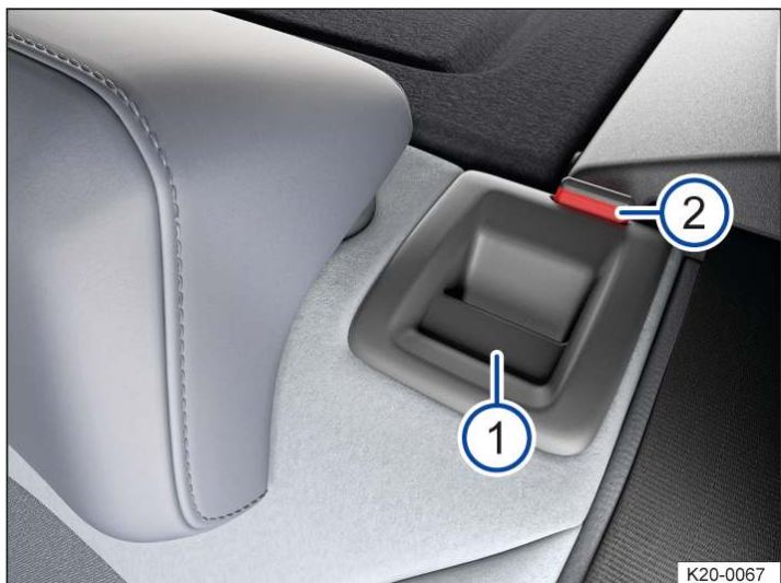
Fig. 2 In the rear seat backrest: release button.
