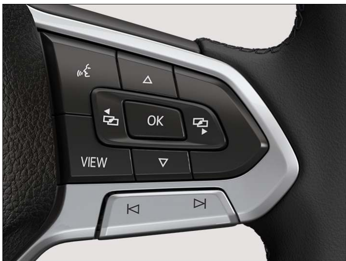
Fig. 1 Right side of the multifunction steering wheel: operating the digital instrument cluster Basic (illustration).
