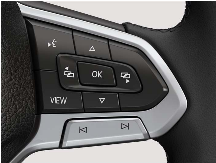
Fig. 1 Right side of the multifunction steering wheel: operating the digital instrument cluster Pro (variant 1).
