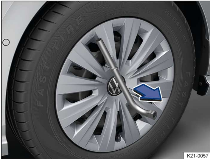
Fig. 1 Removing the wheel cover.
