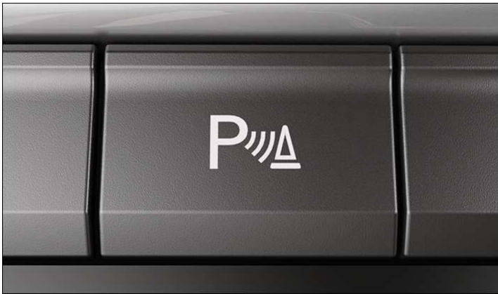
Fig. 1 In the upper section of the centre console: Park Distance Control button (illustration).
