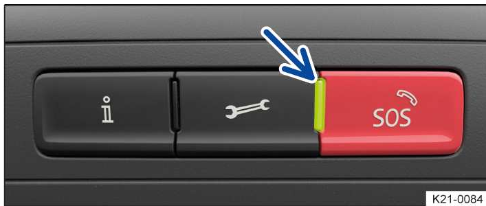
Fig. 1 In the roof console: buttons for voice services and indicator lamp.
