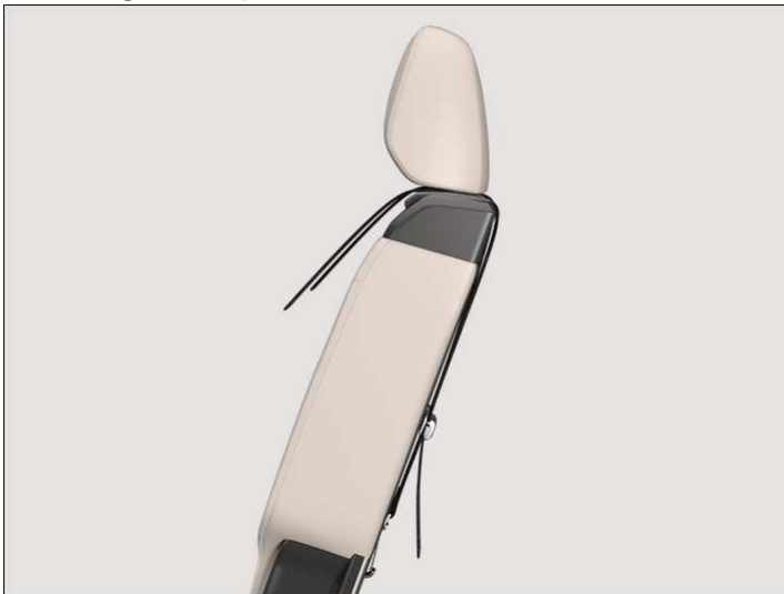
Fig. 2 On the rear of the outer rear seats: attached top tether.
