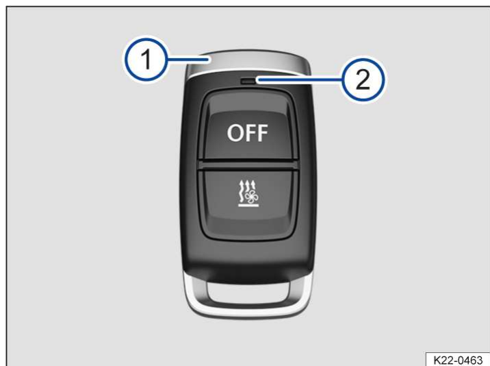
Fig. 1 Remote control for the auxiliary heater.
