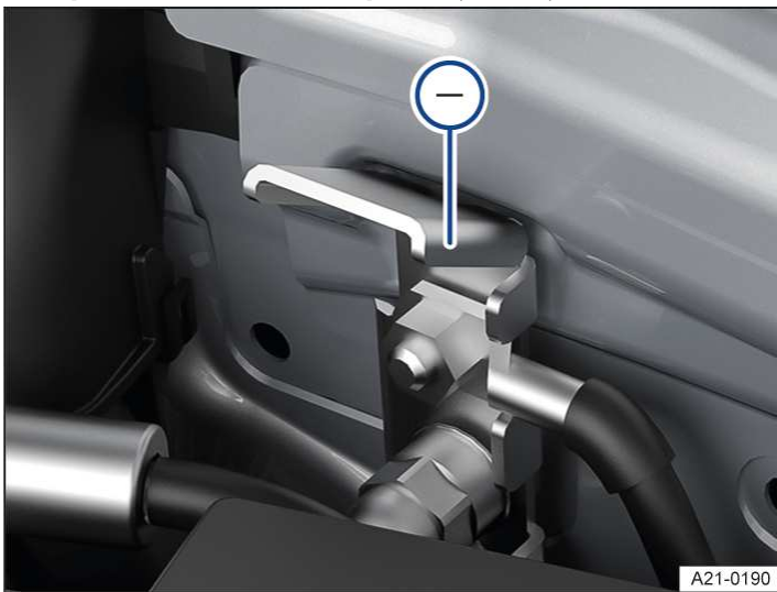
Fig. 1 In the bonnet space: jump-start connection point (earth).
