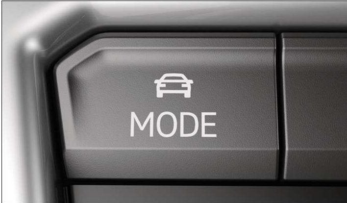
Fig. 1 In the centre console: MODE button for driving profile selection.
