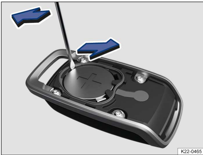
Fig. 2 Replacing the button cell in the remote control.
