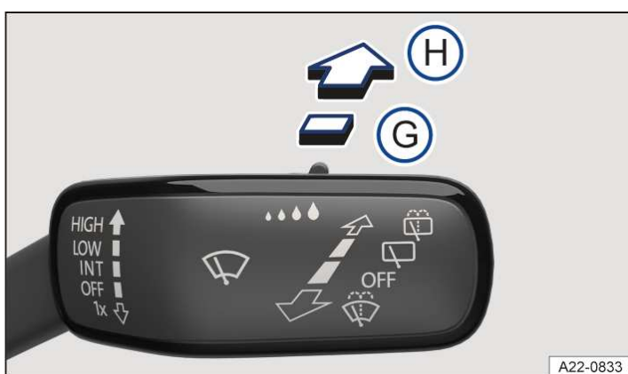
Fig. 2 On the right-hand side of the steering column: operating the rear window wiper.
