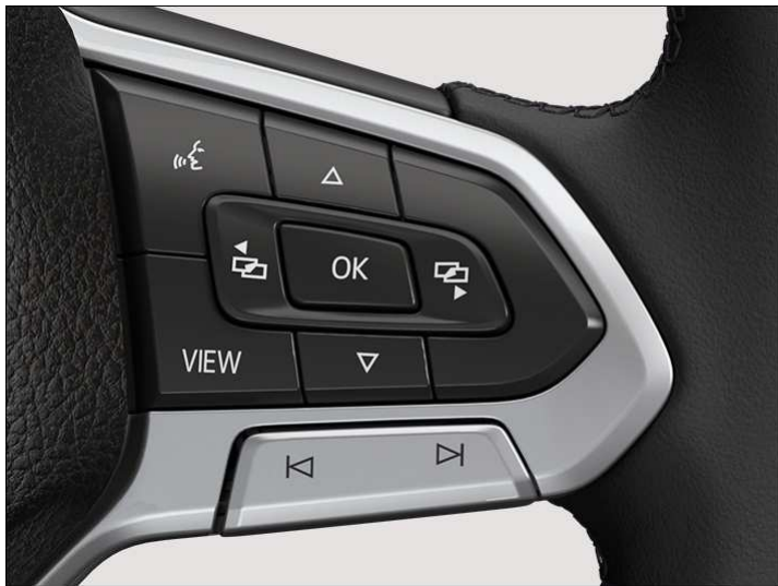
Fig. 1 Right side of the multifunction steering wheel: operating the digital instrument cluster Basic.
