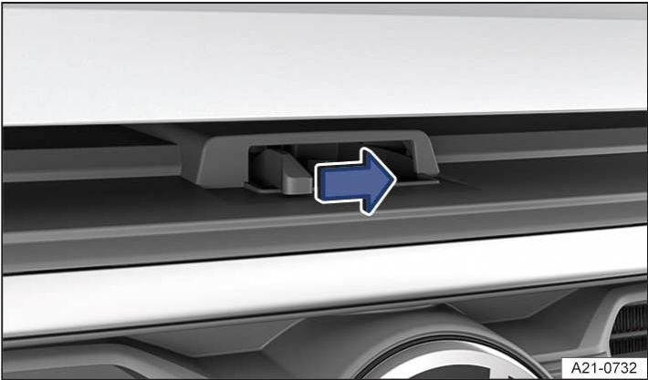
Fig. 2 Above the radiator grille: bonnet control lever.
