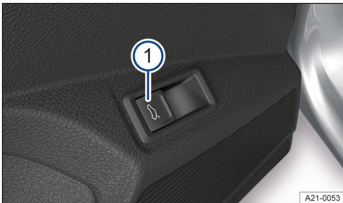
Fig. 2 In the driver door: button for opening the boot lid electrically (illustration).
