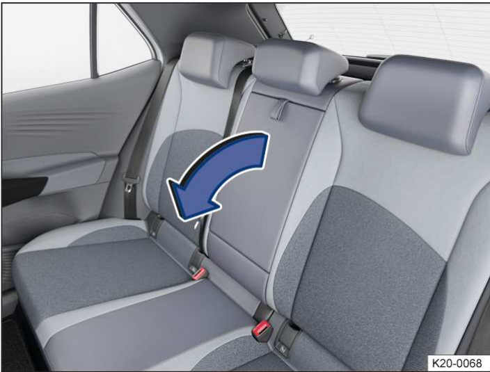
Fig. 2 In the backrest of the middle seat: fold-out rear centre armrest.
