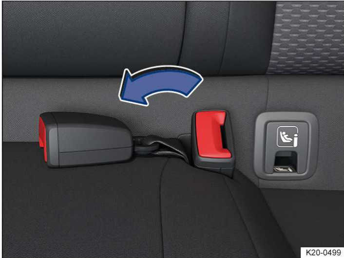
Fig. 1 Middle seat: folding down belt buckle.
