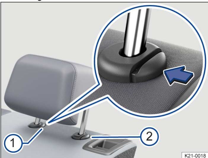
Fig. 2 Removing a rear head restraint (illustration).
