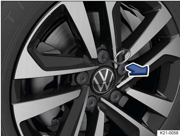
Fig. 1 Removing the wheel bolt caps.
