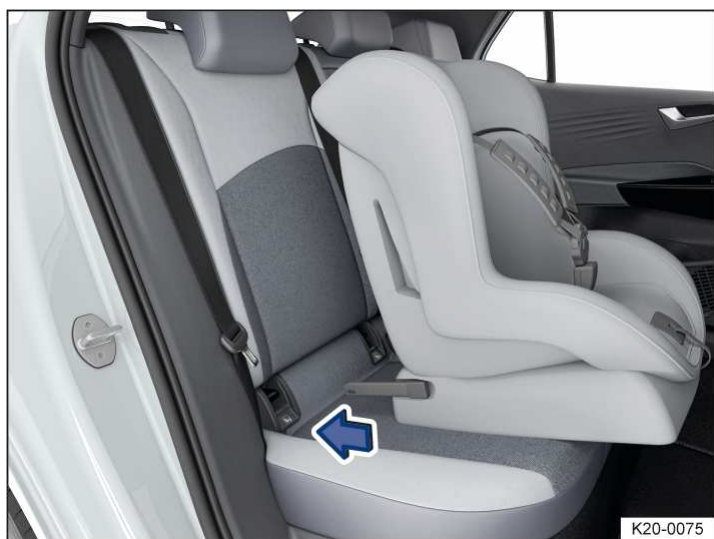
Fig. 1 Fitting a child seat with attachment arms (illustration).
