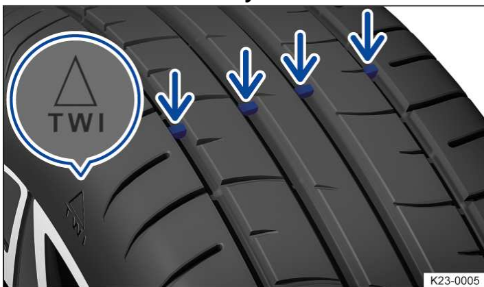
Fig. 1 In the tread grooves: tread wear indicator.
