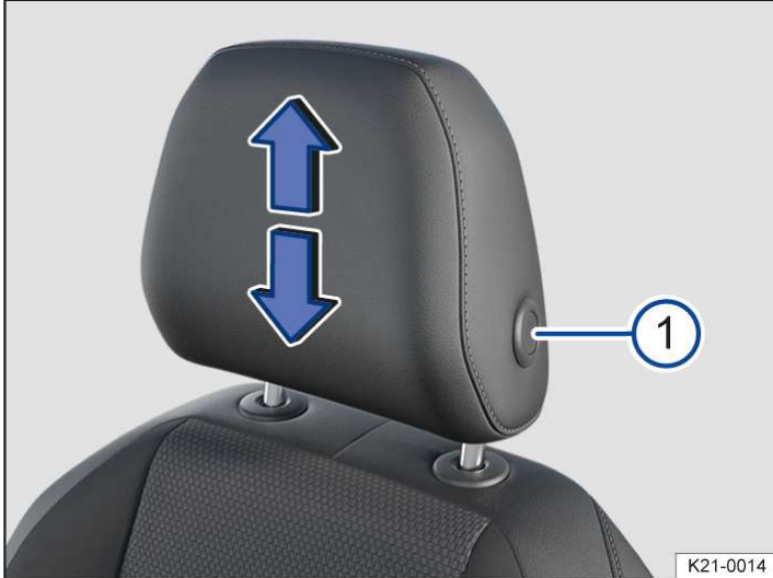
Fig. 1 Adjusting a front head restraint (illustration).
