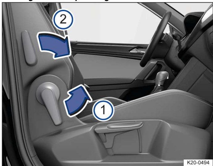
Fig. 1 Front passenger seat: folding backrest forwards.
