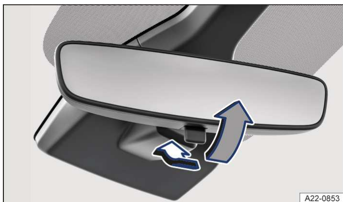
Fig. 2 On the windscreen: manual anti-dazzle interior mirror.
