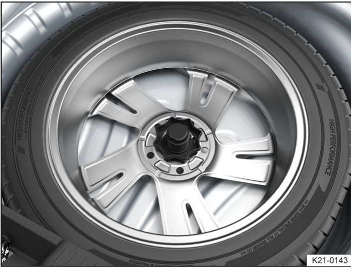
Fig. 1 Under the luggage compartment floor: handwheel for securing the spare wheel or temporary spare wheel.
