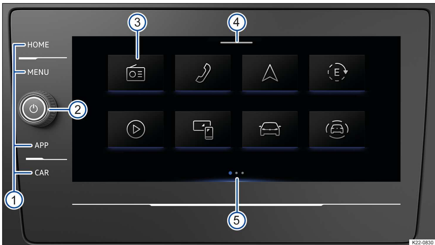
Fig. 3 Overview of the Infotainment system (illustration).
