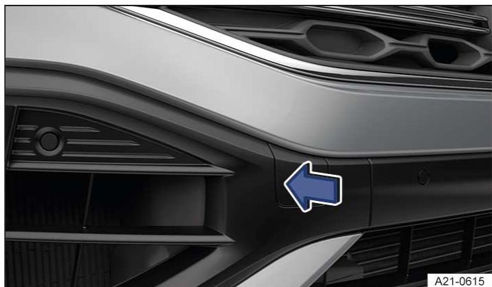
Fig. 2 In the front bumper on the right: removing the cover, variant 2.
