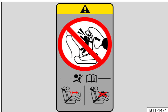
Fig. 2 On the B-pillar: airbag label (illustration).
