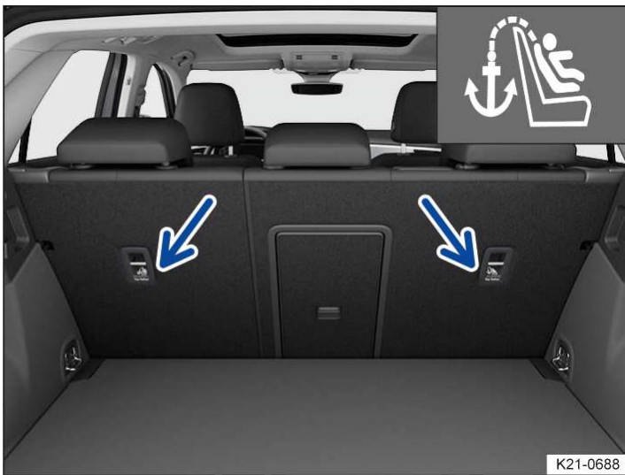
Fig. 1 On the rear of the rear seats: top tether anchor points for top tether.
