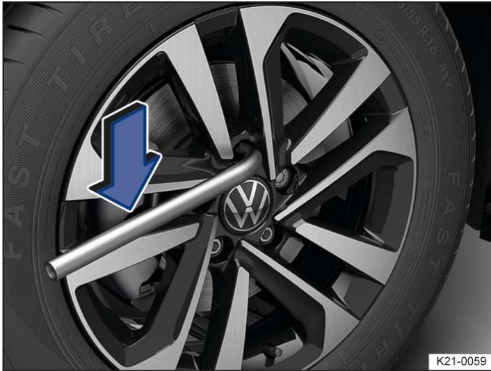
Fig. 1 Loosening wheel bolts.
