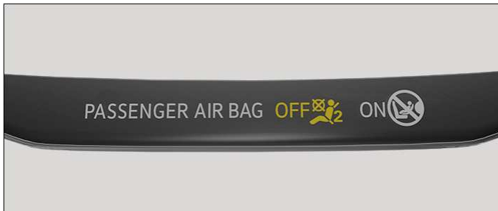
Fig. 3 In the roof console: indicator lamp for switched off front passenger front airbag.
