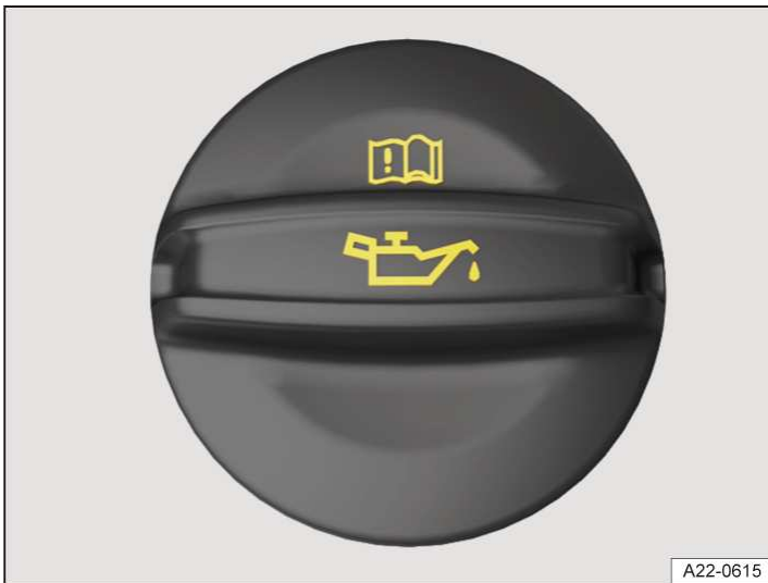
Fig. 1 In the bonnet space: engine oil filler opening cap (illustration).
