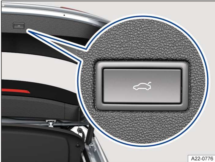
Fig. 1 In the open boot lid: button for closing boot lid electrically.
