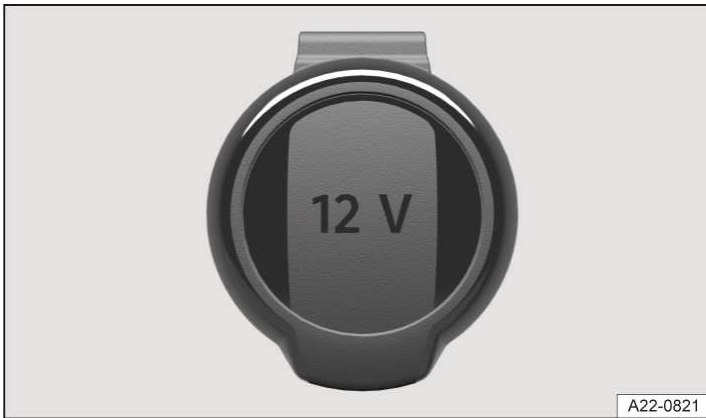
Fig. 1 In the lower part of the centre console: fold-open 12-volt socket (illustration).
