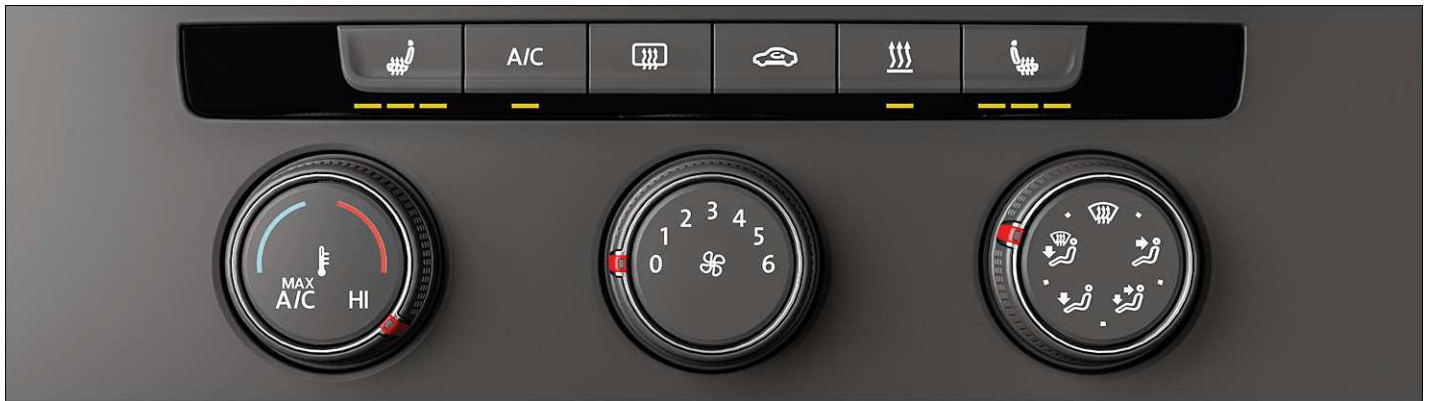
Fig. 1 In the upper section of the centre console: air conditioning block for the manual air conditioning system.
