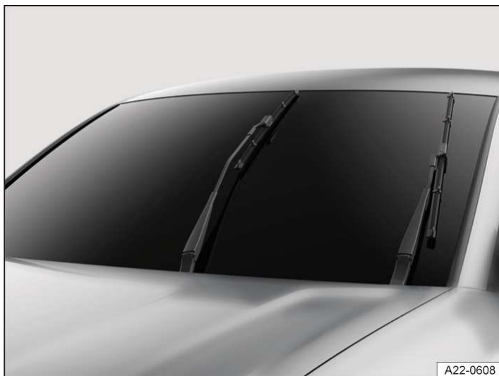
Fig. 1 Wipers in service position (illustration).
