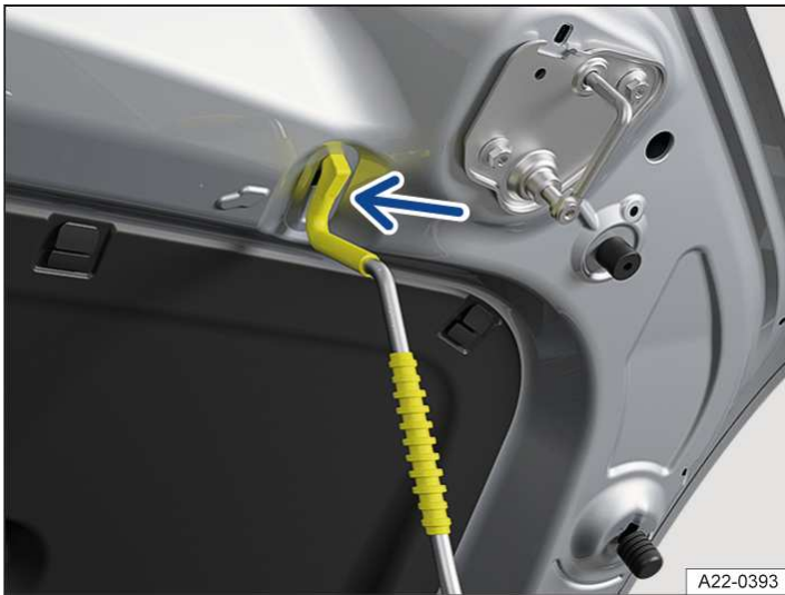
Fig. 4 On the bonnet: holder for bonnet stay.
