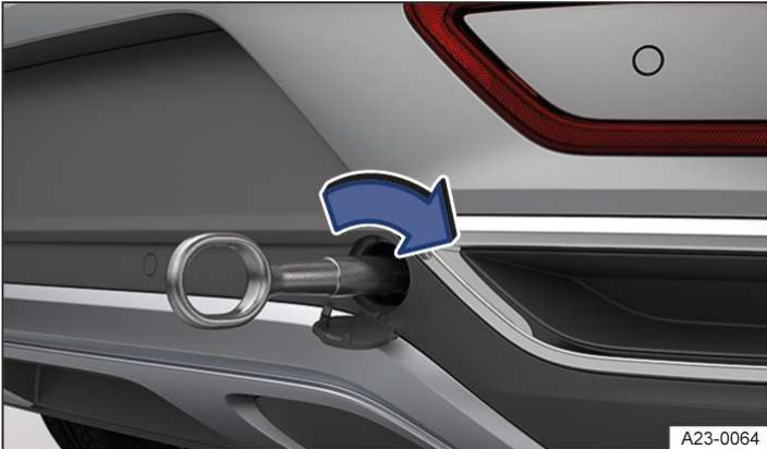
Fig. 3 In the rear bumper on the right: screwing in the towing eye, variant 1.
