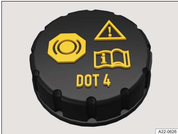
Fig. 1 In the bonnet space: cap of the brake fluid reservoir.
