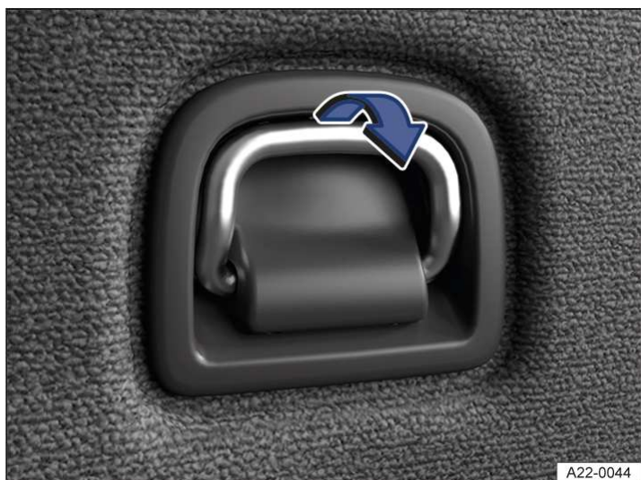
Fig. 2 In the luggage compartment: folding fastening ring (illustration).
