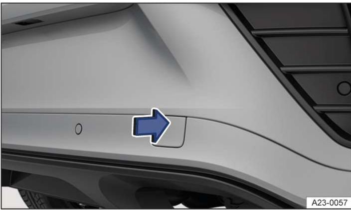
Fig. 2 In the rear bumper on the right: removing the cover, variant 2.
