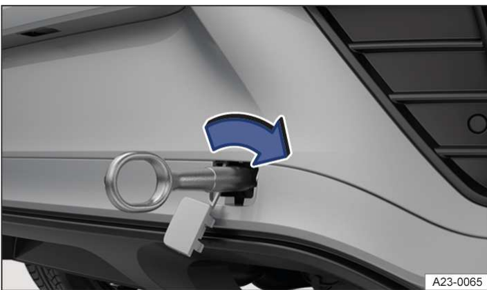
Fig. 4 In the rear bumper on the right: screwing in the towing eye, variant 2.
