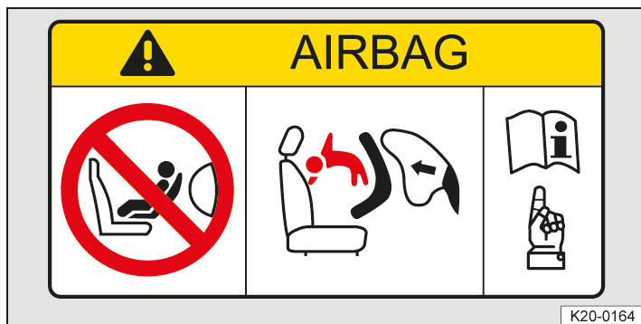
Fig. 1 On the sun visor: airbag label (illustration).
