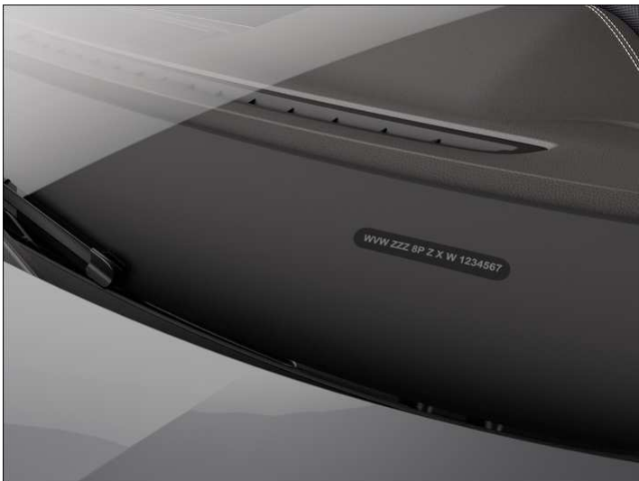
Fig. 1 In the windscreen: vehicle identification number.
