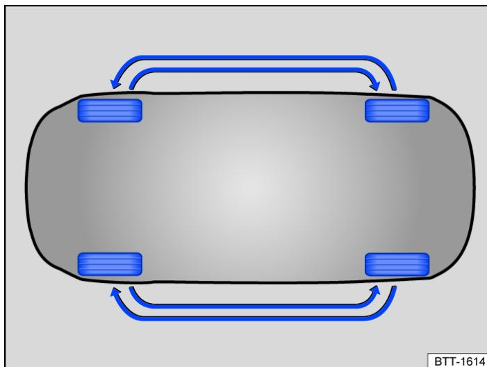
Fig. 1 Illustration: diagram showing how to swap wheels.
