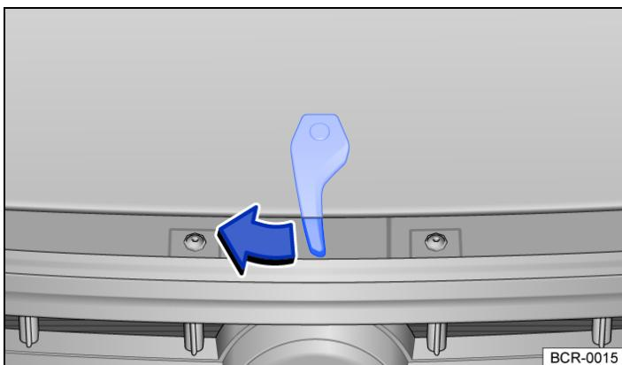
Fig. 2 Above the radiator grille: bonnet control lever.
