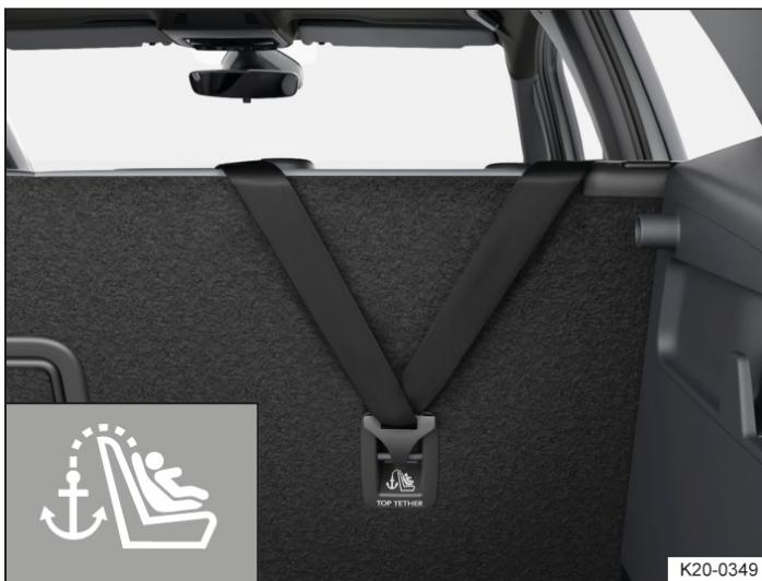
Fig. 1 In the luggage compartment: attached top tether.
