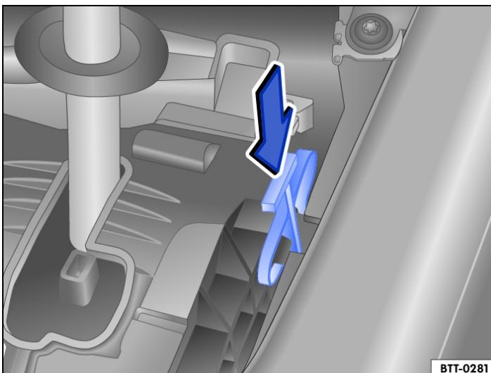
Fig. 2 Manually release selector lever lock (variant 2)
