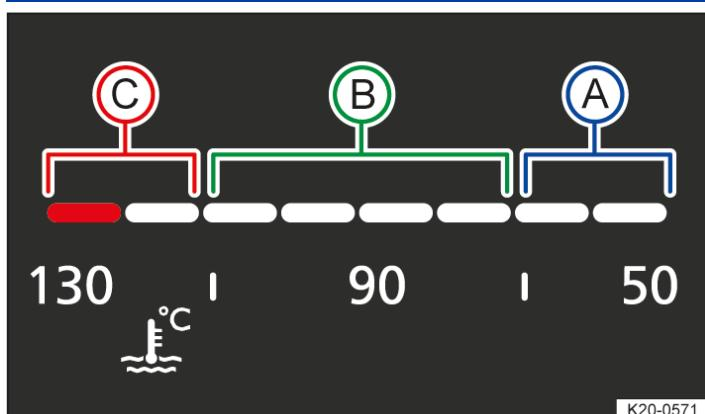
Fig. 2 Coolant temperature display in the digital instrument cluster Basic version (illustration).
