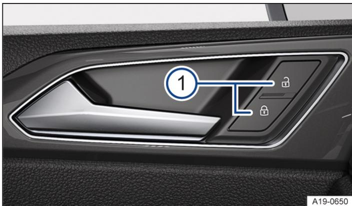
Fig. 1 In the driver door: central locking button.
