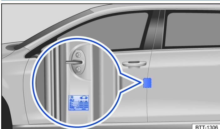
Fig. 2 On the driver door pillar: tyre pressure sticker
