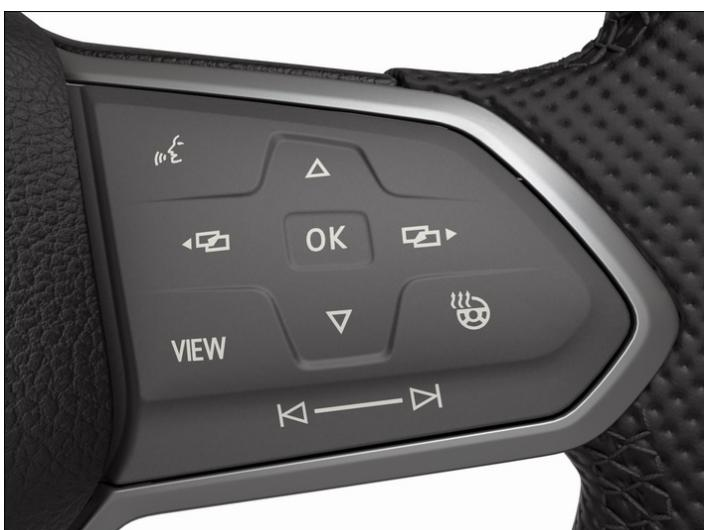
Fig. 2 Right-hand side of the multifunction steering wheel: controls for using the menus and information displays in the digital instrument cluster Pro version (variant 2).
