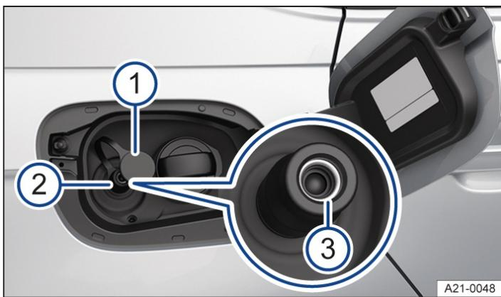
Fig. 1 Behind the tank flap: gas filler neck.
