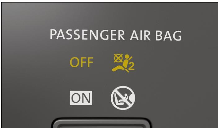
Fig. 1 In the centre console: indicator lamp for disabled front passenger front airbag.
