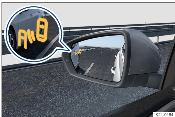
Fig. 1 In the exterior mirror: visual signals of the lane change system.
