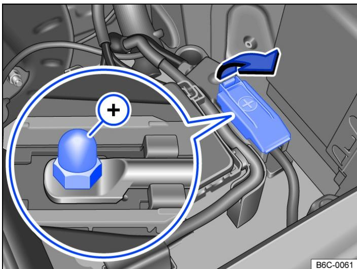
Fig. 1 In the engine compartment underneath a cover: jump-start connection point (positive battery terminal).
