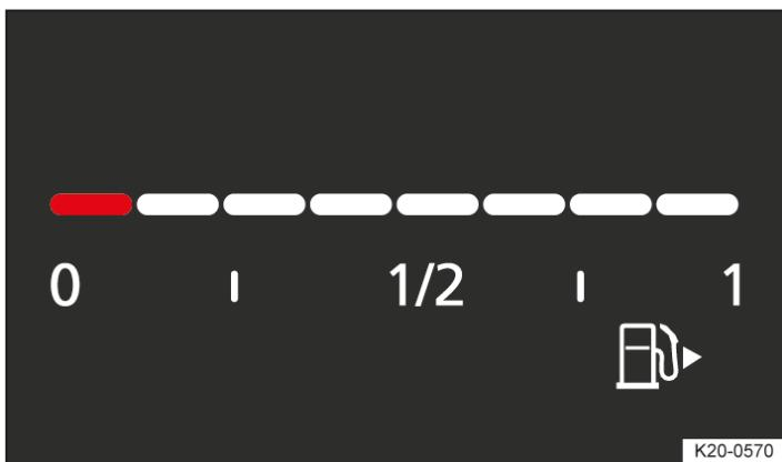
Fig. 2 Fuel gauge in the digital instrument cluster Basic version (illustration).
