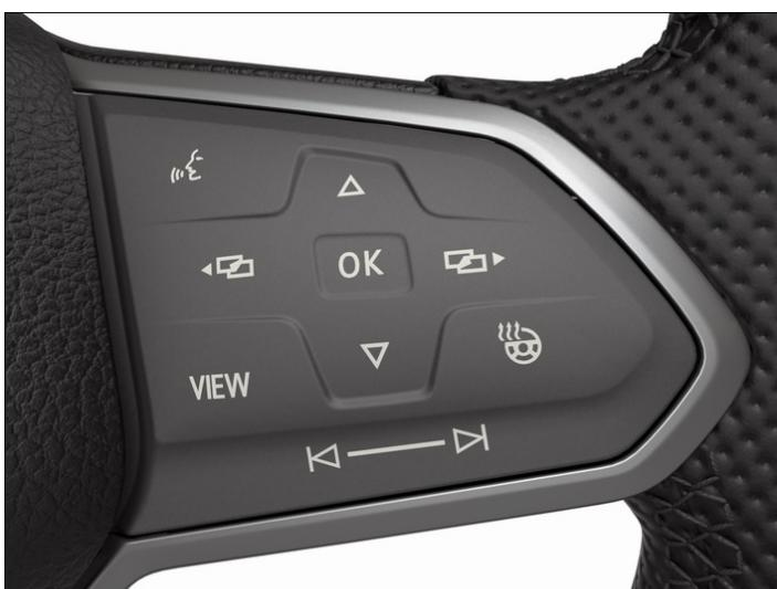
Fig. 2 Right-hand side of the multifunction steering wheel: controls for using the menus and information displays in the digital instrument cluster Basic version (variant 2).
