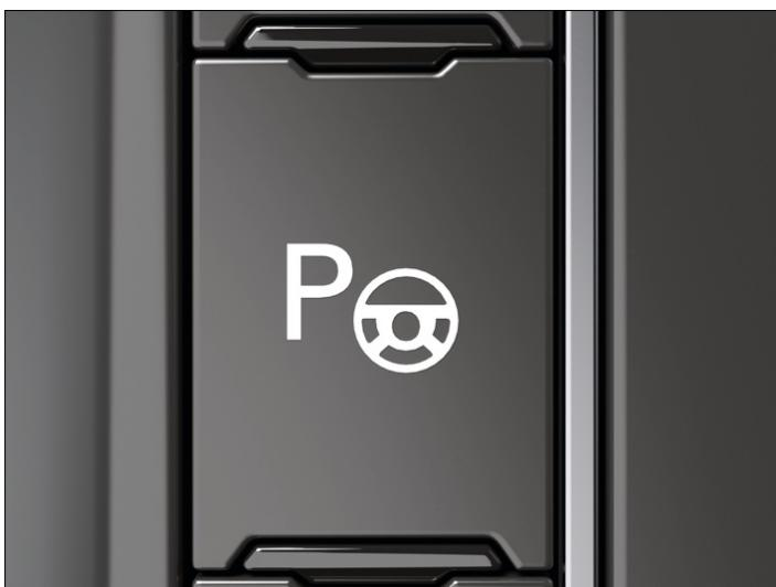
Fig. 1 In the centre console: button for Park Assist.
