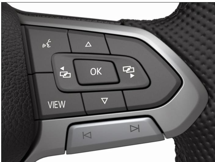
Fig. 1 Right-hand side of the multifunction steering wheel: controls for using the menus and information displays in the digital instrument cluster Pro version (variant 1).
