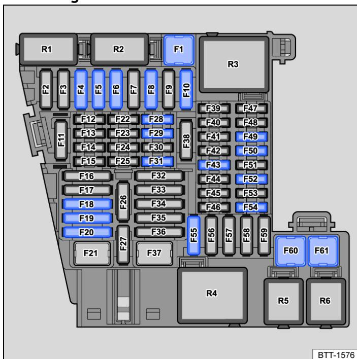
Fig. 1 In the dash panel: fuse locations.
