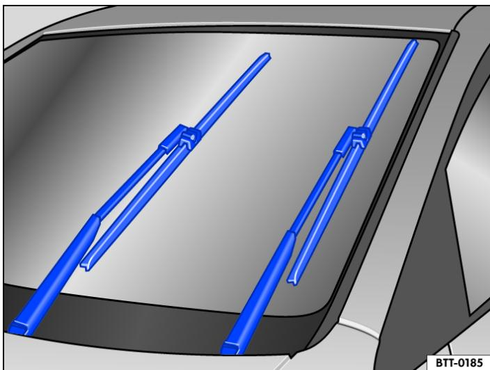
Fig. 1 Wipers in service position (illustration).
