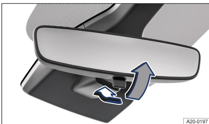
Fig. 2 On the windscreen: manual anti-dazzle interior mirror.
