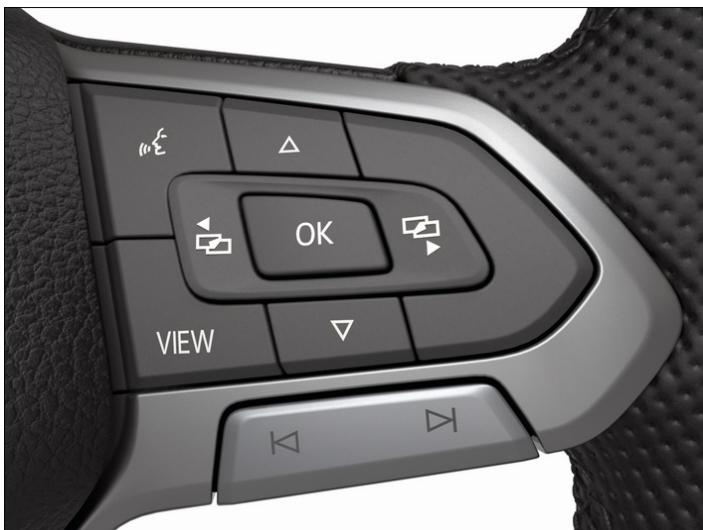
Fig. 1 Right-hand side of the multifunction steering wheel: controls for using the menus and information displays in the digital instrument cluster Basic version (variant 1).
