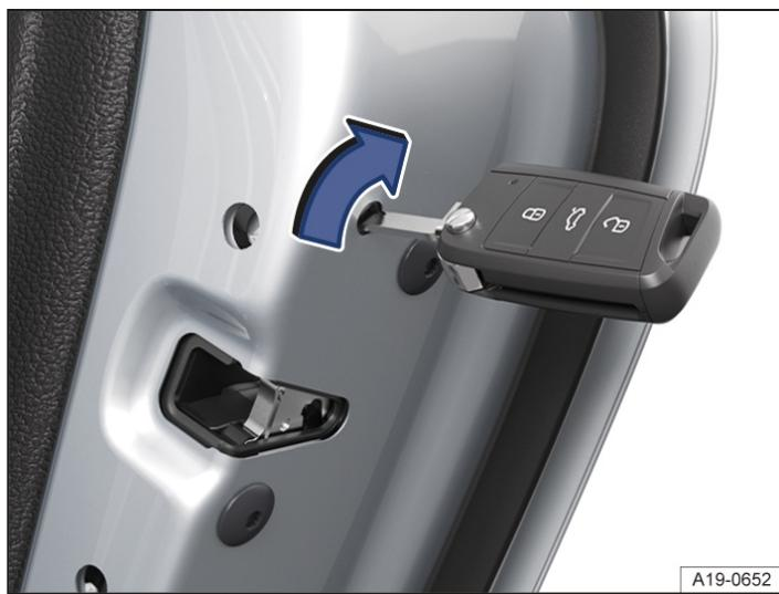
Fig. 1 In the front edge of the rear right-hand door: manually locking the vehicle with the vehicle key (illustration).
