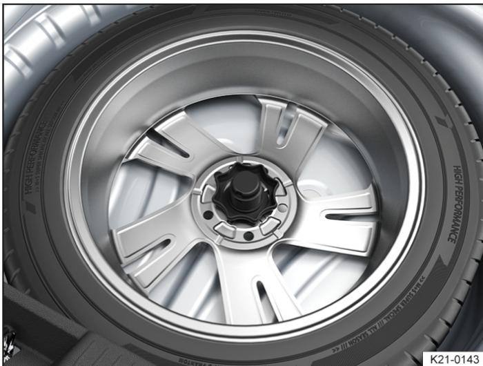
Fig. 1 In the luggage compartment: handwheel for securing the spare wheel or temporary spare wheel.
