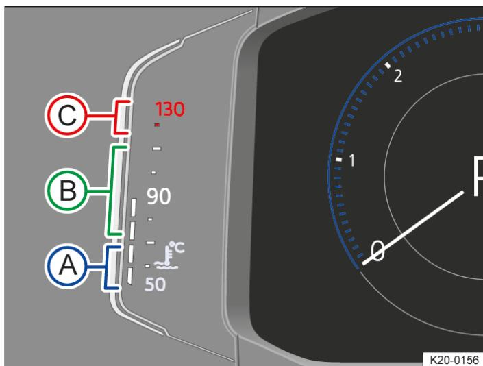
Fig. 1 Coolant temperature display in the digital instrument cluster Pro version (illustration).
