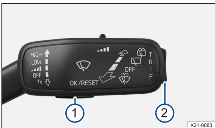
Fig. 3 On the right of the steering column: buttons on the wiper lever.
