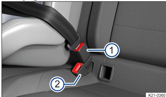
Fig. 1 Position of seat belt buckles on the rear bench seat.
