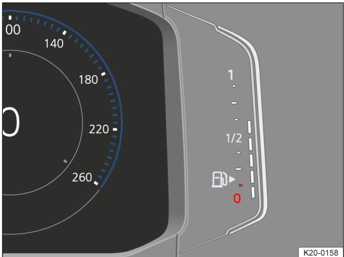
Fig. 1 Fuel gauge in the digital instrument cluster Pro version (illustration).
