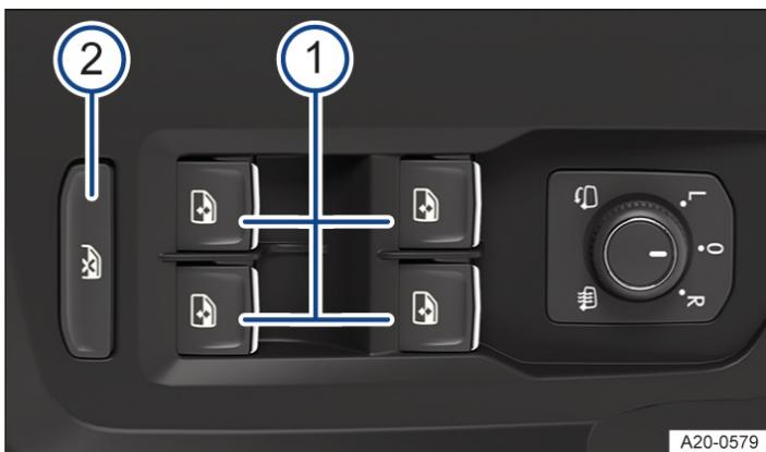
Fig. 1 In the driver door: electric window buttons.
