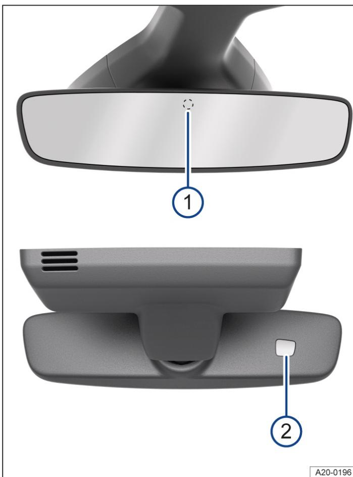
Fig. 1 On the windscreen: automatic anti-dazzle interior mirror.
