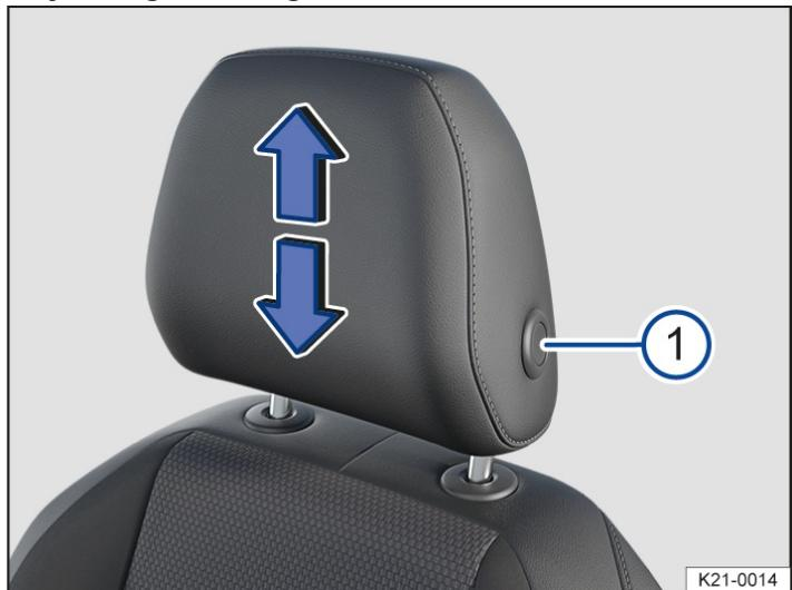
Fig. 1 Illustration: adjusting the front head restraint.
