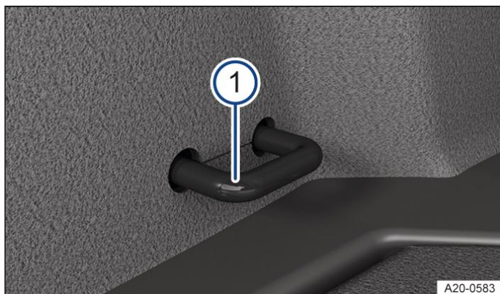
Fig. 1 In the luggage compartment: fastening ring.
