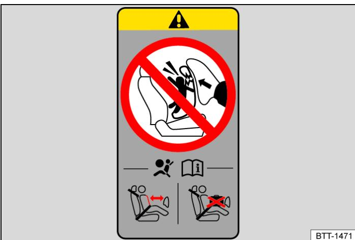
Fig. 2 Illustration: airbag label on the B-pillar.
