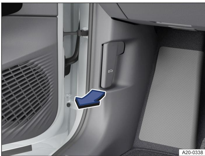
Fig. 1 In the footwell on the driver side: bonnet release lever (schematic diagram).
