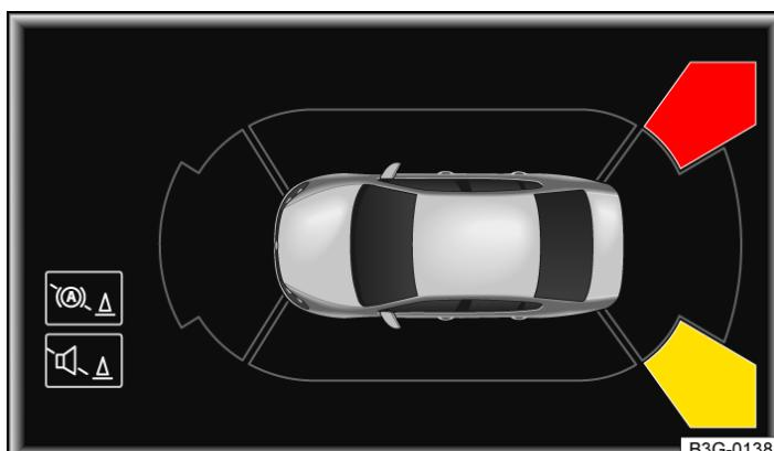
Fig. 2 Infotainment system: Rear Traffic Alert display.
