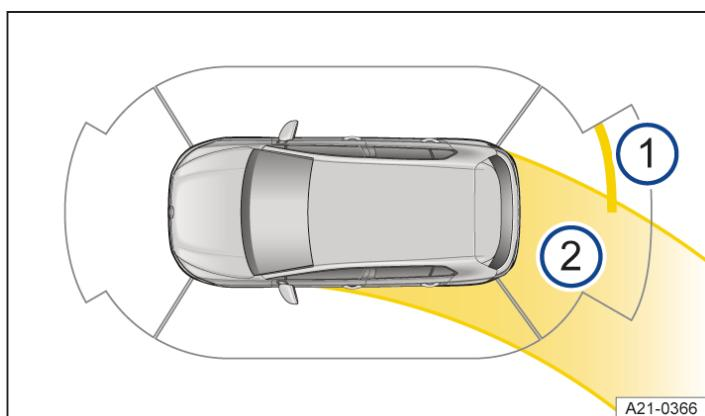
Fig. 1 Infotainment system: Park Distance Control display (illustration).
