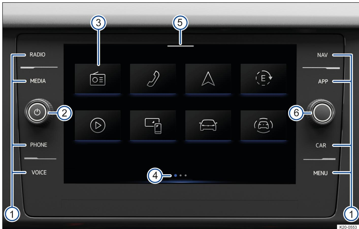
Fig. 1 Overview: display and operating unit of the 8" version
