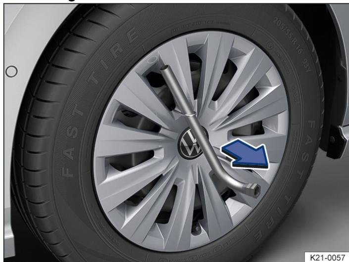
Fig. 1 Removing the wheel cover.
