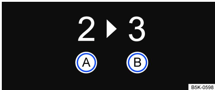
Fig. 1 On the instrument cluster display: gear-change indicator.
