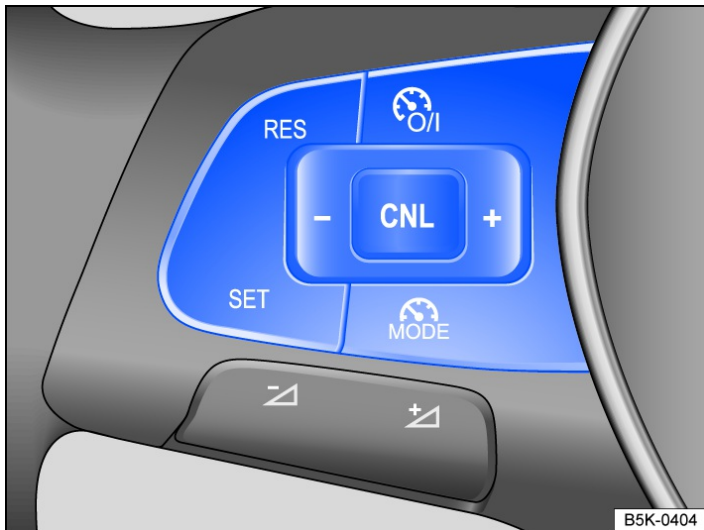
Fig. 1 Lefthand side of the multifunction steering wheel.
