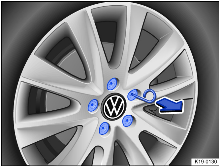
Fig. 1 Removing the wheel bolt caps.
