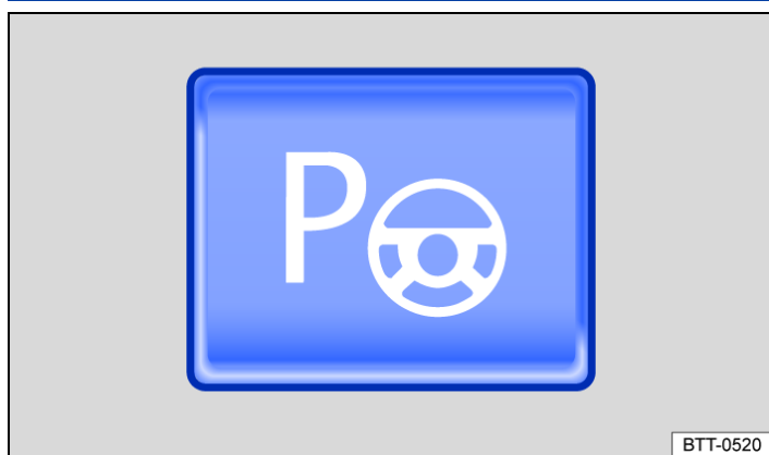
Fig. 2 In the centre console: button for switching on the Park Assist system (illustration).
