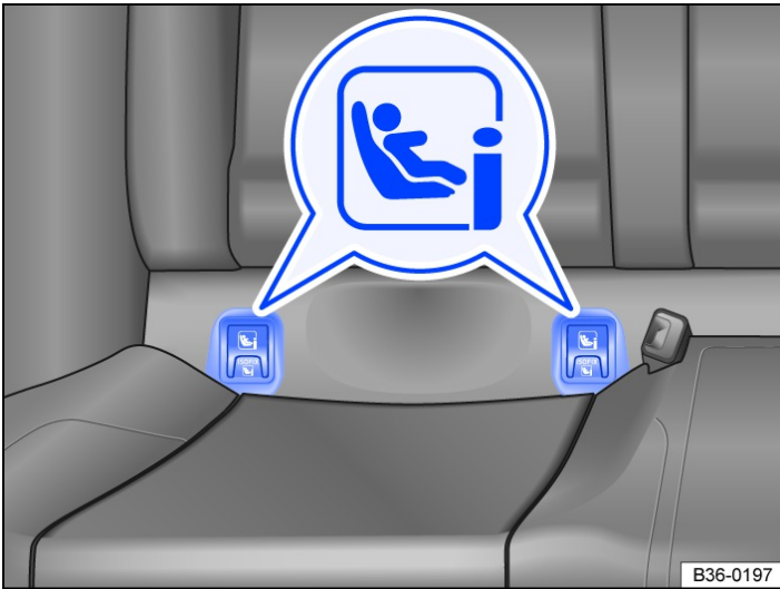
Fig. 3 Markings identifying the i-size anchorage points for child seats.
