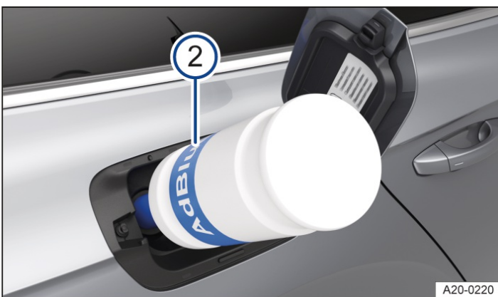
Fig. 2 Behind the tank flap: refilling AdBlue using the refill bottle (illustration).
