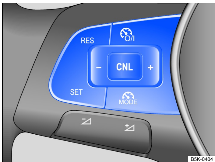
Fig. 1 Left-hand side of the multifunction steering wheel.
