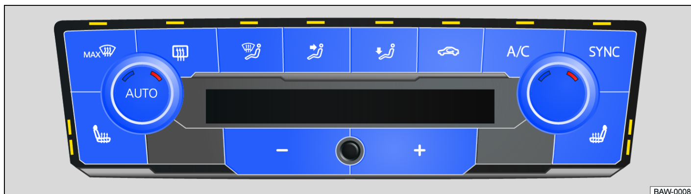
Fig. 2 In the upper part of the centre console: Climatronic air conditioning block.
