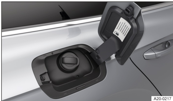
Fig. 1 Behind the tank flap: tank cap (illustration).
