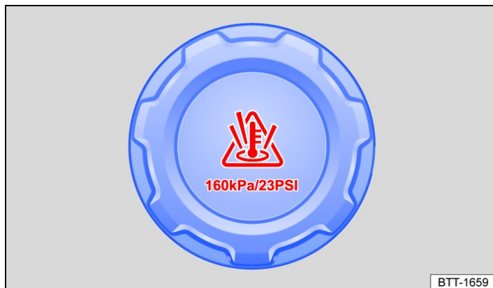
Fig. 1 In the engine compartment: coolant expansion tank cap (illustration).
