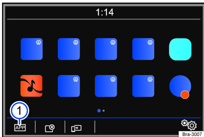
Fig. 1 MirrorLink main menu: function buttons in the overview of compatible apps.
