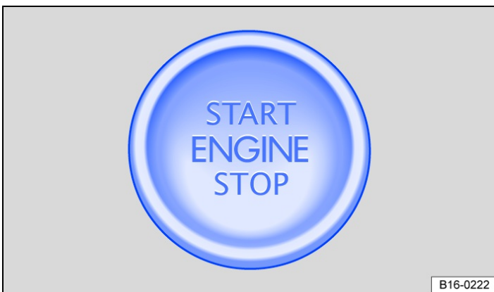
Fig. 1 In the lower section of the centre console: starter button for starting the engine.
