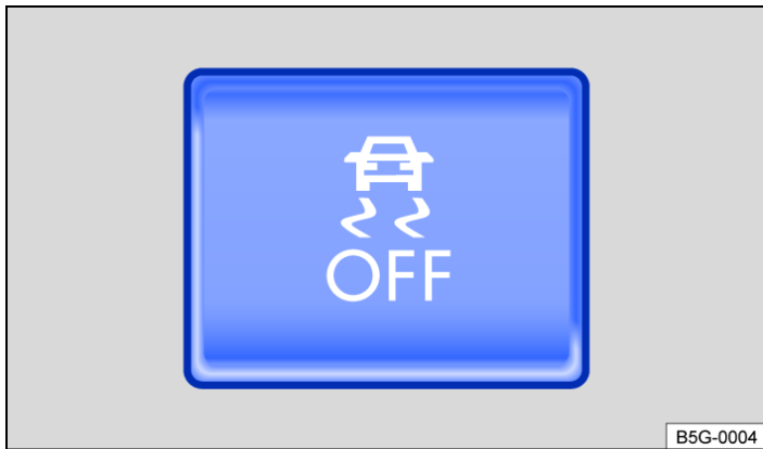
Fig. 1 In the centre console: button for switching TCS or ESC Sport on and off manually (with some equipment levels).
