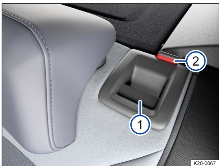
Fig. 1 In the rear seat backrest: release button.
