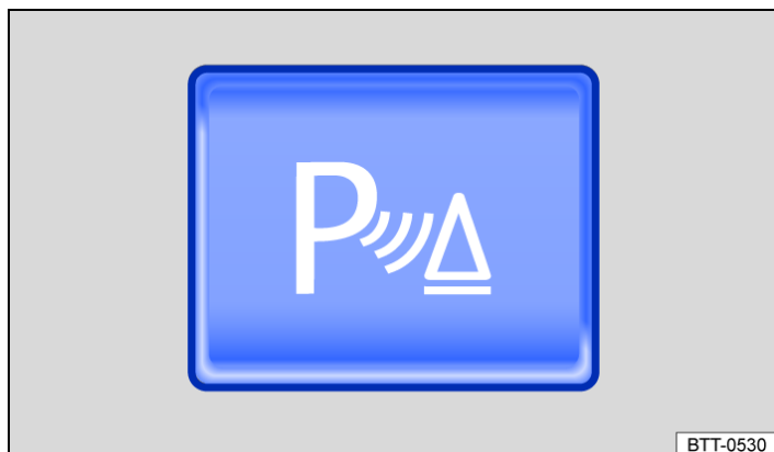
Fig. 1 In the centre console: button for switching Park Distance Control on and off (schematic diagram).
