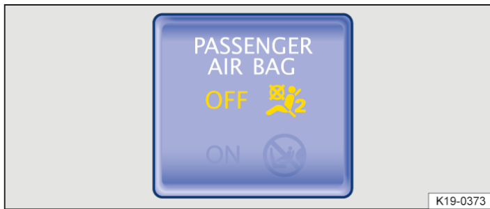
Fig. 1 In the centre console: indicator lamp for disabled front passenger front airbag.
