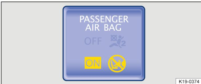
Fig. 2 In the centre console: indicator lamp for activated front passenger front airbag.
