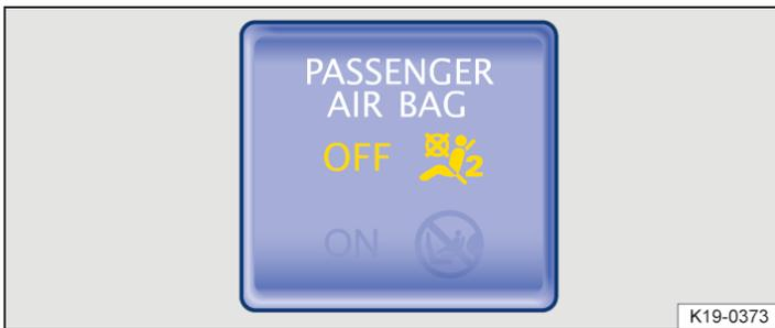
Fig. 1 In the centre console: indicator lamp for deactivated front passenger front airbag.
