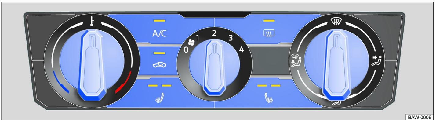
Fig. 1 In the upper section of the centre console: air conditioning block for the manual air conditioning system.
