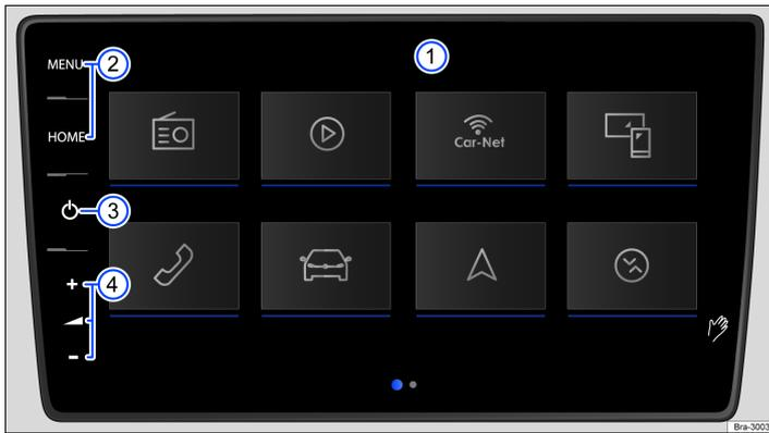
Fig. 1 Overview of control elements (9.2 inch).
