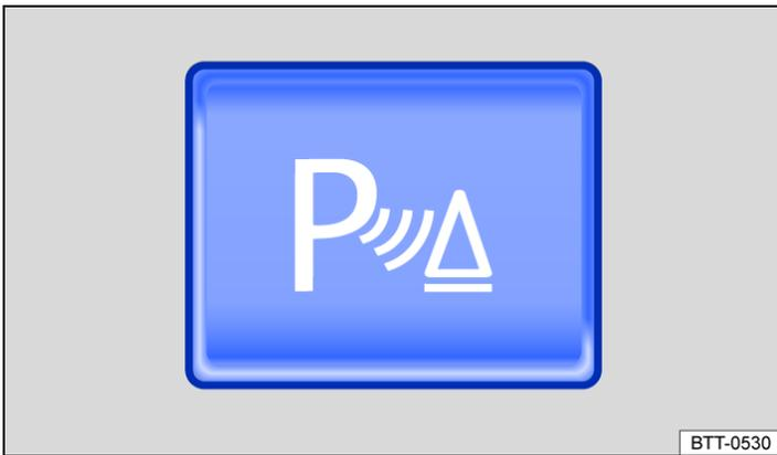
Fig. 1 In the centre console: button for switching Park Distance Control on and off.
