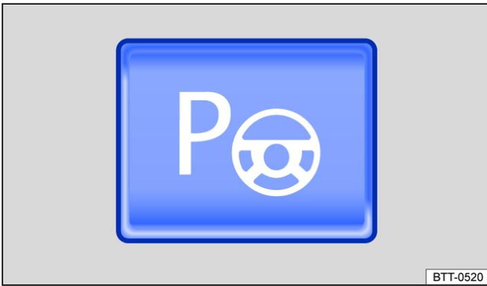
Fig. 1 In the centre console: button for switching on the Park Assist system.
