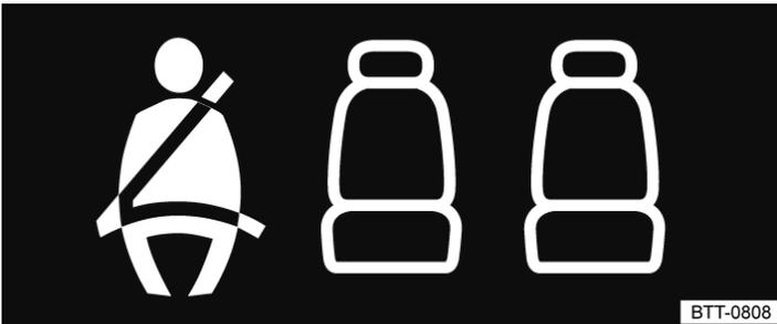
Fig. 2 On the instrument cluster display: seat belt status for the rear seats.
