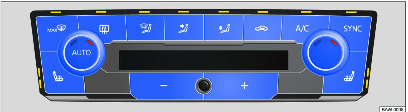
Fig. 2 In the upper part of the centre console: Climatronic air conditioning block.
