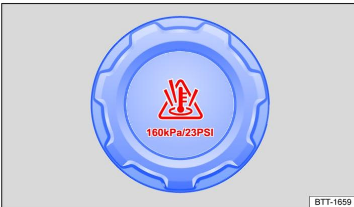
Fig. 2 In the engine compartment: coolant expansion tank cap (illustration).
