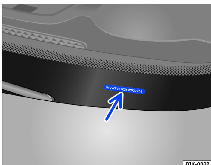
Fig. 1 In the windscreen: vehicle identification number.
