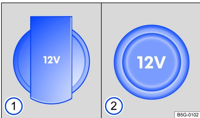
Fig. 1 In the front centre console: fold-open 12-volt socket 1 or 12-volt socket with removable cover 2.
