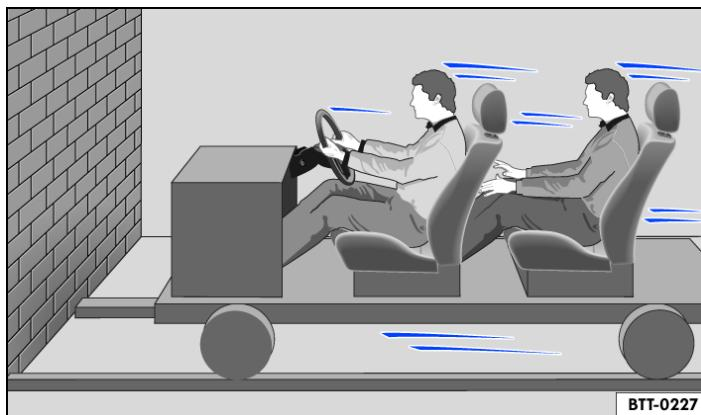
Fig. 1 Unbelted occupants in a vehicle heading for a brick wall.
