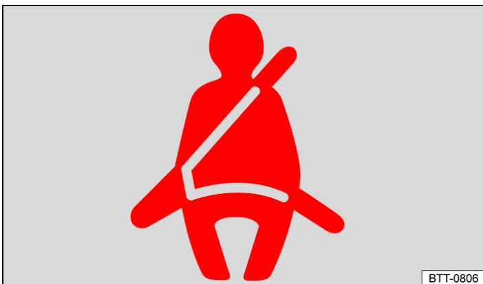
Fig. 1 On the instrument cluster display: warning lamp.
