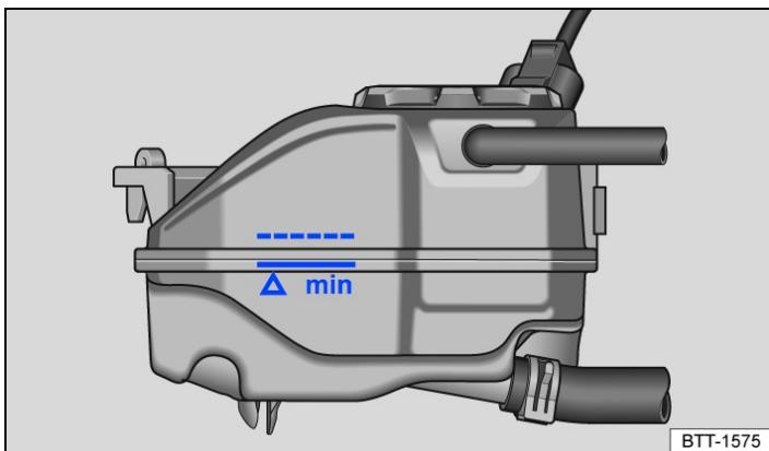
Fig. 1 In the engine compartment: markings on the coolant expansion tank (illustration).
