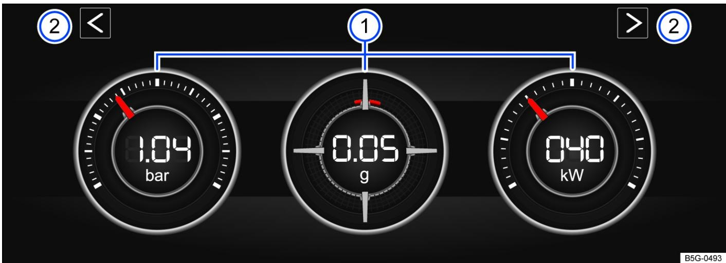
Fig. 1 On the Infotainment system display: performance monitor.
