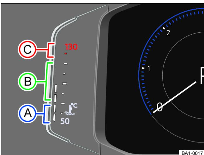
Fig. 2 Coolant temperature gauge in the Active Info Display.
