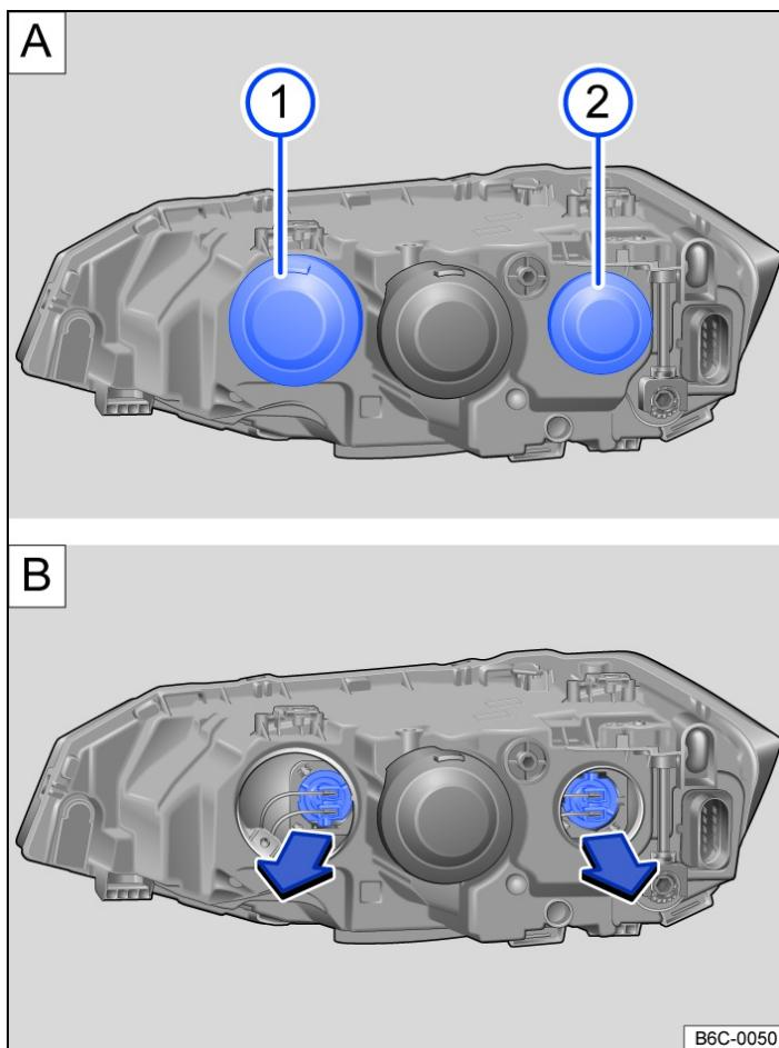
Fig. 1 Rear view of the right-hand H7 headlight: 1 dipped beam, 2 main beam.
