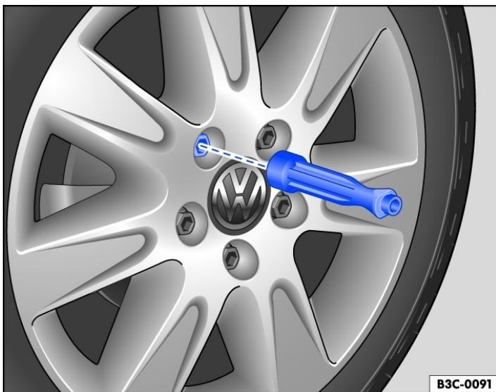
Fig. 1 Changing a wheel: removing the wheel bolts with the screwdriver handle.
