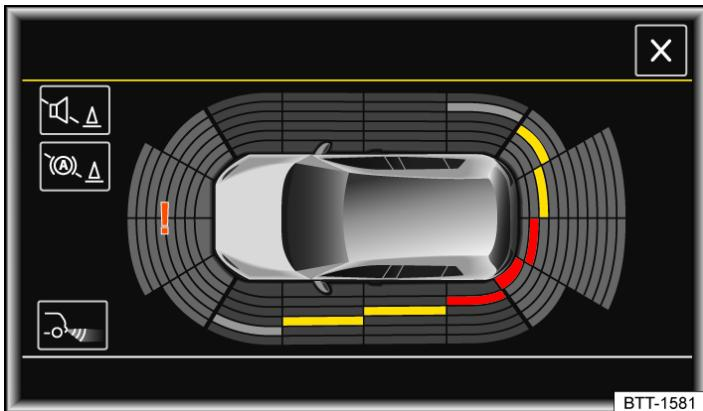
Fig. 1 On the Infotainment system screen: detection ranges of the Park Distance Control.
