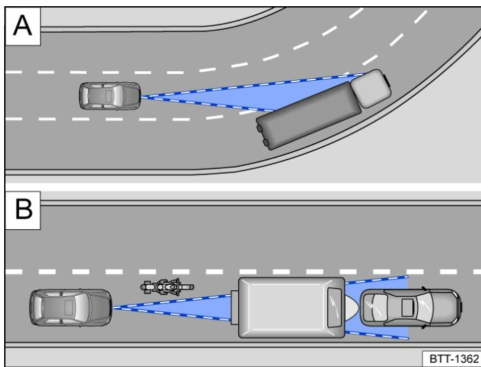
Fig. 1 **A** Driving through bends. **B** Vehicles outside the range of the radar sensor.
