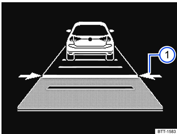
Fig. 1 On the instrument cluster display: setting the distance (illustration, the ACC is active).
