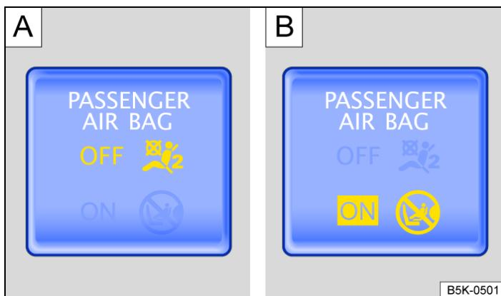
Fig. 1 In the centre console: indicator lamp for deactivated front passenger front airbag **A** or for activated front passenger front airbag **B**.
