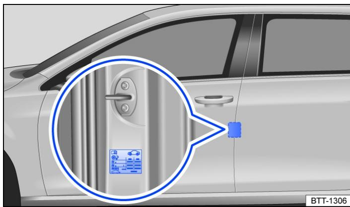
Fig. 2 On the driver door pillar: tyre pressure sticker (alternatively on the inside of the fuel flap).
