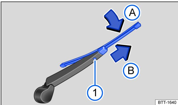
Fig. 2 Changing the rear window wiper blade.
