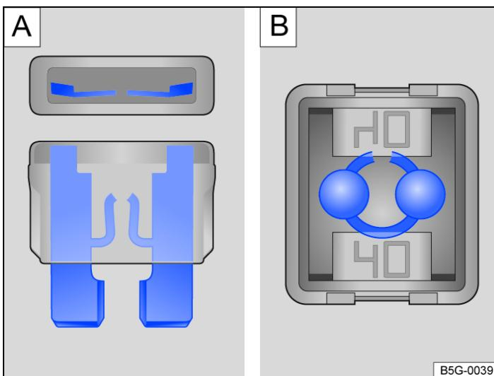
Fig. 1 Blown fuse: **A** flat blade fuse, **B** cartridge fuse.
