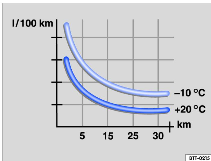
Fig. 1 Fuel consumption in litres per 100 km at two different outside temperatures.
