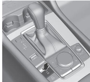
When the parking brake is released, the EPB indicator light (P) in the instrument cluster and the EPB switch indicator light turn off.
