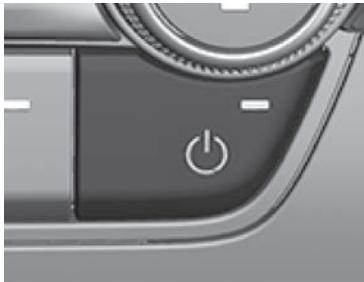
Switches the air-conditioning system on and off.
