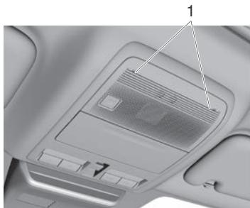
1. Intrusion sensor and intrusion sensor bezel
