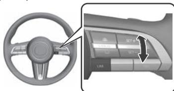
When you set the speed, the set speed is displayed on the screen. In addition, the ASL standby indication (white) **LIM** changes to the ASL set indication (green) **LIM**.
