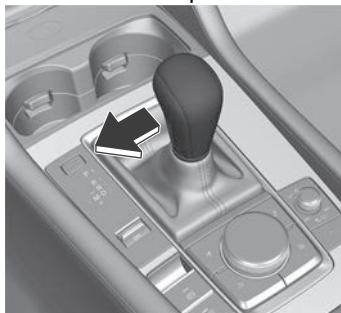
The gear position can be switched manually in manual shift mode.
