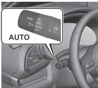
The HBC determines the surrounding conditions and operates automatically. When the HBC operates, the HBC indicator light (green)
