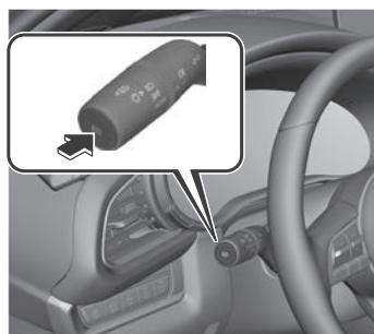
When the ALH is cancelled, the ALH indicator light (green)
