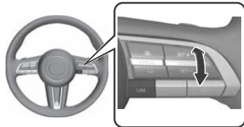
When you set the speed, the set speed is displayed on the screen. In addition, the ISA standby indication (white) **LIM** changes to the ISA set indication (green) **LIM**.
