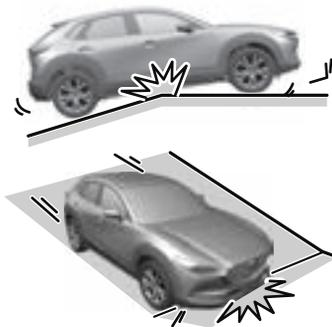
This vehicle is equipped with low profile tires allowing class-leading performance and handling. As a result, the sidewall of the tires are very thin and the tires and wheels can be damaged if driven through potholes or on rough/uneven roads at excessive speeds. Use care and reduce speed when traveling on rough/uneven roads or through potholes.
