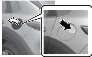
3. To remove the fuel-filler cap, turn it counterclockwise.
