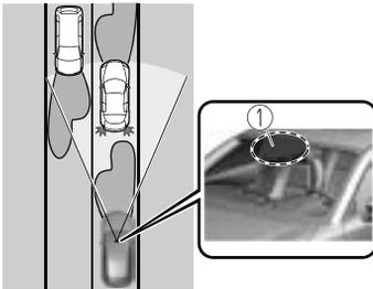
1. Forward Sensing Camera (FSC)\*<sup>1</sup>
