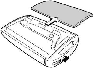
2. Remove the auxiliary key.
