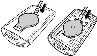
6. Remove the battery using tape-wrapped flathead screwdriver.
