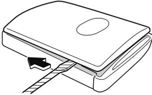
4. Twist the flathead screwdriver in the direction of the arrow and remove the upper cover.
