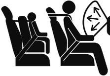
**Do not install a front-facing child-restraint system on the front passenger seat unless it is unavoidable:**
