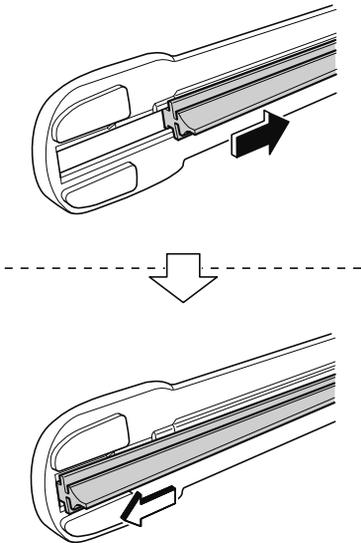
8. Make sure that the blade rubber is correctly installed to the blade holder.
