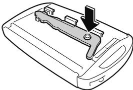
2. Insert the tabs of the lower cover into the slots of the transmitter and install the lower cover.
