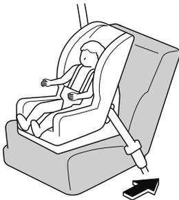
3. Remove the head restraint. However, when installing a backless booster seat, always install the vehicle head restraint to the seat where the backless booster seat is installed.
