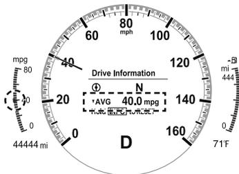
The average fuel economy can be reset by pressing the INFO switch for 1.5 seconds or more. After the data is cleared, the fuel consumption is recalculated and the - - - L/100 km ( - - - mpg) for the 30 seconds prior to it being displayed is indicated.
