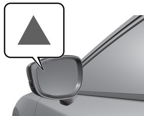
When the ignition is switched ON, the warning indicator light turns on momentarily and then turns off after a few seconds.
