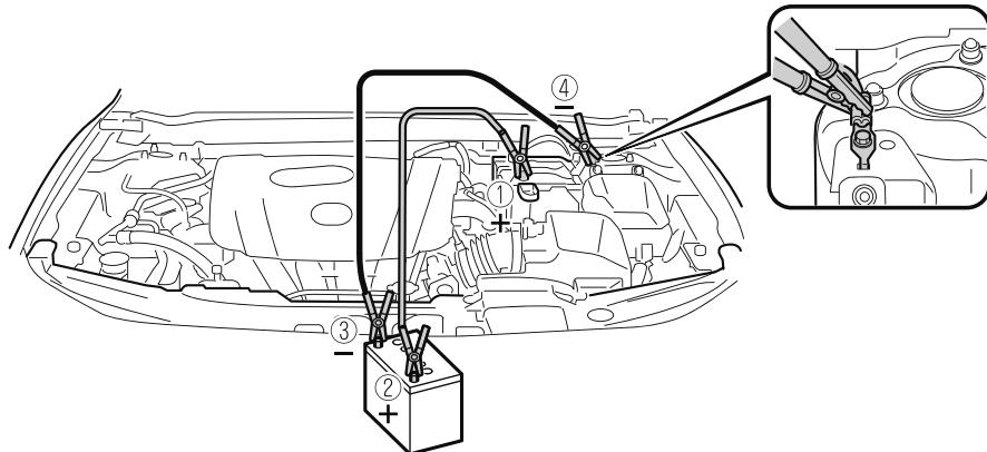
5. Start the booster vehicle's engine and rev the engine.
