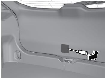
2. Turn the lever to the right to unlock the liftgate.
