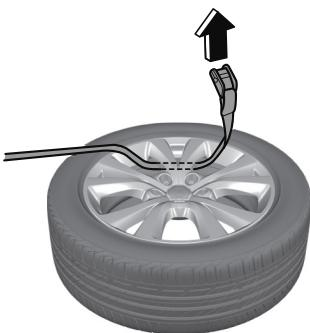
13. Thread the belt through the buckle, then pull the belt end to secure the flat tire.
