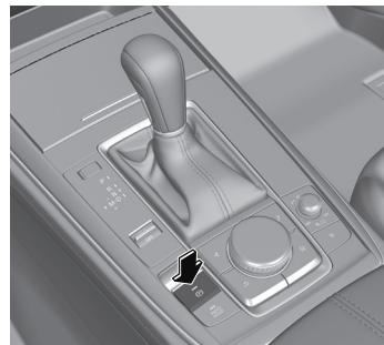
If the EPB switch is pressed without depressing the brake pedal, a message is displayed on the multi-information display to notify the driver to depress the brake pedal.
