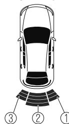
1. Right rear corner ultrasonic sensor gauge/Right rear side ultrasonic sensor gauge\*
