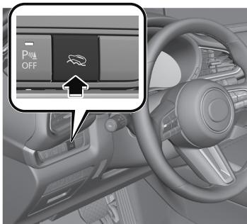
If the switch is pressed again, the Off-Road Traction Assist is stopped and the Off-Road Traction Assist indicator light turn off.
