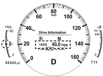
The average fuel economy and trip meters can be reset by pressing the INFO switch for 1.5 seconds or more while in each mode. After the data is cleared, the fuel consumption is recalculated and the  $\text{--- L/100 km}$  ( $\text{--- mpg}$ ) for the 30 seconds prior to it being displayed is indicated.
