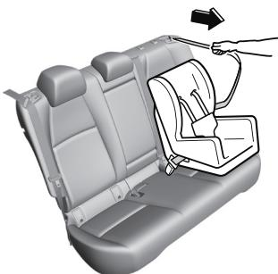
5. Push the child-restraint system firmly into the vehicle seat. Be sure the belt retracts as snugly as possible. A clicking noise from the retractor will be heard during retraction if the system is in the automatic locking mode. If the belt does not lock the seat down tight, repeat this step.
