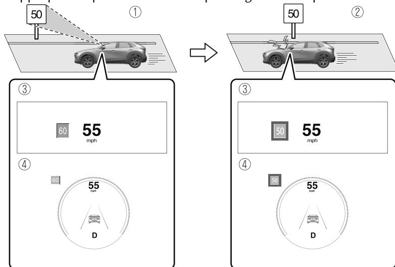
1. Vehicle is doing 55 mph when 50 mph speed limit sign is recognized.
