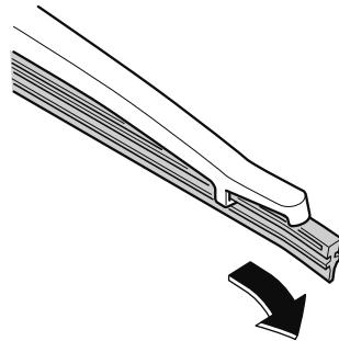
5. Remove the metal stiffeners from the blade rubber and install them in the new blade.
