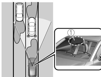
1. Forward Sensing Camera (FSC)\*<sup>1</sup>
