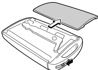
2. Press in the tab to unlock the upper cover.
