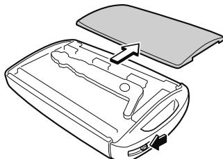
2. Remove the auxiliary key.
