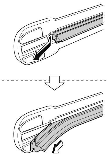
6. Insert the end of the new blade rubber into the groove of the blade holder until it contacts the end of the blade holder.
