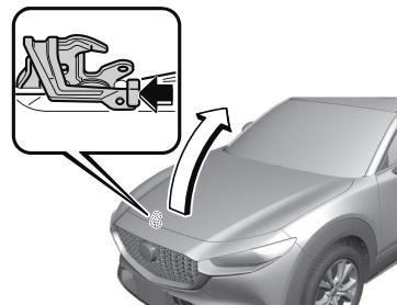
3. Grasp the support rod in the padded area and secure it in the support rod hole indicated by the arrow to hold the hood open.
