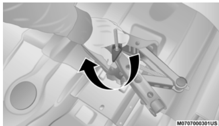
Tighten Jack Fastener
