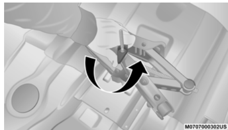
Loosen Jack Fastener
