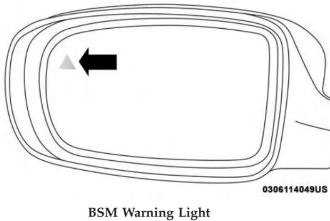
The BSM detection zone covers approximately one lane width on both sides of the vehicle 12 ft (3.8 m). The zone length starts at the outside rear view mirror and extends approximately 10 ft (3 m) beyond the rear bumper of the vehicle. The BSM system monitors the detection zones on both sides of the vehicle when the vehicle speed reaches approximately 6 mph (10 km/h) or higher and will alert the driver of vehicles in these areas.
