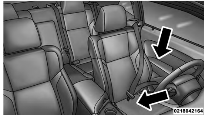
Pulling Out The Latch Plate
