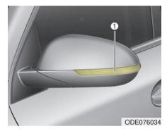
If the side repeater lamp (LED) does not operate, have the vehicle checked by an authorized Kia dealer.
