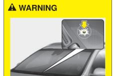
The Aux. Battery Saver+ relies on the high voltage battery to charge the 12V battery. The charging indicator lamp will blink rapidly when this is occurring. To reduce the risk of electrical shock, do not touch any high voltage components (orange) or other electrical devices while charging is occurring.
