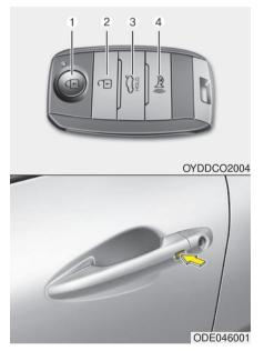
Pressing the button of the front outside door handles with all doors (and liftgate) closed and any door unlocked, locks all the doors (and liftgate).
