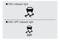
When engine start/stop button is turned to ON, the indicator light illuminates, then goes off if the ESC system is operating normally.
