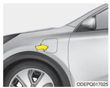
3. After unlocking doors, open the charging door by pressing it.
