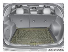
To keep items from shifting in the cargo area, you can use the holders located in the cargo area to attach the luggage net.
