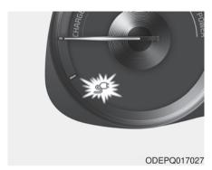
Check if the charging cable connection indicator of the high voltage battery in the instrument clus-
