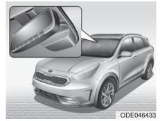
Auto defogging reduces the probability of fogging up the inside of the windshield by automatically sensing the moisture of inside the windshield. The auto defogging system operates when the heater or air conditioning is
