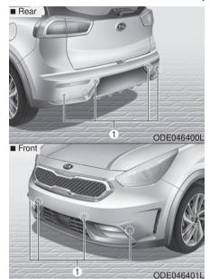
The parking assist system assists the driver during movement of the vehicle by chiming if any object is sensed within the distance of 100 cm (39 in.) in front and 120 cm (47 in.) behind the vehicle
