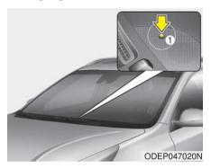
You can check the charging status at the outside of vehicle when charging or using (it is not driving status) the high-voltage battery.
