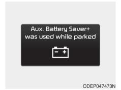
This message is displayed when the Aux. Battery Saver+ function has been completed when the vehicle is turned ON
