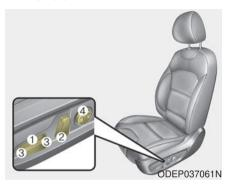
The front seat can be adjusted by using the control switches located on the outside of the seat cushion. Before driving, adjust the seat to the proper position so you can easily control the steering wheel, pedals and switches on the instrument panel.
