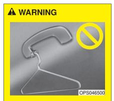
Do not hang other objects such as hangers or hard objects except clothes. Also, do not put heavy, sharp or breakable objects in the cloth pockets. In an accident or when the curtain air bag is inflated, it may cause vehicle damage or personal injury.
