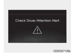
When the "Check Driver Attention Alert" warning message appears, the system is not working properly. In this case, have the vehicle inspected by an authorized Kia dealer.
