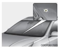
When scheduled charging is set and the normal charger or the portable charging cable (ICCB: In-Cable Control Box) is connected for charging, the indicator lamp blinks (for 3 minutes) to indicate that scheduled charging is set.
