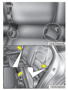
3. When folding the seat back, insert the rear seat belt buckle in the pocket between the rear seatback and cushion then make sure both seatbelts do not interfere with stowed luggage and cargo. Then, insert the seat belt into the two holes located on both sides.
