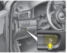
If you press the scheduled charging deactivation (()) button to immediately charge the battery, charging must be initiated 3 minutes after the charging cable has been connected.
