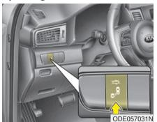
The indicator on the switch will illuminate when the Blind Spot Detection System (BSD) switch is pressed with the Engine Start/Stop Button ON.
