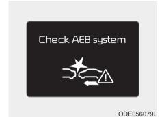
When the AEB is not working properly, the AEB warning light ( ) will illuminate and the warning message will appear for a few seconds. After the message disappears, the master warning light ( ) will illuminate. In this case, have your vehicle inspected by an authorized Kia dealer.
