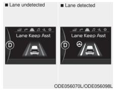
If the speed of the vehicle is over 64 km/h (40 mph) and the system detects lane markers, the color changes from gray to white. When the conditions below are met, LKAS will be enable to assist steering.
