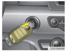
If the battery is weak or the smart key does not work correctly, you can start the engine by pressing the engine start/stop button with the smart key.
