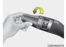
When the light switch is in the headlight position, the head, tail, license lights will turn ON.
