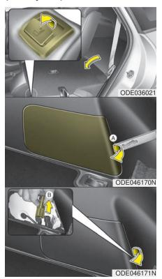
When the vehicle is under regular maintenance, make sure to separate the (-) cable inside the luggage room before maintenance.
