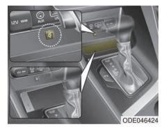
A wireless smart phone charging system located in front of the center console
