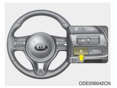
This function allows you to program the vehicle to maintain relative distance to the vehicle ahead without depressing the accelerator pedal or brake pedal. The vehicle to vehicle distance will automatically activate when the SCC is on.
