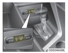
If your vehicle has an AUX and/or USB(universal serial bus) port, you can use the AUX port to connect audio devices and the USB port to plug in a USB device or iPod<sup>®</sup>.
