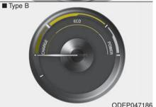
The hybrid system gauge indicates whether the current driving condition is fuel efficient or not.
