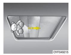
If an object or part of the body is detected while the sunroof glass automatically, it will reverse the direction, and then stop.
