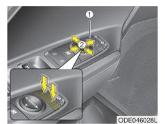
The electric remote control mirror switch allows you to adjust the position of the left and right outside rearview mirrors. To adjust the position of either mirror, press the R or L button (1) to select the right side mirror or the left side mirror, then press a corresponding point (▲) on the mirror adjustment control to position the selected mirror up, down, left or right. After adjustment, press the R or L button again to prevent the inadvertent adjustment.
