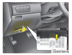
Always set the fuse switch to the ON position before using the vehicle.
