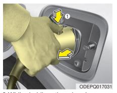
While holding the charging connector, pressing the locking release button (1) and then pull it out.
