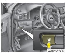
The fuel filler lid must be opened from inside the vehicle by pushing the fuel filler lid button.
