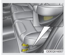
Do not put objects on the left side of rear seats. This could block the battery cooling duct causing battery degradation.
