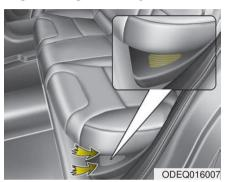
The hybrid battery air intake is located on bottom and side of the rear seats. The air intake cools down the hybrid battery. When the hybrid battery air intake is blocked, the hybrid battery may be overheated. Do not obstruct the air intake with any other objects.
