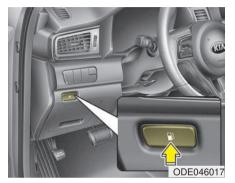
The fuel filler lid must be opened from inside the vehicle by pressing the fuel filler lid opener button.
