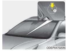
You can check the charging status at the outside of vehicle when charging or using (it is not driving status) the high-voltage battery.
