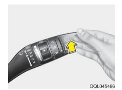
Push the lever away from you to spray rear washer fluid and to run the rear wipers 1  $\sim$  3 cycles. The spray and wiper operation will continue until you release the lever
