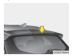
If the high mounted stop lamp (LED) does not operate, have the vehicle checked by an authorized Kia dealer.
