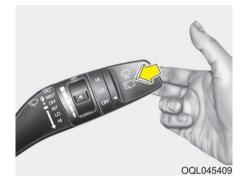
In the OFF position, pull the lever gently toward you to spray washer fluid on the windshield and to run the wipers 1-3 cycles.
