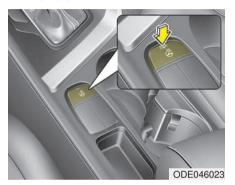
With the Engine Start/Stop button is ON position, pressing the heated steering wheel button warms the steering wheel. The indicator on the button will illuminate.
