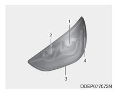
If the Low/High beam lamp (1), Low beam lamp (2), Front turn signal lamp/Position lamp(3), Side marke r(4) does not operate, have the vehicle checked by an authorized Kia dealer.
