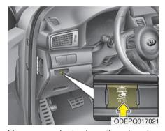
You may select when the charging connector can be locked and unlocked in the charging inlet.
