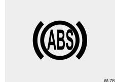
The ABS warning light will stay on for approximately 3 seconds after the engine start/stop button is ON. During that time, the ABS will go through self-diagnosis and the light will go off if everything is normal. If the light stays on, you may have a problem with your ABS. Contact an authorized Kia dealer as soon as possible.
