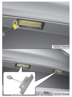
1. Using a flat-blade screwdriver, gently pry the lens cover from lamp housing.
