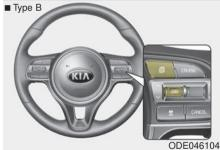
The LCD window modes can be changed by using the control buttons on the steering wheel.
