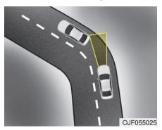
The SCC may have limits to its ability to detect distance to the vehicle ahead due to road and traffic conditions.
