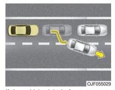
If the vehicle right in front moves to another direction, the SCC system may not sense stopped vehicle in front and may crash. Always maintain safe distance.
