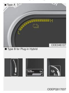
This gauge indicates the remaining hybrid battery power.
