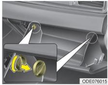
1. Open the glove box and remove the stoppers on both sides.
