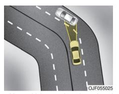
Your vehicle speed can be reduced due to a vehicle in the adjacent lane. Adjust your vehicle speed by depressing the brake pedal according to the road condition ahead and driving condition. Apply the accelerator pedal and select the appropriate set speed. Check to be sure that the road conditions permit safe operation of the SCC.
