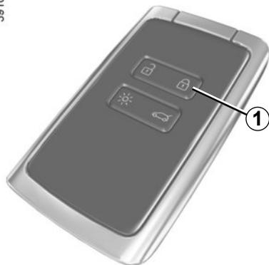
If the vehicle is equipped with a deadlocking function, this allows you to lock the opening elements and to prevent the doors from being unlocked using the interior handles (for example, by breaking the window and then trying to open the door from the inside).
