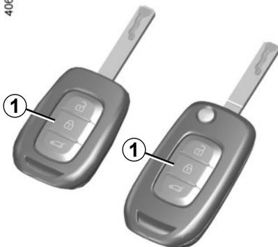
If the vehicle is equipped with a deadlocking function, this allows you to lock the opening elements and to prevent the doors from being unlocked using the interior handles (for example, by breaking the window and then trying to open the door from the inside).
