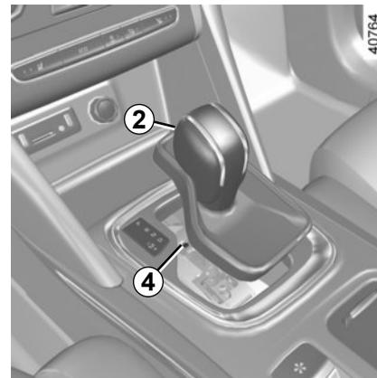
**When activated**, in the event that the lever is stuck in **P**, depress the brake paddle. It is possible to free the lever manually. To do this, unclip the base of the lever, then insert a tool (rigid rod) into the slot **4** and press simultaneously on the button **2** in order to unclick the lever.
