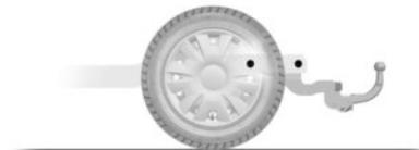
If the towbar ball obscures the registration plate or the rear fog lights, it should be removed when not in use.
