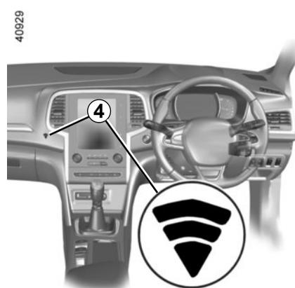
Press the brake or clutch pedal, then place the RENAULT **3** card (logo side) for around 2 seconds in contact with.
