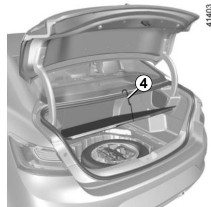
The false floor can be attached using the hook **4** in the housing **3**.
