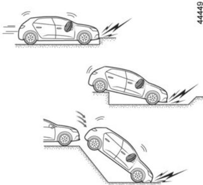
In the following examples, the pretensioners or the airbags could operate:
