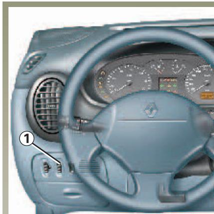
With the ignition on, press switch **1**. A indicator light will illuminate on the instrument panel.
