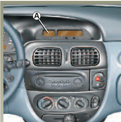
If one of the four doors is open, indicator light **5** switches on and the four doors in picture **4** are open on display **A**.
