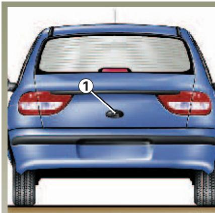
The boot lid is locked and unlocked at the same time as the doors.
