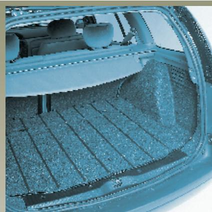
To roll up the flexible part, pull it, lifting it slightly, and allow the luggage compartment cover to roll up.
