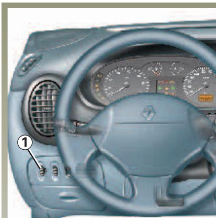
The tumblewheel **1** allows the height of the beams to be adjusted in relation to the load.
