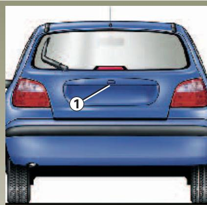
The tailgate is locked and unlocked at the same time as the doors.
