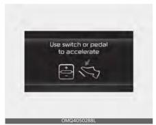
When Highway Driving Assist is operating, your vehicle will stop if the vehicle ahead of you stops. Also, if the vehicle ahead of you starts moving within 30 seconds after the stop, your vehicle will start as well. In addition, after the vehicle has stopped and 30 seconds have passed, the 'Use switch or pedal to accelerate' message will appear on the cluster. Depress the accelerator pedal or push the + switch, - switch or (| `) switch to start driving.
