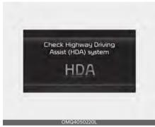
When Highway Driving Assist is not working properly, the 'Check Highway Driving Assist (HDA) system' warning message will appear, and the (\(\bigcap\)) warning light will illuminate on the cluster.
