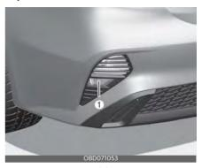
If the back up lamp (1) does not operate, have the vehicle checked by an authorized Kia dealer.
