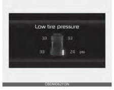
When the tire pressure monitoring system warning indicators are illuminated and warning message displayed on the cluster LCD display, one or more of your tires is significantly under-inflated.
