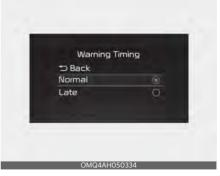
With the ignition switch or ENGINE START/STOP button in the ON position, select 'Driver Assistance → Warning
