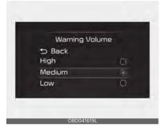
With the ignition switch or ENGINE START/STOP button in the ON position, select 'Driver Assistance → Warning Volume' from the 'User Settings (LCD display) or Setup → Vehicle (Infotainment System screen)' menu to change the Warning Volume to 'High', 'Medium' or 'Low' for Rear Cross-Traffic Collision-Avoidance Assist.
