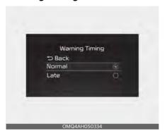
With the ignition switch or ENGINE START/STOP button in the ON position, select 'Driver Assistance → Warning Timing' from the 'User Settings (LCD display) or Setup → Vehicle (Infotainment System screen)' to change the initial warning activation time for Rear Cross-Traffic Collision Warning.
