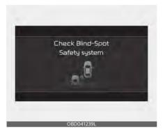
When Blind-Spot Collision-Avoidance Assist is not working properly, the 'Check Blind-Spot Safety system' warning message will appear (turns off after a certain time), and \(\bigcap\) warning light will illuminate on the cluster. In this case, have your vehicle inspected by an authorized Kia dealer.
