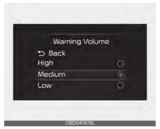
With the ignition switch or ENGINE START/STOP button in the ON position, select 'Driver Assistance → Warning Volume' from the 'User Settings (LCD display) or Setup → Vehicle (Infotainment System screen)' to change the Warning Volume to 'High', 'Medium', 'Low' for Highway Driving Assist.
