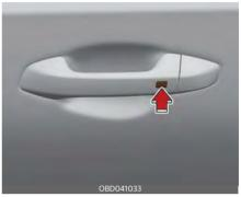
Pressing the button of the front driver side door handles with all doors (and trunk) closed and any door unlocked, locks all the doors (and trunk). If all doors (and trunk) and engine hood are closed, the hazard warning lights will blink once and the chime will sound once to indicate the vehicle is locked.
