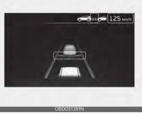
If you want to speed up temporarily when Smart Cruise Control is on, depress the accelerator pedal for a certain amount. While depressing the accelerator pedal for a certain amount, the set speed, distance level and target distance will blink on the cluster. However, if the accelerator pedal is insufficiently depressed, the vehicle may slow down.
