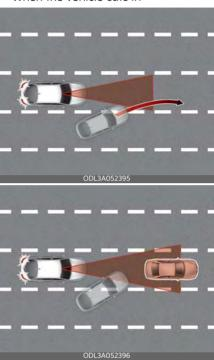
If a vehicle cuts in front of your vehicle, Leading Vehicle Departure Alert may not operate properly. When the vehicle ahead sharply steers
