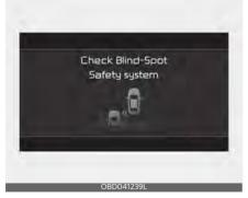
When Blind-Spot Collision Warning is not working properly, the 'Check Blind-Spot Safety system' warning message will appear on the cluster, and the function will turn off automatically, or the function will be limited. In this case, have your vehicle inspected by an authorized Kia dealer.
