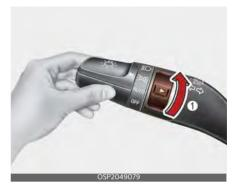
The fog lights will turn on when the fog light switch (1) is turned to the on position after the headlight is turned on. To turn off the fog lights:
