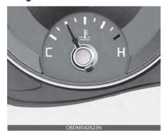
This gauge indicates the temperature of the engine coolant when the ignition switch or the ENGINE START/STOP button is ON.
