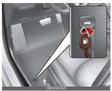
The fuel-filler door must be opened from inside the vehicle by pulling up on the fuel-filler door opener located on the front floor area on the driver's seat. If the fuel filler door does not open because ice has formed around it, tap lightly or push on the door to break the ice and release the door. Do not pry on the door. If necessary, spray around the door with an approved de-icer fluid (do not use radiator anti-freeze) or move the vehicle to a warm place and allow the ice to melt.
