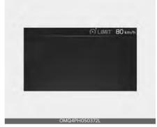
The set speed limit will be displayed on the cluster. If you would like to drive over the preset speed limit, depress the accelerator pedal beyond the pressure point to activate the kickdown function.
