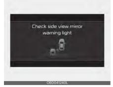
When the warning light on the side view mirror (outside mirror) is not working properly, the 'Check side view mirror warning light' warning message will
