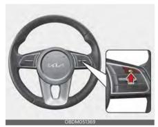
Press the Driving Assist button to turn Smart Cruise Control off.
