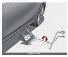
9. Loosen the wheel nuts and remove them with your fingers. Slide the wheel off the studs and lay it flat so it cannot roll away. To put the wheel on the hub, pick up the spare tire, line up the holes with the studs and slide the wheel onto them.
