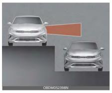
Blind-Spot Collision Warning may not operate properly when driving where the heights of the lanes are different. The function may not detect the vehicle on a road with different lane heights (underpass joining section, grade separated intersections, etc.).
