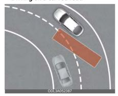
Blind-Spot Collision Warning may not operate properly when driving on a
