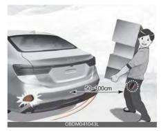
If you are positioned in the detecting area ( $50 \sim 100$  cm ( $20 \sim 40$  inches) behind the vehicle) carrying a smart key, the hazard warning lights will blink and chime will sound to alert you the smart key has been detected and the trunk will open.
