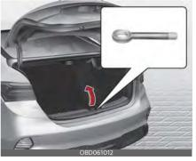
Remove the hole cover pressing the lower (front) part of the cover on the bumper.
