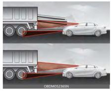
In the following cases, the vehicle in front cannot be detected by the sensor:
