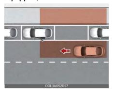
After the vehicle stops, when an approaching vehicle from the rear area is detected after a passenger opens the door, Safe Exit Warning will warn the driver with a warning message and an audible warning to help prevent a collision.
