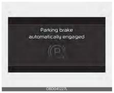
If the driver turns the engine off by mistake while Auto Hold (if equipped) is operating, EPB will be automatically applied. But if the driver turns the engine off and pushes the EPB switch for 1 second, the EPB does not apply.
