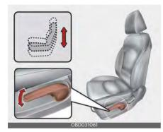
To change the height of the seat, push the lever upwards or downwards.
