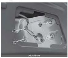
Remove the rear combination lamp assembly from the body of the vehicle.
