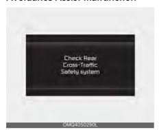
When Rear Cross-Traffic Collision-Avoidance Assist is not working properly, the 'Check Rear Cross-Traffic Safety system' warning message will appear (turns off after a certain time), and the warning light will illuminate on the cluster. In this case, have your vehicle inspected by an authorized Kia dealer.
