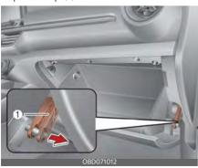
Remove the climate control air filter cover while pressing the lock on the left side of the cover.
