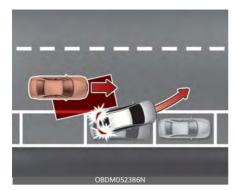
When changing lanes by detecting the lane ahead, if Blind-Spot Collision-Avoidance Assist judges that there is a collision risk with an approaching vehicle in the blind spot, it can help avoid collisions by applying the differential brake.
