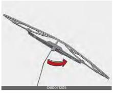
2. Compress the clip (1) and slide the blade assembly (2) downward.
