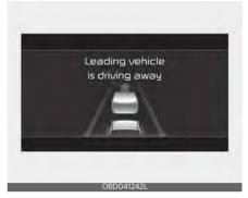
When a detected vehicle in front departs from a stop, Leading Vehicle Departure Alert will inform the driver by displaying the 'Leading vehicle is driving away' message on the cluster and an audible warning will sound.
