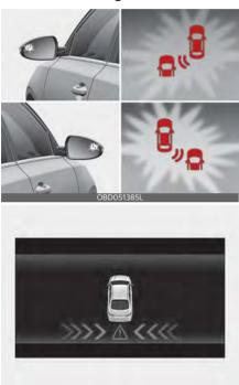
To warn the driver of an approaching vehicle from the rear left/right side of your vehicle, the side view mirror will blink and a warning will appear on the cluster. At the same time, an audible warning will sound. If Rear View Monitor is operating, a warning will also appear on the infotainment screen.
