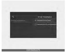
With the ignition switch or ENGINE START/STOP button in the ON position, select 'Driver Assistance → Driving Convenience' from the 'Setup' menu to set whether to use each function.
