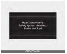
When the rear bumper around the rear corner radar or sensor is covered with foreign matters, such as snow or rain, or installing a trailer or carrier, it can reduce the detecting performance and temporarily limit or disable Rear Cross-Traffic Collision-Avoidance Assist.
