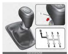
The shift lever can be moved without pushing the button (1).
