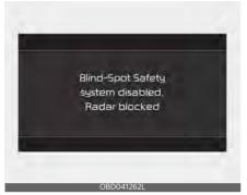
When the rear bumper around the rear corner radar or sensor is covered with foreign matters, such as snow or rain, or installing a trailer or carrier, it can reduce the detecting performance and temporarily limit or disable Safe Exit Warning. If this occurs, the 'Blind-Spot Safety system disabled. Radar blocked' warning message will appear on the cluster. Safe Exit Warning will operate properly when such foreign matters or trailer, etc., is removed, and then the engine is restarted.
