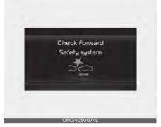
When Forward Collision-Avoidance Assist is not working properly, the 'Check Forward Safety system' warning message will appear (turns off after a certain time), and the and and warning lights will illuminate on the cluster. In this case, have the vehicle inspected by an authorized Kia dealer.
