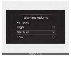
With the ignition switch or ENGINE-START/STOP button in the ON position, select 'Driver Assistance → Warning Volume' from the 'User Settings (LCD display) or Setup → Vehicle (Infotainment System screen)' to change the Warning Volume to 'High', 'Medium', 'Low' for Rear Cross-Traffic Collision Warning. If you change the Warning Volume, the Warning Volume of other Driver Assistance systems may change.
