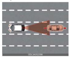
If the vehicle in front abruptly departs, Leading Vehicle Departure Alert may not operate properly.  When a pedestrian or cyclist is between you and the vehicle ahead
