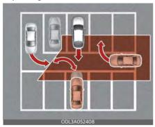
Rear Cross-Traffic Collision-Avoidance Assist may detect vehicles which are parking or pulling out near your vehicle (for example, a vehicle leaving beside your vehicle, a vehicle parking or pulling out in the rear area, a vehicle approaching your vehicle making a turn, etc.). If this occurs, the function may unnecessarily warn the driver and control the brake.
