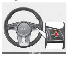
Press the Driving Assist button to turn Cruise Control off. The Cruise indicator will go off.
