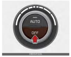
Press the OFF button to turn off the air climate control system. However, you can still operate the mode and air intake buttons as long as the ignition switch or the ENGINE START/STOP button is in the ON position.
