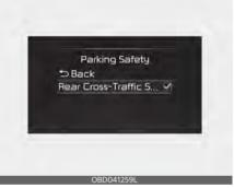
With the ignition switch or ENGINE START/STOP button in the ON position, select 'Driver Assistance → Parking Safety → Rear Cross-Traffic Safety' from the 'User Settings (LCD display) or Setup → Vehicle (Infotainment System screen)' menu to turn on Rear Cross-Traffic Collision Warning and deselect to turn off the function.
