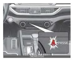
As a reminder to the front passenger, the front passenger's seat belt warning lights will illuminate for approximately 6 seconds each time you turn the ignition switch or the ENGINE START/STOP button in ON regardless of belt fastening. If the front passenger continue not to fasten the seat belt and drives below 20km/h, the warning light will stay illuminated.
