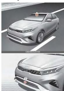
[1]: Front view camera, [2]: Front radar The front view camera and front radar are used as a detecting sensor to detect vehicles in front. Refer to the picture
