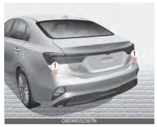
[1]: Rear corner radar Refer to the picture above for the detailed location of the detecting sensor.
