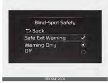
With the ignition switch or the ENGINE START/STOP button in the ON position, and select 'User Settings (LCD display) or Settings → Vehicle (Infotainment System screen) → Driver Assistance → Blind-Spot Safety → Safe Exit Warning' to turn on Safe Exit Warning and deselect to turn off the function.
