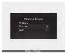
With the ignition switch or ENGINE START/STOP button in the ON position, select 'Driver Assistance → Warning Timing' from the 'User Settings (LCD display) or Setup → Vehicle (Infotainment System screen)' menu to change the initial warning activation time for Blind-Spot Collision-Avoidance Assist. When the vehicle is first delivered, Warning Timing is set to 'Normal'. If you change the Warning Timing, the Warning Timing of other Driver Assistance systems may change.
