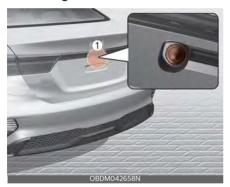
[1]: Wide-rear view camera Refer to the picture above for the detailed location of the detecting sensor.
