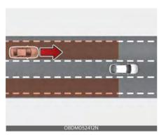
Blind-Spot Collision Warning helps detect and informs the driver that a vehicle is approaching at high speed from the blind spot area.
