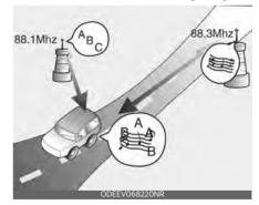
Multi-Path Cancellation - Radio signals being received from several directions can cause distortion or fluttering. This can be caused by a direct and reflected signal from the same
