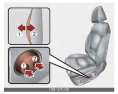
The lumbar support can be adjusted by pressing the lumbar support switch on the side of the seat.
