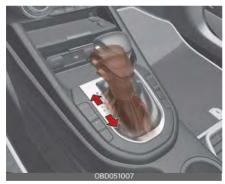
Whether the vehicle is stationary or in motion, manual mode is selected by pushing the shift lever from the D (Drive) position into the manual gate. To return to D (Drive) range operation, push the shift lever back into the main gate.
