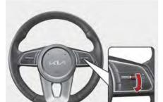
Push the + switch up or - switch down and hold it. The speed will increase or decrease to the nearest multiple of ten (multiple of five in mph) at first, and then increase or decrease by 10 km/h (5 mph).
