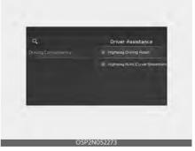
With the ignition switch or ENGINE START/STOP button in the ON position, select 'Driver Assistance → Driving Convenience → Highway Auto Curve Slowdown' from the 'Setup → Vehicle (Infotainment System screen)' menu to set whether to use each function.
