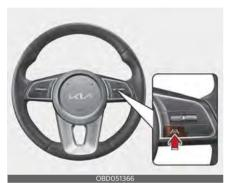
With the ignition switch or ENGINE START/STOP button in the ON position, press and hold the Lane Driving Assist button ( ) located on the steering wheel to turn off Lane Keeping Assist. Press and hold the button again to turn on the function.
