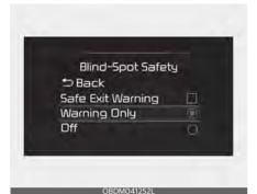
With the ignition switch or ENGINE START/STOP button in the ON position, select or deselect 'User Settings (LCD display) or Setup  $\rightarrow$  Vehicle (Infotainment System screen)  $\rightarrow$  Driver Assistance  $\rightarrow$  Blind-Spot Safety' to set whether to use each function.
