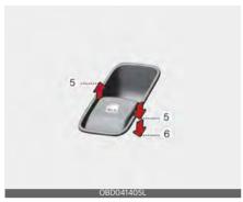
Pressing the power window switch momentarily to the second detent position (6) completely lowers the window even when the switch is released. To stop the window at the desired position while the window is in operation, pull up the switch momentarily to the opposite direction of the window movement.
