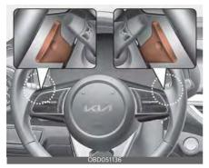
The paddle shifter is available when the shifter lever is the D (Drive) position or the manual mode.
