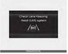
When Lane Keeping Assist is not working properly, the 'Check Lane Keeping Assist (LKA) system', warning message will appear and the yellow ( ) indicator light will illuminate on the cluster. In this case, have the function inspected by an authorized Kia dealer.
