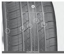
This shows there is less than 1.6 mm (1/16 inch) of tread left on the tire. Replace the tire when this happens.
