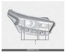
If the position lamp/daytime running lamp (LED) (1) does not operate, have the vehicle checked by an authorized Kia dealer.
