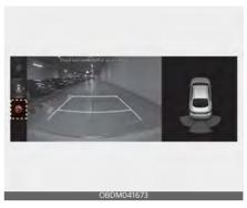
You can change Rear View Monitor 'Display Contents' of 'Display Settings' by touching the setup icon (♠) on the screen while Rear View Monitor is operating, or selecting 'Setup → Vehicle → Driver Assistance → Parking Safety → Camera Settings' from the Infotainment System screen while the engine is on.
