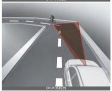
The front view camera or radar sensor recognition function may not detect the vehicle, pedestrian or cyclist traveling in front on a curved road.
