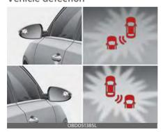
To warn the driver a vehicle is detected, the warning light on the side view mirror will illuminate.  Blind-Spot Collision-Avoidance Assist will operate when your vehicle speed is above 20 km/h (12 mph) and the speed of the vehicle in the blind spot area is above 10 km/h (7 mph).
