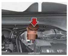
1. Before removing the reservoir cap and adding brake/clutch fluid, clean the area around the reservoir cap thoroughly to prevent brake/clutch fluid contamination.
