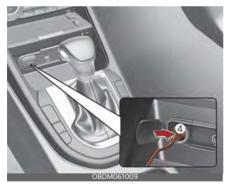
10. With the ignition switch or ENGINE START/STOP button position on: switch on the compressor and let it run for approximately 5~7 minutes to fill the sealant up to proper pressure. (Refer to "Tires and wheels" on page 7-36.) Be careful not to overinflate the tire and stay away from the tire when filling it. When the tire and wheel are damaged, do not use Tire Mobility Kit for your safety.
