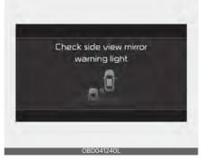
When the outside rear view mirror warning light is not working properly, the 'Check side view mirror warning light' warning message will appear on the cluster for several seconds, and the master ( ) warning light will appear on
