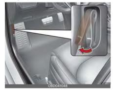
Open the hood after turning off the engine on a flat surface, shifting the shift lever to the P (Park, for Dual Clutch Transmission/ Intelligent Variable Transmission) or first gear or R (Reverse, for Manual Transmission) and set the parking brake.
