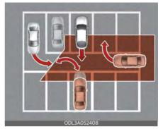
Rear Cross-Traffic Collision Warning may detect vehicles which are parking or pulling out near your vehicle (for example, a vehicle leaving beside your vehicle, a vehicle parking or pulling out in the rear area, a vehicle approaching your vehicle making a turn, etc.). If this occurs, the function may unnecessarily warn the driver.
