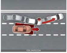
When you are driving forward out of a parking space, if Blind-Spot Collision-Avoidance Assist judges that there is a collision risk with an approaching vehicle in the blind spot, it can help avoid collisions by applying the brake.
