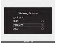
With the ignition switch or ENGINE START/STOP button in the ON position, select 'Driver Assistance → Warning Volume' from the 'User Settings (LCD display) or Setup → Vehicle (Infotainment System screen)' menu to change the Warning Volume to 'High', 'Medium' or 'Low' for Lane Keeping Assist.
