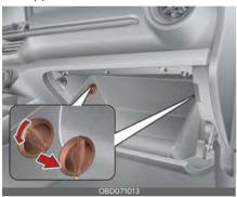
2. With the glove box open, pull the support strap (1).
