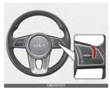
To resume Manual Speed Limit Assist after the function was canceled, push the +, - or (Pause/Resume symbol) switch. If you push the + switch up or - switch down, set speed will be set to the current speed on the cluster. If the current speed of the vehicle is less than 30 km/h (19 mph), the set speed will set as 30 km/h (19 mph). If you press the
