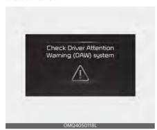
When Driver Attention Warning is not working properly, the 'Check Driver Attention Warning (DAW) system' warning message will appear on the cluster (turns off after a certain time) and \(\binom{\text{N}}{\text{N}}\) warning light will illuminate. In this case, have your vehicle inspected by an authorized Kia dealer.
