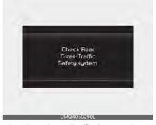
When Rear Cross-Traffic Collision Warning is not working properly, the 'Check Rear Cross-Traffic Safety system' warning message will appear on the cluster,
