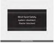
When the rear bumper around the rear corner radar or sensor is covered with foreign material, such as snow or rain, or installing a trailer or carrier, it can reduce the detecting performance and tempo-
