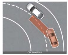
Blind-Spot Collision Warning may not operate properly when driving on the curved road. The function may recognize the vehicle in the same lane.
