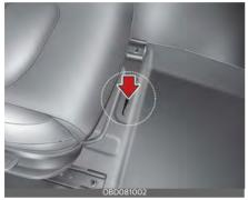
The number is punched on the floor under the passenger seat. To check the number, open the cover.
