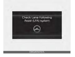
When Lane Following Assist is not working properly, the 'Check Lane Following Assist (LFA) system' warning message will appear on the cluster (turns off after a certain time) and the \( \bigcite{1} \) warning light will illuminate. In this case, have the function checked by an authorized Kia dealer.
