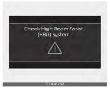
When High Beam Assist is not working properly, the warning message will come on for a few seconds. After the message disappears, the master warning light (\hat{\Lambda}) will illuminate.
