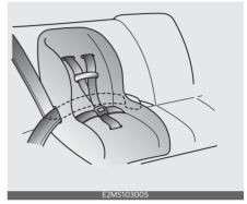
Since all passenger seat belts move freely under normal conditions and only lock under extreme or emergency conditions (emergency locking mode), you must manually pull the seat belt all the way out to shift the retractor to the "Automatic Locking" mode to secure a child restraint.
