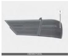
If the side marker (LED) (1) does not operate, have the vehicle checked by an authorized Kia dealer. The LED lamp cannot be replaced as a single component because it is an integrated unit. The LED lamp has to be replaced with the unit. A skilled technician should check or repair the side marker (LED), for it may damage related parts of the vehicle.
