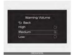
With the ignition switch or ENGINE START/STOP button in the ON position, select 'Driver Assistance → Warning Volume' from the 'User Settings (LCD display) or Setup → Vehicle (Infotainment System screen)' to change the Warning Volume to 'High', 'Medium', 'Low' for Blind-Spot Collision Warning.
