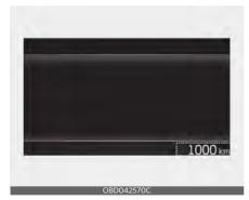
The odometer Indicates the total distance that the vehicle has been driven and should be used to determine when periodic maintenance should be performed.
