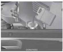
Use a funnel to help prevent oil from being spilled on engine components. Use only the specified engine oil. (Refer to "Recommended lubricants and capacities" on page 8-7.)
