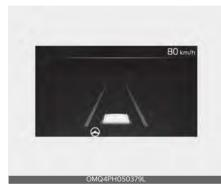
If the vehicle ahead or both lane markings are detected and your vehicle speed is below 180 km/h (110 mph), the green ( ) indicator light will illuminate on the cluster, and the function will help center the vehicle in the lane by controlling the steering wheel.
