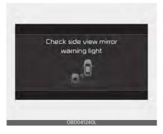
When the warning light on the side view mirror is not working properly, the 'Check side view mirror warning light' warning message will appear (turns off after a certain time), and \( \frac{1}{2} \) warning light will illuminate on the cluster. In this case, have your vehicle inspected by an authorized Kia dealer.
