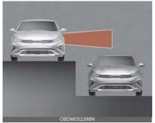
Blind-Spot Collision-Avoidance assist may not operate properly when driving where the heights of the lanes are different. The function may not detect the vehicle on a road with different lane heights (underpass joining section, grade separated intersections, etc.). Always pay attention to road and driving conditions while driving.
