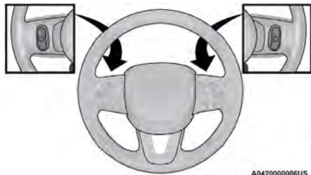
Remote Sound System Controls
