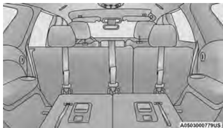
Seven Passenger Top Tether Strap Mounting (2nd Row Bench)
