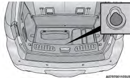
Winch Plug Location
